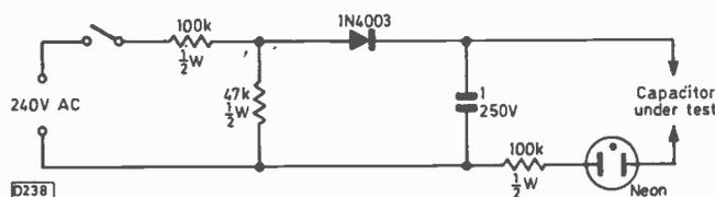
Fig. 1: Suggested simple capacitor tester circuit.
