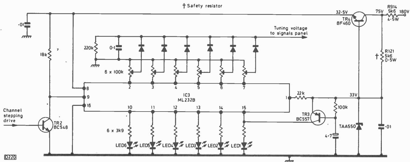
Fig. 1: Channel selection circuit, Fidelity Model CTV14R.
