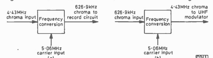
Fig. 28: Basic chroma signal processing, (a) on record, (b) on playback.
