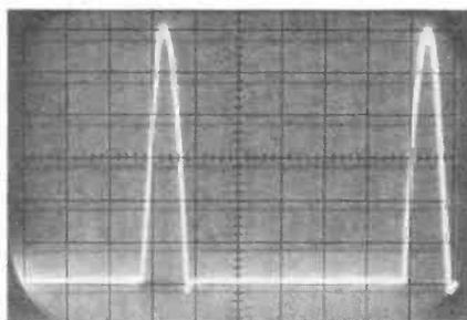
8: Anode of SCR1, timebase board. 1.2kV peak-to-peak.
