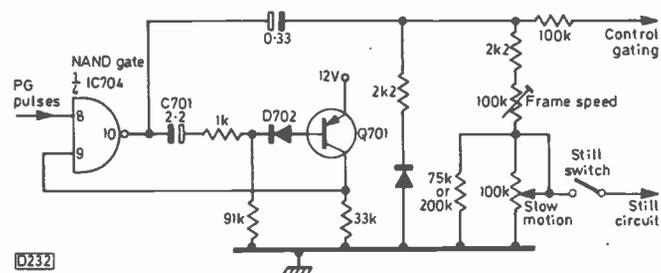
Fig. 2: Divide-by-four monostable multivibrator circuit used on the SJ-1 panel in the Sony C7.
