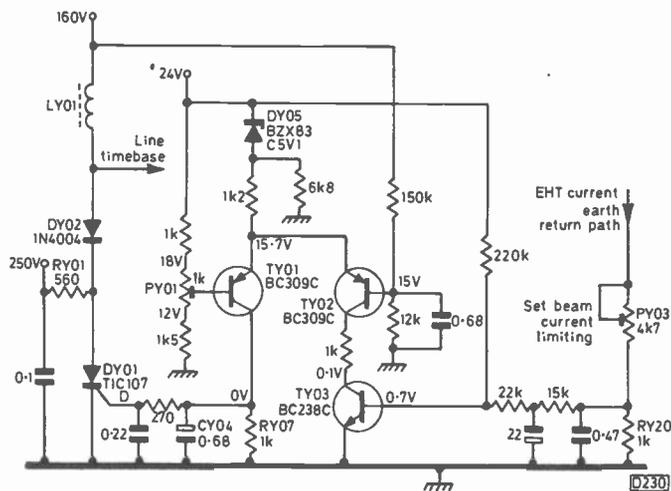
Fig. 4: The electronic trip circuit.
