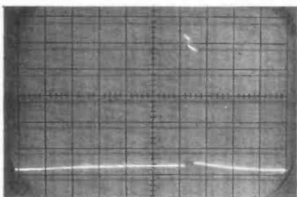
10: Pin 3 of IC2, timebase board. 24V peak-to-peak.
