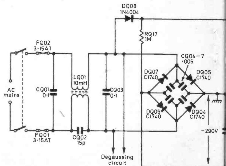
Fig. 1: The mains input and switch
