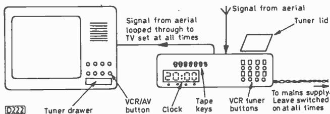
Fig. 1 (left): Elements of a simple video installation.
