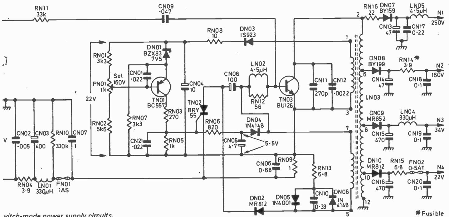
switch-mode power supply circuits.
