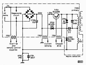
Fig. 2: Simplified circuit showing the mains input and chopper power supply arrangements. The chopper transformer T705 has a diode-split secondary to provide the e.h.t.
