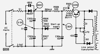
Fig. 1: Power supply arrangements used in the Indesit T12LGB monochrome portable, showing the mains input and rectifier, the start-up circuit and the pump transistor Tr902.
