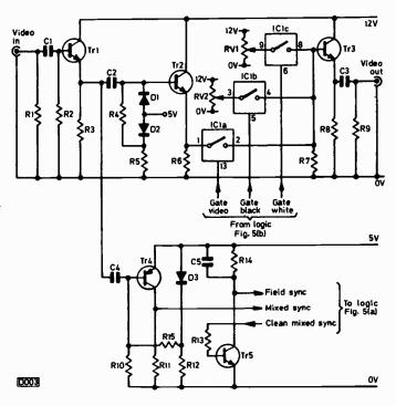
Fig. 6: Circuitry on the video board.
