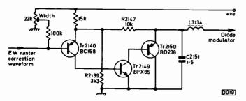
Fig. 3: A triple Darlington configuration, with pnp and npn transistors, used to provide the EW modulator drive with a 20AX tube (Philips G11 chassis).
