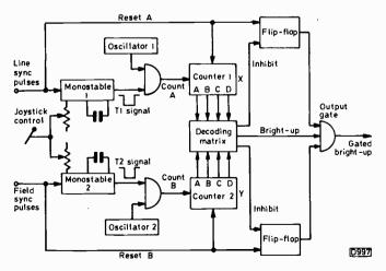
Fig. 2: Simplified diagram showing the logic required to produce a right-pointing arrow.
