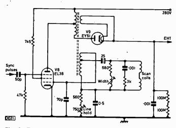
Fig. 2: The single-valve (plus e.h.t. rectifier) line timebase circuit used in the CN390 series.
