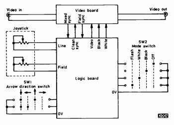
Fig. 7: Interconnections between the video and logic boards.
