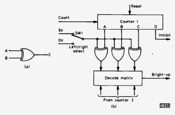
Fig. 3 (above): (a) NEV gate symbol. (b) Modification to the basic system to give left/right pointing arrows.
