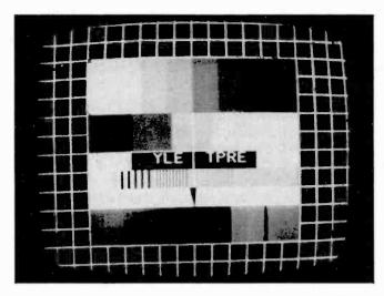
Fubk test pattern used by Finland, with Tampere identification (ch. E2). Photo from Petri Pöppönen.
