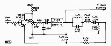
Fig. 5: Simplified circuit showing the way in which NS raster correction is carried out in the Thorn 4000 chassis. The signal developed across R411 is also used as feedback in the field timebase and is fed to the convergence circuits.
