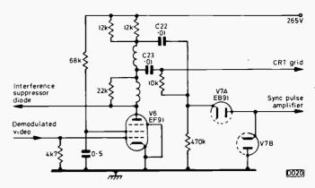
Fig. 1: The video output and diode sync separator stages used in the CN370.
