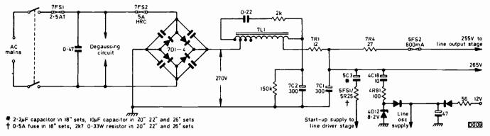
Fig. 2: The mains input, h.t. and start-up circuits used in the Rank Z718 solid-state colour chassis. The mains bridge rectifier 7D1-4 produces the h.t. supply, stabilisation being carried out via the EW modulator circuit.
