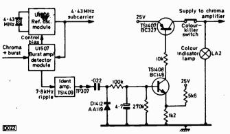
Fig. 1: Ident/colour-killer arrangement used in the Philips N1500 VCR.
