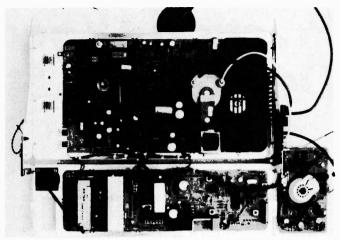
The Thorn TX10 chassis, with the signals section at the bottom in the hinged down position. The mains-live section is beneath the plastic cover shown at the top right.
