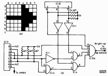
Fig. 10: Decoding circuit for an arrow with a closed head.
