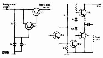
Fig. 1 (left): Darlington pair of transistors in a simple voltage regulator circuit without feedback. The output is stabilised at 1.4V less than the voltage, set by zener diode D1, at the base of Tr1. The circuit acts as an active filter, since the value of C1 is much less than would otherwise be necessary to provide
