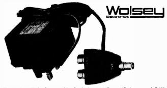
The Wolsey 'Twin Set' provides 2 wideband UHF amplified outputs (+7dB) with a low noise figure (3.5dB) from a single aerial and is intended for the '2 set household'.
