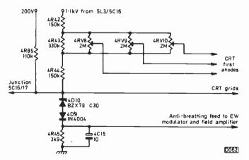
Fig. 6: The first anode supply and beam limiter circuit. The e.h.t. current returns to chassis via 4R42-4/4D10/4D9/4R45, 4R85 providing bias for 4D10. In the event of excessive e.h.t. current, 4D10 ceases to conduct and the negative voltage then present at the junction of 4R44/4R85 is applied to the c.r.t. grids, biasing back the tube. E.H.T. variations are sensed across 4R45, which provides an anti-breathing signal for the line and field timebases. 4R85 later changed to  $150k\Omega$ .
