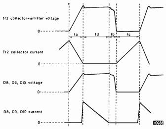
Fig. 1: Self-oscillating switch-mode power supply waveforms.
