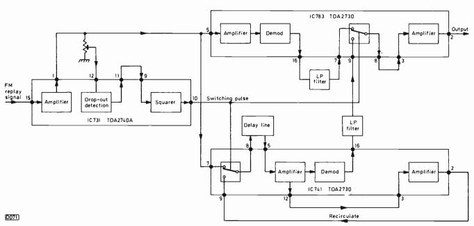
Fig. 1: The luminance playback/drop-out compensation system used in the Grundig  $2 \times 4$  VCR. When a drop-out occurs, the f.m. playback signal envelope collapses. This is detected by IC731, which produces a switching signal at pin 10 to operate the electronic switches in IC783 and IC741. As a result, the signal is obtained from the  $64\mu$  sec delay line. In the event of a sustained drop-out (longer than one line), the signal is recirculated via pins 12, 3, 2, 9 and 8 of IC741.
