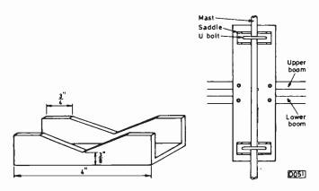
Fig. 6: Method of clamping the aerial to the mast.
