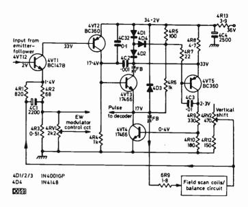
Fig. 2: field driver and output stage circuit.
