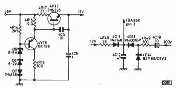
Fig. 4 (left): The 12V regulator circuit.
