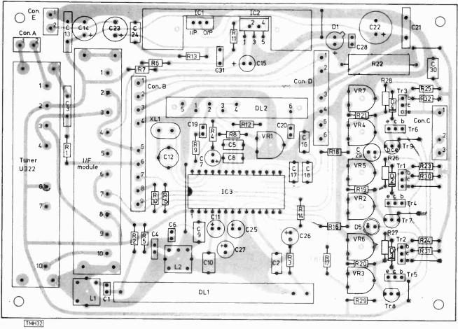
Fig. 2: The copper pattern (top) and component location diagram (bottom).
