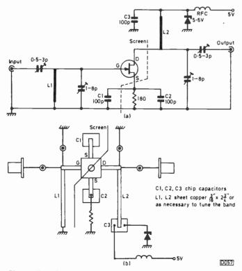
Fig. 1: Experimental gallium-arsenide f.e.t. u.h.f. preamplifier constructed by Jerry Pulice. (a) Circuit. (b) Layout.
