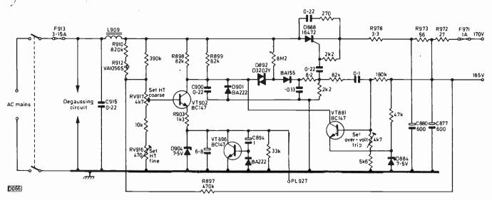
Fig. 3: Regulated power supply circuit used in the Pye 725 etc. chassis. If the zener diodes need to be replaced, use type BZX79C7V5. To reduce drift and improve the regulation, the following modifications were introduced in late production: R898/899 changed to  $56k\Omega$ , 1W; R910/R912 deleted; R897 changed to  $330k\Omega$  and R903 to  $680\Omega$ ; an  $82k\Omega$ , 1W resistor (R929) added between the collector of VT896 and the cathode of the thyristor D888.
