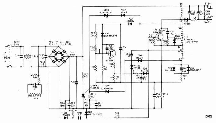
Fig. 1: Circuit of the self-oscillating switch-mode power supply (type T114A).
