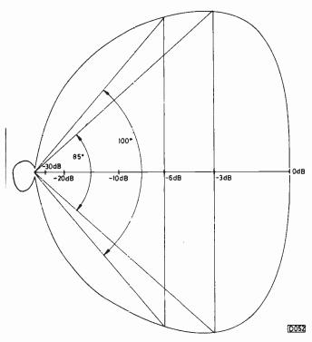
Fig. 7: Polar response at 94-9MHz.
