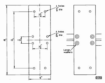
Fig. 5: Centre support/mounting plate.
