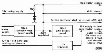
Fig. 1: Power supply arrangements, Rank T20/T22 chassis.
