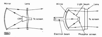
Fig. 1 (left): The basic Schmidt optical system.
