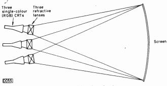
Fig. 3: Use of three tubes with refractive lenses.
