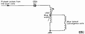
Fig. 1: The blue lateral convergence circuït used in the Thorn 9800 chassis.
