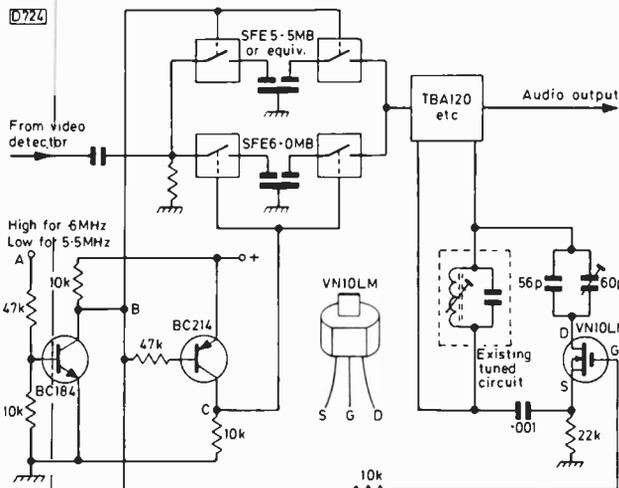
Fig. 2: 5.5/6MHz switched sound circuit with a 4066 selecting one or other ceramic input filter and a small power MOSFET switching in or out extra capacitance in the detector tuned circuit – the exact value of the added capacitance will depend on the existing detector circuit.
