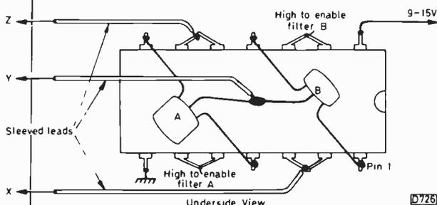
Fig. 4: Solder the filters directly to the pins of the 4066, on its underside. Wires X, Y and Z can then be inserted in the holes used by the original filter – their stiffness will support the assembly above the board. Keep the connecting wires as short as possible.
