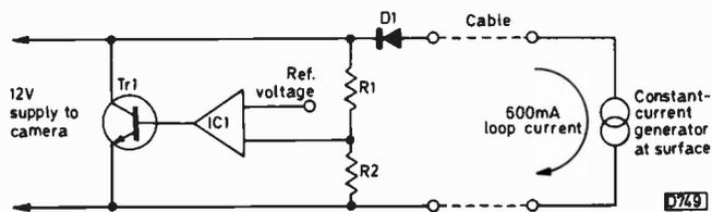
Fig. 2: Constant-current system with shunt regulator.
