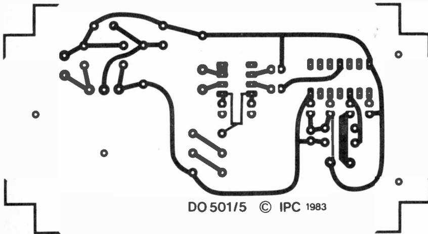
Fig. 3 (above): Prescaler 2 board track pattern (scale 1:1).
