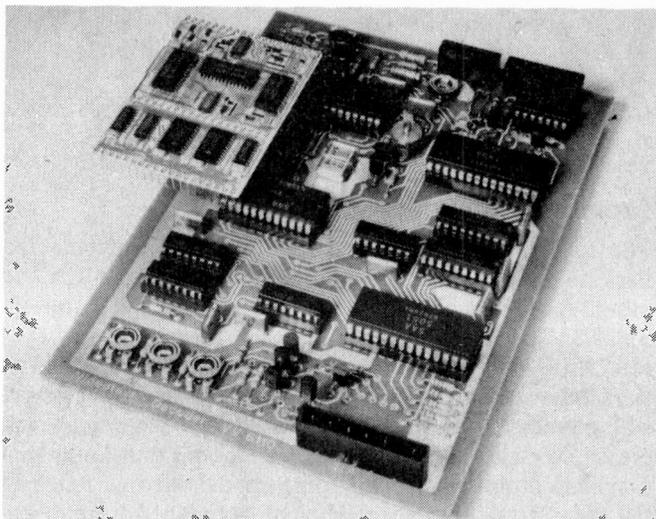
*Comparison between a teletext decoder using conventional through-panel component mounting and the equivalent using surface mounting technology.*
