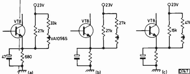
Fig. 6: Field oscillator bias circuit modifications. (a) Early. (b) With circuit shown in Fig. 4. (c) With Fig. 5.
