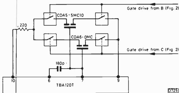
Fig. 3: Use of a second 4066 when ceramic filters are used in the detector circuit.
