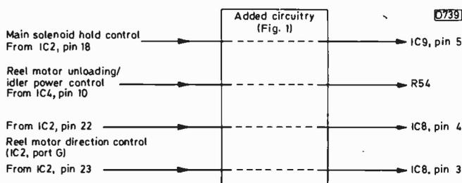
Fig. 3: Connections to the pulse stretcher circuit.
