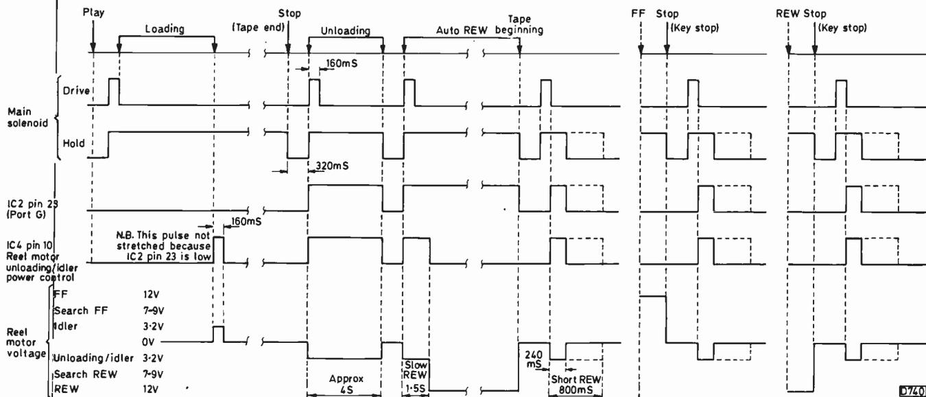
Fig. 4: Timing diagram for various control functions.
