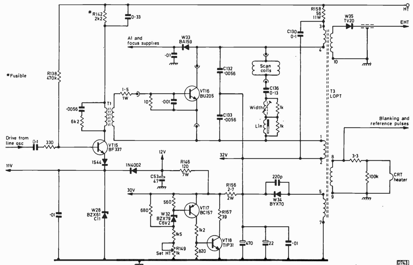
Fig. 2: The line driver and output stage circuits, with shunt regulator VT17/VT18 and associated components.
