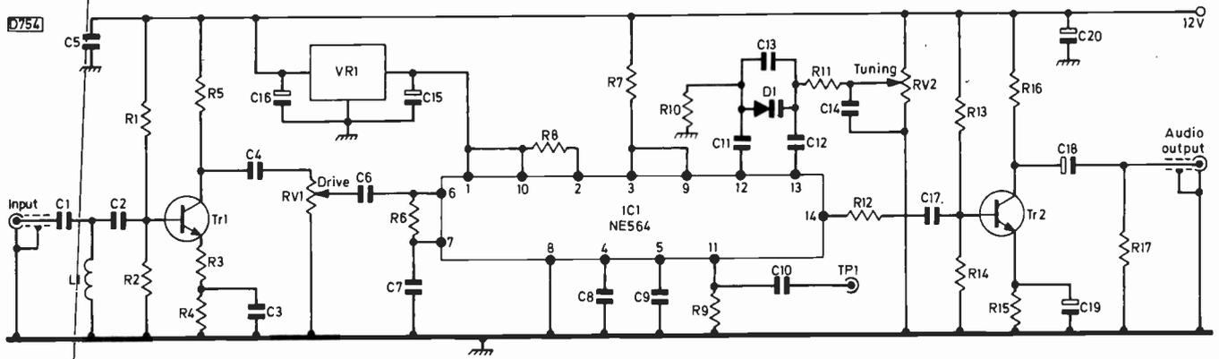
Fig. 8: The PLL sound detector circuit.
