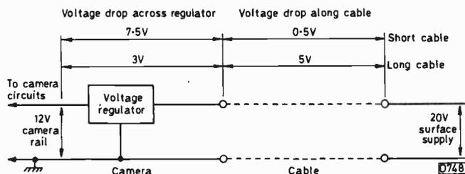
Fig. 1: Constant-voltage supply arrangement.
