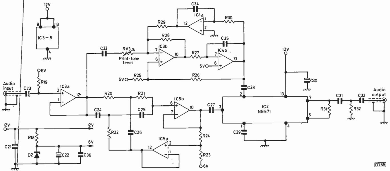
Fig. 9: Audio expander circuit.
