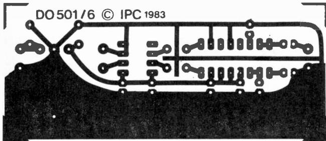
Fig. 5: Prescaler 3 board track pattern (scale 1:1).
