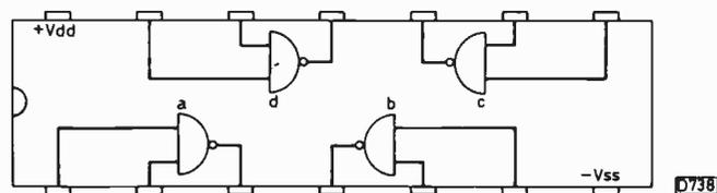
Fig. 2: Pin connections for the 4011 gate i.c.
