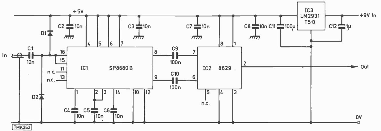
Fig. 2: Circuit diagram, prescaler 3.
