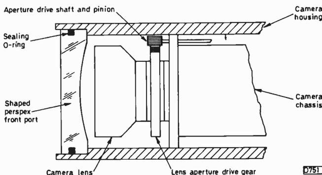
Fig. 4: Underwater camera port and optical arrangements.
