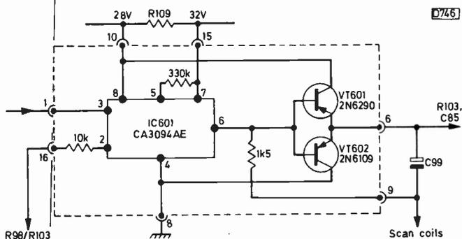
Fig. 5: Final field amplifier/output circuit using module.
