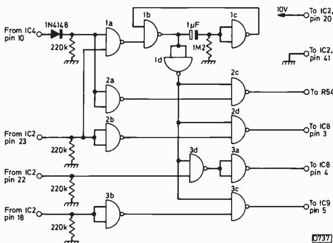
Fig. 1: Pulse stretcher circuit for the JVC HR7300EK.
