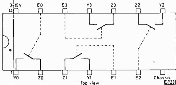
Fig. 1: Pin connections for the 4066 switch i.c. Pins E0-E3 are the control terminals for the four switches.
