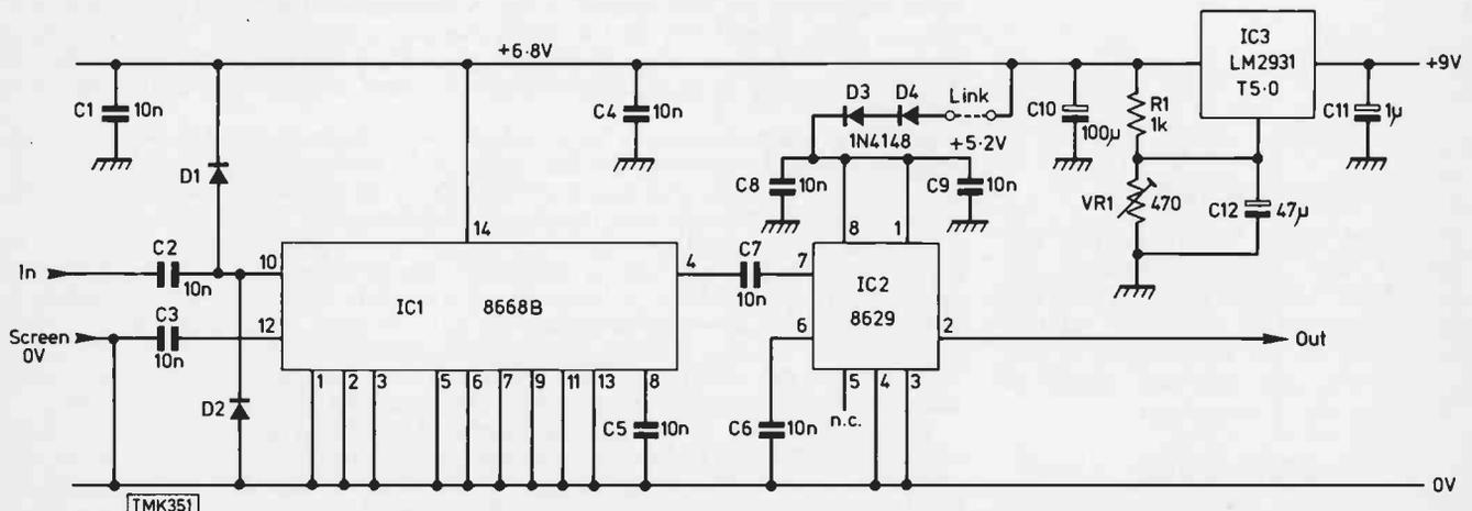
Fig. 1: Circuit diagram, prescaler 2.
