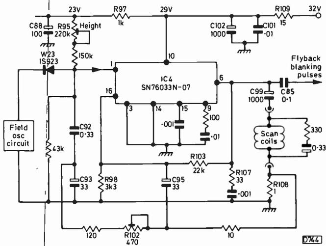
Fig. 3: Field amplifier/output circuit used in early sets.
