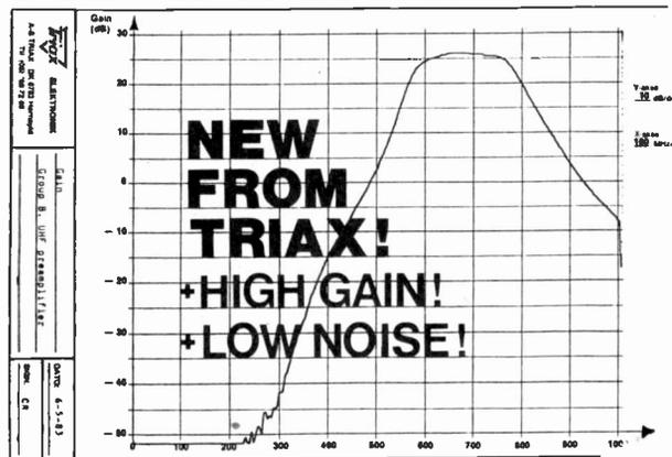
NEW FROM TRIAX - the 2000 range of low noise masthead UHF group amplifiers, high gain (26dB) with low noise (2.2dB typ) within the prescribed groups (A,B,C/D) and sharp cut-off in adjacent groups - ideal for fringe area use and 'non-local' group amplification. The lowest noise UK group amplifier now on the UK market with the high quality expected from Triax equipment.
