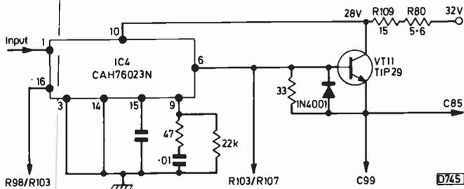
Fig. 4: Modified field output circuit with VT11 added.
