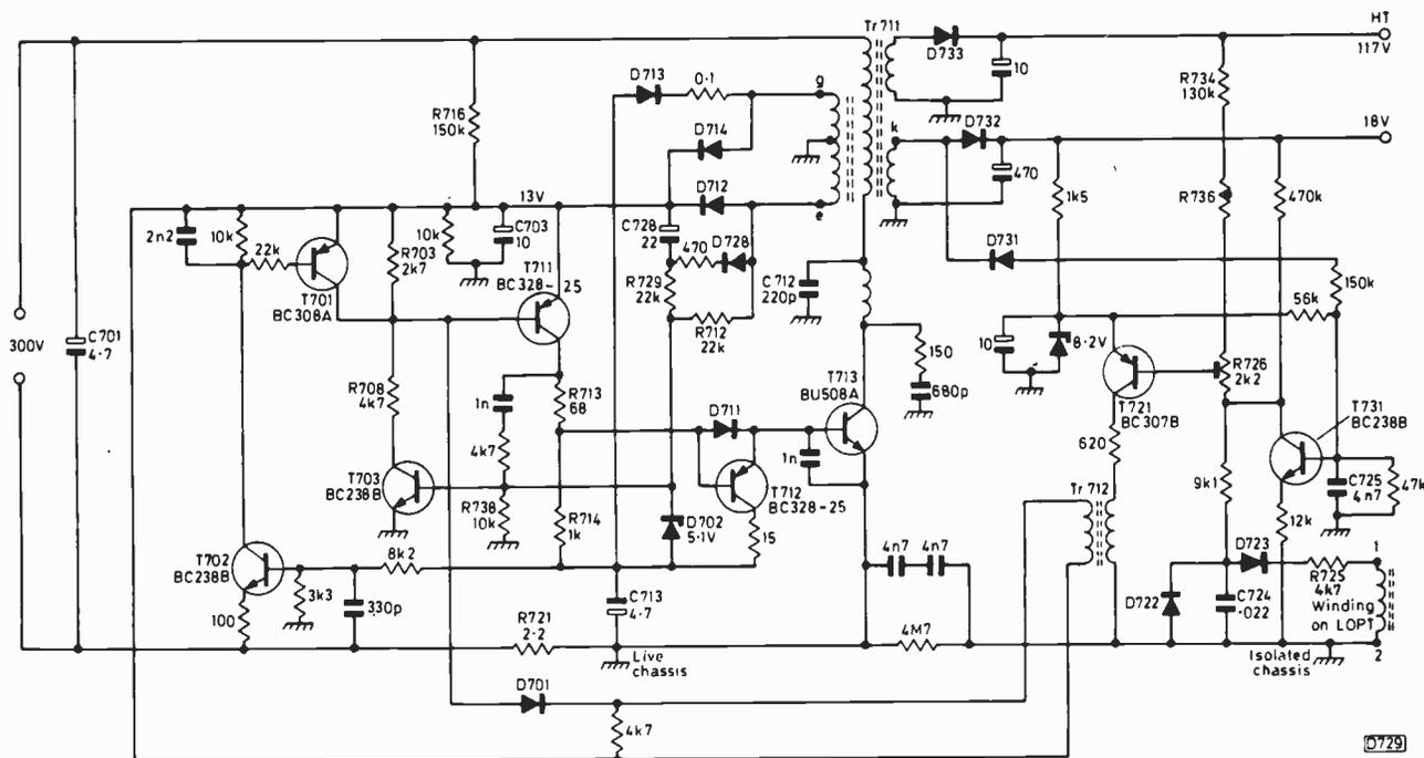
Fig. 1: Simplified circuit of the switch-mode power supply used in the ITT CVC1200 series chassis. The h.t. is 117V in the 90° 20in. version, 145V in the 110° 22/26in. version, the l.t. rails being 18V and 24V respectively. The values of the flyback tuning capacitor C712 and the resistors (R734/R736) feeding the set h.t. control R726 differ in the two versions of the chassis: the values shown above apply to the 90° version.
