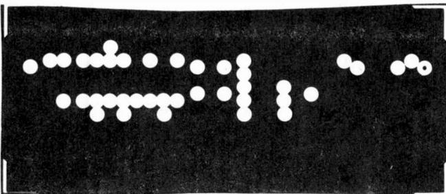
Fig. 6: Prescaler 3 board pattern, component side.
