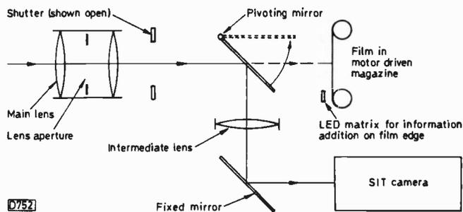
Fig. 5: Simplified diagram of a combined stills and TV camera.
