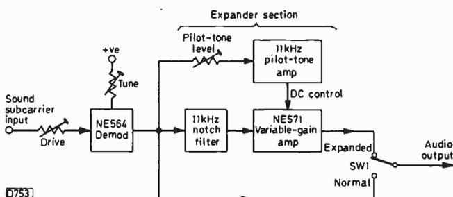
Fig. 7: Block diagram of the sound board.
