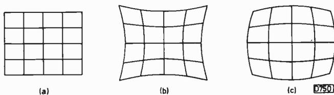
Fig. 3: Image distortion. (a) Object; (b) pincushion distortion; (c) barrel distortion.
