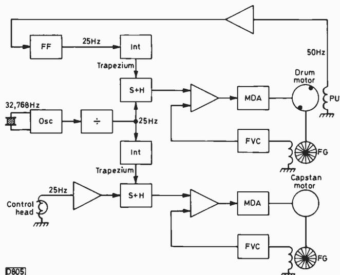
Fig. 118: Block diagram of the playback servo system.
