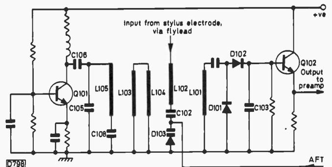
Fig. 2: The resonant circuits and detector used to retrieve the f.m. signal from the disc.
