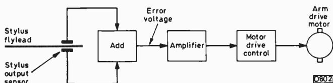
Fig. 6: The arm servo system.
