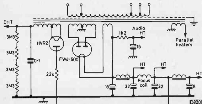
Fig. 1: The Ferguson 841T's power supply circuit.
