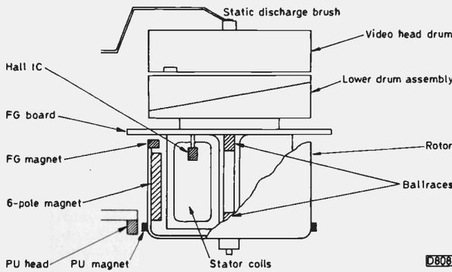
Fig. 121: Basic construction of the drum motor.
