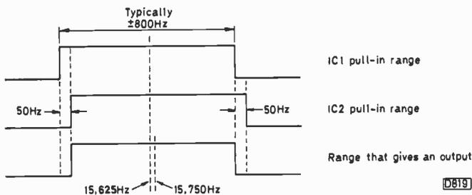
Fig. 4: Principle of the PLL narrow-band filter.
