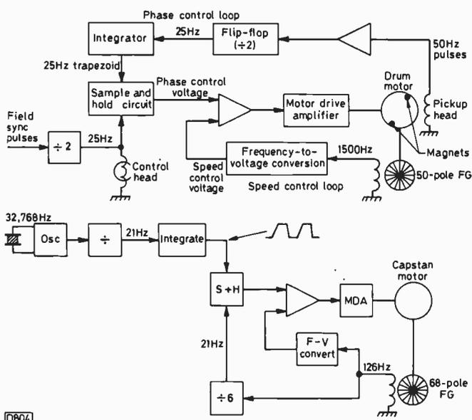
Fig. 117: Block diagram of the record servo system.
