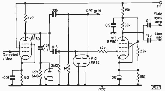
Fig. 2: The video amplifier and sync separator circuits, with d.c. restoration in both feeds.
