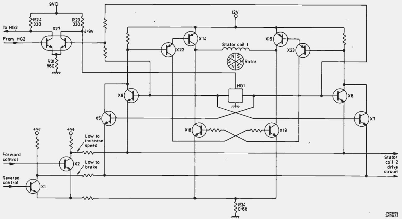
Fig. 120: The drum motor drive amplifier circuit.
