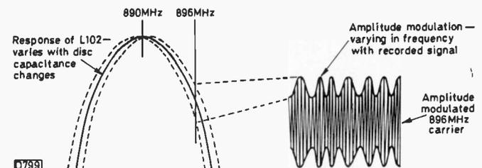
Fig. 3: Principle of signal retrieval. The frequency of the 890MHz resonant circuit varies with the disc capacitance variations, giving rise to an amplitude modulated carrier. The amplitude modulation varies in frequency.
