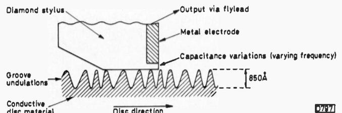
Fig. 1: Cross-section showing the stylus resting on the base of the V-shaped groove. The groove undulations, which cause capacitance variations, vary in frequency.
