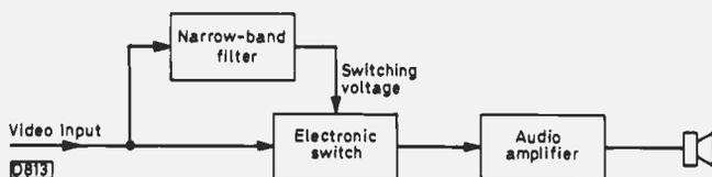
Fig. 1: Principle of the DX signal detector/alarm.
