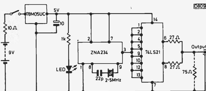
Fig. 1: Black level generator circuit.
