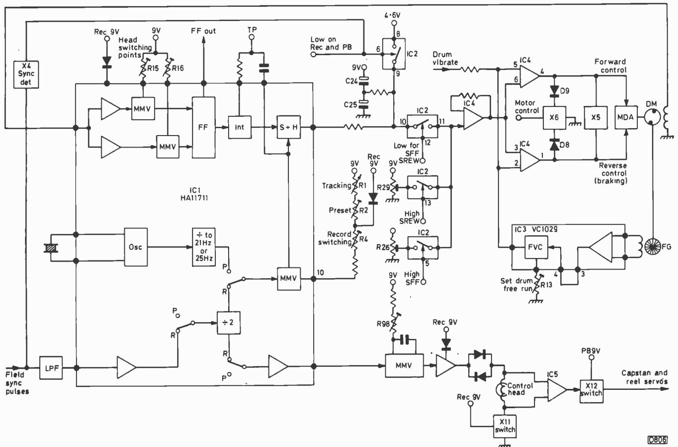
Fig. 119: Main features of the drum servo.
