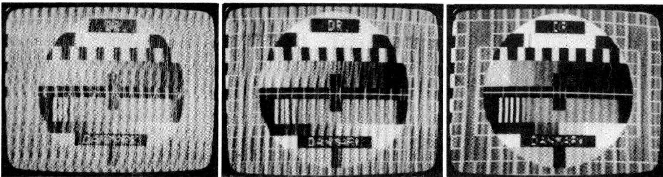
*Tropospheric reception from Denmark ch. E8 on December 4th, showing progressive reduction of the bandwidth from 6 to 3 to 2MHz to reduce interference, using the equipment described in the February-April 1982 issues of Television.*
