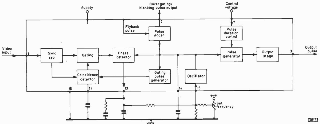
Fig. 3: Block diagram of the sections of the i.c.s used.
