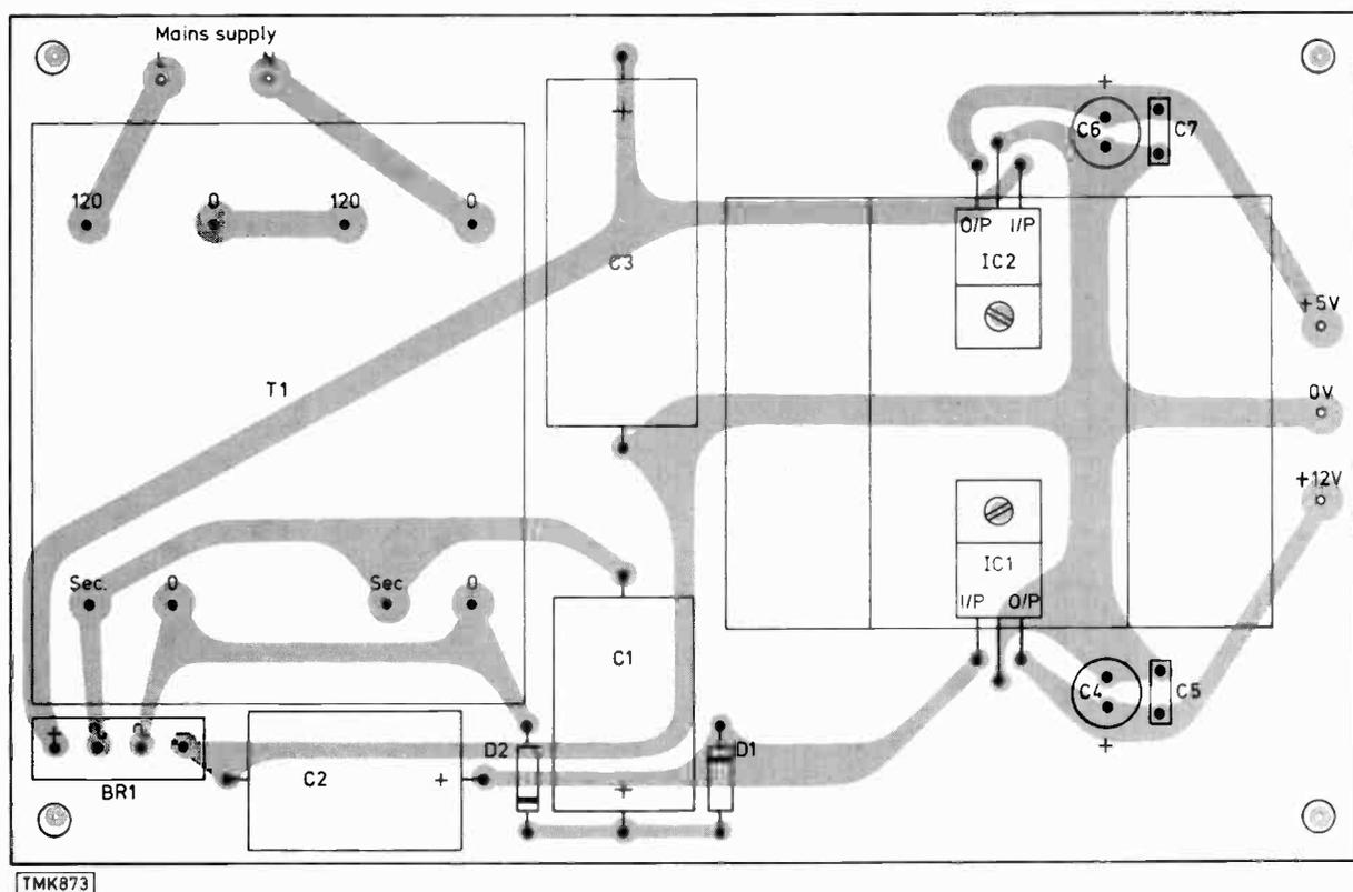
Fig. 12: Power supply panel component layout.
