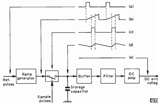
Fig. 5: Sample-and-hold principle.
