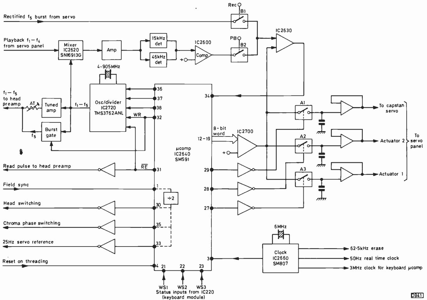
Fig. 6: Block diagram of the DTF panel.
