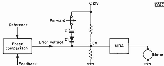
Fig. 3: Addition of a simple speed control arrangement.
