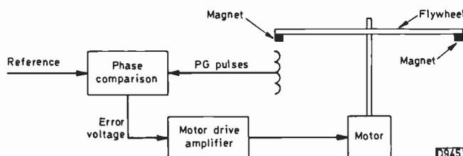
Fig. 1: Basic servo control loop.
