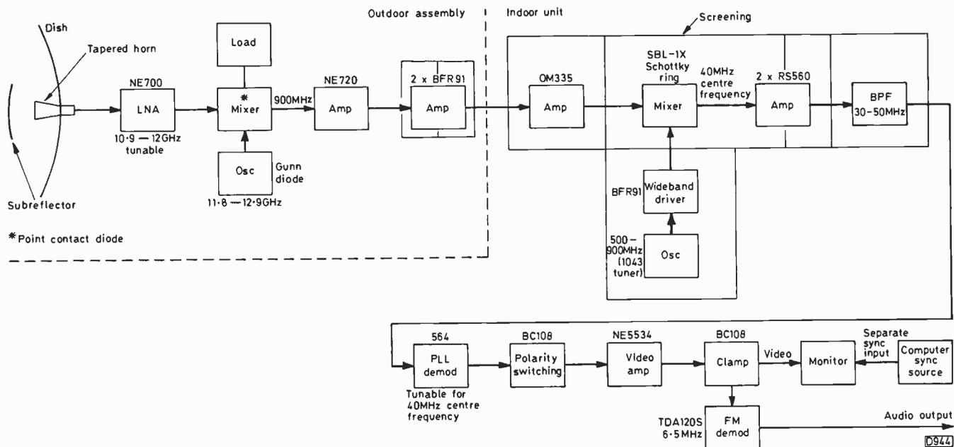
Fig. 1: Block diagram of Chris Wilson's present 12GHz satellite receiver system.
