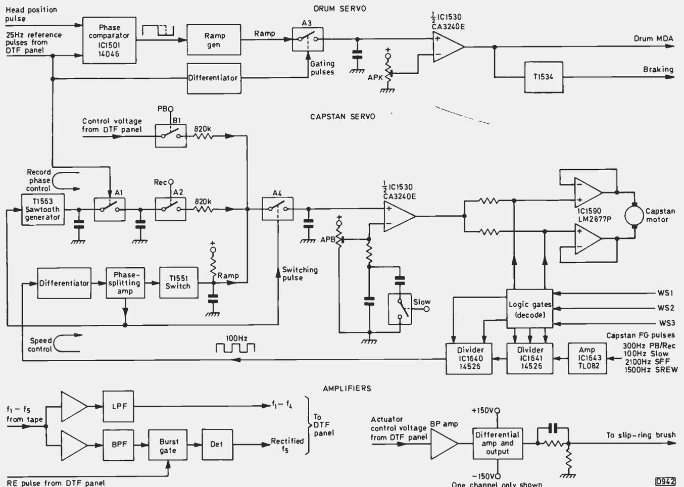
Fig. 5: Block diagram of the servo panel.
