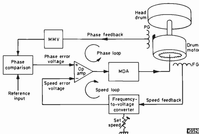
Fig. 8: Dual-loop servo system using an FG for speed feedback and a PG for phase control.
