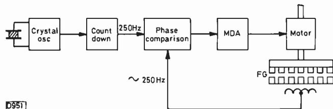
Fig. 7: Use of a frequency generator (FG). In the first FG circuits the "tone wheel" output was matched to a crystal oscillator in a phase-lock loop.
