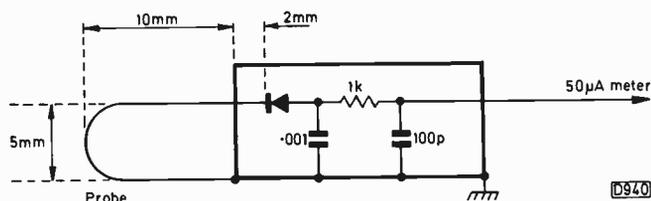
Fig. 3: Diode sniffer probe. Can be built on Veroboard.
