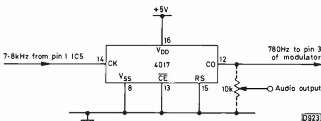
Fig. 10: Simple way of obtaining a 780Hz audio signal.
