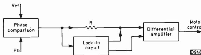
Fig. 4: Lock-in system used in Philips N1500 machines.
