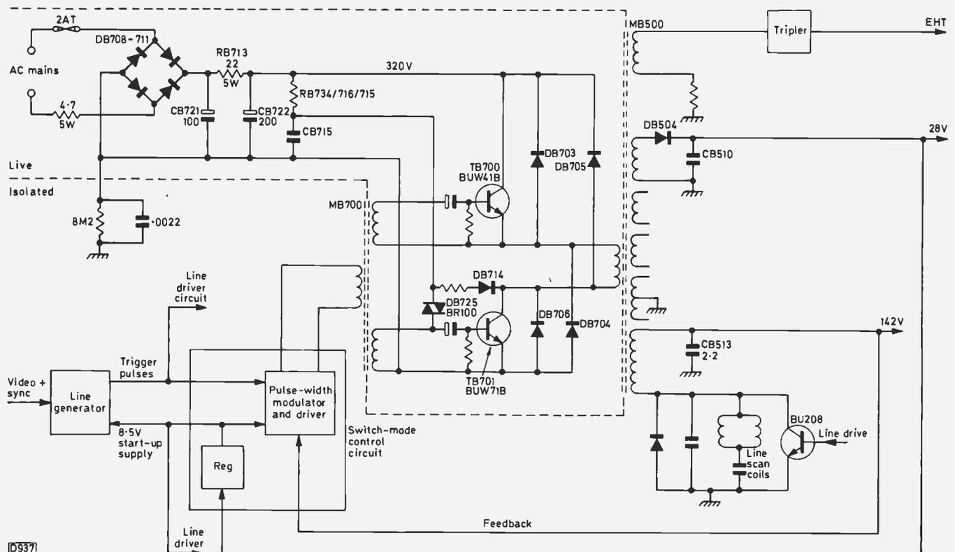
Fig. 1: Simplified circuit/block diagram of the Salora Ipsalo-2 system.
