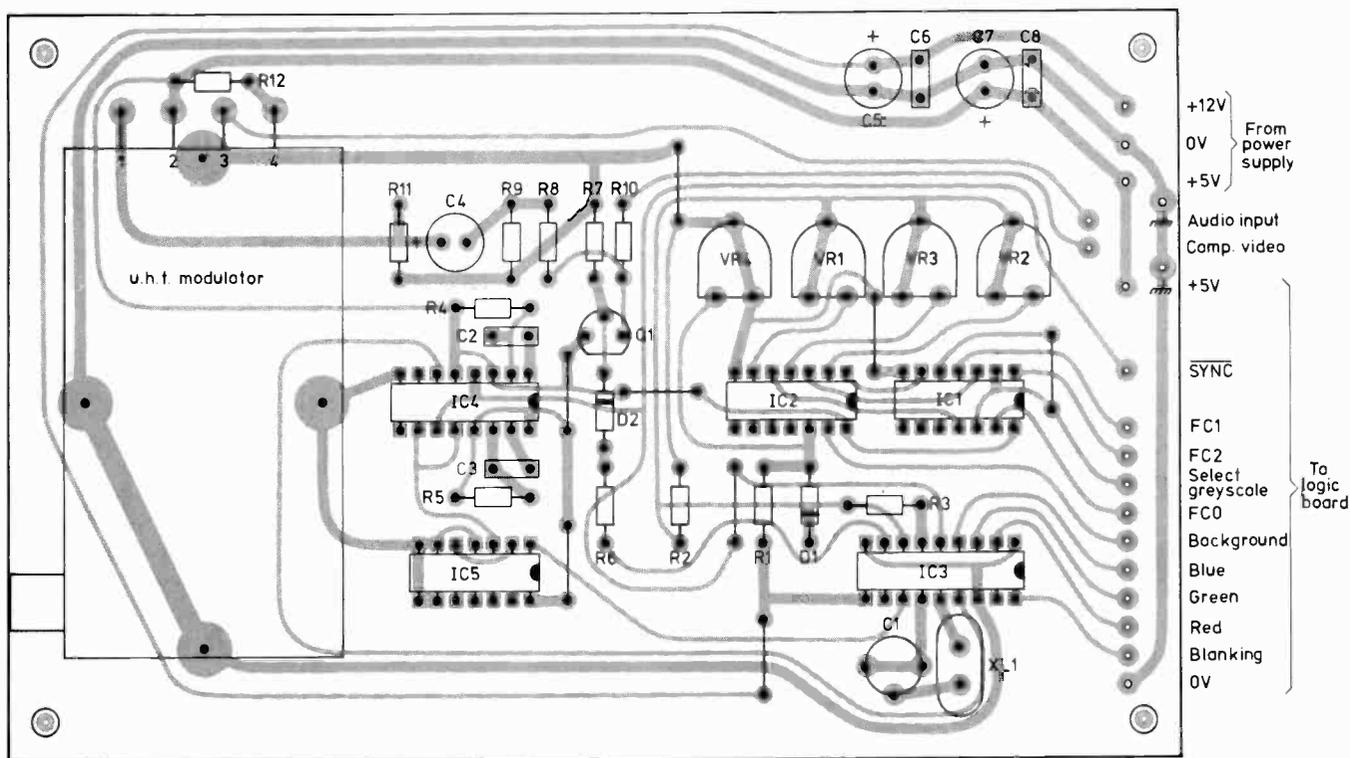
Fig. 11: Encoder/modulator board component layout.
