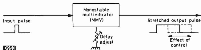
Fig. 6: Use of a monostable multivibrator (MMV) for pulse stretching, providing an adjustable delay.
