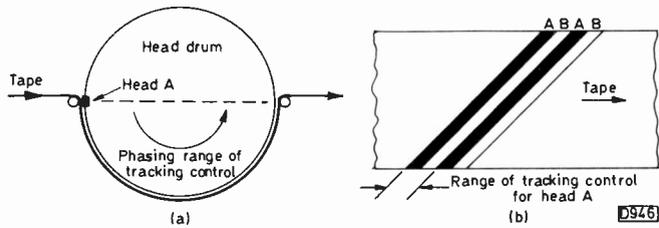
Fig. 2: Effect of the playback tracking control.
