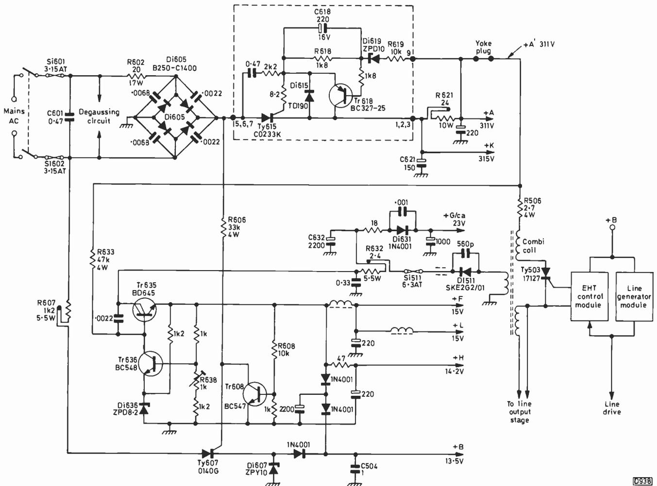
Fig. 1: Power supply arrangements used in the GSC100 chassis.
