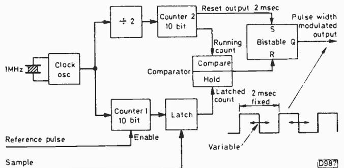
Fig. 15: Simplified outline of a digital servo used to provide phase control.
