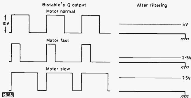
Fig. 16: Low-pass filtering (integration) produces a d.c. error voltage proportional to the mark-space ratio of the squarewave output from the SR bistable.
