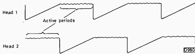
Fig. 9: DTF waveforms at slipping brushes.
