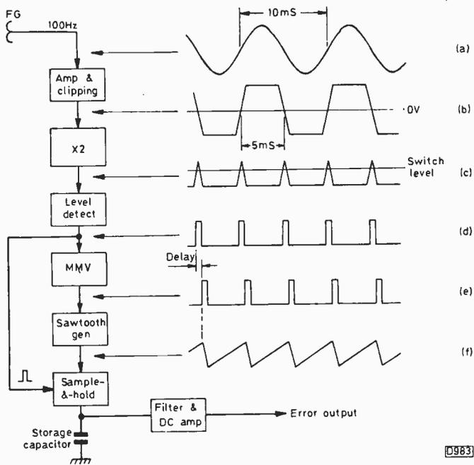
Fig. 11: Speed control system used in the Hitachi VT8000. This employs frequency-to-voltage conversion by means of a ramp and sample system. The duration of the ramp is set by the FG frequency.
