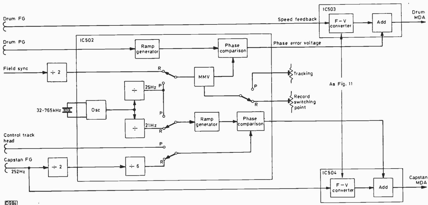
Fig. 12: Addition of the phase and speed control signals. The four-loop system used in the Hitachi VT8000.
