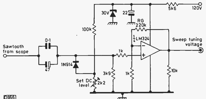
Fig. 4: D.C. restorer and amplifier circuit.
