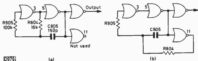
Fig. 1: CMOS gate oscillator circuits.
