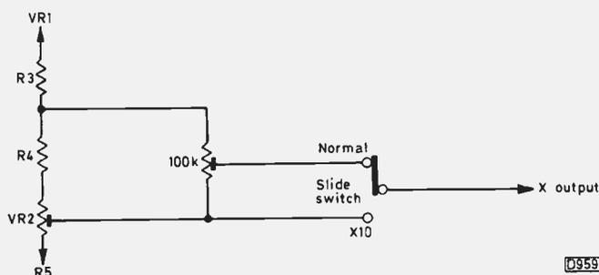
Fig. 2: Modification to the scope component test unit.
