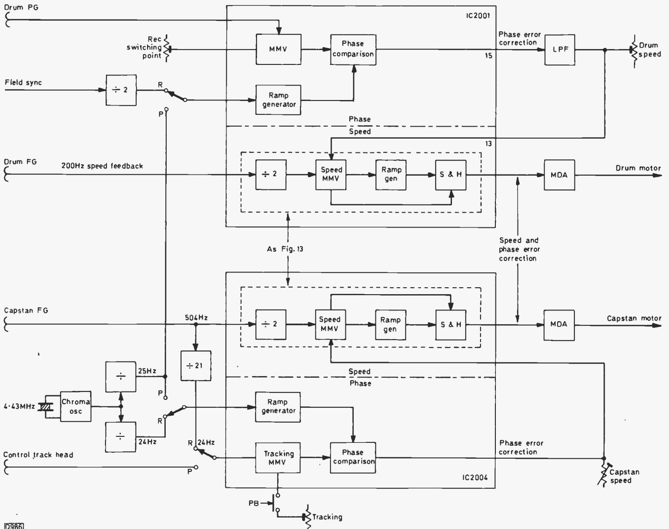
Fig. 14: Phase loops operating on the speed MMVs - Panasonic NV7000. The 4.43MHz chroma reference crystal also provides the servo reference signals.
