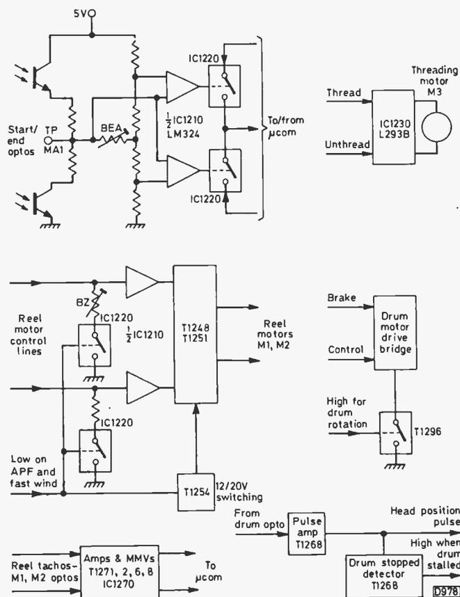
Fig. 7: Motor connection board block diagram.
