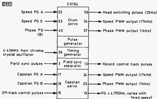
Fig. 18: LSI servo chip used in the Sony F1 and C9. These machines have no drum servo as such: regularly positioned magnets on the drum give six pulses per revolution to PGs A and S. Because the PG S coil is offset by 30° under the drum its pulse lags A by 3msec and the speed loop works to maintain this interval. PG B provides one pulse per drum revolution for phase control.
