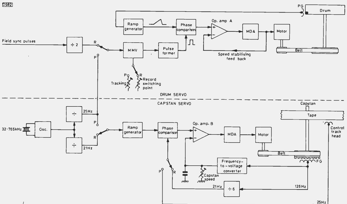
Fig. 10: Block diagram of the servo system used in the Hitachi VT5000 to control two d.c. motors.
