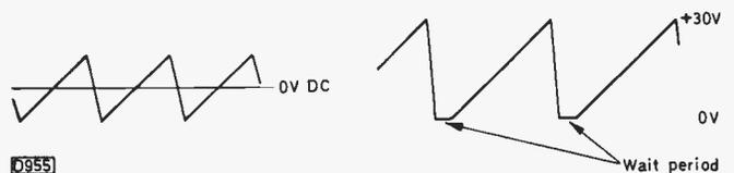
Fig. 2 (left): A.C. sawtooth waveform.
