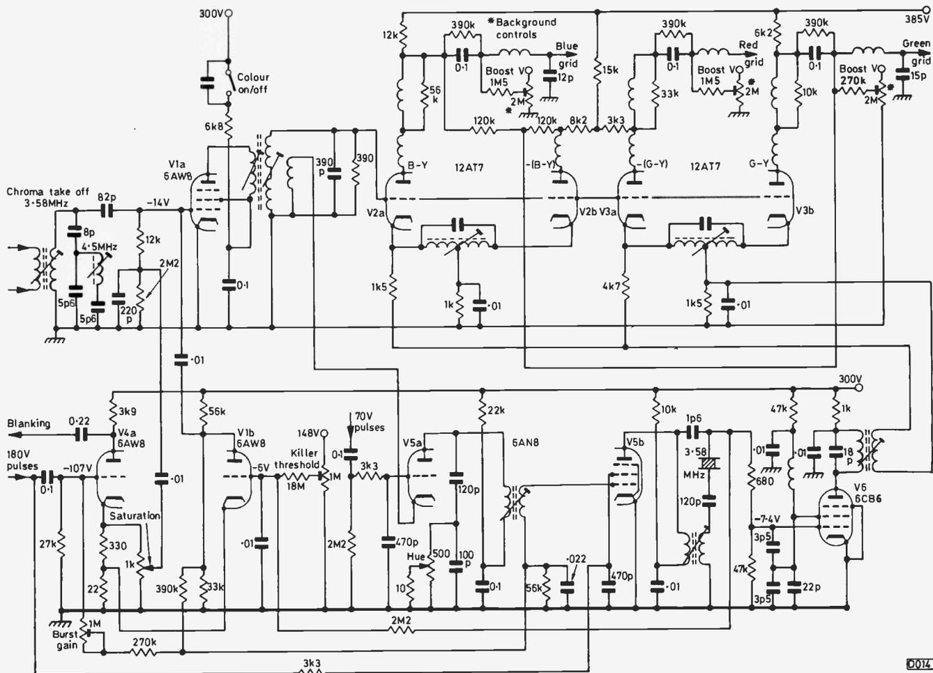
Fig. 1: The colour decoder circuit used in late-production 1957 RCA Super and Special models. The burst/reference signal section was simplified by the use of a passive subcarrier regenerator, hence no need for an a.p.c. loop. Demodulation was carried out on the B - Y and G - Y axes, with matrixing to obtain the R - Y colour-difference signal. Only a single chroma amplifier stage was used.
