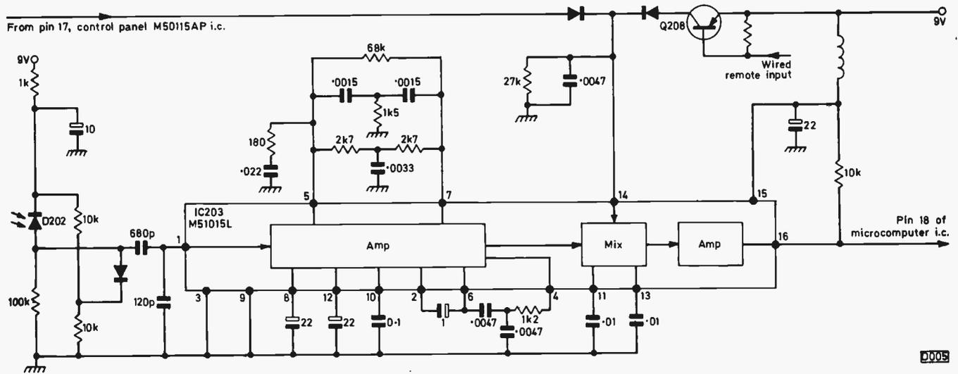
Fig. 7: Infra-red remote control receiver circuit, Ferguson Model 3V35.
