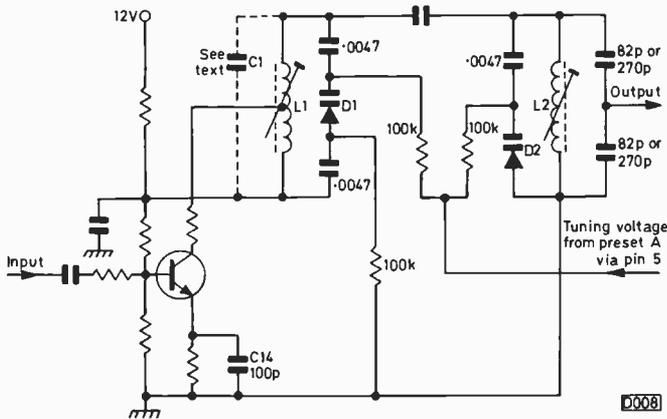
Fig. 2: Selectivity module after modification.
