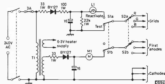
Fig. 1: C.R.T. tester/booster circuit.
