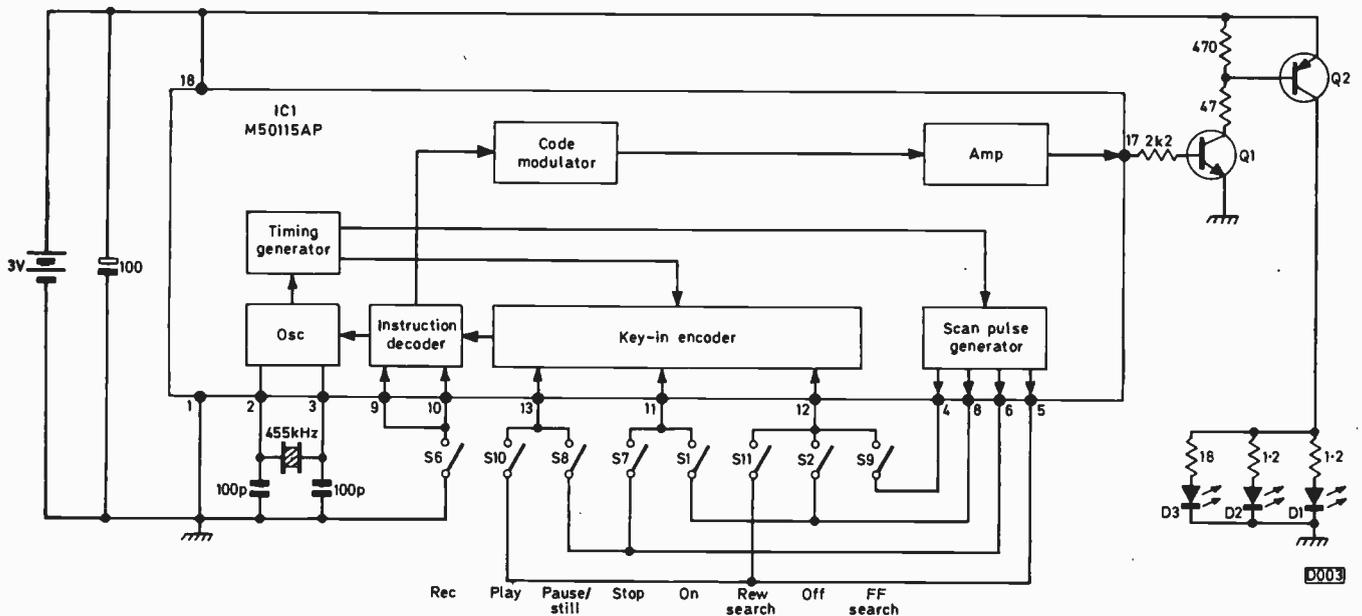
Fig. 5: Infra-red remote control transmitter circuit, Ferguson Models 3V35/3V36.
