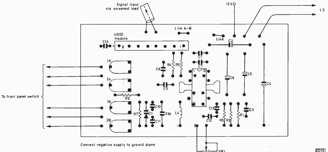
Fig. 4: Component layout. The components are mounted on the groundplane side of the board. Board actual size.
