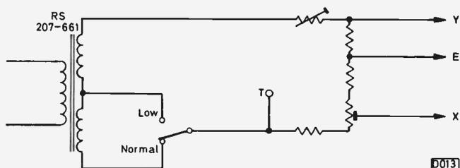
*Fig. 1: Suggested method of reducing the output voltage provided by the component tester.*
