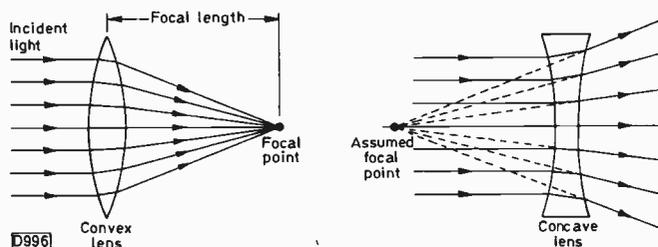
Fig. 2 (left): When parallel rays encounter a convex glass surface they are bent inwards. The angle of refraction is greater for the outside rays than for the inner ones because the angle of incidence is greater, due to the surface curvature. Thus all the rays converge at a certain point (the focal point).
