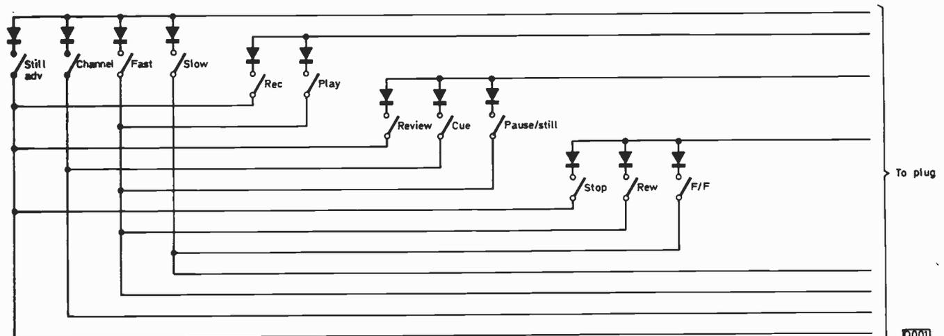
Fig. 3: Multicore cable remote control switch circuit used with the Panasonic NV7000.
