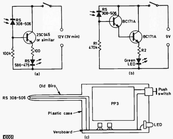
Fig. 8: Infra-red detector arrangements that can be used for test purposes. Adjust the value of R1 in (b) for the sensitivity required; add R2 if necessary to control the brightness and current.
