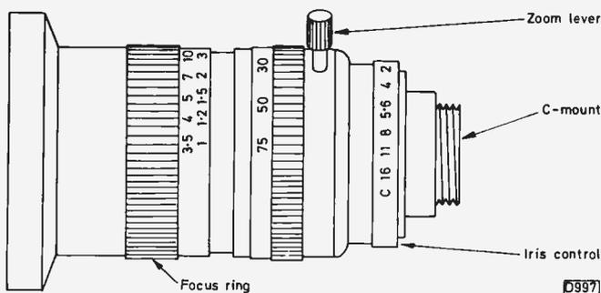
Fig. 4: A typical detachable zoom lens. The first control from the end is the focus ring, which is calibrated in feet and metres. More adjustment is needed at the near end of the scale than the distant one, as the wider spacing of the calibration shows. Next is the zoom control, which is sometimes calibrated with focal length. Finally there's the iris control, which is marked with the *f* numbers. The C position denotes closed, i.e. no light enters.
