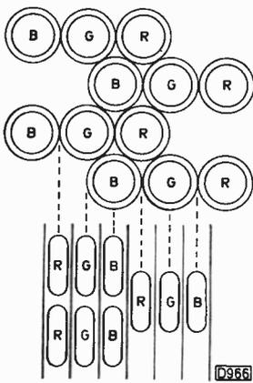
Fig. 8 (left): To achieve the same order of resolution, a striped screen tube needs a finer "triad" structure than a delta-format tube.
