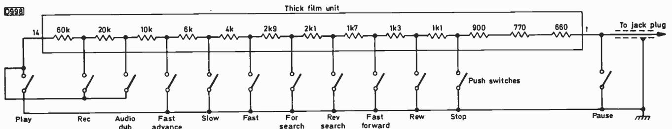
Fig. 1: Circuit of the Hitachi VT8300's remote control handset.
