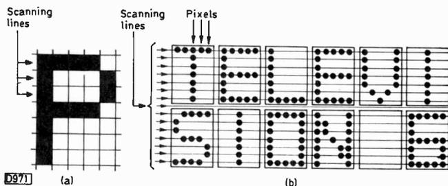
Fig. 13: (a)  $7 \times 5$  dot matrix used for data displays. (b) Dots, cells and their relationship to the TV raster.
