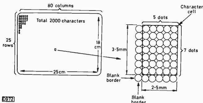
Fig. 14: Character structure for an 80-column display, related to a 37cm screen. Beam diameter is of the order of 0.45mm.
