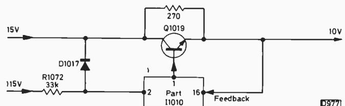
Fig. 1: 10V regulator used in the Sharp Model C2092's digital tuning system.
