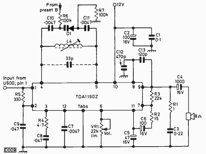
Fig. 3: Demodulator and a.f. circuit.
