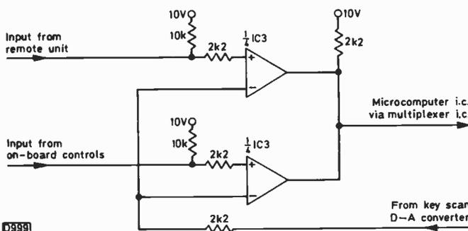
Fig. 2: Arrangement used in the Ferguson 3V29 to combine the remote and on-board control commands.
