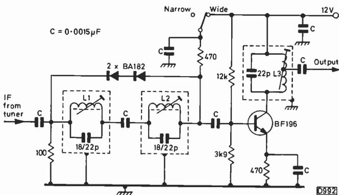
Fig. 1: Circuit of Paul Barton's i.f. selectivity module. L1 and L2 consist of 15 turns, close spaced, of 28 s.w.g. wire on a 3/16in. (4.5mm) former with core. L3 is the same but centre tapped.
