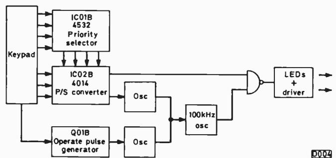
Fig. 6: Block diagram of the infra-red remote control transmitter used with the Hitachi VT8500.
