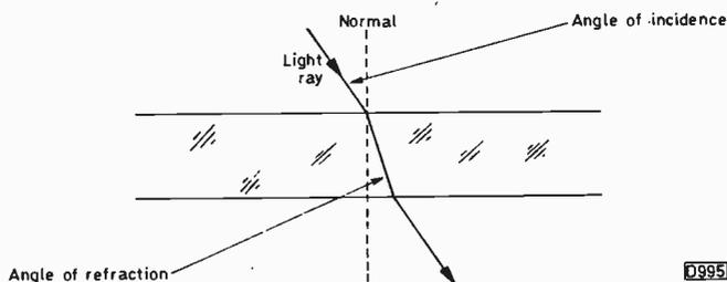
Fig. 1: When a ray of light strikes a dense medium such as glass it's refracted. The angle of refraction away from the normal is dependent on the angle of incidence.
