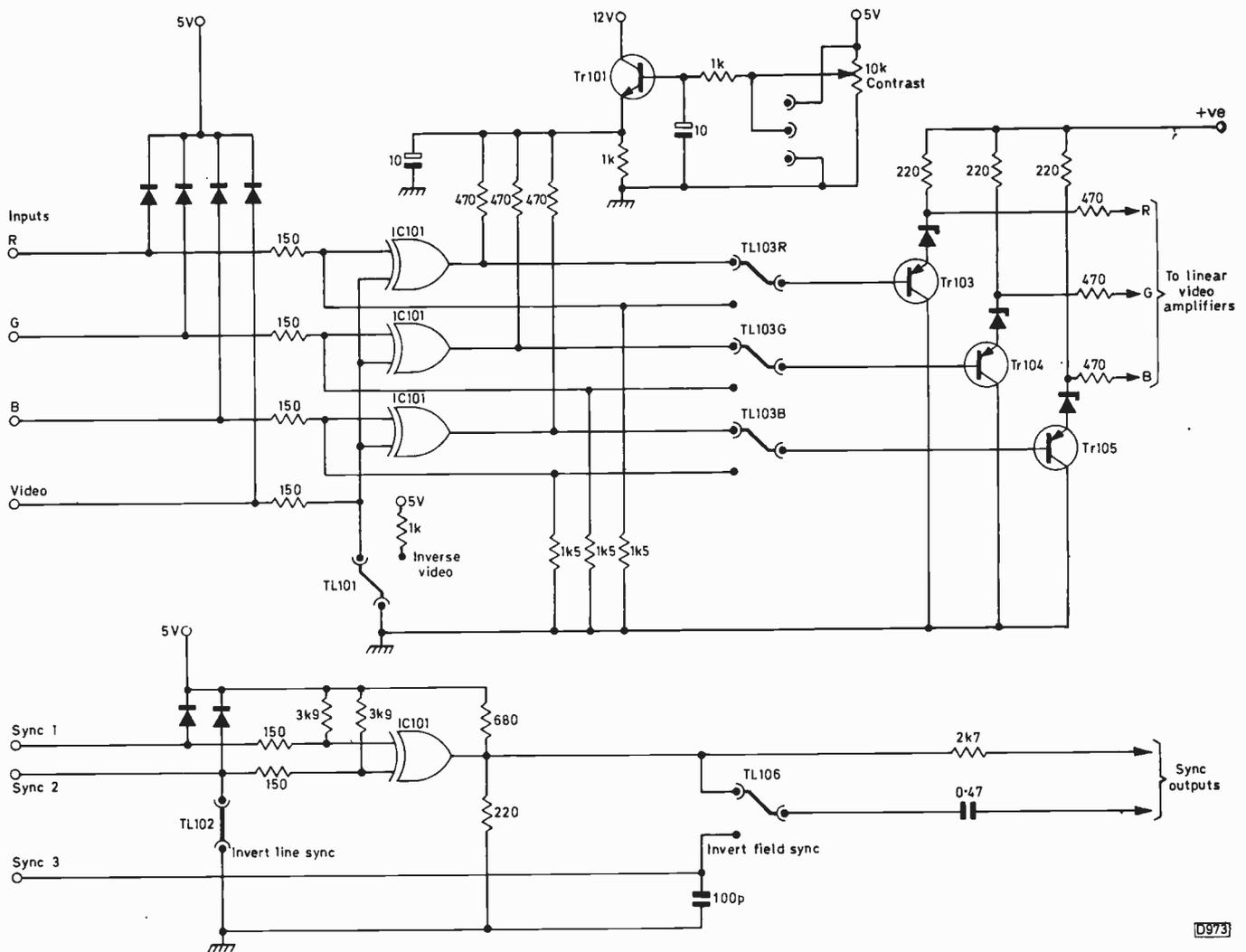
Fig. 15: Representative computer monitor video input circuitry. TTL or linear operation is selected by means of links TL103R/G/B. The exclusive-OR gates in IC101 invert the video pulses when link TL101 is changed and the line sync pulses when TL102 is present. Transistor Tr101 forms the upper leg of a resistive attenuator for contrast control in the TTL mode. Tr103/4/5 and the accompanying zener diodes provide level-shifting and temperature compensation.
