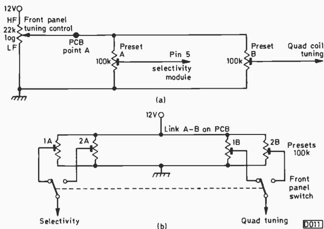
Fig. 5: Alternative tuning arrangements. (a) For continuous tuning, (b) for two-position switched tuning.
