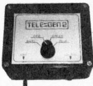
Telegen 2 is a colour bar generator at a very modest price and yet is extremely effective, stable and durable. It is the perfect compliment to Telegen 1, giving colour bars arranged in the following sequence: white, yellow, cyan, green, magenta, red, blue and black. The unit provides a signal in the UHF band approx. Channel 35 and requires a supply of 14 to 18 volts 0.C.
