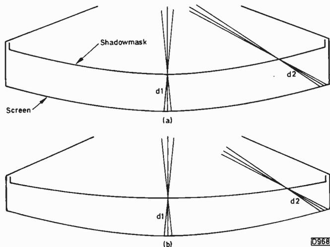
Fig. 10: (a) Constant mask/screen spacing used with earlier delta-gun tubes. Distance  $d_2$  is greater than  $d_1$ , and the phosphor dots are more widely spaced at the extremes of the display. (b) When the mask and screen have different radii distances  $d_1$  and  $d_2$  remain the same and the dot pitch is uniform over the entire screen area.
