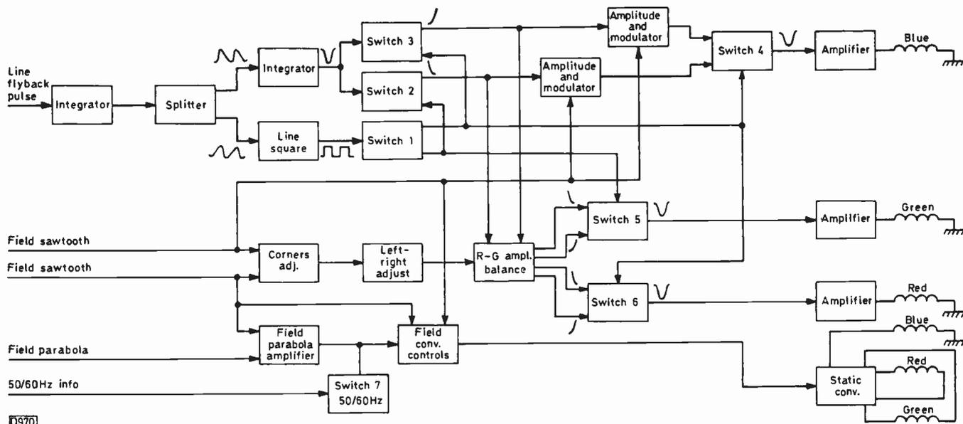
Fig. 12: Block diagram of the precision convergence system used by Barco with high-resolution delta-type tubes.
