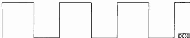
Fig. 2: Waveform at the collector of Q602 with an 18V supply. The waveform can vary a lot – the important thing is that it's present.
