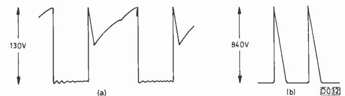
Fig. 4: (a) Waveform at the collector of Q502. (b) Waveform at the collector of Q503 (measure with care).
