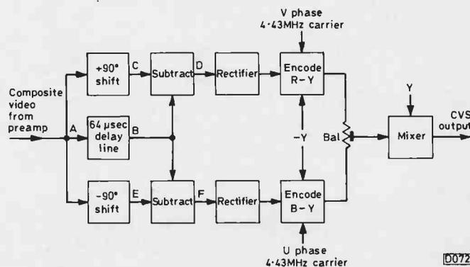
Fig. 3: Block diagram of the colour signal processing arrangement in a camera using phase colour separation.
