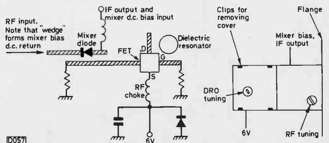
Fig. 2: Left, approximate circuit of the Mitsubishi FO-UP-11K oscillator/mixer module. Right, pin connections.
