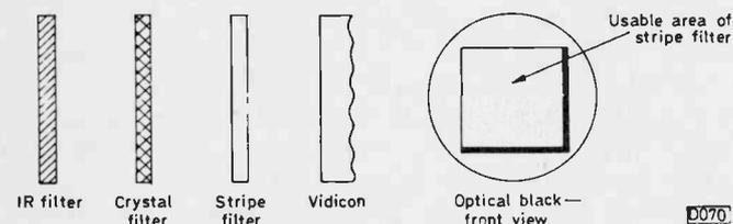
Fig. 1: Elements at the front of a colour vidicon tube.
