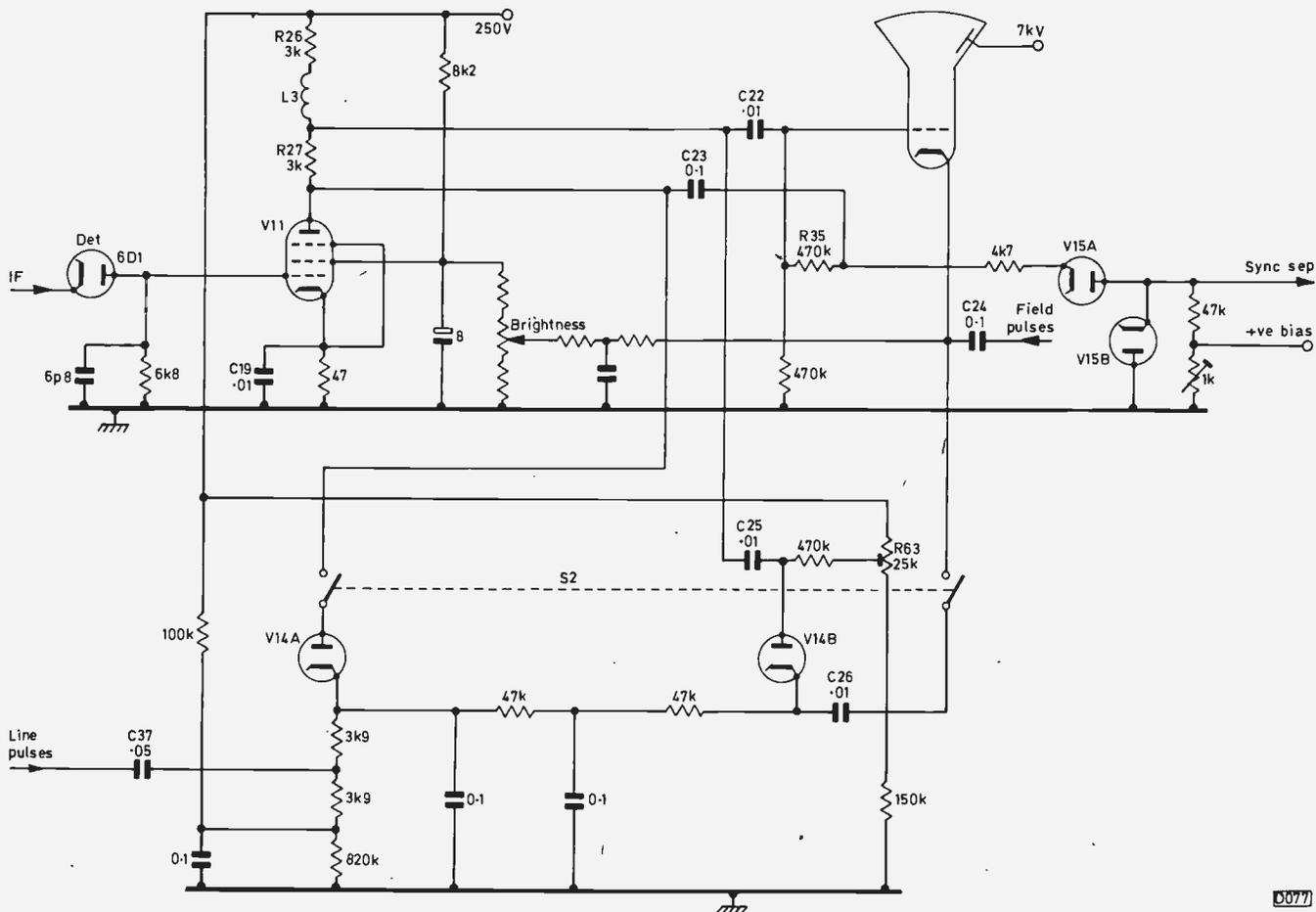
Fig. 1: The video and vision interference limiter circuitry used in the RGD B2351T.
