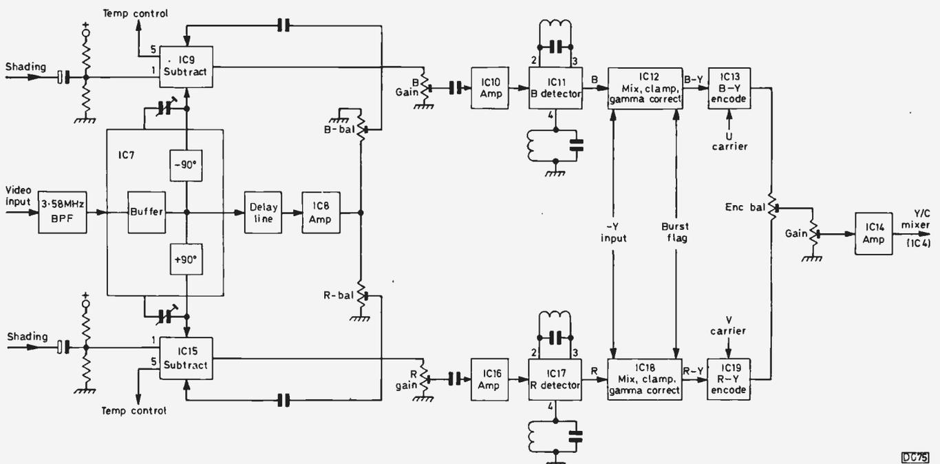
Fig. 6: Block diagram of the colour signal processing system used in the Ferguson 3V17 camera.
