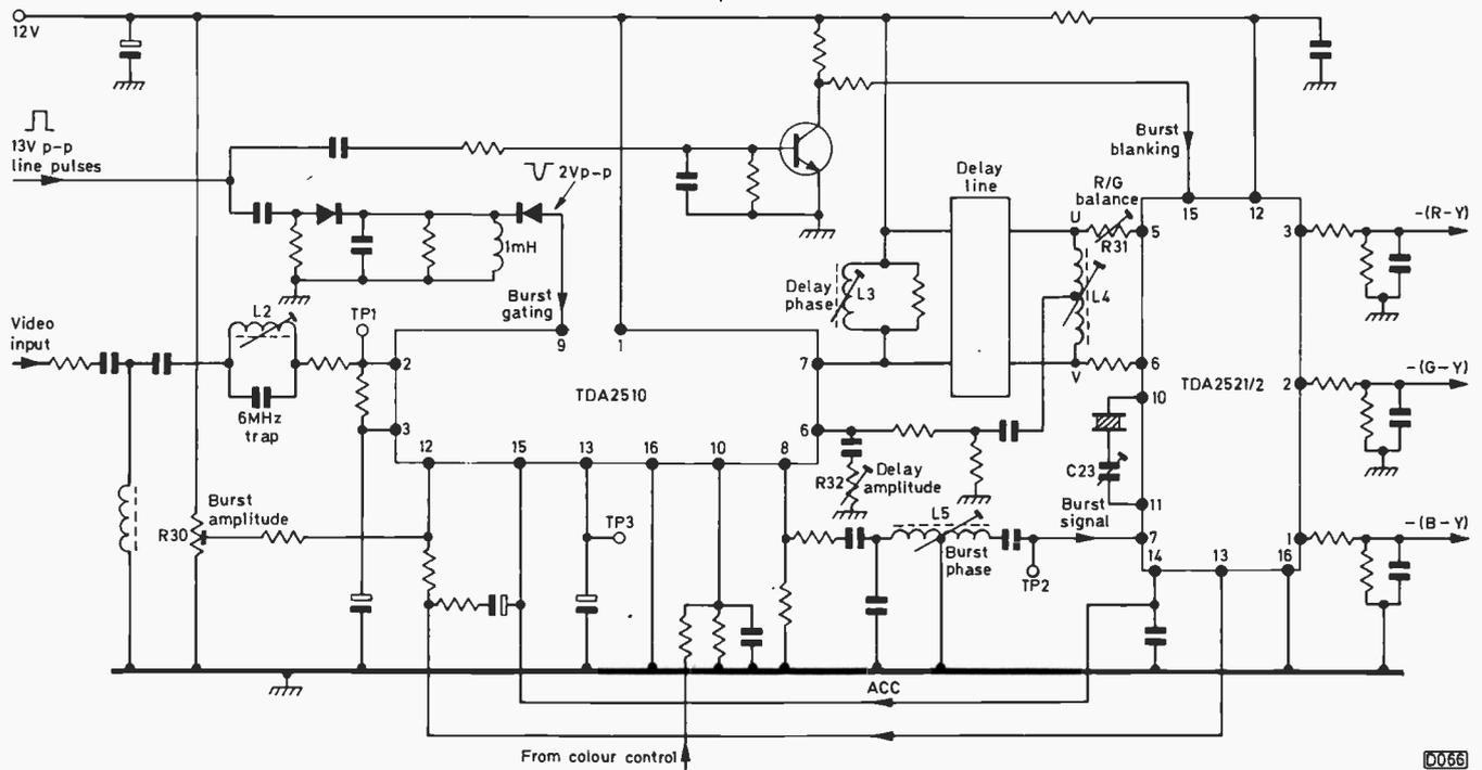
Fig. 3: The two-chip decoder used in Network Models NWC1401 and NWC1402 (simplified circuit).
