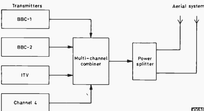
Fig. 3: Combining the outputs from four transmitters to drive the aerial system.
