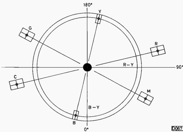
Fig. 4: Scope vector display obtained with a correctly adjusted decoder. The display arises from the fact that the scope's X and Y axes coincide with the B - Y and R - Y axes respectively: with a colour bar signal of the type used outer dots are obtained at the phase positions corresponding with the colours in the pattern.
