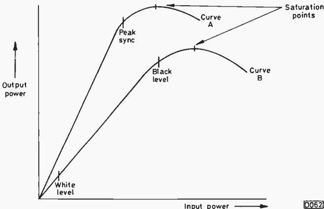
Fig. 2: Klystron power characteristic curves. Efficiency can be increased by pulsing the klystron so that its characteristic is altered for different parts of the input signal waveform.
