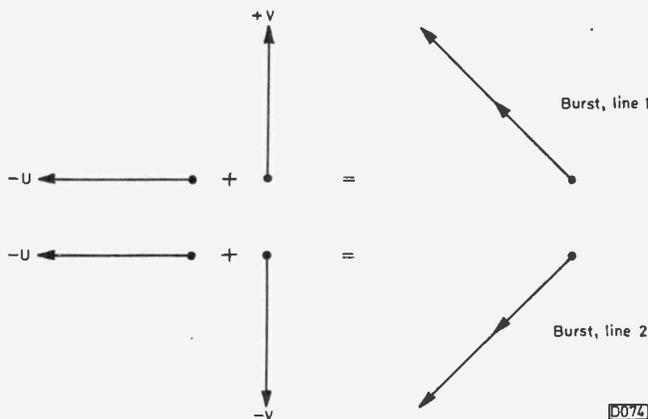
Fig. 5: Forming the burst signal.
