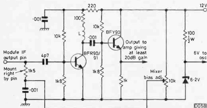
Fig. 3: U.H.F. i.f. preamplifier and mixer bias circuits. Take the output to a further wideband u.h.f. amplifier with a gain of at least 20dB. An additional amplifier prior to the receiver may help as well. Coil L consists of two turns 1/8in. diameter wound on a resistor.
