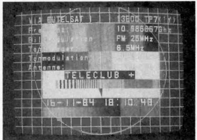
Photo 4: Same signal as shown in Fig. 3 but this time received with the addition of an LNA.
