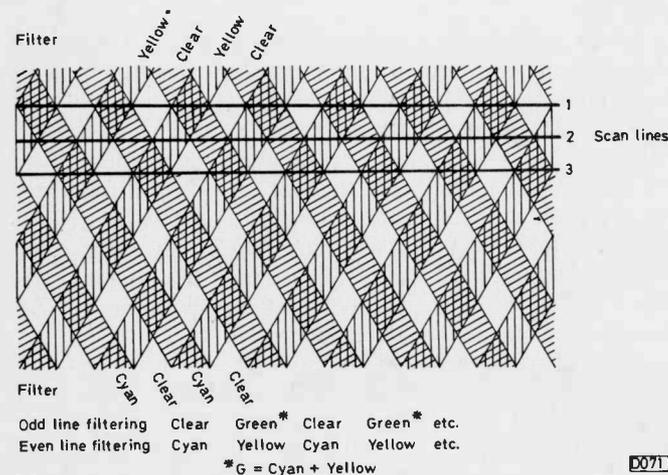
Fig. 2: Phase colour filter arrangement.
