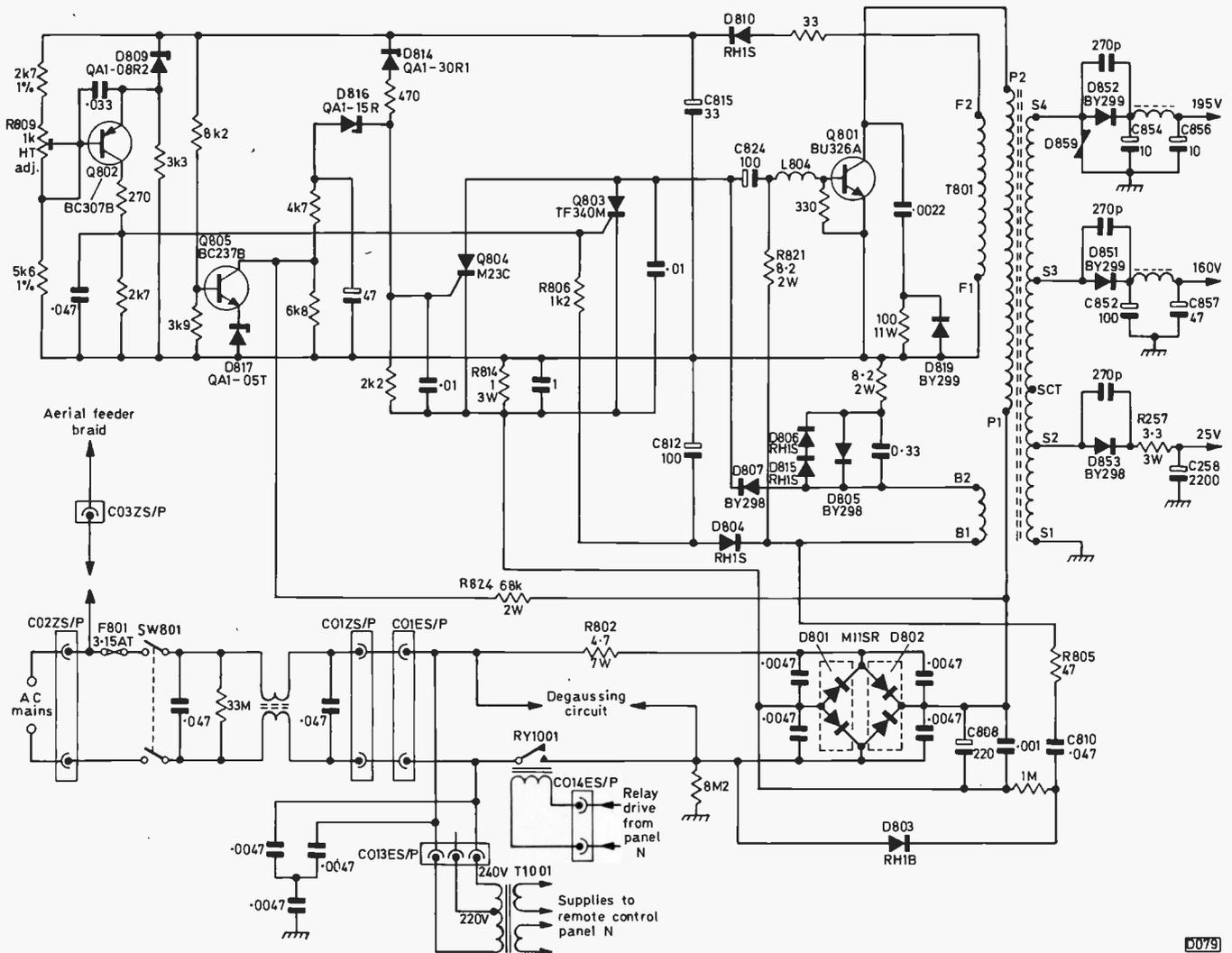
Fig. 1: The switch-mode power supply circuit used in the Panasonic Model TC2205 (chassis U2). It's not immediately apparent, but R824 is Q805's collector load resistor. Note that the circuit diagram in the manual shows R814 connected incorrectly (blob missing).
