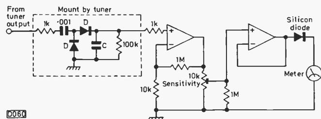
Fig. 5: Signal strength meter circuit. Diodes D type OA90 or similar. C is 0.001µF – if the readings vary a lot with the video content, increase the value of C to 0.1µF or more. The 10kΩ potentiometer adjusts the meter's sensitivity. Any type of operational amplifier will do.
