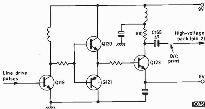
Fig. 2: High-voltage pack drive circuit, Panasonic video camera type WV3000.
