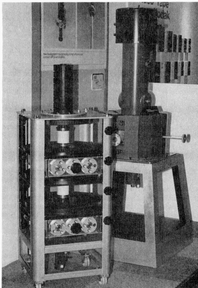
High-power devices for u.h.f. TV transmitters: a four-cavity klystron on the left and a klystrode on the right. Klystrons are tuned by adjusting the cavities: two of the four cavities of the device on the left are shown in position. The klystrode is a new, experimental type of amplifying device that combines some of the features of a tetrode and a klystron output amplifier.
