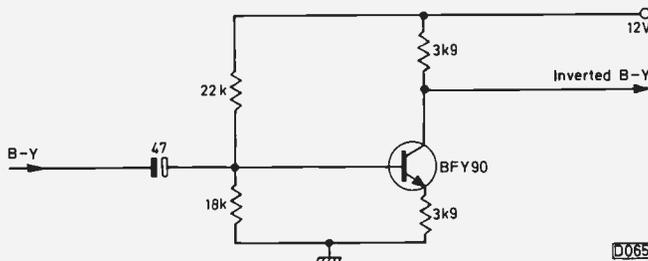
Fig. 2: Simple signal inverter circuit.
