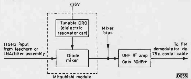
Fig. 1: Block diagram of the downconverter/u.h.f. i.f. amplifier system. The oscillator can be tuned over approximately 10.4-11.4GHz.
