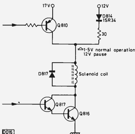
Fig. 1: Pinch roller solenoid circuit, Sanyo VTC9300.
