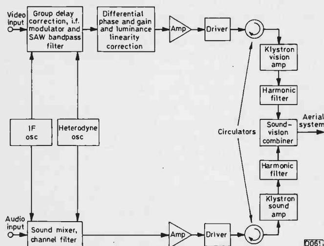
Fig. 1: Block diagram of a high-power u.h.f. TV transmitter using i.f. modulation and klystron output stages. The sound and vision channels are both shown: the outputs from the two klystrons are combined.
