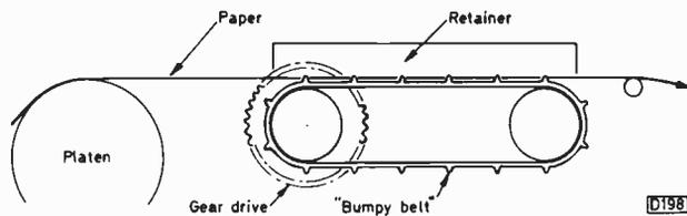
Fig. 8: Tractor feed arrangement.
