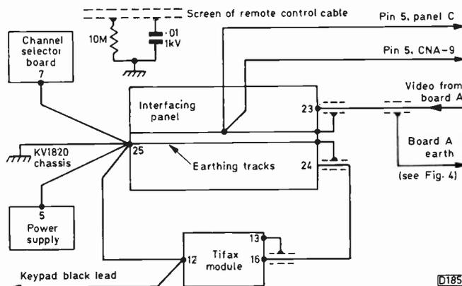
Fig. 7: Recommended earthing arrangements.
