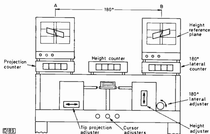
Fig. 1: Layout of the head alignment console.
