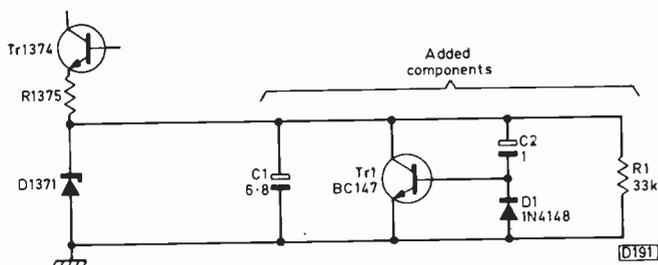
Fig. 1: Soft-start circuit for the Philips G8 chassis.
