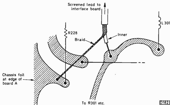
Fig. 4: Method of tapping the video from board A in the Sony Model KV1820UB.
