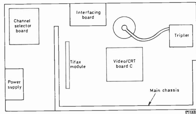
Fig. 10: Positions of the extra panels and the Tifax module in the Sony Model KV1820UB.
