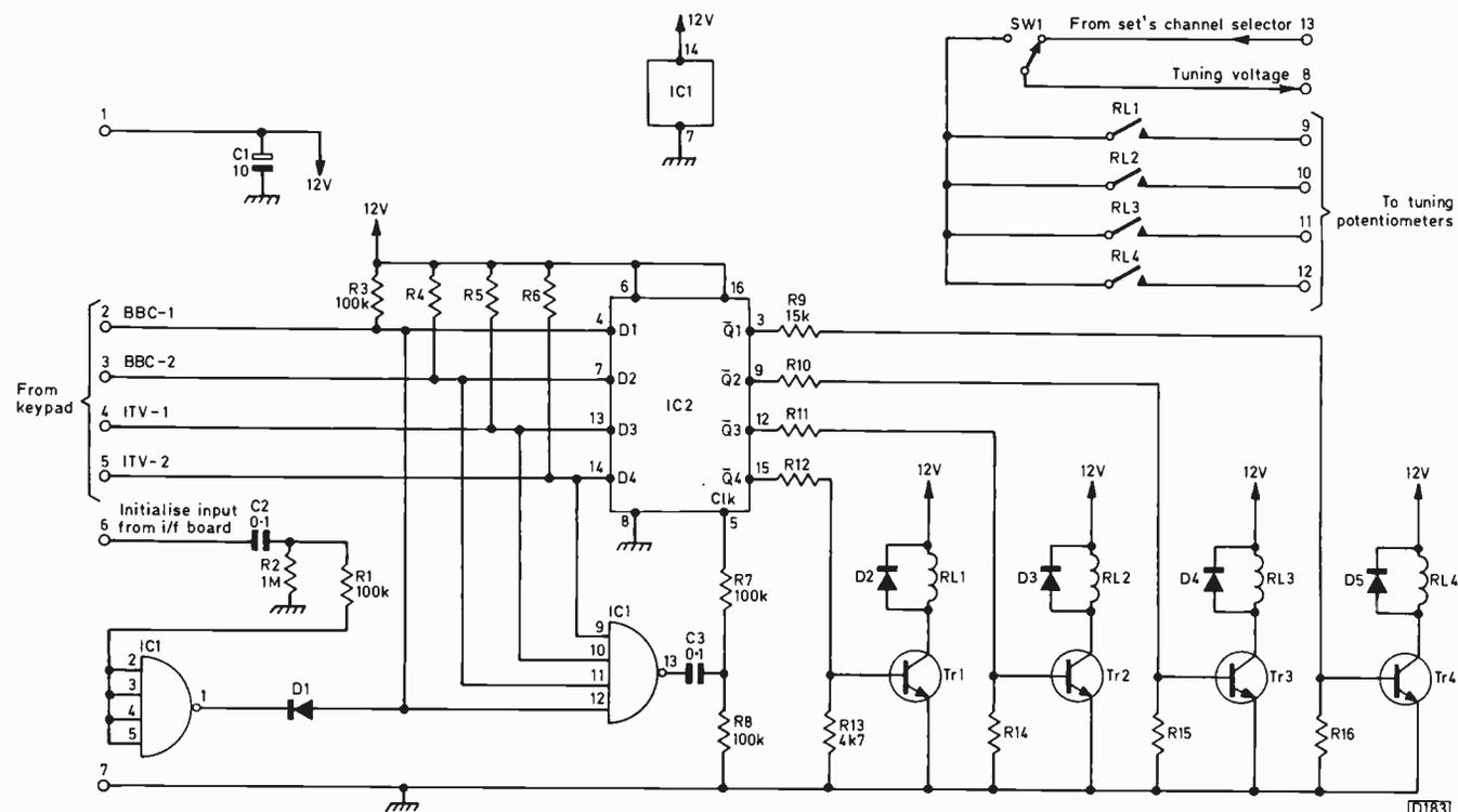
Fig. 5: Remote channel selector circuit.
