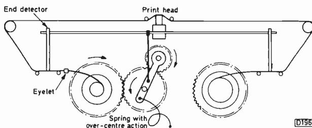
Fig. 6: Ribbon reversing mechanism.
