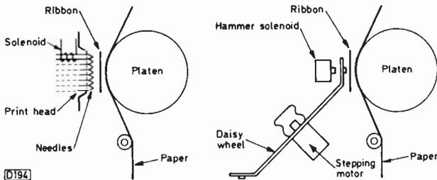
Fig. 3 (left): Matrix printer operation.
