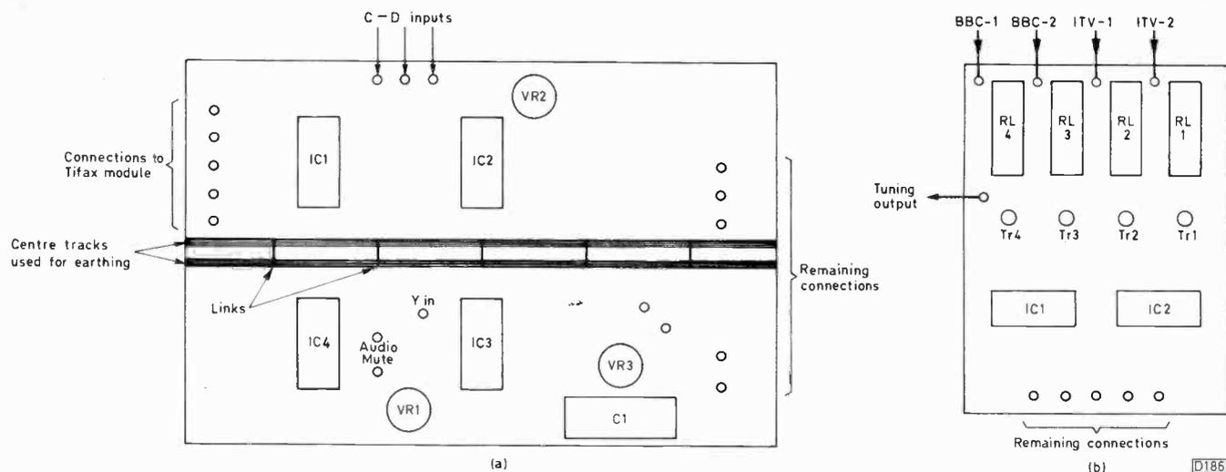
Fig. 8: Basic board layouts: (a) interface panel; (b) remote channel selector panel.
