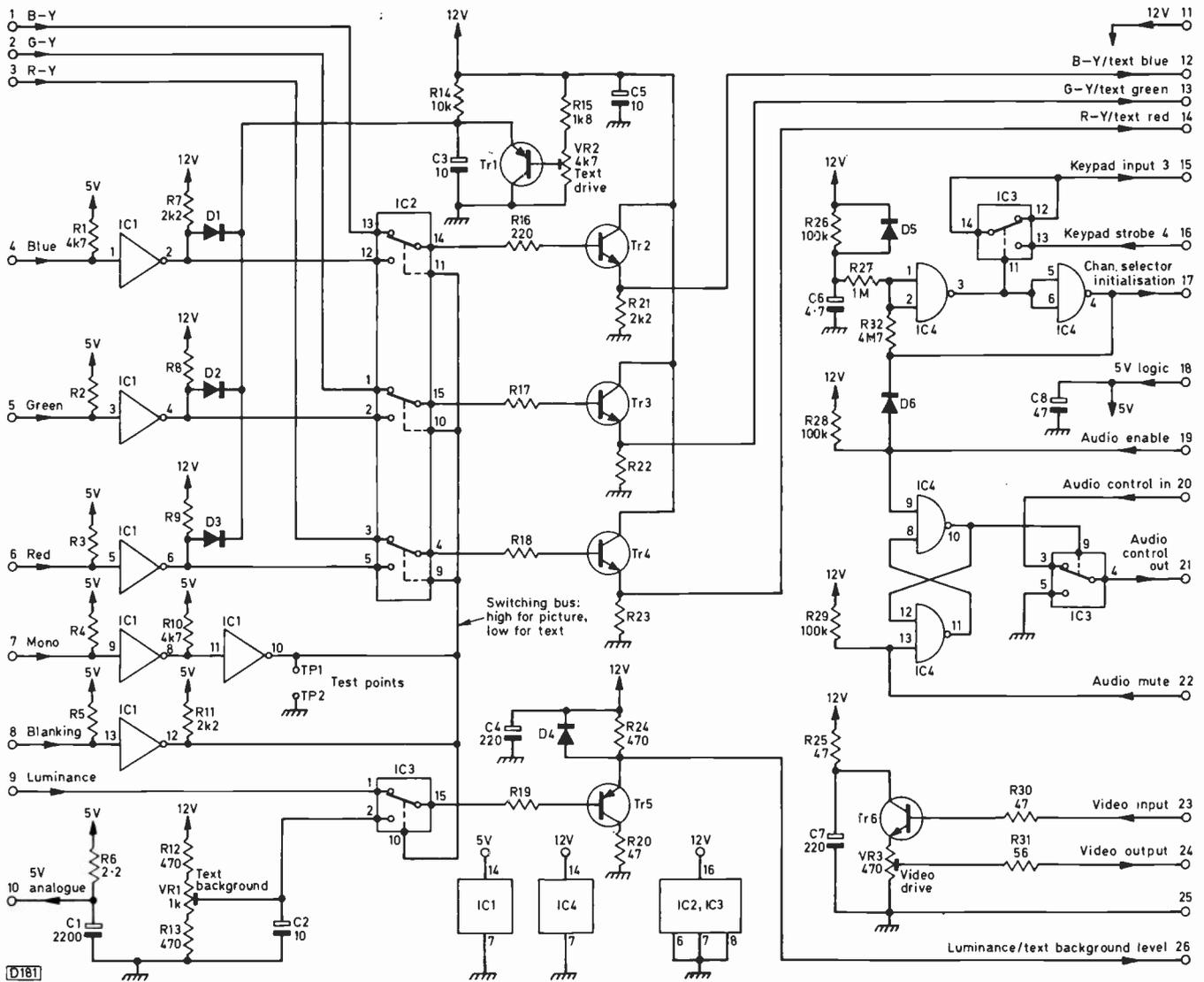
Fig. 3: Interface board circuit.
