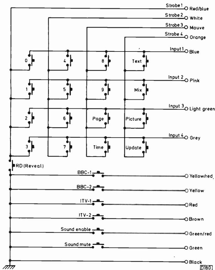
Fig. 2: Circuit of the keypad.
