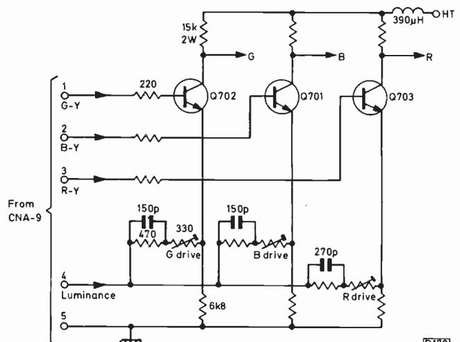
Fig. 1: RGB output stage circuits, Sony Model KV1820UB.
