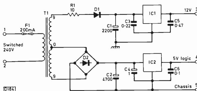
Fig. 6: Circuit of the power supply for the Tifax decoder and the interface and remote channel selector panels.
