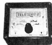
Telegen 2 is a colour bar generator at a very modest price and yet is extremely effective, stable and durable. It is the perfect compliment to Telegen 1, giving colour bars arranged in the following sequence: white, yellow, cyan, green, magenta, red, blue and black. The unit provides a signal in the UHF band approx. Channel 35 and requires a supply of 14 to 18 volts D.C.
