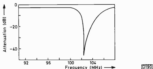
Fig. 1 (top left): Czech notch filter.
