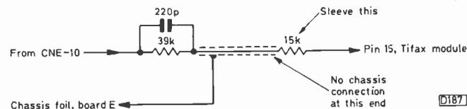
Fig. 9: Providing the line pulse required by the Tifax decoder.
