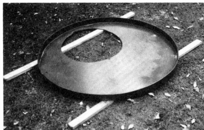
Photo 3: The now painted dustbin lid at rest on the wooden frame. Take care not to cut away the access hole lip too close to the main outside lip.
