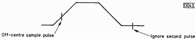
Fig. 12: Basic sample-and-hold circuit waveform.
