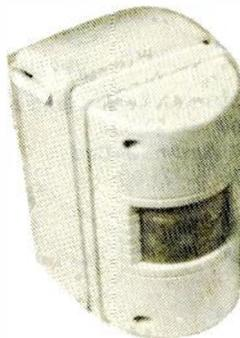
**ES36** This PIR (passive infra-red) detector reacts instantly to body heat and will activate lighting up to 600W when any person enters the detected zone. After a preset time it turns off. Detection range 110° x 12m long. Mounting angle adjustable 15° from vertical and ± 20° horizontal. Lighting adjustable from 5 secs to 10 minutes. Daytime lighting controllable. 230V operation, 600 watts max. Size 110 x 75 x 85mm.
