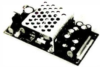
**Z5256** Switch mode PSU made by Tamura Corporation. Board 195x100mm with outputs on PCB pins. Input 120/240V ac; Outputs: +5V @ 7.5A; +12V @ 1.25A (2A peak); -12V @ 0.1A. All this for just **£12.95**
