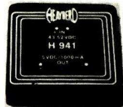
Two 5 watt regulators PCB mounting. DC-DC converters. These are encapsulated in a 51x51x10mm package with output pins on 0.1 pitch. These are ex-equip but guaranteed. Dp £59.75
