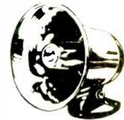
**A370** Gold coloured horn with fixing plate. Emits high powered wailing note of varying pitch. Output 115dB(A) at 3m. Power 12V DC, 1.5A. 130mm dia x 160mm. 160 cycles per minute.
