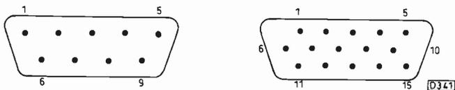
Fig. 1: 9-pin and 15-pin monitor connector plug configurations. See Table 1 for standard pin connections.
