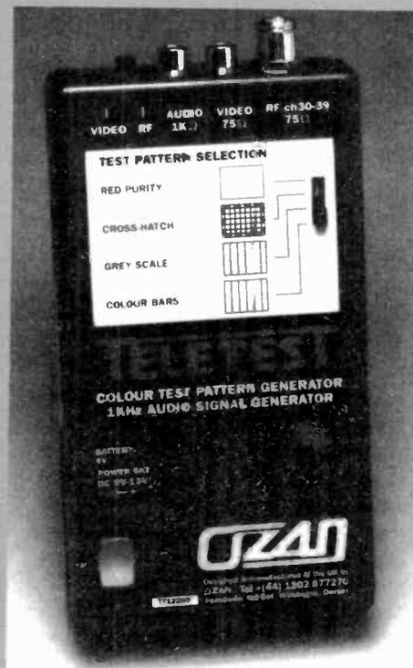
This month we have a Teletest TV test pattern and audio signal generator to give away in a free-to-enter prize draw. The Teletest is Ozan's popular battery-powered, hand-held test signal source for checking TV sets and VCRs.
