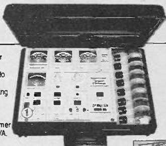
● **BMR 95** unique Regenerating-Computer and Analyser for CRTs, regenerates picture tubes even better, also if all other machines do not succeed, removes short filament-cathode-grid 1-grid 2, with FLASH-EX against remaining gas. 162 adapters available, list with 12,500 tubes-types, pays itself within 4 weeks.
