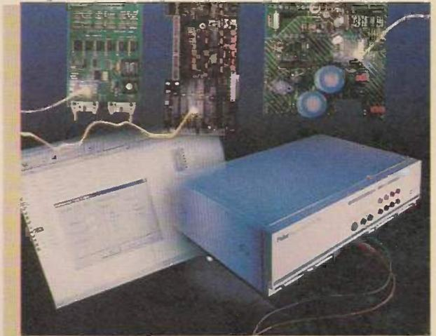
*Polar Instruments has introduced the PFL780 Windows '95-based PCB fault locator, which enables staff with very little experience of electronics to test and repair PCBs. The basic idea is to be able to change from the 'board-swapping' approach to component-level repairs, with consequent cost saving. For further details contact Polar Instruments Ltd., Garenne Park, St. Sampsons, Guernsey, Channel Islands GY2 4AF (01481 53 081).*
