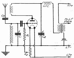
Fig. 2.—A modification of Fig. 1.—This is the throttle reaction control.
