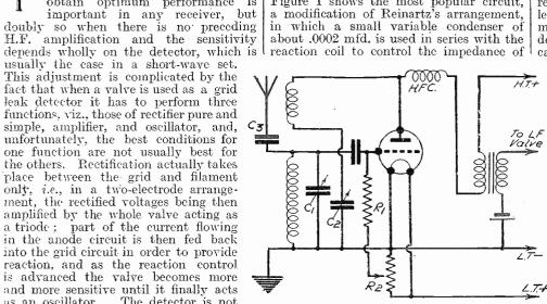
Fig. 1.—A simple reaction arrangement.
