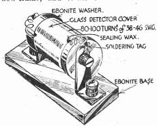
Making a short-wave choke from a crystal detector.
