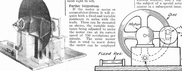
Variable Res: Fig. 2.—A rough layout of the disc model television apparatus.
