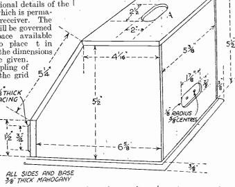
Fig. 5.—Details of cabinet for coupling absorption wavemeter.
