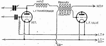
Fig. 22.—Method of feeding the L.F. valve through a transformer.
