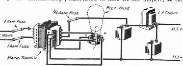
Fig. 15.—A rectifier unit showing suggested position of suses:
