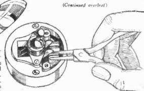
Fig. 2.—Sparking in wall switches may often be overcome by pinching the contacts closer together.
