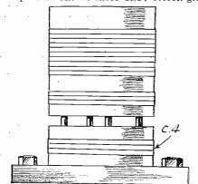
Fig. 4.-Mounting the coupling coil on the same base as the tuning coil.
