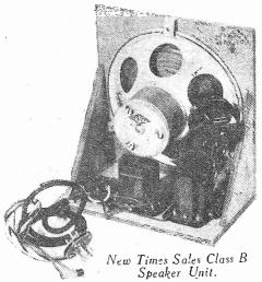
efficient Class B output choke. A tonecontrol condenser is fitted across the primary sections, to eliminate some of the higher frequencies and so give a slightly richer effect to music. The values chosen appear very suitable and certainly avoid the rather high pitched tone which is
