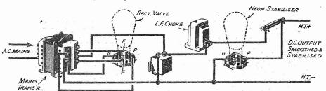
Fig. 14.—Adding a neon tube voltage stabilizer for an eliminator supplying a Class B valve.
