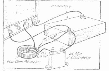
Fig. 5- Automatic grid bias can be provided in the manner shown above by making use of an old potentiometer.
