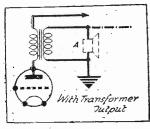
Wiring diagrams showing how a bell system may be used for speaker extensions.
