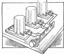
Fig. 3.--A convenient method of mounting the flat wave-change switch beside a set of coils.
