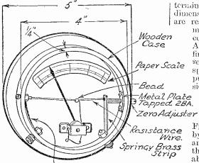
Connecting Strip Fig. 1.—Sketch of the finished hot-wire meter described : dimensions are only approximate.
