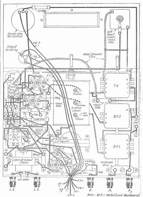
Fig. 6.—Complete wiring plan for the Nucleon Class B Four.
