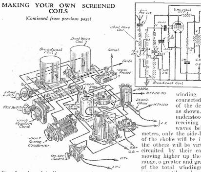
Fig. 5.-A useful all-wave two-value circuit using two of the coils described.
