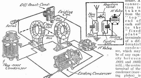
Fig. 1.—This sketch shows a simple means of converting the aerial not used. The tuning condenser of a re- tarkh ceiver to a simple band-pass arrangement. arrangement shown and do
