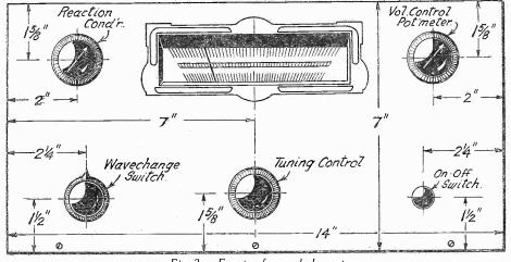
Fig. 2.-Front of panel layout.
