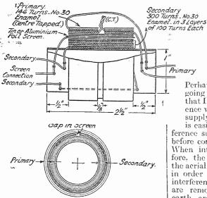
Fig., 3.—Details of the transformer.
