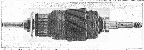
Fig. 5.—" Skewing" or inclining the armature slots of a television motor is sound practice.
