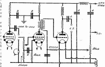
and Fig. 9.—A suggested arrangement for the L.F. side of a quality receiver.
