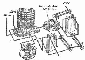
Fig. 5.—Gain control by variable-mu S.G. valve in a mains set.
