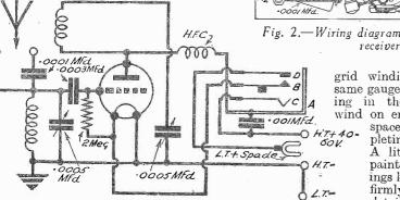
Fig. 3.-Theoretical circuit of the Pocket Portable.
