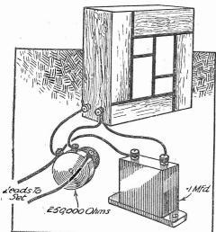
Fig. 1.—A simple system of effecting remote control of volume.
