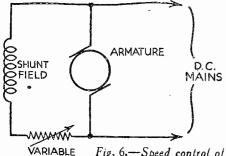
VARIABLE Fig. 6.—Speed control of RESISTANCE shunt motors is effected by using a variable resistance in series with the field winding. in the armature which hold the coils at an angle to the axis of the armature, and this is shown very clearly in Fig. 5, which depicts the armature of an actual motor I have used with great success in many of my experiments. This avoids certain periodic oscillation of the magnetic flux which is liable to cause sparking.
