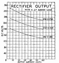
Fig. 2.-Regulation, or output curves for a typical Class A rectifying value. These are referred to in the text.
