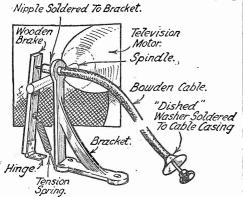
Simple speed regulator for a television motor.
