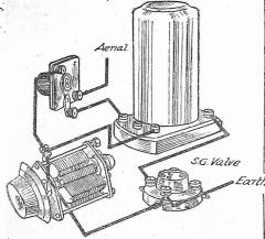
Fig. 3.—Employing a differential condenser for volume control.
