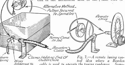
cable is used to operate the tuning condenser. Sometimes it is desirable to fit small pulleys on the condenser and drive spindles to obtain a better movement.
