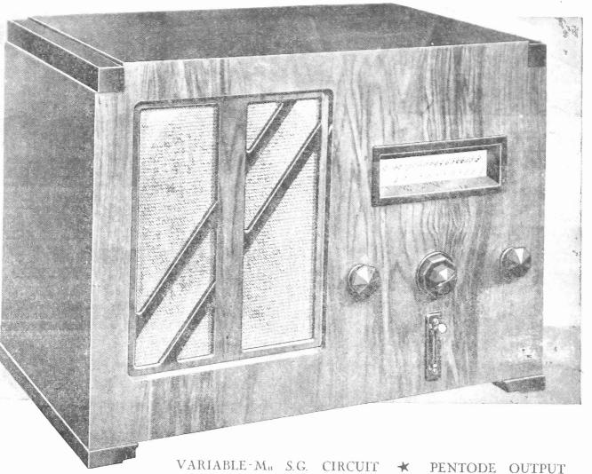
PENTODE DETECTOR \* ENERGISED MOVING COIL SPEAKER
