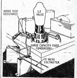
Fig. 5.—Measuring the A.C. volts developed across an anode feed resistance.
