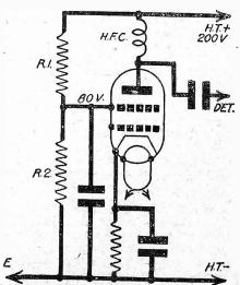
Fig. 4.—Several interesting points arise when calculating the values of resistances required for a fixed screening grid potentiometer.
