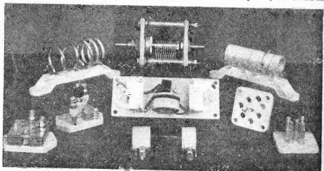
An interesting group of short-wave components in which every precaution has been taken to avoid losses. These B.T.S. components are characterised by silver-plated metal parts and ceramic material losses. for insulation purposes.
