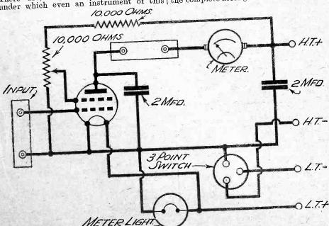
Fig. 2.—Theoretical circuit of the valve voltmeter.
