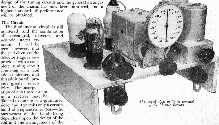
required for the modifications it is necessary first to consider to what stage you ultimately wish to take the receiver. In its final stage it will incorporate the superhet principle, but it is, as has been pointed out in the introductory articles, possible to leave the receiver at any stage and it will be complete in that form. modifications which are introduced this week will demand that a new chassis is obtained, in addition to an extra
