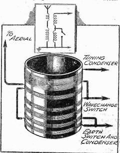
Fig. 1.—Showing aerial transformer coupling.
