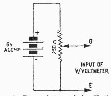
Fig. 3.—Theoretical circuit of the calibration apparatus.
