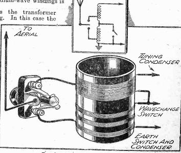
Fig. 2.—Tap method of aerial coupling.
