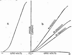
1.—The standard grid-volts/anode-current Fig. curve, and the effect of varying loads shown graphically.
