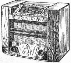
This is the Philips receiver in which the dial is hinged, and may be set at various angles without affecting the indicating mechanism.
