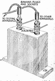
A method of making connections quickly for test purposes.
