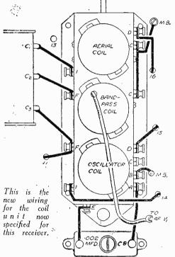
is not required, as the coils incorporate a special coupling winding and therefore hole number 13 is not used.
