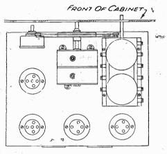
Fig. 3.—The set can be used as its own template by first making a hole for the longest spindle, and then marking the positions of the others, and drilling the holes in turn.
