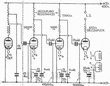
Fig. 2.—Where a succession of L.F. stages is employed, an efficient triode output valve should be used, and one with a large grid swing is necessary to avoid overloading.
