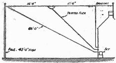
there has been a complete absence of signals. I have switched over to the Dipole and managed to hear one or two. Another advantage of the Dipole is that during windy weather signals are much more steady. Of course, it must be coupled up to the set by some means, and I find a transformer as follows the best way:—
