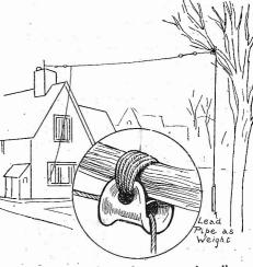
A method of suspending an aerial to allow for automatic adjustment.
