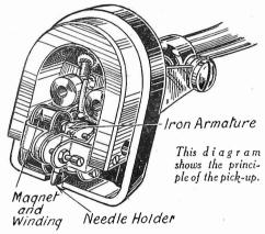
example of which is shown here, the magnet has usually two poles, and the needle is inserted into a holder which is extended and rests between the two poles. As the needle is moved by the sound grooves on the record, the armature moves, and this varies the magnetic field causing a varying current to flow in the windings. This current variation is applied to a valve, just as in the case of wireless signals, and so produces the signal.
