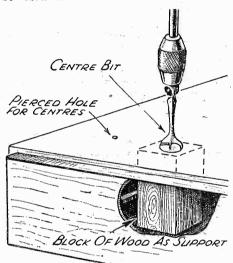
Fig. 2.—After making small centre holes from the inside of the cabinet full size holes should be traced out on the front, using a centre bit.
