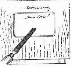
Fig. 4.—How the opening in the cabinet is finished off. The file is inclined.
