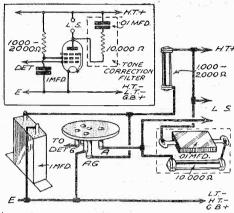
Fig. 5.—A pentode used with tone-correction filter and decoupler for the auxiliary grid.
