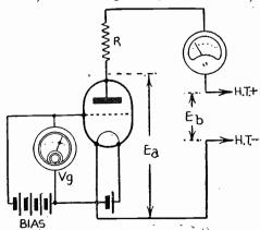
Circuit arrangement for taking dynamic curves or other valve data.
