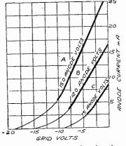
Fig. 1.—Anode-current-grid-volts characteristic curves for a typical small power valve. Straight portions of the "curve" are shown heavier to simplify reference.
