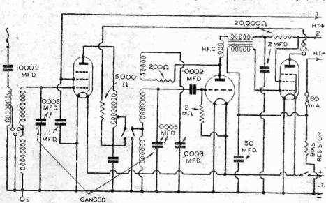
Fig. 3.—A three-valve circuit, with H.F. stage, which is more effective than the arrangement shown
