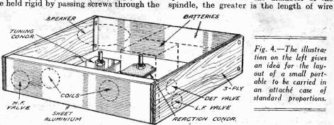
Fig. 4.—The illustra: tion on the left gives an idea for the layout of a small portable to be carried in an attaché case of standard proportions.
