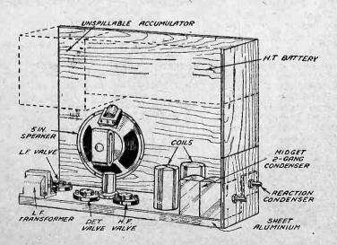
Fig. 2.—A suggested arrangement of parts when making a simple portable suitable for housing in a container similar in proportion to a gramophonerecord case. The drawing on the left is not necessarily to exact scale and the lay-out is intended mainly as a suggestion. How the finished set would appear is shown on the right.
