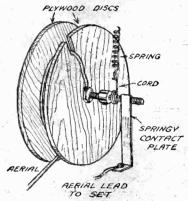
Fig. 5.—How a self-winding throw-out aerical can be made when the space permits. The "wheel" can be made when the space permits. The "wheel" should be as large as permitted by the design of the
