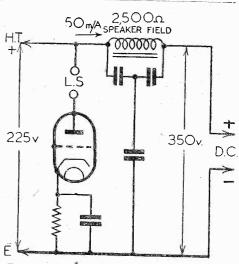
Fig. 6.—A speaker field winding produces a pronounced voltage drop.
