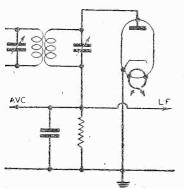
Fig. 1.—The basic circuit for automalic volume control, using a diode.
