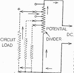
Fig. 4.—When a potential divider is used we have, in effect, a number of resistors in parallel with each other and with parts of the divider resistor.
