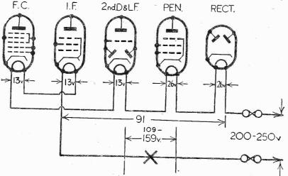
Fig. 5.—The allocation of voltages between the heaters of the valves in an A.C./D.C. circuit.
