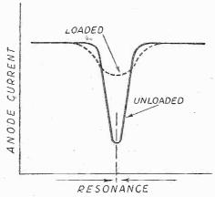
Fig. 2.—A typical anode current curve of a P.A.
