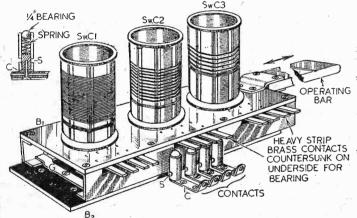
A coil switching unit to avoid coil changing.
