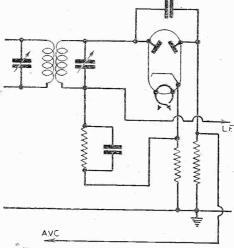
Fig. 2.—The basic form of delayed A.V.C.
