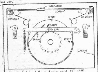
Fig. 2.—Details of the mechanism which is mounted on the side of the receiver casing.
