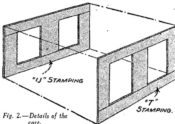
Fig. 2.—Details of the core.
