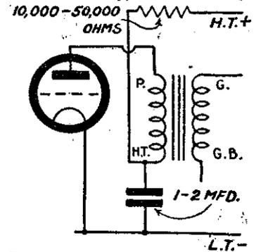
Fig. 5.—How to fit a decoupling resistance and condenser to stop motor-boating.
