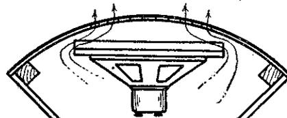
Fig. 3.—Plan of shelf of corner cabinet, showing how sound waves from back of speaker pass round the baffle.
