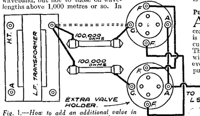
Fig. 1.—How to add an additional valve in parallel with an existing valve.
