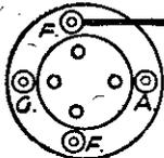
Fig. 4.—Always earth the filament terminal shown so that valves of the metallised type may be interchanged.
