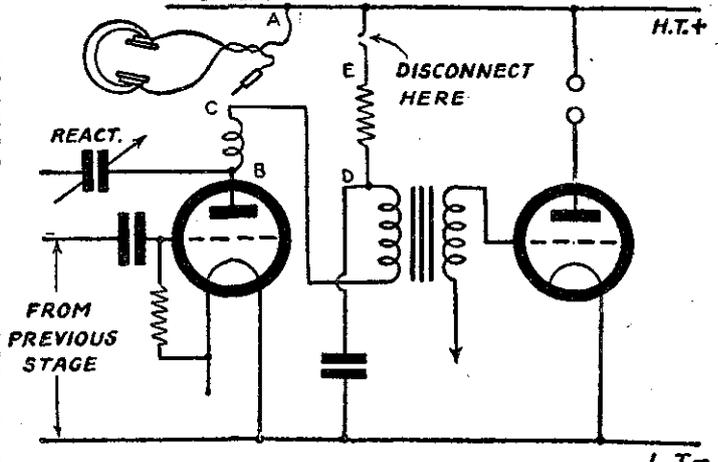
Fig. 9.—How to test for "crackling" noises. To test the H.F. and detector stages disconnect H.T. from E and join 'phones across A and B. To test H.F. choke as well join 'phones across A and C. To include transformer join them across A and D. To include decoupling resistance join across A and E.
