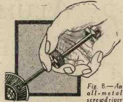
Fig. 8.—An all-metal screwdriver which is held in the palm of the hand.
