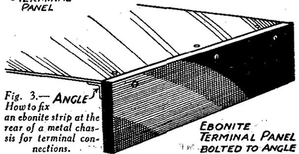
Fig. 3.—ANGLE How to fix an ebonite strip at the rear of a metal chassis for terminal connections.
