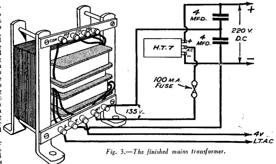
Fig. 3.—The finished mains transformer.
