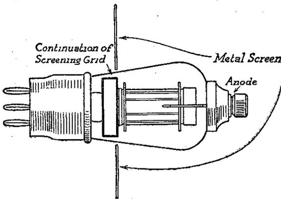
Fig. 3.—The screen should be level with the screening grid of the valve.
