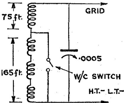
Fig. 1.—Diagram illustrating reply concerning frame aerial windings.
