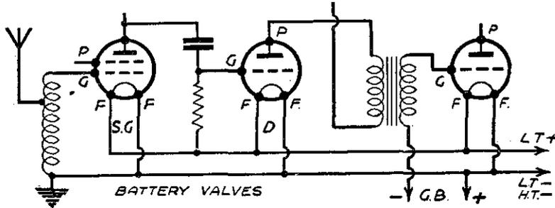
Fig. 3—Diagrams showing alterations required to a battery set when converting it for all A.C. operation.
