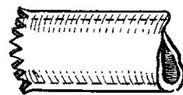
Fig. 9.—The cutting end of a wall drill.
