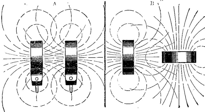
Fig. 1.—Showing the shape of the electro-magnetic field of coils of the usual plug-in type.
