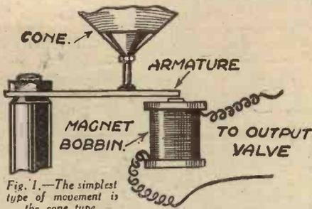
Fig. 1.—The simplest type of movement is the cone type.
