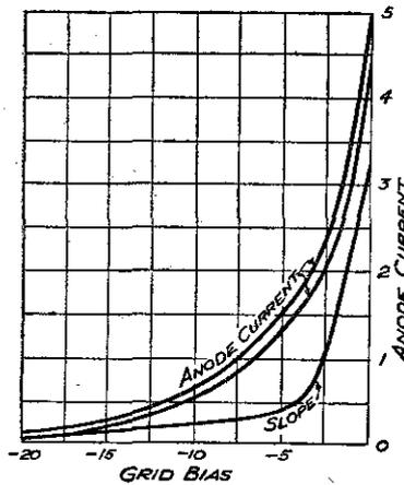
Fig. 1. The characteristic curve of the variable mu valve. Note the long, gentle slope caused by the irregularly spaced grid.
