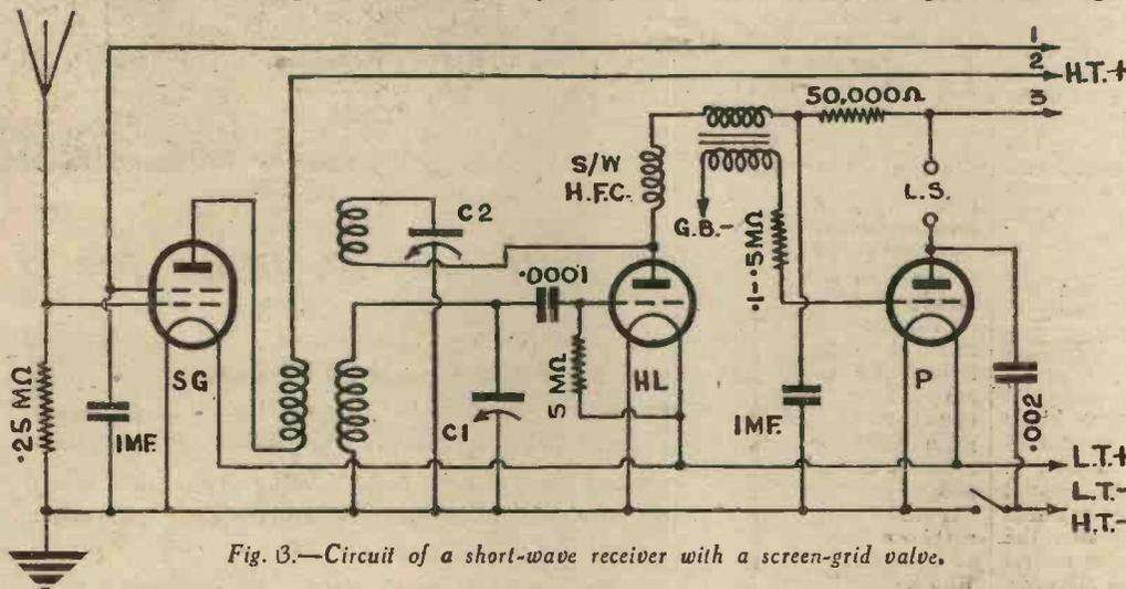
Fig. 3.—Circuit of a short-wave receiver with a screen-grid valve.
