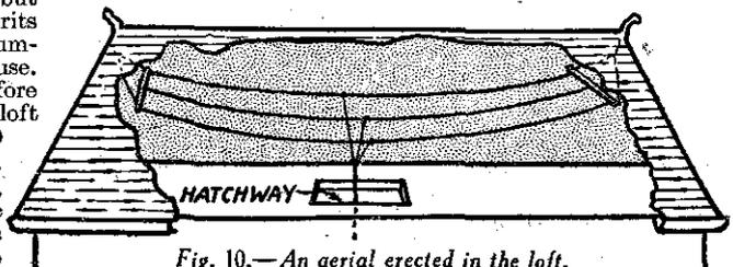
Fig. 10.—An aerial erected in the loft.
