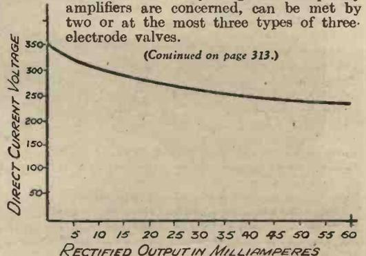
Fig. 3.—Typical performance curve of a rectifier valve.
