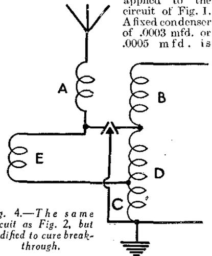
Fig. 4.—The same circuit as Fig. 2, but modified to cure break-through.
