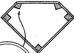
Fig. 10.—Plan of the same cabinet using home-made uprights. Inset shows how to cut uprights from square-sectioned stuff.
