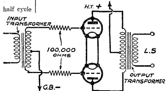
Fig. 3.—The circuit arrangement of push-pull valves, showing the resistances arranged for ensuring stability.
