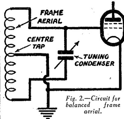
Fig. 2.—Circuit for balanced frame aerial.
