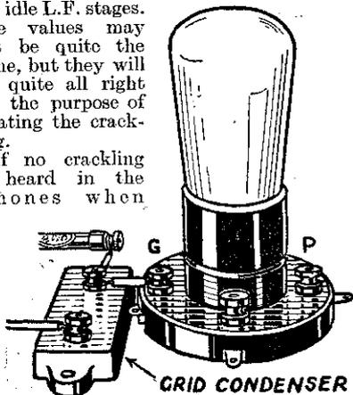
Fig. 8.—By placing the grid condenser close to the valve-holder the lead from grid to condenser is kept short—which makes for stability.
