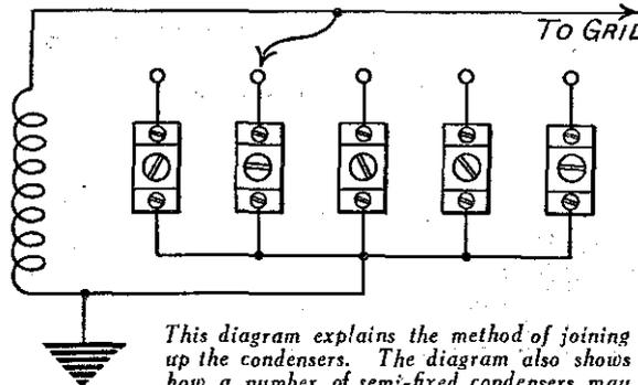
This diagram explains the method of joining up the condensers. The diagram also shows how a number of semi-fixed condensers may be connected up to enable the scheme described in this article to be carried out.
