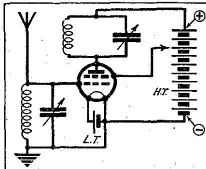
Fig. 3.—A screen-grid valve employing tuned-anode coupling.
