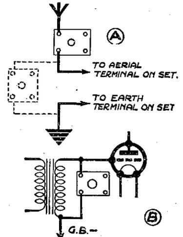
Fig. 2.—Two methods of using the control: (A) on the aerial circuit, and (B) across a transformer.
