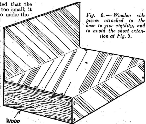
Fig. 6.—Wooden side pieces attached to the base to give rigidity, and to avoid the short extension at Fig. 5.
