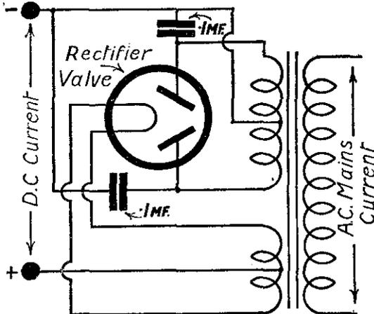
Fig. 1.—Rectifier hum can be cured by connecting two .1 mfd. fixed condensers between the two rectifier anodes and high-tension negative.
