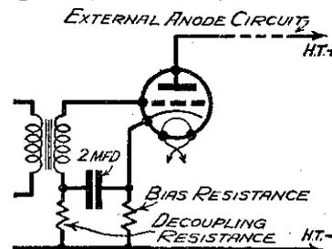
Fig. 2.—The arrangement of Fig. 1 with a de-coupling circuit added.
