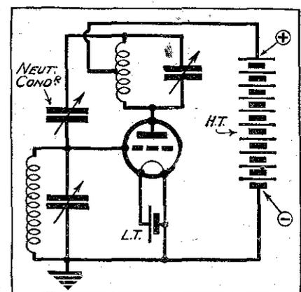
Fig. 2.—The well-known neurodyne method of H.F. coupling.
