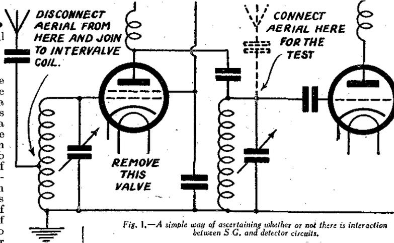
Fig. 1.—A simple way of ascertaining whether or not there is interaction between S.G. and detector circuits.
