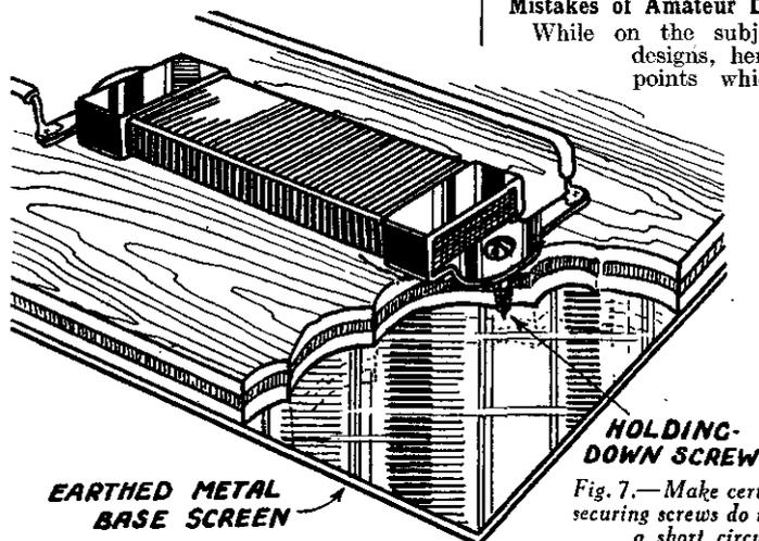
Fig. 7.—Make certain that securing screws do not cause a short circuit.
