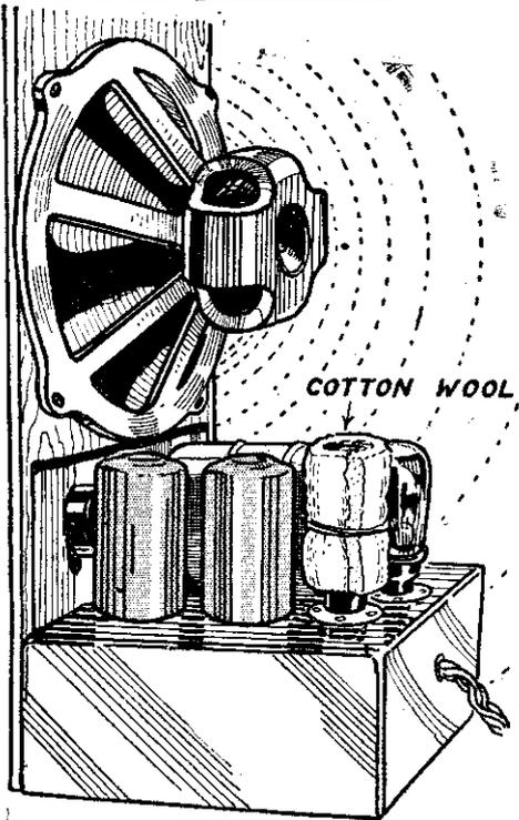
Fig. 1.—A jacket of cotton wool round the detector valve, so as to prevent sound waves from the speaker impinging on it, will often stop a microphonic howl.
