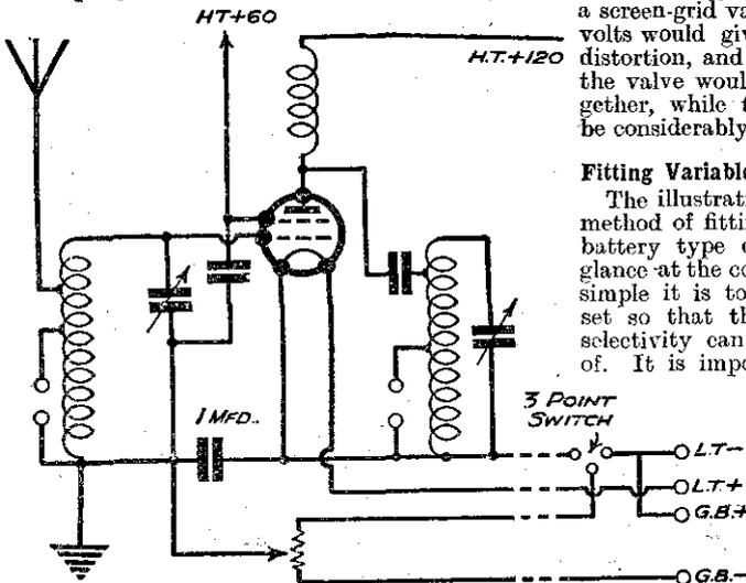
Fig. 2. The method of fitting variable bias to a battery type of variable mu.
