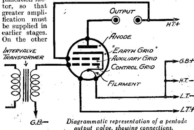
Diagrammatic representation of a pentode output valve, showing connections.
