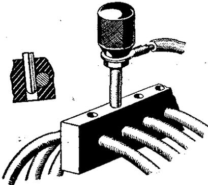
Simple method of tapping short-wave coils.
