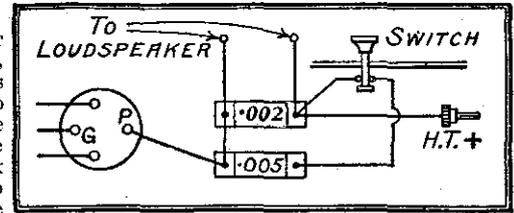
Showing how an additional condenser can be used for smoothing purposes.
