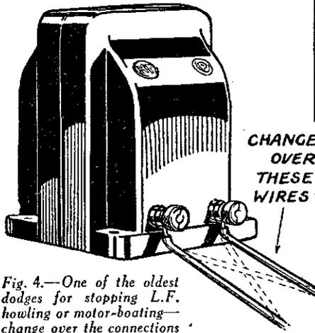
Fig. 4.—One of the oldest dodges for stopping L.F. howling or motor-boating—change over the connections to one of the windings of the L.F. transformer as shown by dotted lines.
