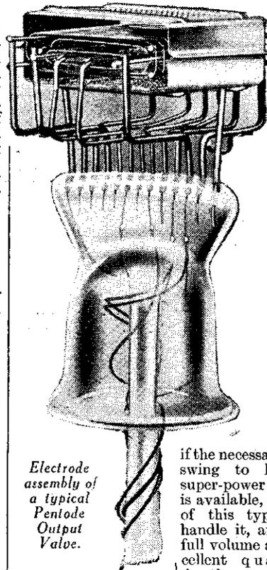
Electrode assembly of a typical Pentode Output Valve.
