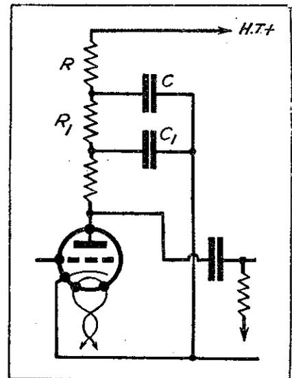
Fig. 6.—R.C.C. stage with double decoupling by resistance R and R<sub>1</sub>, C and C<sub>1</sub>.
