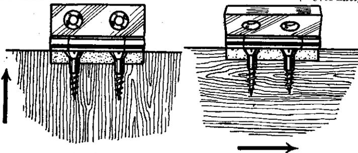
Fig. 8.—Incorrect and correct methods of fixing hinges.
