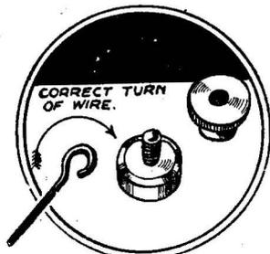
Bend the wire in a clockwise direction, as shown, and the terminal nut will then grip the wire tighter round the thread.
