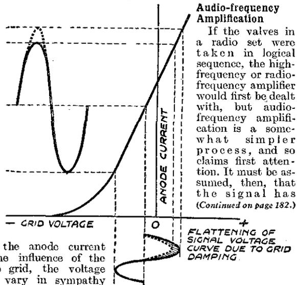
Indicating the result of under-biasing an amplifying valve. The grid becomes positive with respect to the filament during a part of the alternate half cycles. Grid current flows and reduces the effective signal, as shown by the shaded arcs, while the effect on the anode current is shown at the top left of the diagram.
