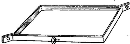
Fig. 7.—Clip for attaching a pulley direct to a chimney.
