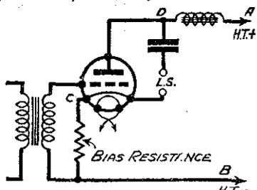
Fig. 1.—A resistance inserted in the cathode lead of an indirectly-heated valve.
