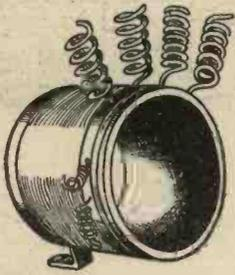
Fig. 1.—The single layer wound solenoid coil.
