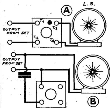
Fig. 3.—(A) Using the control to modify the volume at the speaker, and (B) converted as a tone control.
