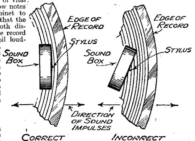
The “tracking” angle—which was fully explained in a recent issue. Note how the sound-box or pick-up must be parallel with the sound grooves.
