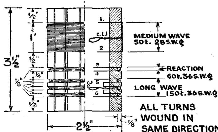
Fig. 1.—Constructional details of a tuner made on an eight-ribbed 2 1/2in. diameter ebonite former.
