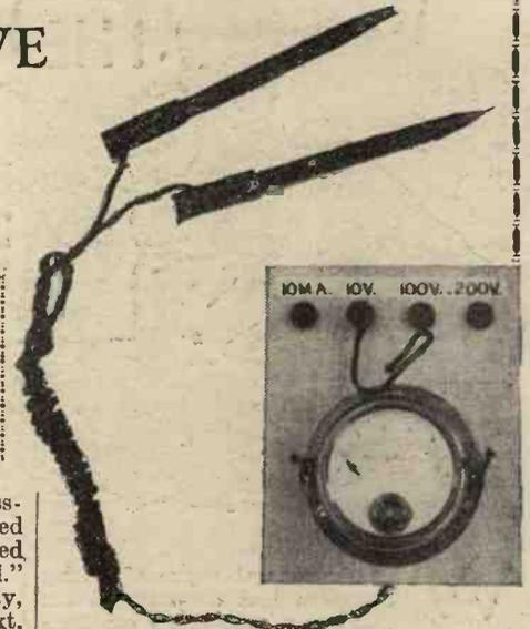
Fig. 2.—The complete four-range test meter with test prods.
