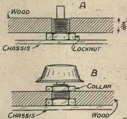
Recessing a panel to take back nuts on components.
