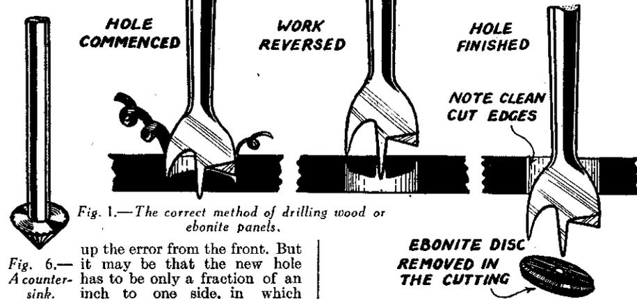
Fig. 1.—The correct method of drilling wood or ebonite panels.
