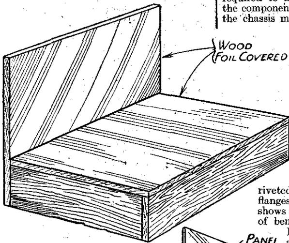
Fig. 1.—A simple way of making a "metal" chassis. A wooden frame-work covered with metal foil.
