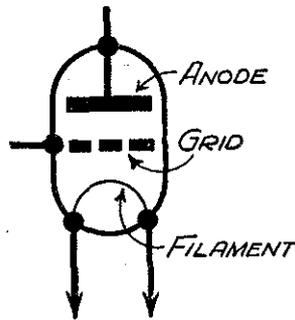
Fig. 3.—Conventional diagram of a three-electrode valve, indicating the essential parts.
