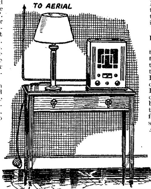
Fig. 8—One cause of hum is the aerial, earth or speaker leads, running parallel to the supply mains.
