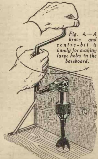
Fig. 4.—A brace and centre-bit is handy for making large holes in the baseboard.
