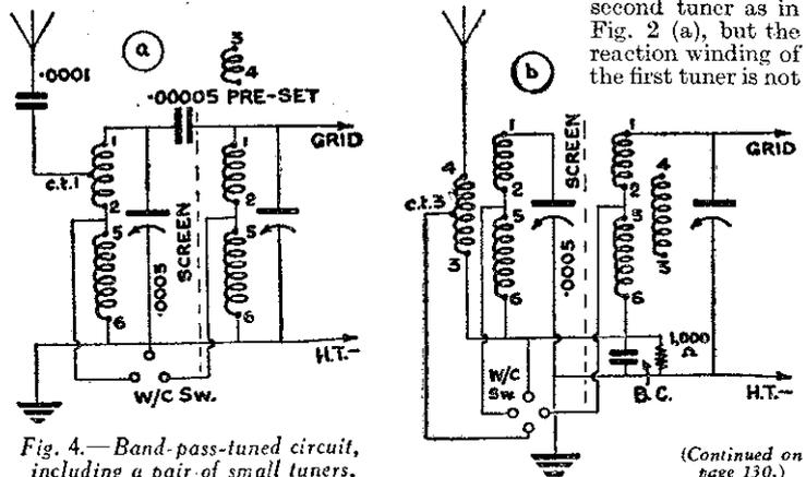
Fig. 4.—Band-pass-tuned circuit, including a pair of small tuners.
