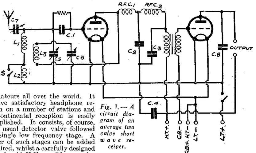
Fig. 1.—A circuit diagram of an average two valve short wave receiver.
