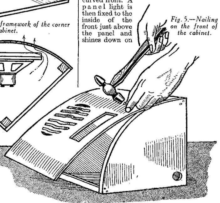
Fig. 5.—Nailing on the front of the cabinet.
