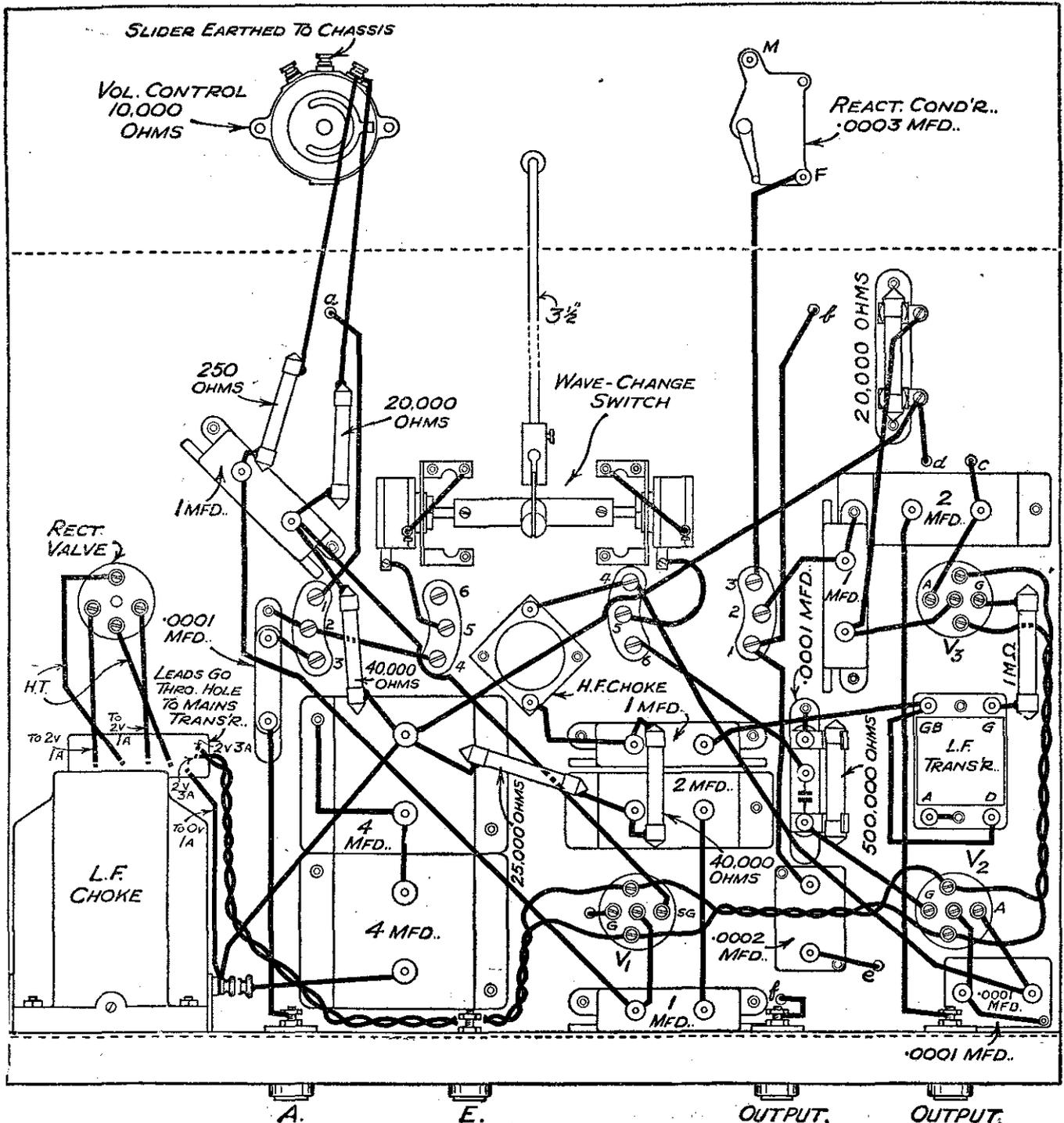
Beneath chassis wiring diagram of the Mains Express Three.
