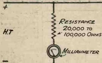
Fig. 2.—Measuring H.T. eliminator voltage with a milliammeter and a resistance of known value.
