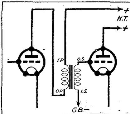
Fig. 2a.—Transformer primary directly in anode circuit.
