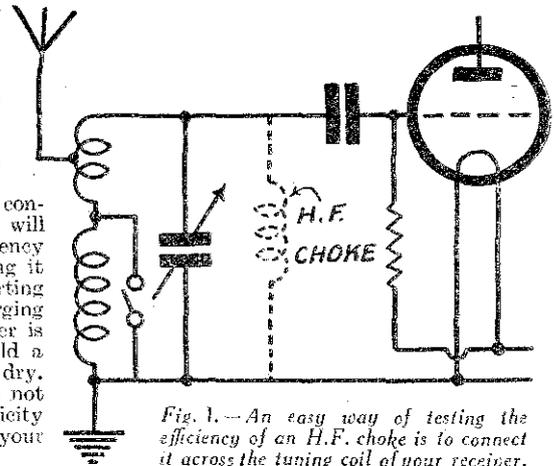
Fig. 1.— An easy way of testing the efficiency of an H.F. choke is to connect it across the tuning coil of your receiver.
