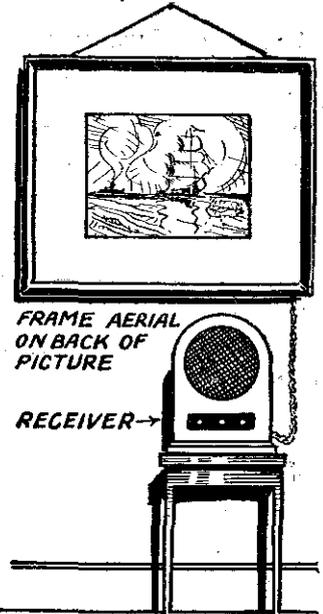
Figs. 5, 6 and 7.—A picture frame can be easily adapted to accommodate an aerial.
