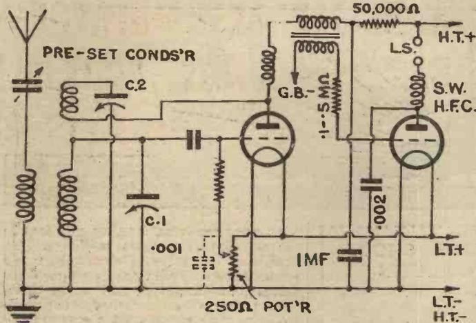
Fig. 2.—A good two-valve short-wave circuit.
