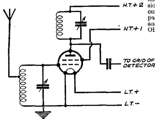
A circuit diagram of a screen-grid-H.F. stage.
