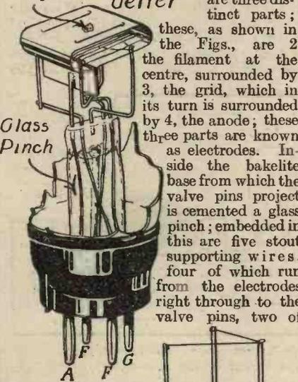
Fig. 1.—Internal parts of a modern valve.
