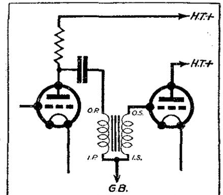
Fig. 2b.—Parallel-fed transformer. With this arrangement no battery current passes through the primary.
