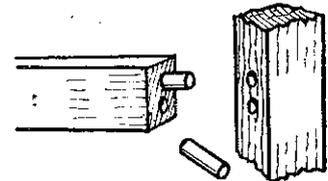
Fig. 15.—The framing rails are fixed to the legs with dowels.
