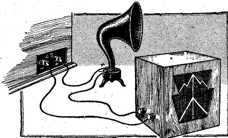
Balancing reproduction by means of two loud-speakers connected in series.
