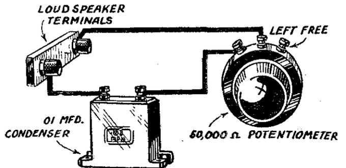
Fig. 10—A high-note filter—a cure for whistle, caused by heterodyning.
