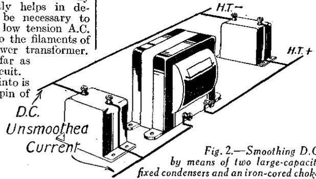
Fig. 2.—Smoothing D.C. by means of two large-capacity fixed condensers and an iron-cored choke.
