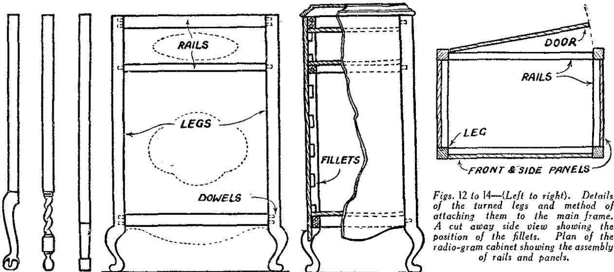
Figs. 12 to 14—(Left to right). Details of the turned legs and method of attaching them to the main frame. A cut away side view showing the position of the fillets. Plan of the radio-gram cabinet showing the assembly of rails and panels.
