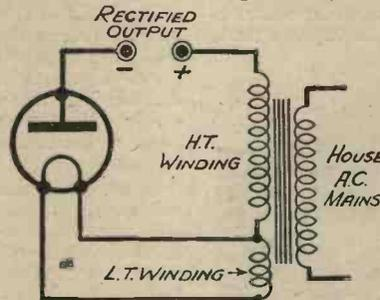
Fig. 1.—The "diode," or two-electrode valve, used as a rectifier in an A.C. mains set.
