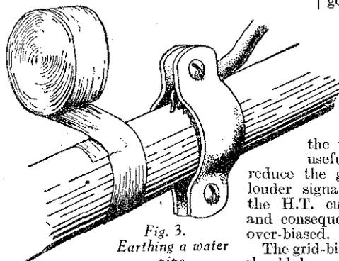
Fig. 3. Earthing a water pipe.
