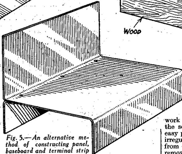
Fig. 5.—An alternative method of constructing panel, baseboard and terminal strip in one piece.
