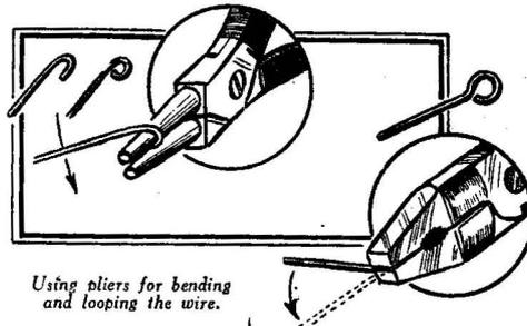
Using pliers for bending and looping the wire.
