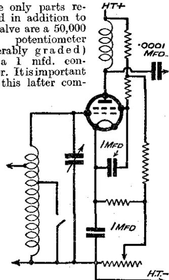
Fig. 3. The method of arranging the bias on an indirectly heated mains valve.
