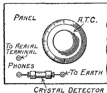
The crystal detector, together with two telephone terminals, can be mounted permanently on the panel, as shown in the sketch, one terminal being connected to the aerial terminal of the set, and the other to one end of the crystal detector. The other side of the crystal detector is connected to the earth terminal.
