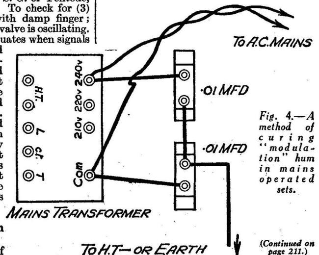
Fig. 4.—A method of curing "modulation" hum in mains operated sets.
