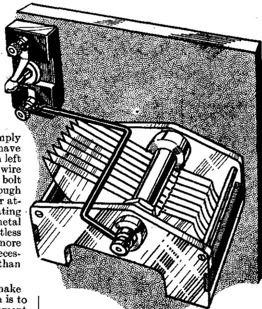
Fig. 9.—Don't let connecting wires foul the condenser vanes.
