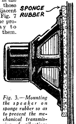
Fig. 3.—Mounting the speaker on sponge rubber so as to prevent the mechanical transmission of vibrations to the set itself.
