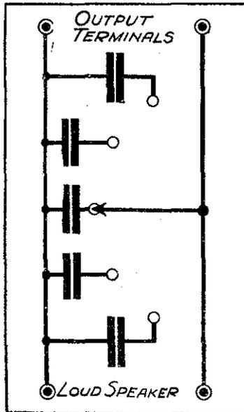
Fig. 1.—How to arrange a number of fixed condensers across the output terminals to vary the tone.
