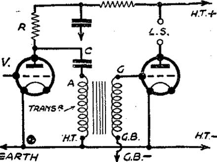
Fig. 2.—The method of parallel-feeding a transformer.
