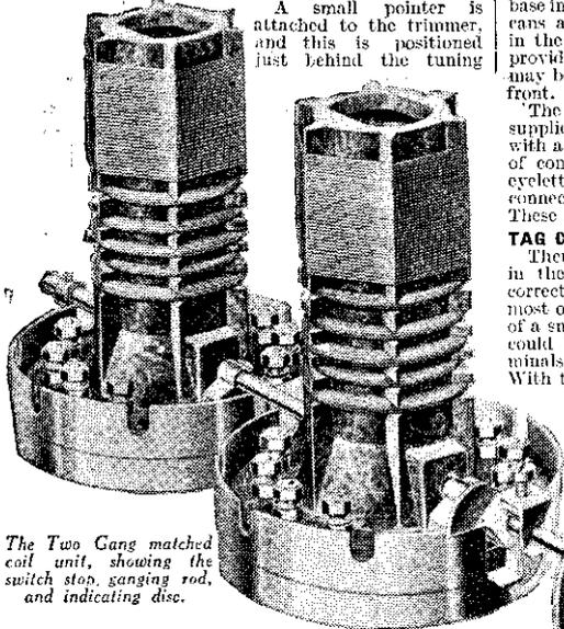
The Two Gang matched coil unit, showing the switch stop, ganging rod, and indicating disc.
