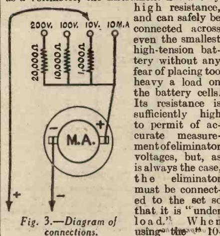
Fig. 3.—Diagram of connections.
