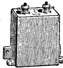
A 2 mfd. Non-inductive T.C.C. Condenser. Price 3/10d. Made in capacities from .01 to 2 mfd. prices 1/10 to 3/10. Working voltage 200 D.C.
