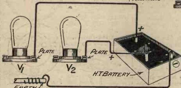
Fig. 1.—The high resistance of the shaded part of the battery will give rise to motor-boating or "feeding back."
