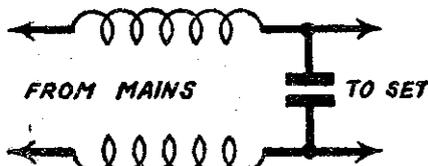
Fig. 4.—A cure for H.F. interference via the mains.
