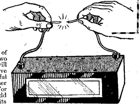
Fig. 3.—Testing the state of a H.T. battery.
