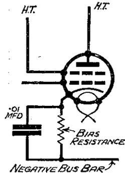
Fig. 5.—The biasing resistance arranged in the cathode lead of an S.G. valve.
