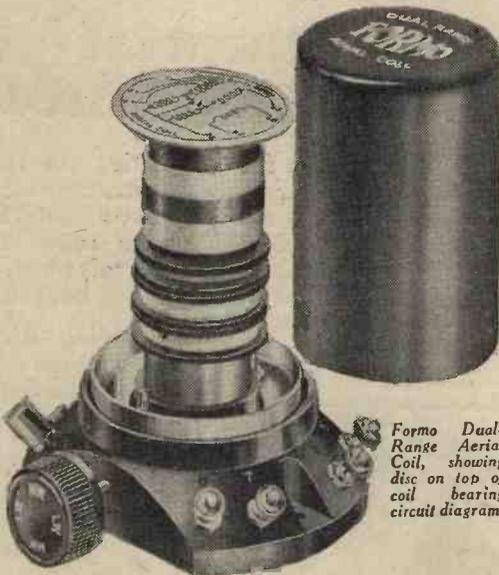
Formo Dual-Range Aerial Coil, showing disc on top of coil bearing circuit diagram.
