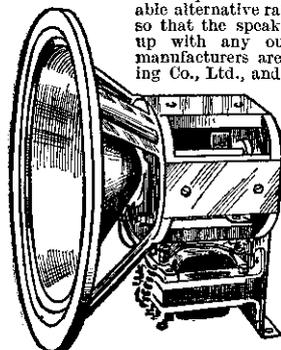
A permanent magnet moving-coil loud-speaker with transformer incorporated.
