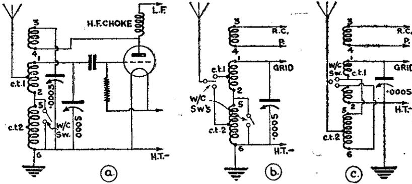
Fig. 2.—Three methods of connecting the tuner shown in Fig. 1 into a detector circuit.
