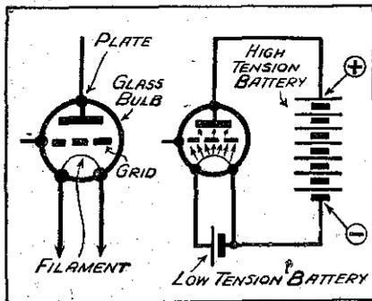
Fig. 1.—The wireless valve, and a diagram of the way in which the electron stream is emitted.
