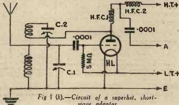
Fig. 1 (b).—Circuit of a superhet. short-wave adaptor.
