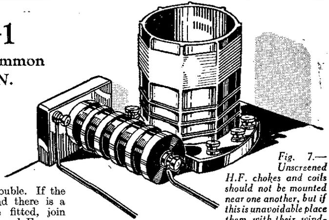
Fig. 7.—Unshielded H.F. chokes and coils should not be mounted near one another, but if this is unavoidable place them with their windings at right angles to prevent interaction and H.F. howling.
