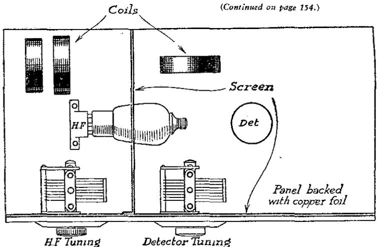
Fig. 2.—A screen the same depth as the baseboard is used for "partitioning off" the H.F. stage.
