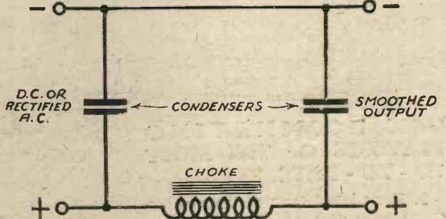
Fig. 2.—A choke connected up in a typical smoothing circuit.
