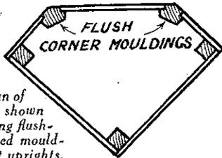
Fig. 9.—Plan of the cabinet shown in Fig. 8, using flush-fitting rebated mouldings for front uprights.
