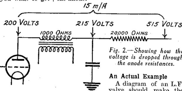
Fig. 2.—Showing how the voltage is dropped through the anode resistances.
