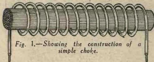
Fig. 1.—Showing the construction of a simple choke.
