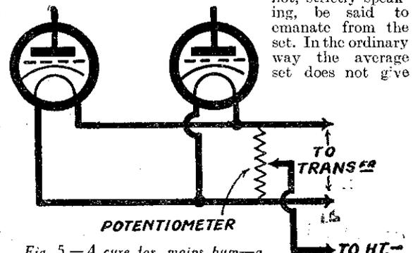
Fig. 5.—A cure for mains hum—a potentiometer is connected across the heater supply wiring.
