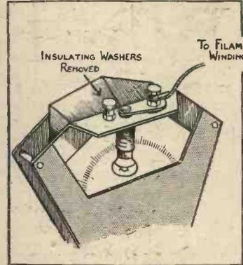
A neat method of fixing a bulb for an illuminated dial.
