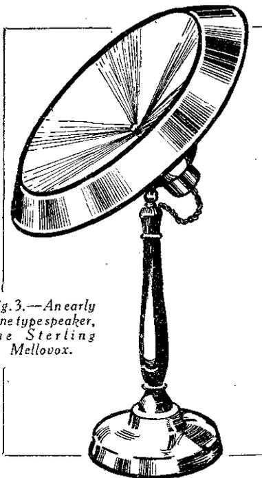
Fig. 3.—An early cone type speaker, the Sterling Mellovox.
