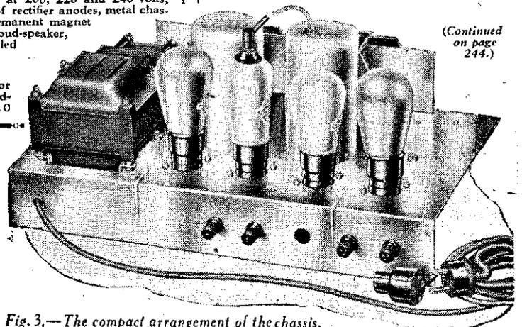
Fig. 3.—The compact arrangement of the chassis.
