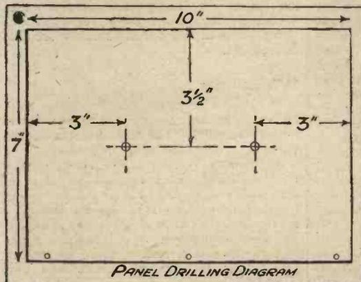
Fig. 2.—How to drill the panel.
