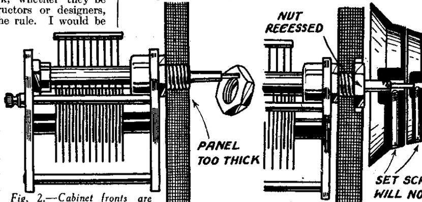
Fig. 2.—Cabinet fronts are often so thick that it is impossible to screw on the locking nuts. Cabinet makers ought to study these points.
