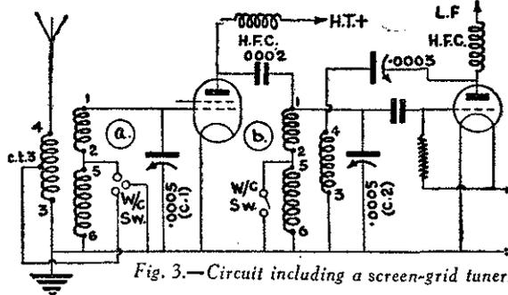
Fig. 3.—Circuit including a screen-grid tuner.
