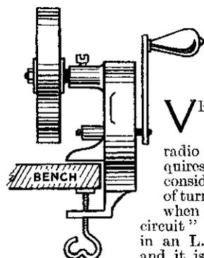
Fig. 1—The grindstone before conversion to a coil winder.
