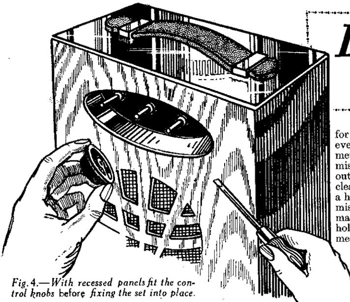
Fig. 4.—With recessed panels fit the control knobs before fixing the set into place.
