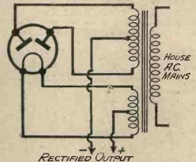
Fig. 2.—Rectifying valve with two anodes fed from a centre-tapped transformer.
