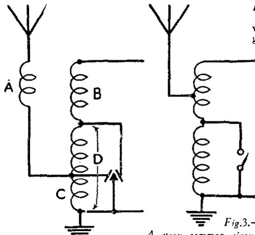
Fig. 2.—Another typical dual-range circuit. A very common circuit employed in commercial coils. Break-through does not occur, but it is unselective on the long waves.
