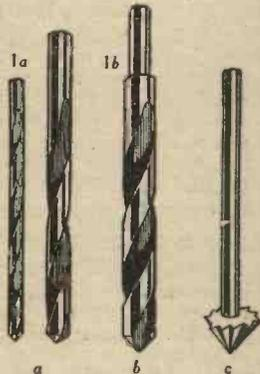
Fig. 1.—Ordinary twist drills; one with a shouldered shank; and a rose bit.
