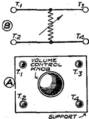
Fig. 1.—(A) The volume control, and (B) its circuit arrangement.
