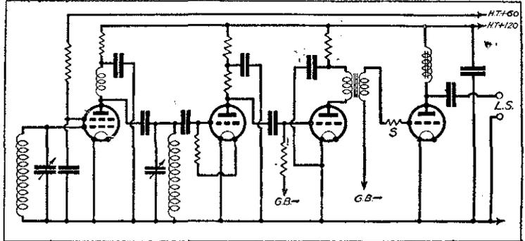
Fig. 7.—A typical four-valve circuit showing the method of inserting the decoupling resistances.
