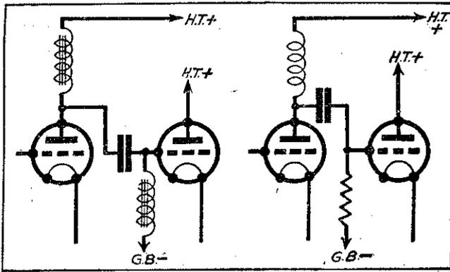
Fig. 3.—Two forms of choke coupling.
