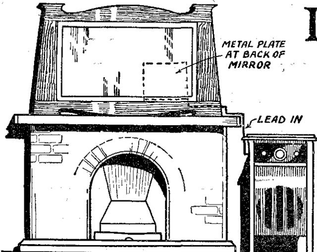
Fig. 3.—The metal backing of an ordinary mirror as an aerial.
