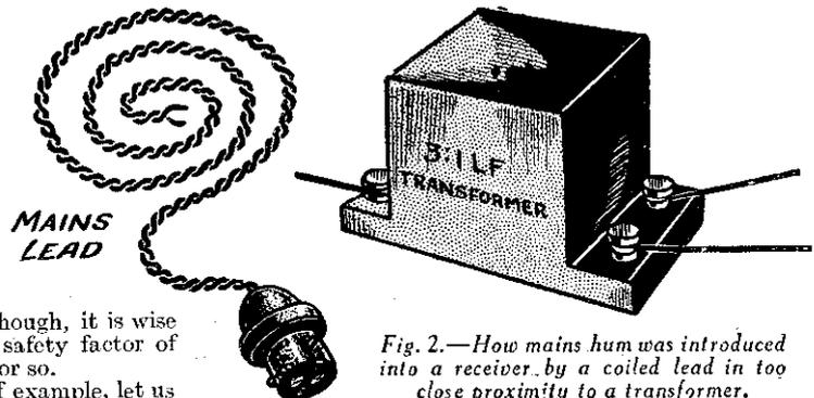
Fig. 2.—How mains hum was introduced into a receiver by a coiled lead in too close proximity to a transformer.
