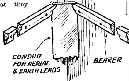
Fig. 7.—Wall bearers support the base of the cabinet—and aerial and earth leads are concealed by a wooden strip in the corner.
