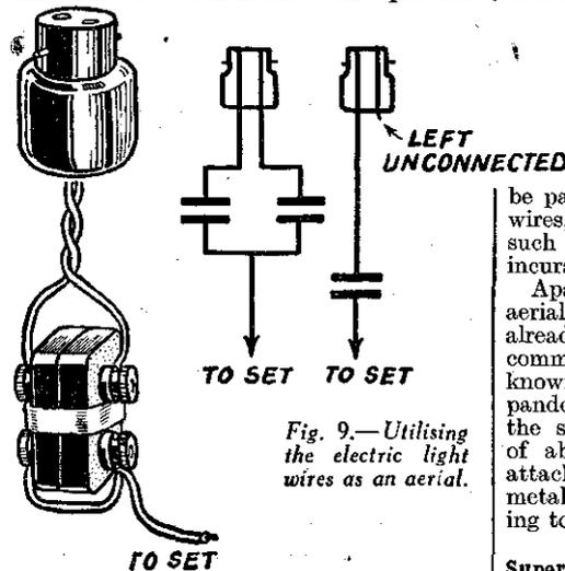
Fig. 9.—Utilising the electric light wires as an aerial.
