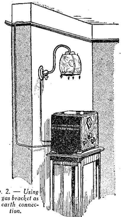
Fig. 2.—Using the gas bracket as an earth connection.
