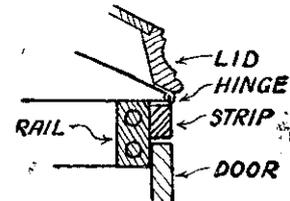
Fig. 16.—How the lid is hinged.
