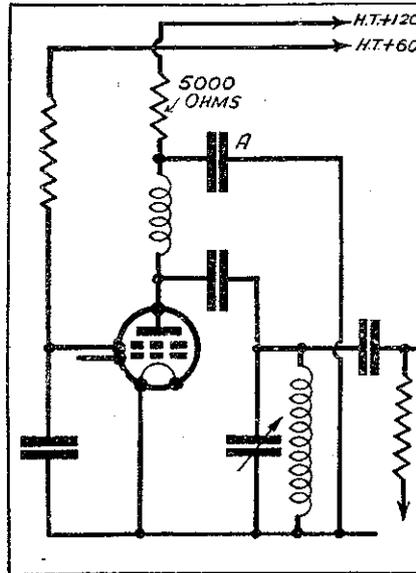
Fig. 4.—S.G. stage decoupled.
