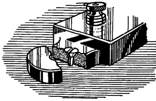
Fig. 5.—Use of the wrong screw will cause this! Don't use countersunk screws unless the lug hole is countersunk.
