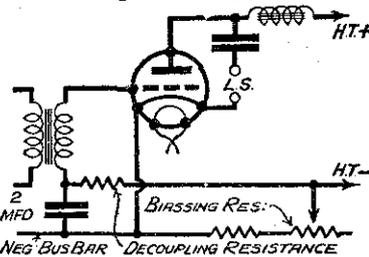
Fig. 3.—An alternative arrangement of Fig. 2, in which the cathode is maintained at the normal negative potential.
