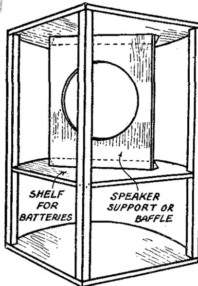
Fig. 2.—The main framework of the corner cabinet.
