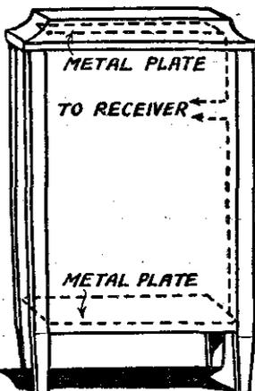
Fig. 8.—A radio-gram cabinet containing aerial and earth plates.
