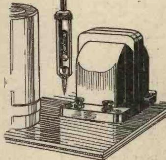
Fig. 6.—A special screw-driver which grips the head of a screw.
