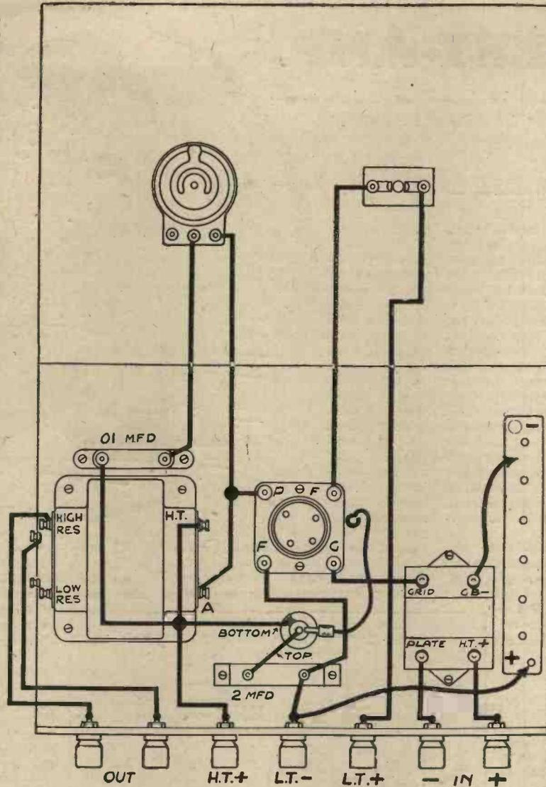
Fig. 4.—Wiring diagram of the Pent-Amp.
