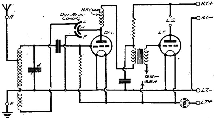
Fig. 2.—Circuit of a two-valve receiver.
