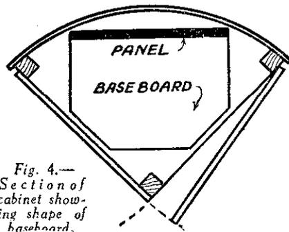
Fig. 4.—Section of cabinet showing shape of baseboard.
