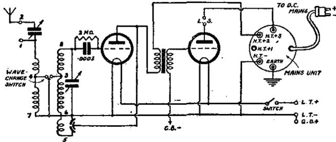
Fig. 1.—The circuit of the battery set before conversion.
