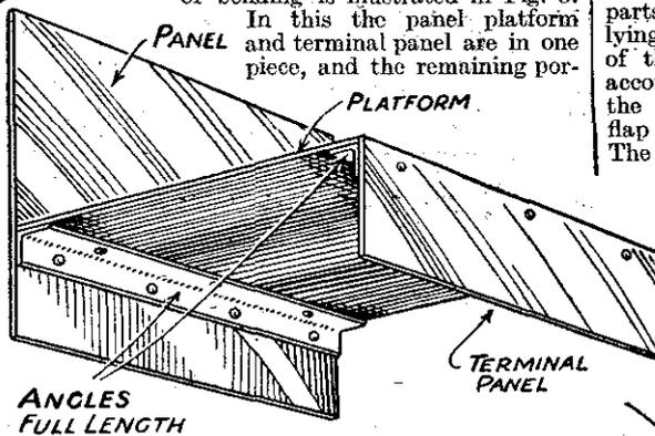
Fig. 2.—A metal chassis using angle-irons instead of bending the aluminium.
