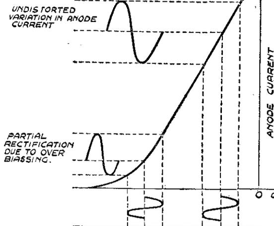
Showing relation between the grid voltage and the anode current in a valve and indicating correct biasing and how distortion is introduced by over-biasing.
