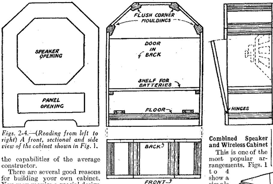
Figs. 2-4.—(Reading from left to right) A front, sectional and side view of the cabinet shown in Fig. 1.
