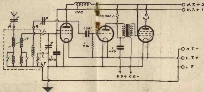
Fig. 1. Circuit Diagram of the Bijou.
