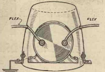
An efficient improvised screen for small H.F. chokes.
