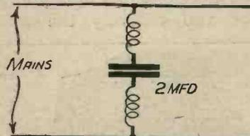
Fig. 1.—A simple device for removing interference from the mains.
