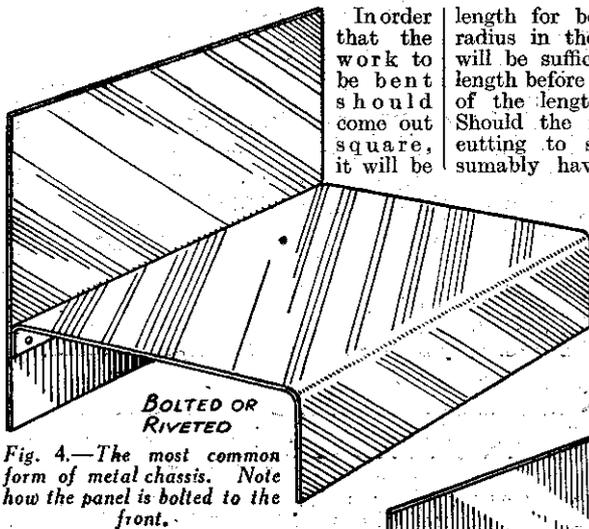
Fig. 4.—The most common form of metal chassis. Note how the panel is bolted to the front.
