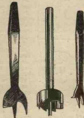
Fig. 5.—Centre-bits, and a panel cutter.
