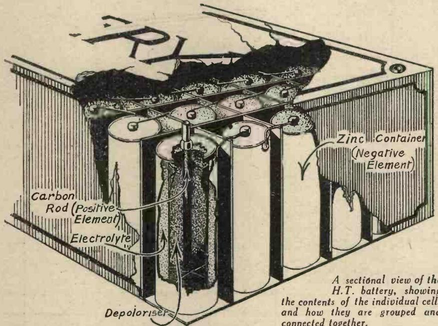
A sectional view of the H.T. battery, showing the contents of the individual cells and how they are grouped and connected together.
