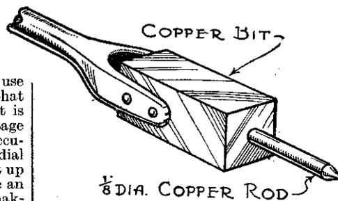
How to fit a small bit to your soldering iron.
