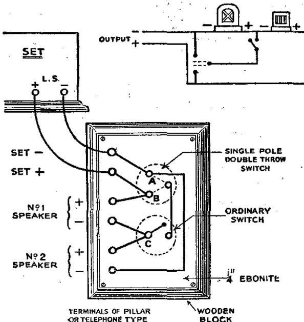
A method of switching loud-speakers. Glazite or similarly insulated wire at back of ebonite. Wiring looped in at points A, B and C.
