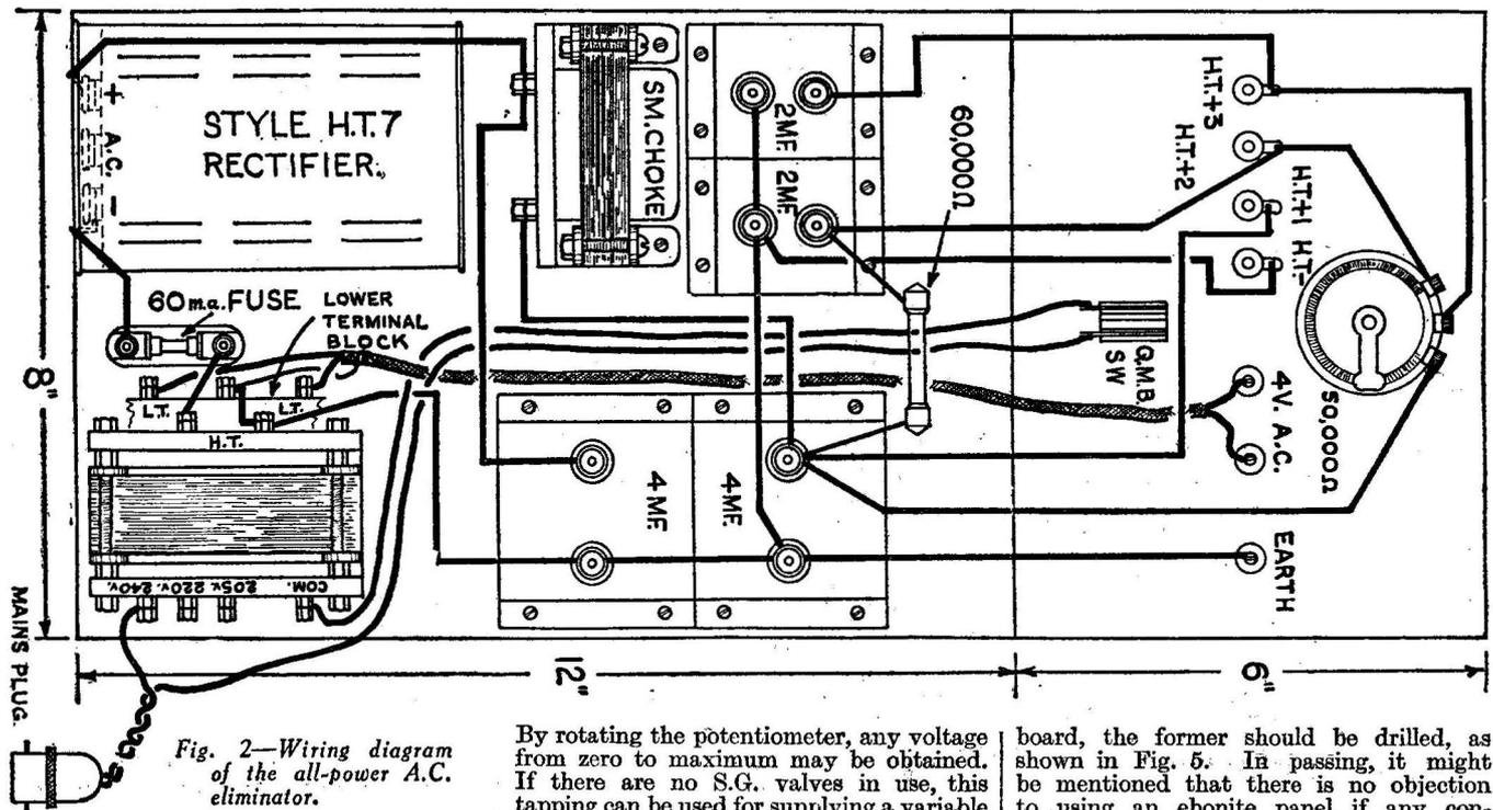
Fig. 2—Wiring diagram of the all-power A.C. eliminator.
