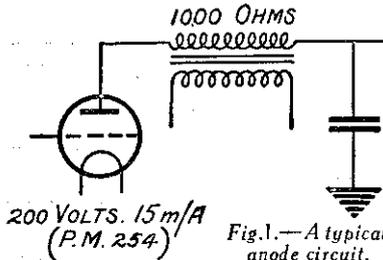
Fig. 1.—A typical anode circuit.
