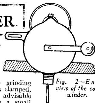
Fig. 2—End view of the coil winder.
