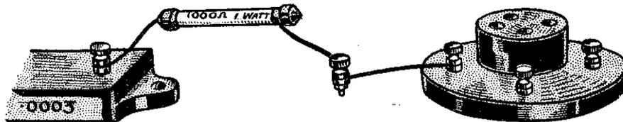
Fig. 1.—Using an extension lead to facilitate the connection of wire-end resistances.
