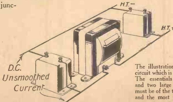
The illustration to the left shows the smoothing circuit which is required in every type of eliminator. The essentials are a high inductance L.F. choke and two large capacity fixed condensers. These must be of the type made to withstand high voltages, and the most useful value is 4 mfd.
