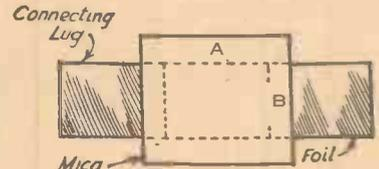
The method of calculating the capacity of a condenser is typified in the above diagram. It will be seen that a certain proportion of each pair of plates overlaps, and this is known as the "effective" surface. The area of this surface should be ascertained—by multiplying A by B—and this should be employed in conjunction with the formula for capacity given in the centre column.
