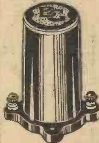
is given by this H.F. Choke. Highly finished, non-corrodible moulded case, mechanically strong, and dust and damp proof. Inductance, 128,000 micro-henries; self-capacity, 4.5 micromicrofarads; D.C. resistance, 400 ohms. Price **5/6**
