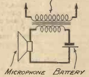
Fig. 2.—The microphone circuit.
