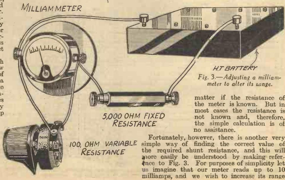
Fig. 3.—Adjusting a milliammeter to alter its range.
