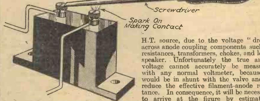
Fig. 11.—Discharge condensers before examining the inside of a set.
