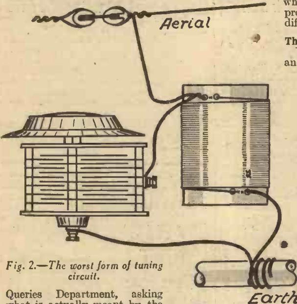
Fig. 2.—The worst form of tuning circuit.
