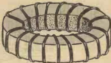
Fig. 6.—A diagram showing the method of making up a Ferrocort coil.
