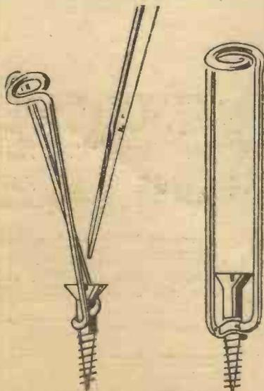
A simple wire clip for holding screws in awkward places.
