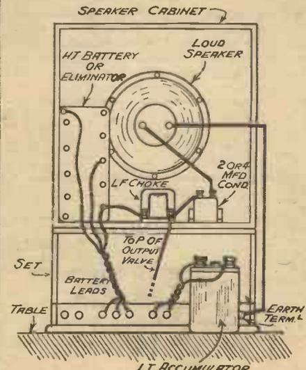
Accommodating the batteries and output filter.
