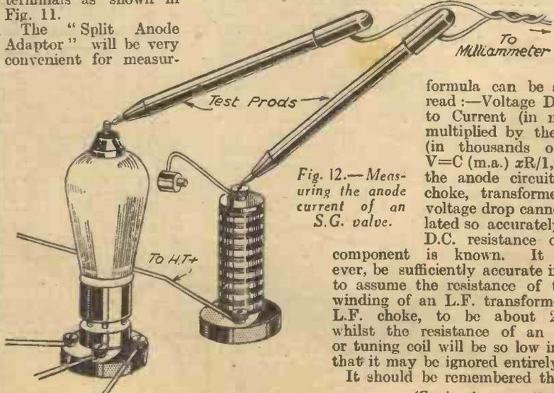
Fig. 12.—Measuring the anode current of an S.G. valve.
