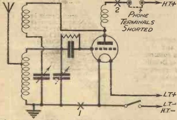
Fig. 1.—A standard one-valve set and the points to alter for transmission.
