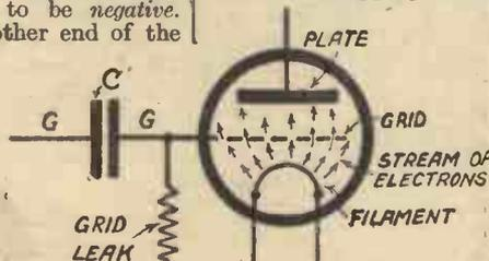
Fig. 4.—The normal electron flow inside the valve.
