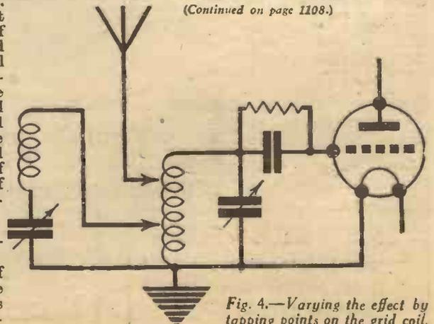
Fig. 4.—Varying the effect by tapping points on the grid coil.
