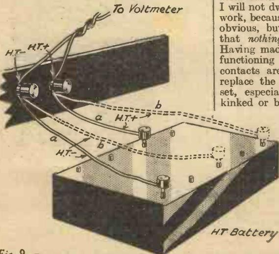
Fig. 9.—Testing an H.T. battery, with a low-reading voltmeter.
