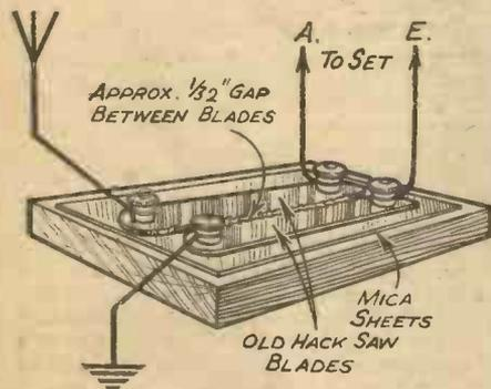
Using hacksaw blades for a lightning arrester.
