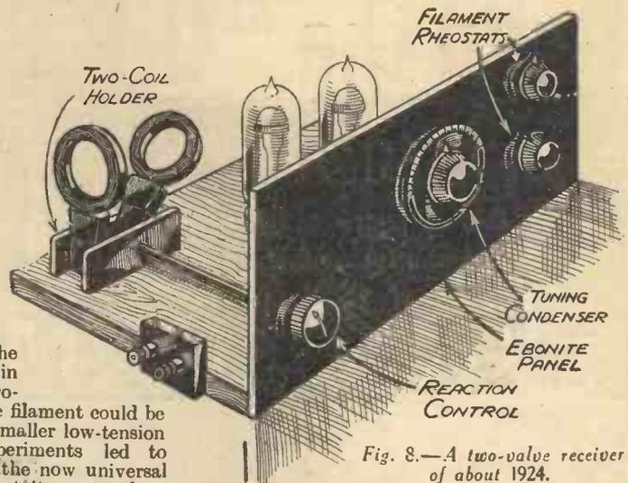
Fig. 8.—A two-valve receiver of about 1924.
