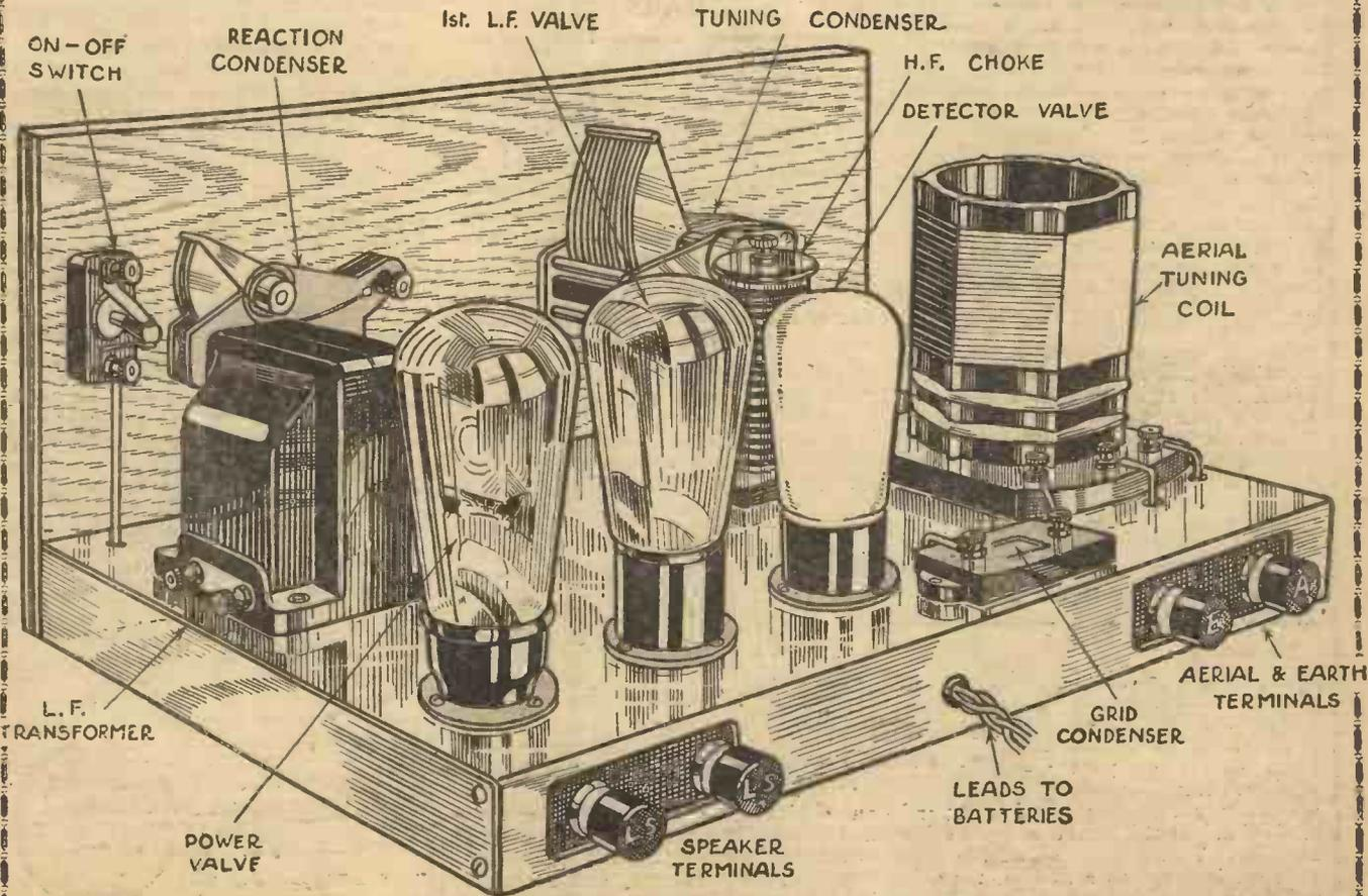
Fig. 7.—The typical three-valve set referred to in this article.
