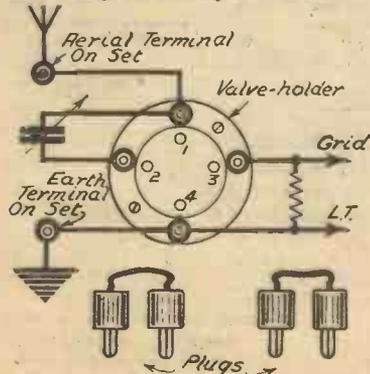
A handy plug and socket switching device.
