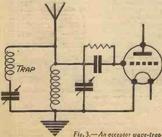
Fig. 3.—An acceptor wave-trap.
