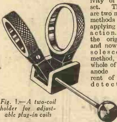
Fig. 1.—A two-coil holder for adjustable plug-in coils
