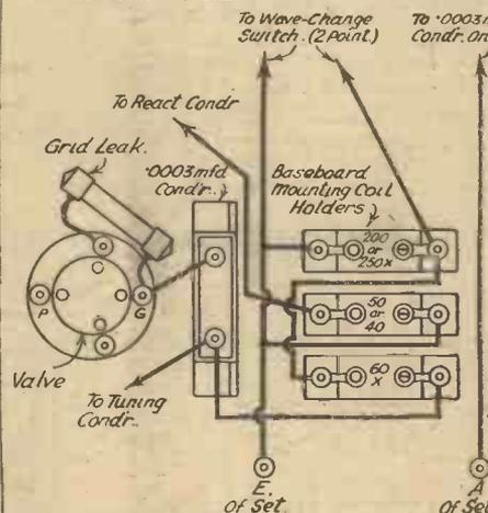
A method of wave-changing with plug-in coils.
