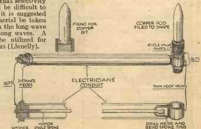
A small soldering iron made from odds and ends.
