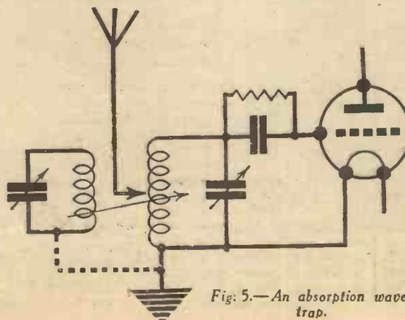
Fig. 5.—An absorption wave-trap.
