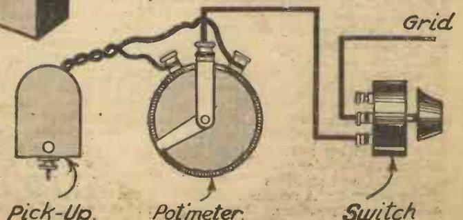
Fig. 3.—Controlling the output from the pick-up.
