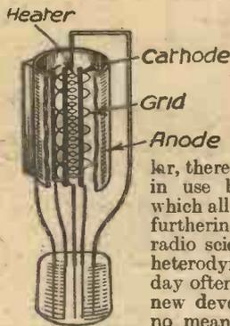
Fig. 13.—Showing the construction of an indirectly-heated valve.
