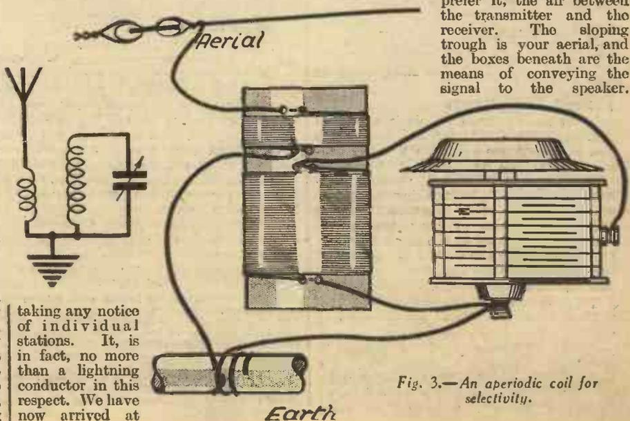
Fig. 3.—An aperiodic coil for selectivity.
