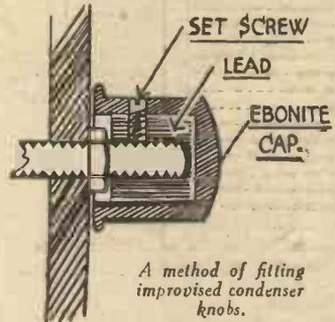
A method of fitting improvised condenser knobs.
