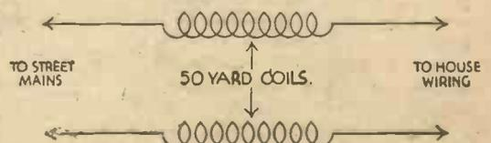
Anti-interference choke coils inserted in the supply mains
