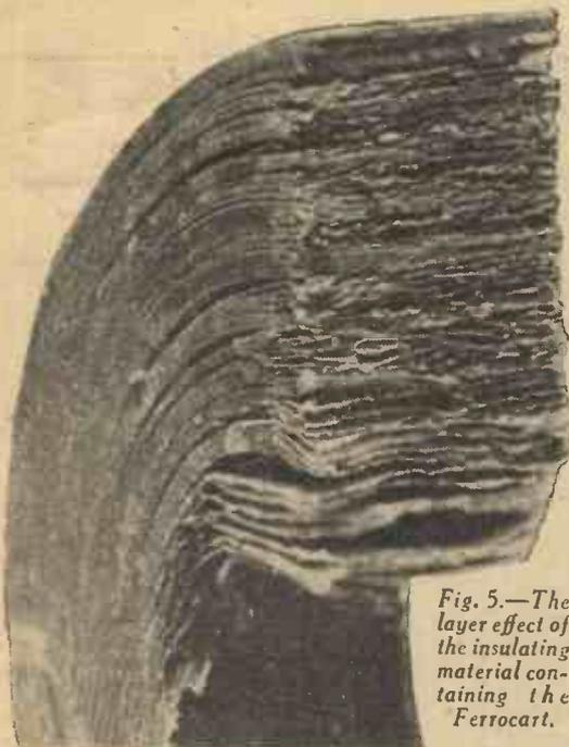
Fig. 5.—The layer effect of the insulating material containing the Ferrocort.
