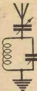
this is to imagine the small coil to be the trough of our graduating machine, and the extra coil and condenser as the particular box in which we are interested. All the balls (signals) will pass along the trough, and the adjustment of the tuning condenser will correspond with the alteration in the size of the hole.
