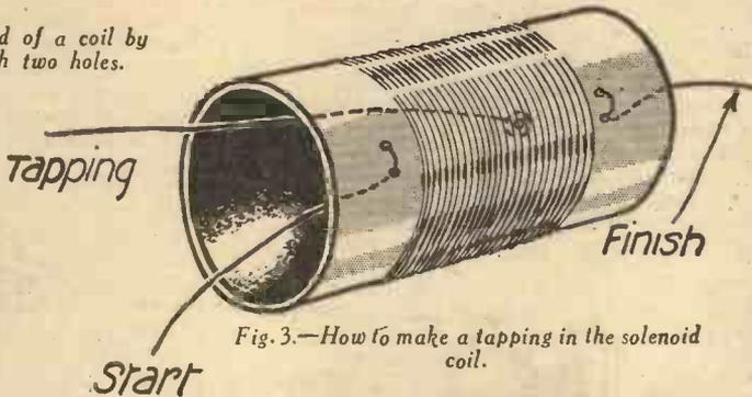
Fig. 3.—How to make a tapping in the solenoid coil.
