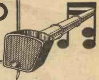
As you probably know, before any signal can be broadcast from a transmitter, it is necessary to convert the sound-waves emanating from the speaker or artiste into an oscillatory electrical current. The oscillations of which will be a faithful copy of the original differences in frequency and intensity of the original sound-waves. For this purpose, a microphone is used,
