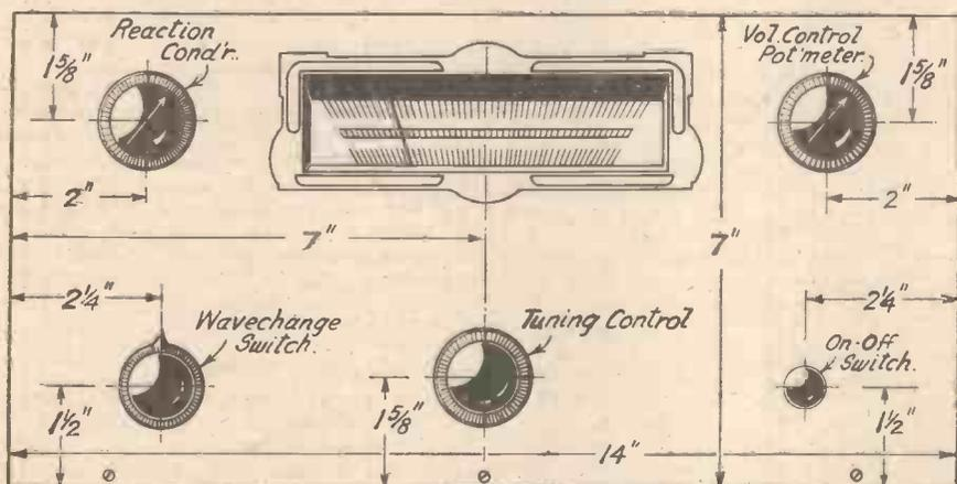
Fig. 2.—Front of panel layout.
