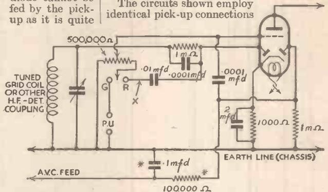
Fig. 2.—The double-diode-triode, arranged for A.V.C. with delay in a "straight" receiver, and fitted for reproducing gramophone records. A filter may be required at "x" in sets inclined to instability. Components marked\* are liable to modification.
