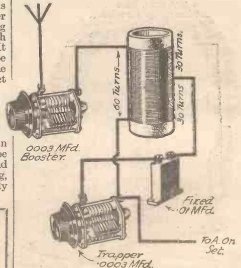
An efficient type of wavetrap.
