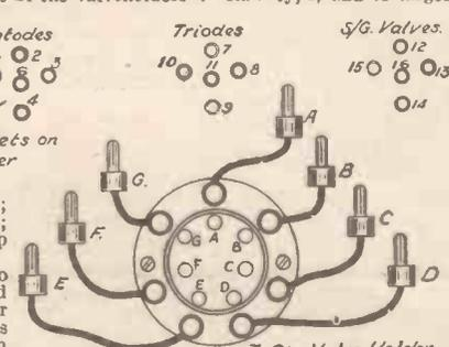
The connection for an additional valve-holder for testing Multi-pin valves on the Six-Sixty and similar test sets.
