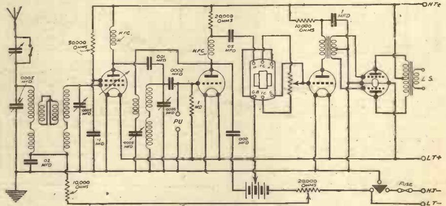
Fig. 3.—Circuit diagram of the Beta Universal Four.
