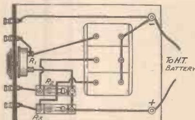
Wiring diagram for a useful filter pack.
