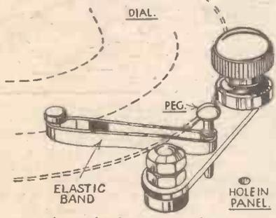
stretching the rubber band and placing the peg in the hole. This prevents wear on the small spindle when the dial is revolved the greater distance, and the small spindle is quickly put in action again by releasing the peg. The operation includes drilling three small holes in the panel, one being beneath the dial, which is removed for the purpose.—W. H. GRAYLING (Cambridge).
