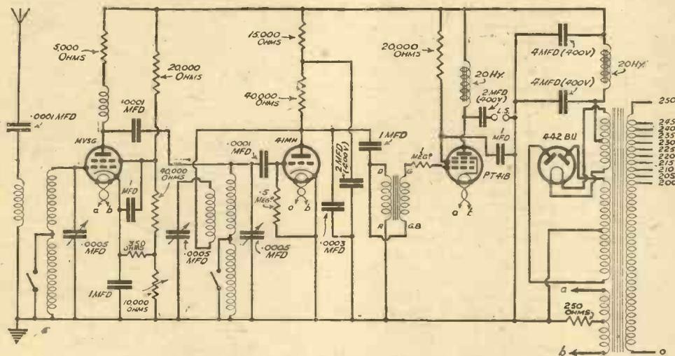
Fig. 1.—A good 3-valve mains circuit, the Mains Express Three.
