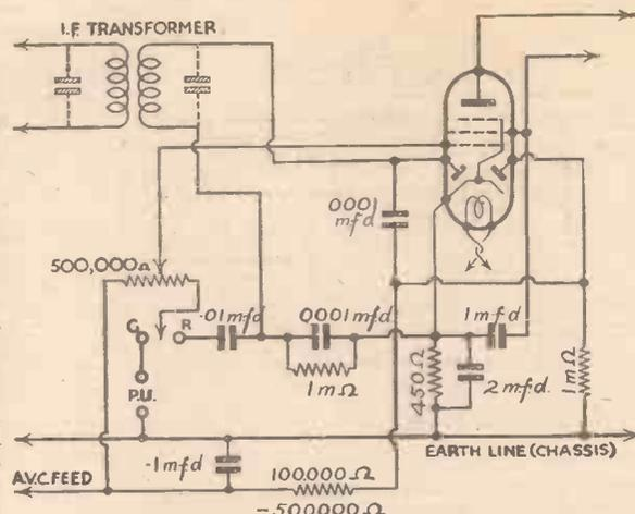
is arranged for use in a straight receiver. When using a pick-up with this type of valve it is often necessary to shield the leads as they are apt to cause mains hum in the speaker unless they are kept very short. This is due to the relatively high sensitivity of the pentode portion.
