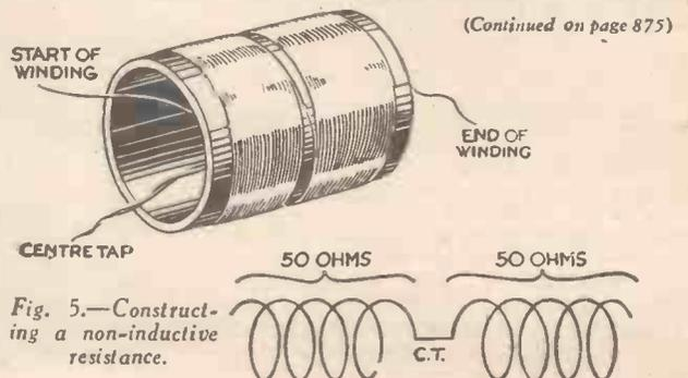
Fig. 5.—Constructing a non-inductive resistance.
