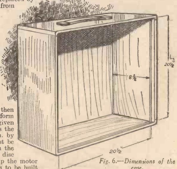
Fig. 6.—Dimensions of the case.
