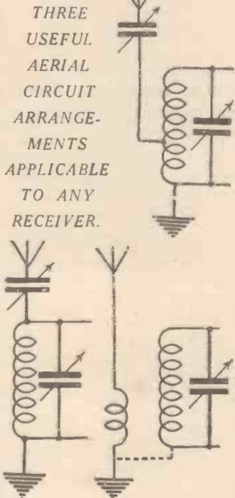
Fig. 3.—Various methods of obtaining selectivity in a single tuned circuit. They all suffer from certain drawbacks. (See text.)
