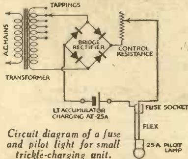
Circuit diagram of a fuse and pilot light for small trickle-charging unit.
