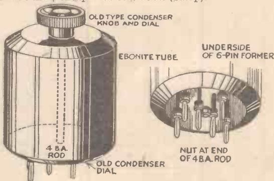
Method of making six-pin coil former from scrap material.
