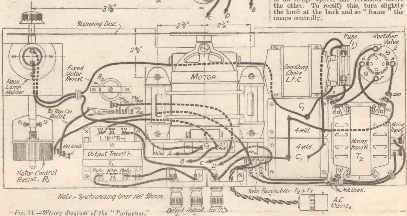
Fig. 11.—Wiring diagram of the "Portovisor."
