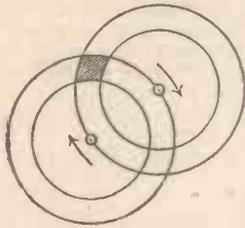
Fig. 7.—The combined action of two prismatic discs to give the required light beam motion.
