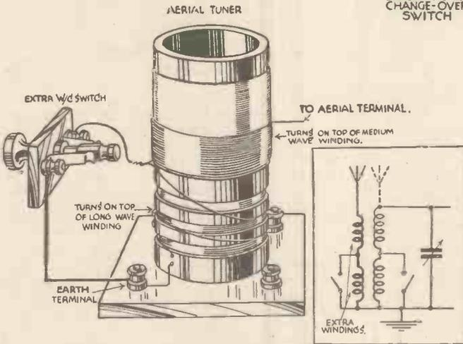
Fig. 21.—Improving selectivity by adding an aperiodic aerial winding.
