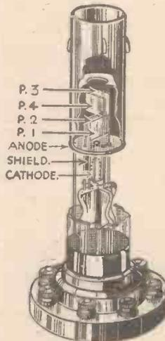
Fig. 18.—Showing the normal electrode system of a cathode ray tube.
