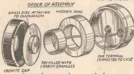
A simple microphone made from a telephone earpiece.
