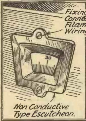
Fixing Screws Connected To Filament Wiring Of Set.
