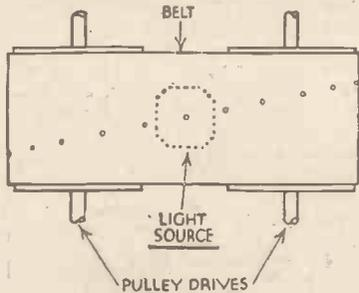
Fig. 12.—A simple scanning belt.
