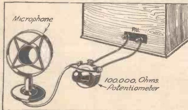
Fig. 2.—A simple method of connecting a volume control between the microphone and set.
