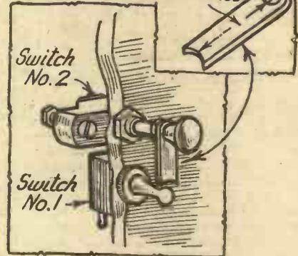
An alternative to a thermal delay.
