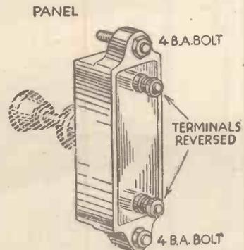
Fig. 12.—It is sometimes more convenient to mount the pre-set condenser on the panel and this can be done as shown, by reversing the terminals.
