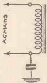
Fig. 3.—A condenser between earth and one side of the primary will prove very useful as a hum remover.
