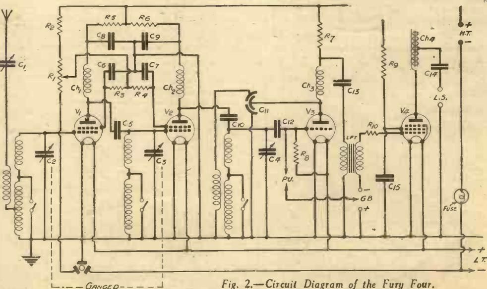
Fig. 2.—Circuit Diagram of the Fury Four.
