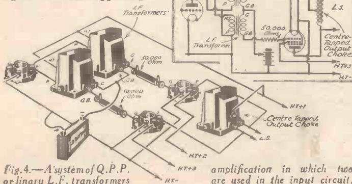
Fig. 4.—A system of Q.P.P. ordinary L.F. transformers amplification in which two are used in the input circuit.
