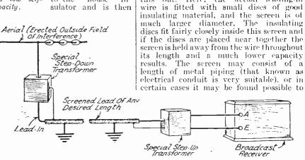
Fig. 2.—Diagram explaining the method of erecting an anti-interference acrial system employing special transformers.
