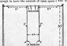
Fig. 4.- A divided aerial: K1 and K2 are equal in length half the wavelength.  $K3 = 4\frac{1}{2}$  inches.
