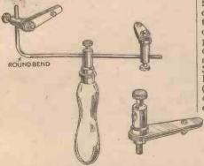
Easily-made soldering tweezers.
