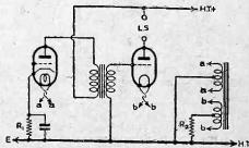
Fig. 9.—When a mains transformer is used which has separate heater windings for the directly-heated and indirectly-heated valves, grid decoupling is generally quite unnecessary, and a circuit such as that shown above can be employed.
