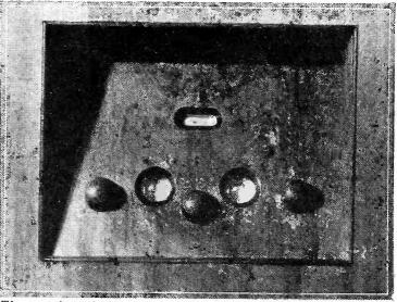
The control panel of one of the new Ferranti receivers, which is fitted with magnifying lenses over the tuning scale. The horizontal opening at the top of the panel is the visual electric tuning indicator.
