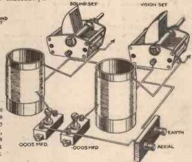
Fig. 2.—Twoffixed (or pre-set) condensers, used to feed the sound and the vision receiver where ordinary tapped coils are employed.
