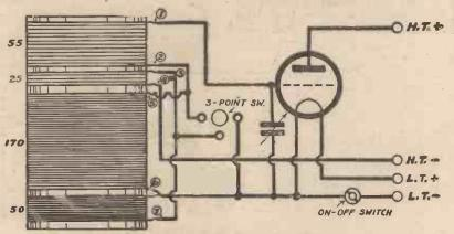
Theoretical diagram of the Heterodyne Wavemeter.
