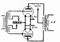
Fig. 8.—A battery operated push-pull stage.
