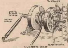
An automatic winding device for L.S. leads.
