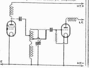
what stereotyped .0002 mfd. and 2 megohms can rarely be improved upon. At the same time it is frequently worth while to experiment with different values, bearing in mind that a reduction in capacity, or an increase in grid-leak resistance, tends to improve selectivity, whilst the opposite usually increases the power-handling capacity of the valve.
