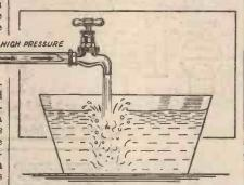
Fig. 2.—The same rate of flow produced by a small pipe but high pressure.
