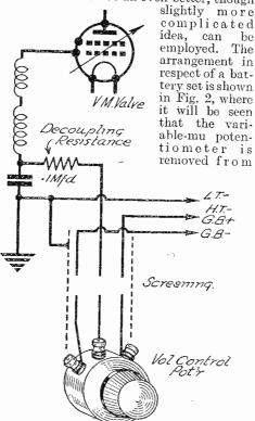
Fig. 2.—Remote volume control is easily arranged in the case of a set having a variable-mu amplifier. The connections shown above refer to a battery-operated set.
