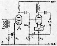
This circuit shows the methods of biassing and decoupling a directly-heated output valve in a mains set.
