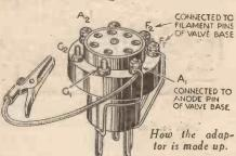
In using the adaptor plug it into the emission tester and place valve to be tested in holder. As only 9 volts are used for high tension, no emission will yet be registered as the anodes of the valve are clip is clipped on to Gl terminal, the emission of one half of the valve will be registered. To test the other half connect the crocodile clip to G2; this utilizes the grids as anodes and a satisfactory emission test can be made.—L. C. DRISCOLL (Plaistow, E.13).
