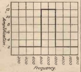
Fig. 2.—This diagram illustrates the ideal! which should be aimed at in designing the frequency response of a broadcast receiver.
