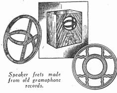
designs shown can easily be cut out with a fretsaw. A black fret will, of course, give a striking contrast to any cabinet, and a very pleasing effect is given by the groove markings on the record. In one of the most beautiful frets of this kind I have seen the grooves were filled up with various blending shades of sealing-wax to match a walnut cabinet.—W. CAPEWELL (West Norwood).
