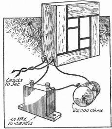
Fig. 4.—A simple and effective remote-control for varying the tone of reproduction. The .01 mfd condenser is not always necessary, but is generally desirable.
