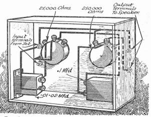
Fig. 5.—A neat unit which combines a tone control and volume control. The unit is connected between the receiver and speaker.
