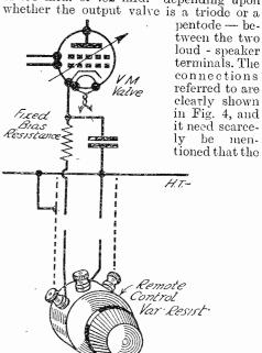
Fig. 3.—This skeleton circuit shows how remote volume control can simply be effected in the case of a mains set having a variable-mu amplifier.
