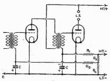
Fig. 4.—This shows grid-bias decoupling arrangements when two battery-operated L.F. valves are automatically biased.
