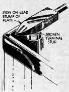
Method of removing broken terminals accumulators
