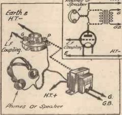
Fig. 1.—An L.F. stage can easily be cut out by connecting a pair of phones or a loud-speaker in the anode circuit of the preceding valve in place of the normal coupling component (L.F. transformer, etc.)
