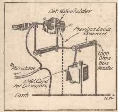
Fig. 2.—Showing the slight alterations to be made to the wiring when connecting a pick-up to the detector valve of an all-mains receiver.
