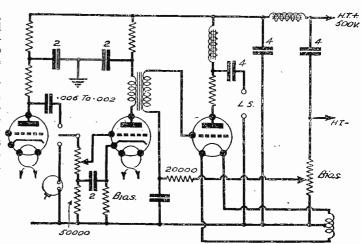
and Fig. 9.—A suggested arrangement for the L.F. side of a quality receiver.
