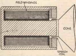
Flg. 3.—Section through an energized moving-coil speaker showing the most important parts.
