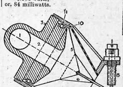
Fig. 2.—1 is an acoustic duct, leading to 2, Pig. 2.—1 is an acoustic duct, leading to 2, Duct in tone arm forming first part of acoustic tube. 3, Main Casting. 4, Conical guard (perforated metal) held by 4a, Screwed ring. 5, Conical diaphragm or "piston." 6, Conical piston extension. 7, Piston rod, connecting to 8, Needle holder, and 9, Needle. 10, Piston skirt, supported by 11, India-rubber rolling ring or obturator. ring or obturator.
