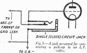
when connecting to one of the L.F. stages the circuit is somewhat simplified since grid bias is already provided. All that is required then to enable a pick-up to be used is a single closed circuit jack and a plug.
