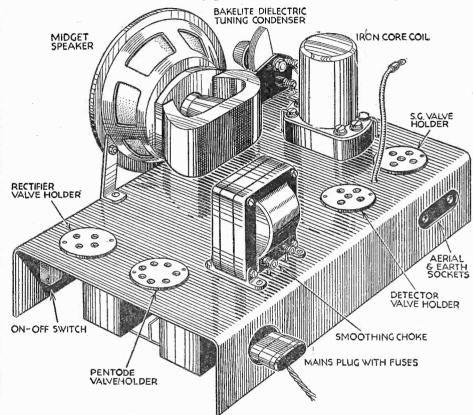
Fig. 1.—A suggested lay-out for a "midget" receiver using the circuit given in Fig. 2.
