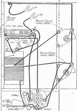
Fig. 2.—Wiring diagram for this neat little receiver.
