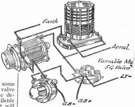
Gain control by variable-mu S.G. valve in battery set.
