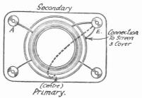
Fig. 4.—Wiring of transformer
