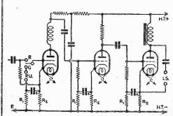
Fig. 6.--Skeleton circuit of the detector and L.F. stages of a mains receiver where two every grid is effectively decoupled.
