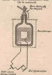
Fig. 9.—Another commercial form of magnetizer, the advantages of which are described.
