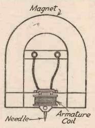
Fig. 1.—The principal parts of a pick-up are shown in this diagram.
