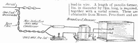
Fig. 5.—Connections for anti-interference device.
