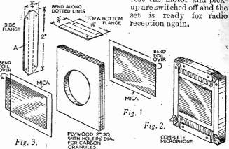
Constructional details for an easily made microphone.
