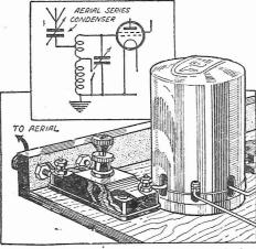
Fig. 1.—The series aerial condenser which is a valuable selectivity device.
