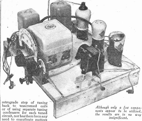
by fitting a multiplicity of unnecessary control knobs. On the contrary, the "Leader" employs a really modern screened two-gang condenser (with separate trimmers, so that the maximum degree of sensitivity can be secured under all conditions of use) in conjunction with a pair of eminently up-to-date screened coils specifically designed to cover the new range of wavelengths as prescribed under the Lucerne Plan. Controls have been
