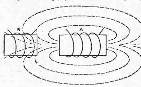
Fig. 2.—Magnetic field leakage between A and B.
