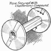
A method of fixing bobbin checks.
