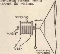
Fig. 2.—This sketch shows the working parts of a moving-iron speaker.
