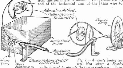
Fig. 7.—A remote tuning control idea where a Bowden cable is used to operate the tuning condenser. Sometimes it is desirable to fit small pulleys on the condenser and drive spindles to obtain a better movement.
