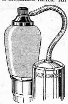
Fig. 6 .--Using a screened wire for connection to the anode cap of an S.G.
