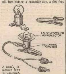
of thin flex, and two plugs. The base of the holder is unscrewed and the crocodile clip fixed in its place. The flex is attached, with plugs, and a flashlamp bulb inserted. The plugs may be slipped into the grid-bias battery and the lamp clipped on to the wiring or anywhere near to the job in hand. When changing batteries it can be placed near, and will greatly facilitate matters.
