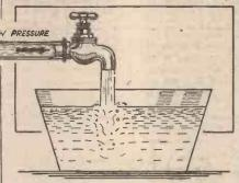
Fig. 1.—The water analogy. A certain rate of flow is produced by a large pipe and low pressure.
