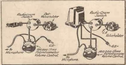
Fig. 3.—On the lest the method of fitting both a change-over switch and volume control to the detector value is shown. The method of making the same additions to an L.F. valve is shown on the right.
