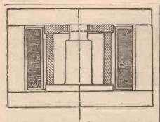
Fig. 5.—Another method of magnetizing, in which the complete magnet assembly is placed within a field winding with iron yoke.
