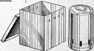
Fig. 4.—The screening box and " can."
