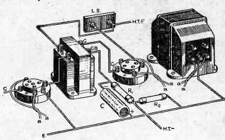
Fig. 8.—A good method of biassing a directly-heated valve which is used along with other indirectly-heated valves and whose cathode (or filament) is heated from the same source.
