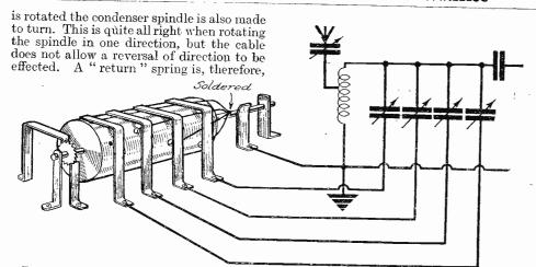
Fig. 8.—A remote tuning scheme which makes use of a relay similar to that shown in Fig. 6. This works in conjunction with a number of pre-set condensers.
