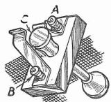
Method of adapting an on/off switch.
