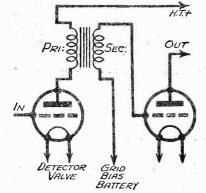
Fig. 10.—The commonest connecting an intervalve transformer.
