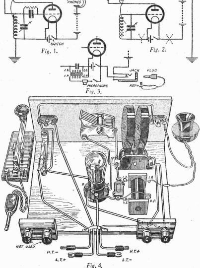
Circuit diagram and layout for a simple one-valve transmitter.
