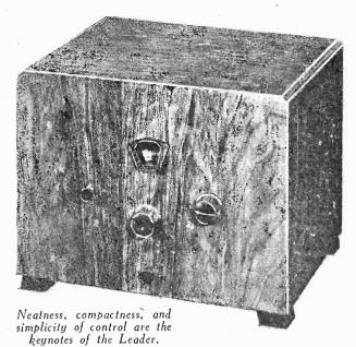
dated April 8th last may be added to The Leader, under which conditions the present output valve becomes the Class B driver. No other alteration of any sort will be required. The input terminals on the unit are connected to the L.S. terminals on The Leader, which means that the primary of the driver transformer is connected direct in the anode circuit of the P.215 valve.
