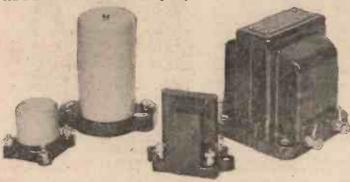
Fig. 3.—Here are two standard components—an H.F. choke and an L.F. the anode circuit of transformer compared with similar midgets. The small choke is a Wearite a valve it is nearly and the miniature transformer a Bulgin "Senator." always parallel-fed
