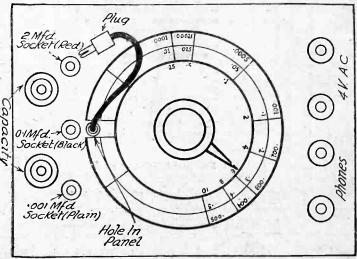
Fig. 3.—Top of panel showing scales. Note the extra long pointer on the knob.
