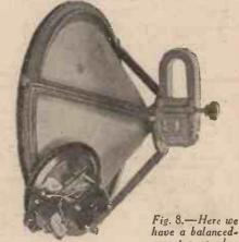
armature speaker chassis of normal type compared with a midget moving-coil unit. The latter is a "Sonochorde."
