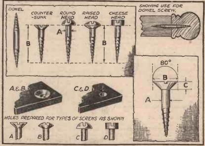
Wood screws and their proportions. This diagram should be used in conjunction with the table at the top of the centre column.
