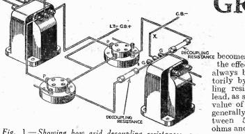
Fig. 1.—Showing how grid decoupling resistances are connected in the case of a battery-operated push-pull amplifier.
