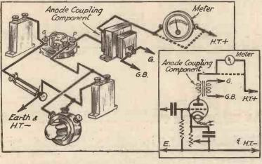
Fig. 3.—The best way to determine the correct G.B. voltage for an L.F. valve is to insert a milliammeter in the anode circuit and vary the bias until the correct anode-current reading is obtained.
