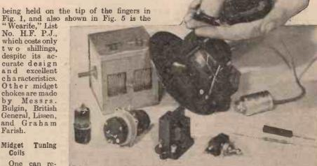
Fig. 1.—An interesting photograph which shows a number of new midget components: their size can be judged by comparison with the hand
