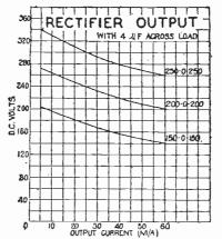
Fig. 2.—Regulation, or output curves for a typical Class A rectifying valve.
