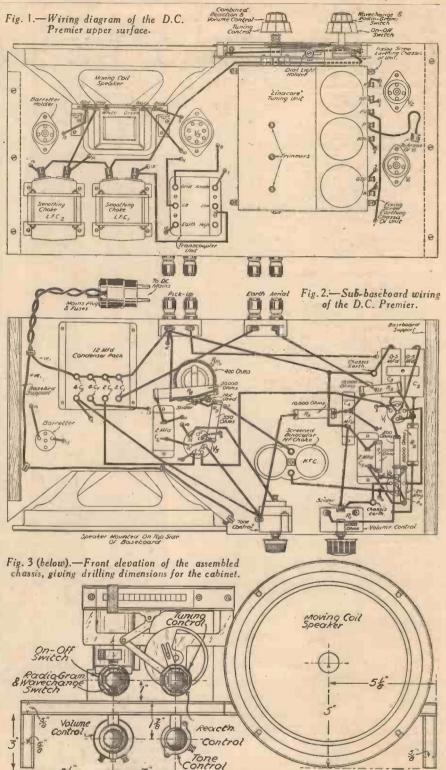
the template once again for this purpose. Fix the escutcheon plate. For convenience in wiring the speaker was held to the baseboard by two small brackets, but I mentioned that the four connecting leads should be left longer than actually required. This was to allow the speaker flange to be screwed to the cabinet front, which acts as the baffle.
