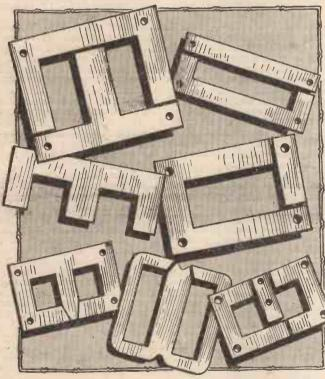
The above drawing shows a variety of types of transformer stampings. volts up to 1,000
