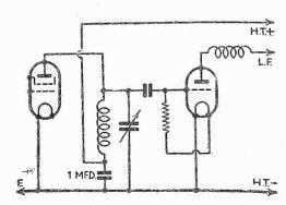
Fig. 5.—Tuned-anode coupling in its simplest form.
