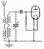
Fig. 4. — Aninductively-coupled aerial input arrangement. This usually works well on medium waves, but is not quite so good on the long-wave band.
