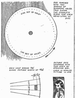
Method of marking out and punching a television scanning disc.
