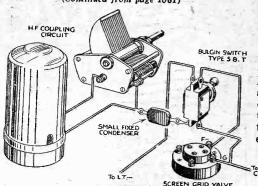
A simple band-pass filter arrangement.
