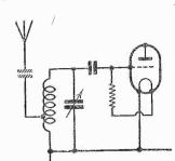
Fig. 1.—The usual form of aerial-grid circuit employed simple in receivers.
