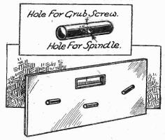
Fig. 4: "Straight knobs" made from ebonite rod.
