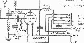
Fig. 3.—Theoretical circuit of the Pocket Portable.
