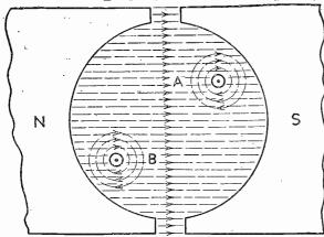
Fig. 2.—When a current is made to pass round the single-turn loop a magnetic field is created round each limb of the loop.
