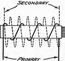
Fig. 6.—A simple transformer made of two coils of wire.
