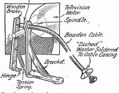
Simple speed regulator for a television motor.
