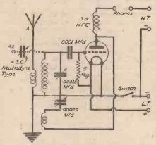
Fig. 1.—A one-valve circuit, suitable for all wave-lengths.
