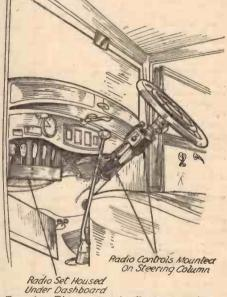
Fig. 1.—This pictorial illustration shows the arrangement of a receiver and its controls in a typical car. Note the mounting of the
