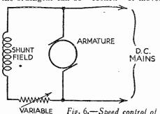
VARIABLE Fig. 6.—Speed control of RESISTANCE shunt motors is effected by using a variable resistance in series with the field winding.
