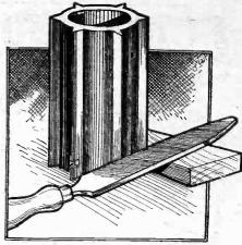
A method of slotting ribbed coil formers.
