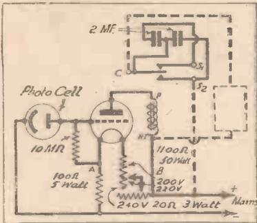
Fig. 9.—The simple connections for a mains-operated photo-cell amplifier. The external circuit is represented by broken lines. Notice that two condensers are connected across the relay contacts to prevent arcing.
