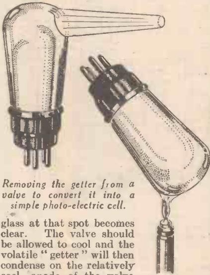
Removing the getter from a valve to convert it into a simple photo-electric cell.
