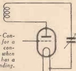
Fig. 3.—Connections for a reaction condenser when the coil has a split winding.
