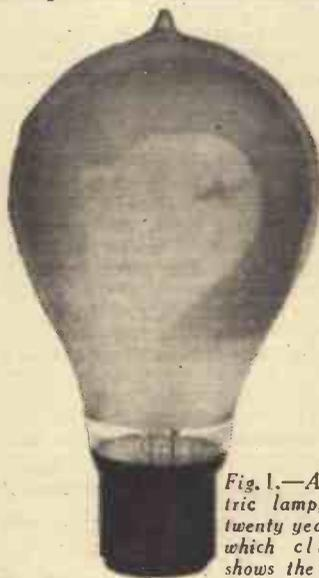
Fig. 1.—An electric lamp, over twenty years old, which clearly shows the "electron shadow" on the bulb.
