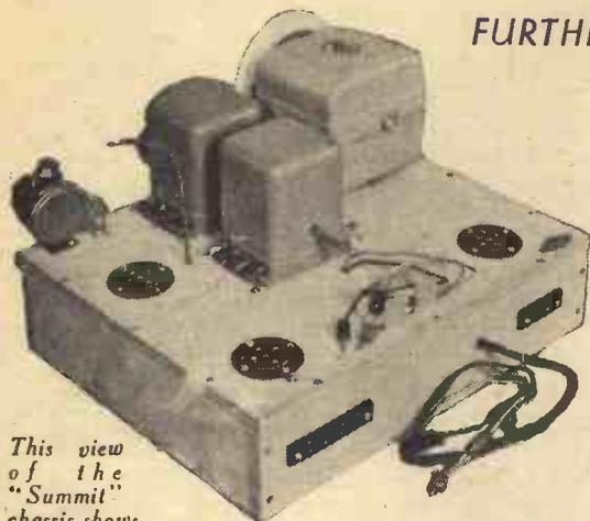
This view of the "Summit" chassis shows the neat layout and absence of wiring on top of the chassis.
