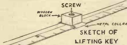
Fig. 2.—The lifting key.
