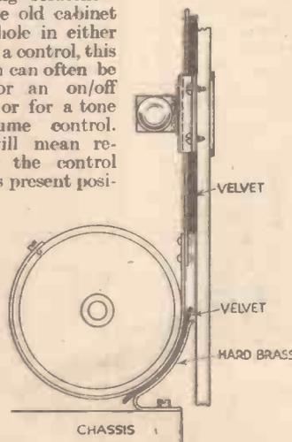
Fig. 2.—A side view of the wavelength scale.
