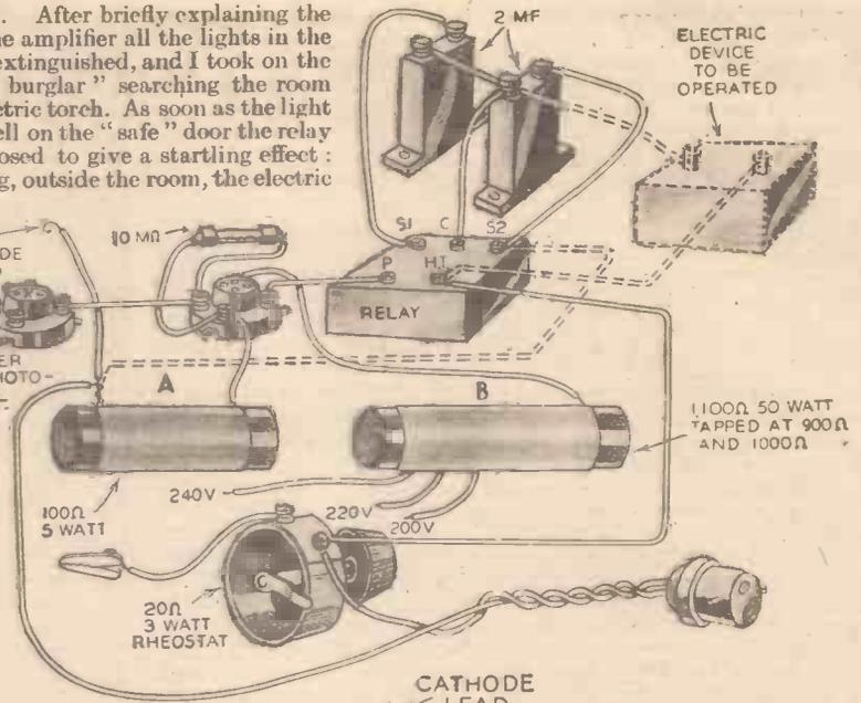
Fig. 7.—Operating an electric light by means of a photo-cell amplifier.
