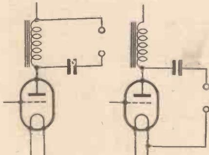
Figs. 1 and 2.—Showing the correct and incorrect methods of connecting a speaker in a choke filter circuit.
