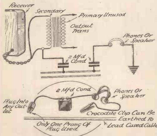
A novel method of fixing an extension speaker.
