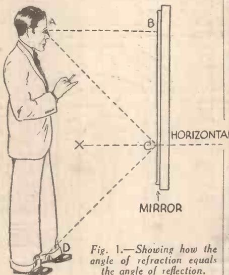
Fig. 1.—Showing how the angle of refraction equals the angle of reflection.
