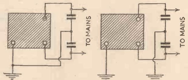
Figs. 4 and 5.—Circuit diagrams showing the connections for an anti-interference filter.
