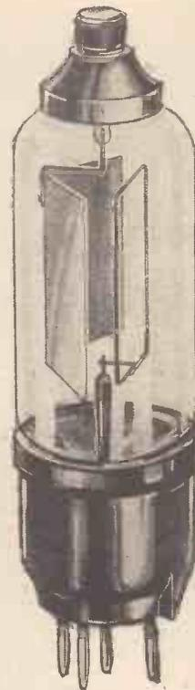
Fig. 1.—The above sketch shows the electrodes in a typical photo-electric cell.
