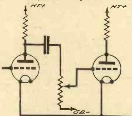
Fig. 1.—The correct position for a volume control in a television amplifier.
