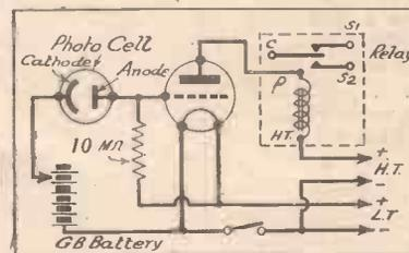
Fig. 2.—Practical and theoretical circuit of a simple and effective type of photo-electric cell amplifier for battery operation.
