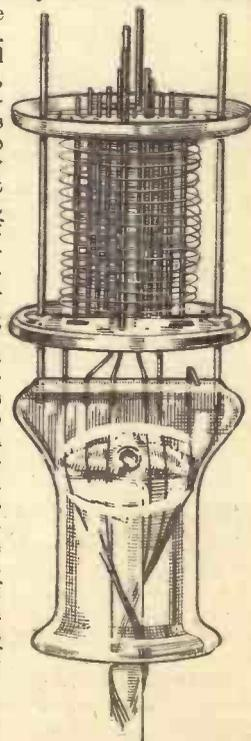
Fig. 3.—The electrode assembly of an octode.
