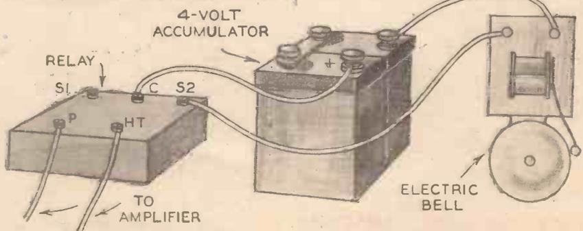
Fig. 8.—An electric bell can be switched into circuit by using the connections shown above.
