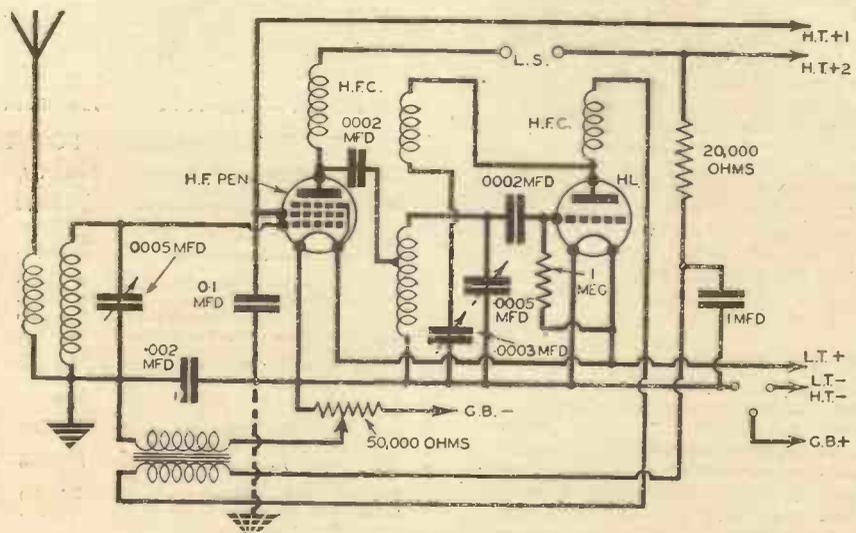
Fig. 2.—The above circuit is a suggestion for a reflex circuit employing modern components. Broken lines show an alternative earth connection, which may be tried.
