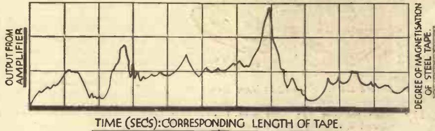
Fig. 3.—A graphical representation of the degree of magnetization of a length of the Blattnerphone tape by comparison with the output from the recording amplifier. The wavy line represents a sound wave.
