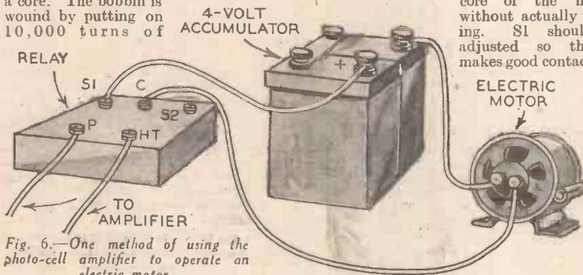
Fig. 6.—One method of using the photo-cell amplifier to operate an electric motor.
