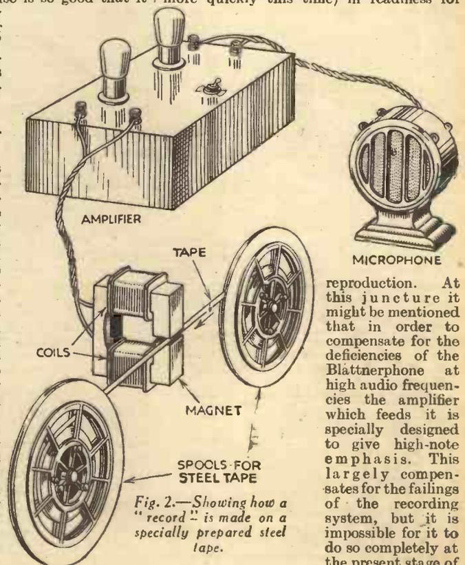
Fig. 2.—Showing how a "record" is made on a specially prepared steel tape.
