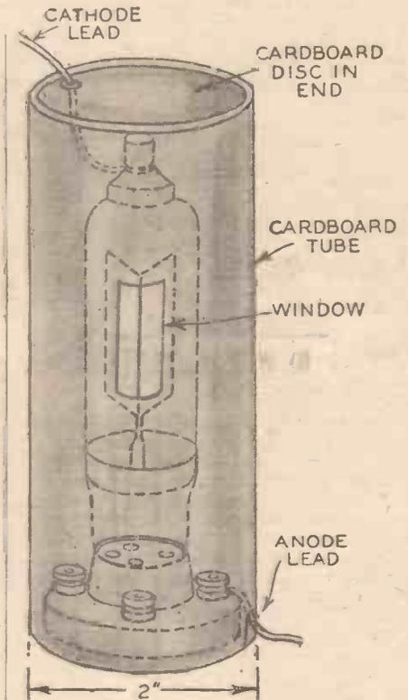
Fig. 5.—A cover for the photo-electric cell.
