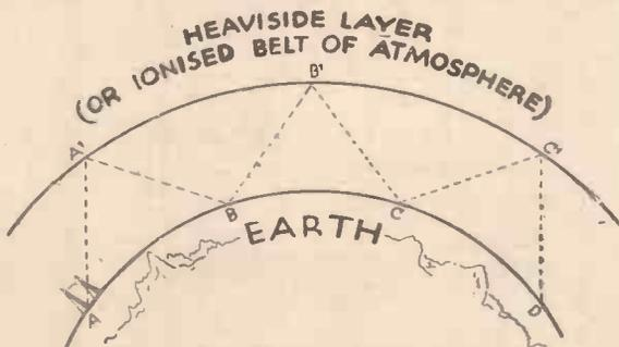
Fig. 2.—How a short-wave signal is deflected back to earth.
