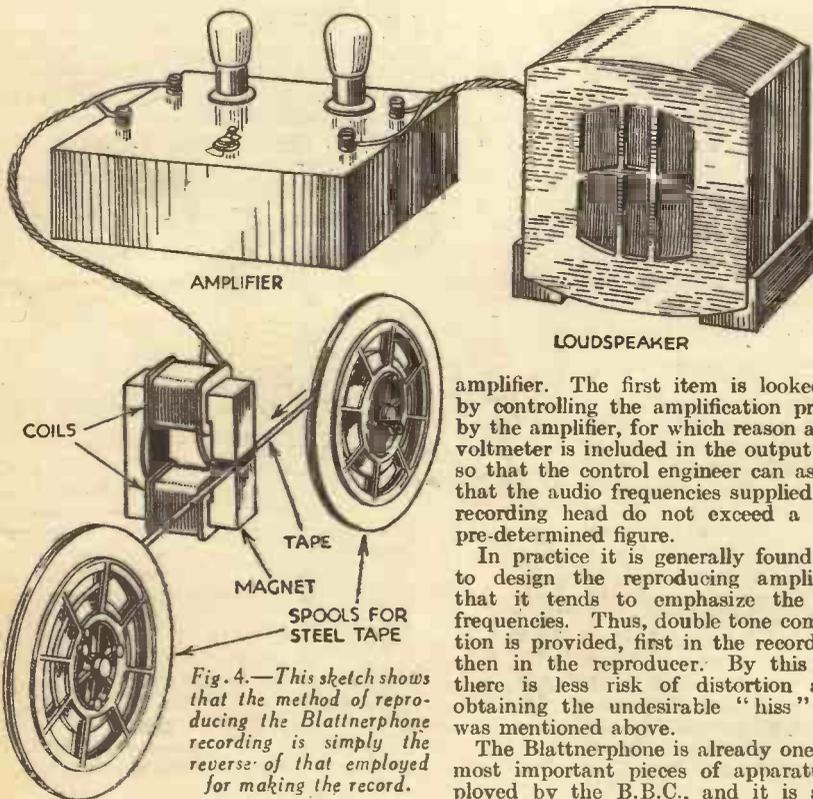
Fig. 4.—This sketch shows that the method of reproducing the Blattnerphone recording is simply the reverse of that employed for making the record.
