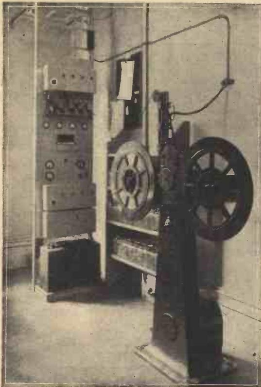
Fig. 1.—This photograph shows the Blattnerphone installed in the B.B.C.'s premises at Savoy Hill in 1931. The amplifier and control panel can be seen in the background.
