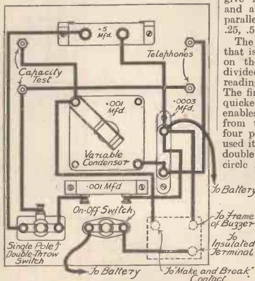
Fig. 2.—Wiring diagram of the simple capacity tester.
