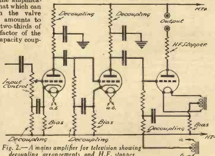
Fig. 2.—A main amplifier for television showing decoupling arrangements and H.F. stopper.
