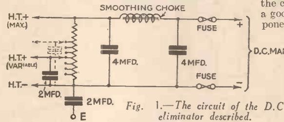
Fig. 1.—The circuit of the D.C. eliminator described.
