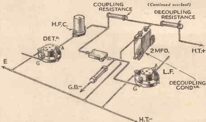
Fig. 1.—Showing the R.C.C. coupling between detector and L.F. valves. The various parts are referred to in the text.
