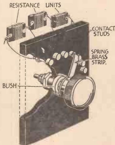
Fig. 6.—Showing one method of making a reliable, though rather cumbersome, variable resistance.
