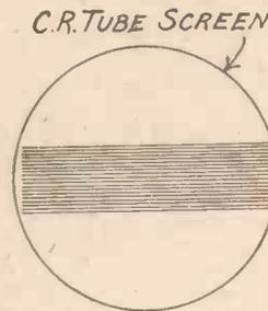
Fig. 2.—Using too large a voltage sweep on the vertical deflector plates, and too little on the horizontal deflector plates.
