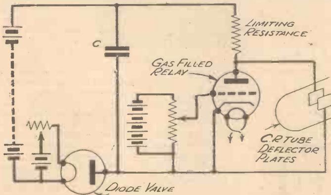
Fig. 1.—The simple single-time-base connections using a gas-filled relay.
