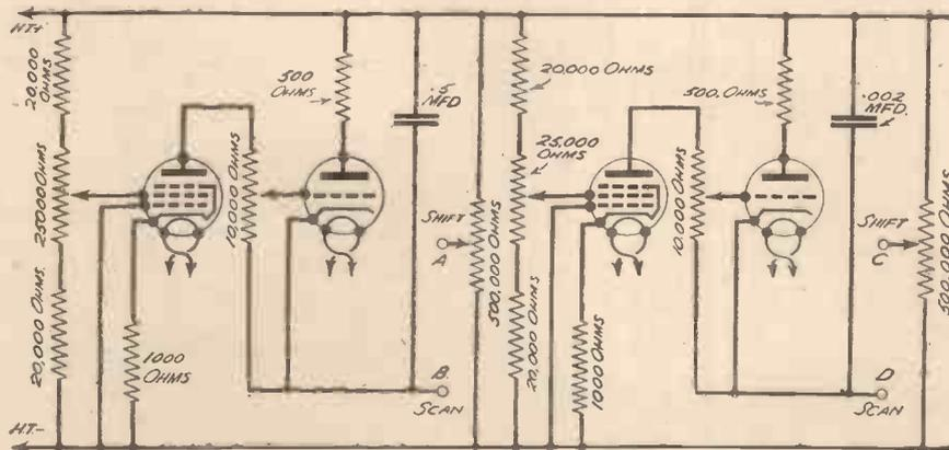
Fig. 4.—A double time-base circuit using gas-filled relays and screened-pentode valve.
