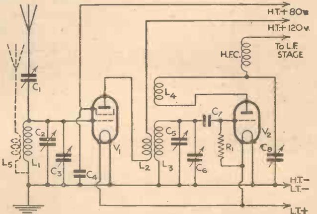
Fig. 2.—This circuit shows a tuned H.F. stage with transformer coupling to the detector valve, and throttle control of reaction.
