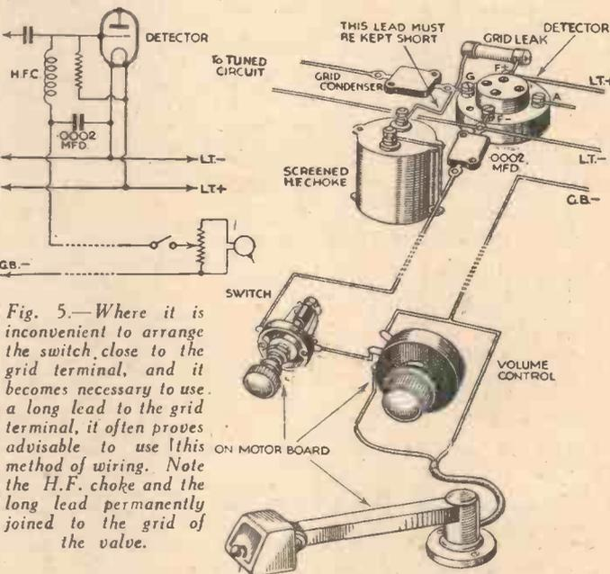
Fig. 5.—Where it is inconvenient to arrange the switch close to the grid terminal, and it becomes necessary to use a long lead to the grid terminal, it often proves advisable to use this method of wiring. Note the H.F. choke and the long lead permanently joined to the grid of the valve.
