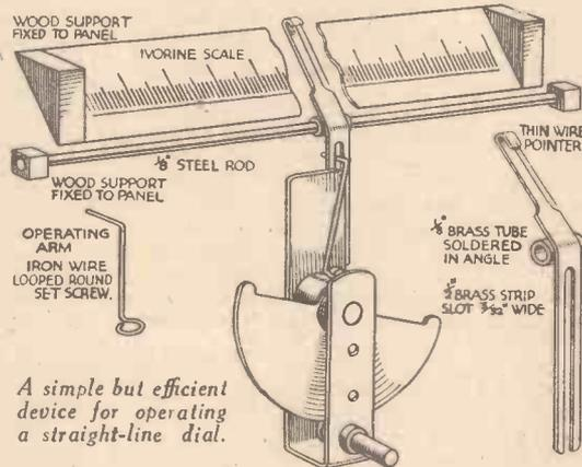
A simple but efficient device for operating a straight-line dial.
