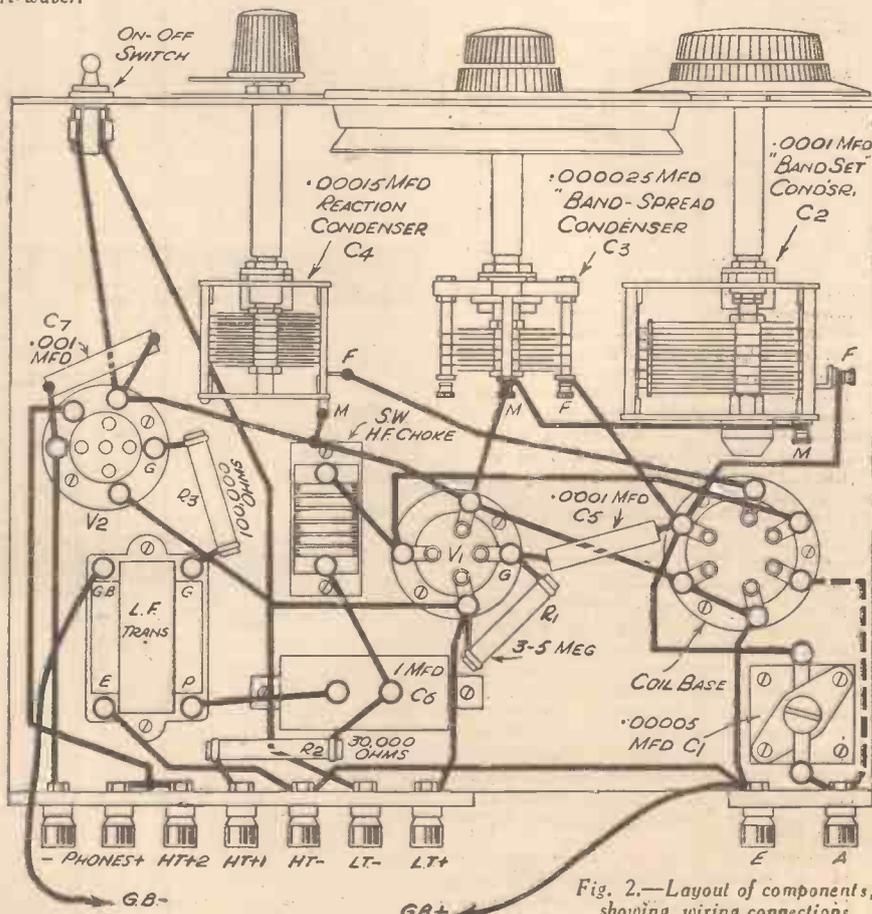
Fig. 2.—Layout of components, showing wiring connections.
