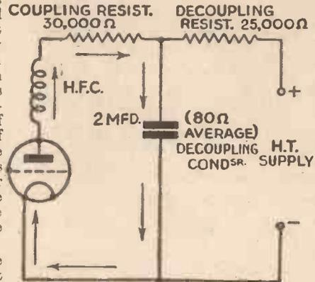
Fig. 3.—This circuit shows how the use of decoupling components prevents the audio-frequency currents from passing through the H.T. battery or unit.
