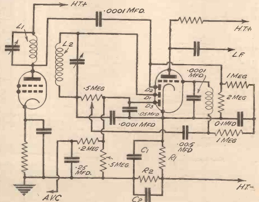
Fig. 1.—This circuit shows the connections for the valve when used for second detector, A.V.C. noise suppressor, and first L.F. amplifier.
