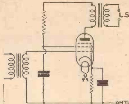
Fig. 2.—Using a mains-operated pentode valve for Class "A" output.
