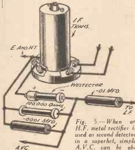
Fig. 5.—When an H.F. metal rectifier is used as second detector in a superhet, simple A.V.C. can be obtained by taking a
