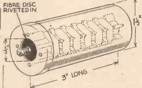
Fig. 4.—Showing a simple method of screening the choke shown in Fig. 3 by means of a cylindrical tin canister.
