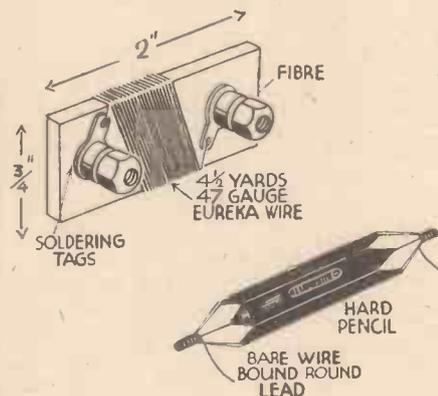
Fig. 3.—Two different methods of making the fixed bias resistance are illustrated above.
