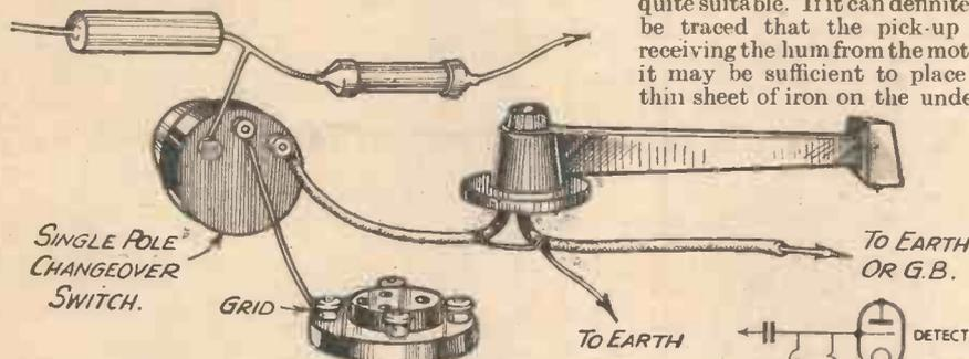
Fig. 4.—The correct way of arranging the pick-up and switch. Note that, as a general rule, screening should be confined to the pick-up lead only, the grid connection, being unshielded, as screening here will be part of the radio circuit and may thus cause other troubles.
