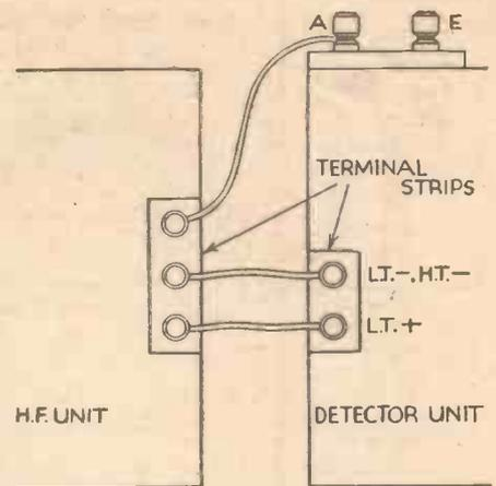
Fig. 7.—When the separate receiver stages are made as units it will be found convenient to fit terminal strips for inter-unit connection as shown here.
