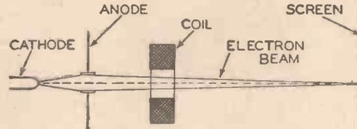
Fig. 4.—Method of bringing the electron beam under the influence of a magnetic field.
