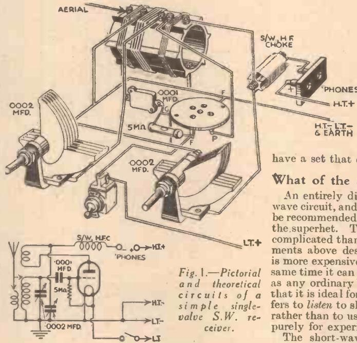
Fig. 1.—Pictorial and theoretical circuits of a simple single-valve S.W. receiver.
