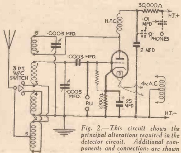
Fig. 2.—This circuit shows the principal alterations required in the detector circuit. Additional components and connections are shown in heavy lines.
