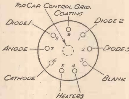
Fig. 2.—Showing the connections for the pins of the triple-diode triode described.
