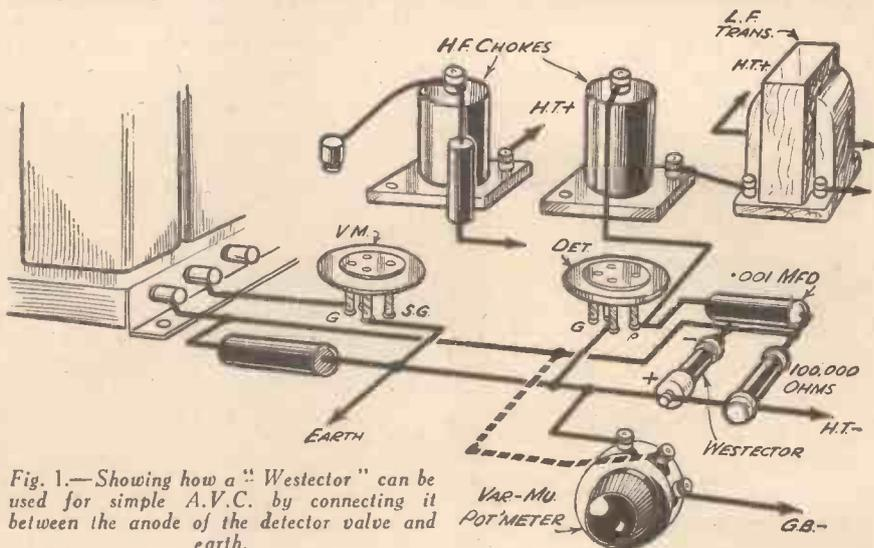
Fig. 1.—Showing how a "Westector" can be used for simple A.V.C. by connecting it between the anode of the detector valve and earth.
