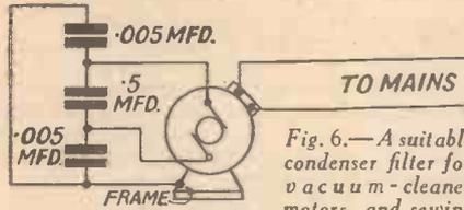
Fig. 6.—A suitable condenser filter for vacuum-cleaner motors, and sewing machines. The mains plug to the motor is reversible.
