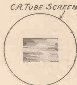
Fig. 1.—A picture area made too small by insufficient sweep voltages on each pair of deflector plates.
