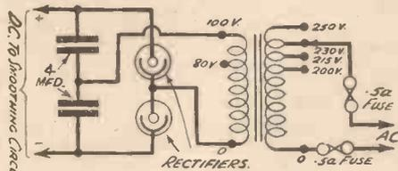
Fig. 1.—The circuit for the transformer and rectifier unit for converting the D.C. eliminator for A.C. operation.
