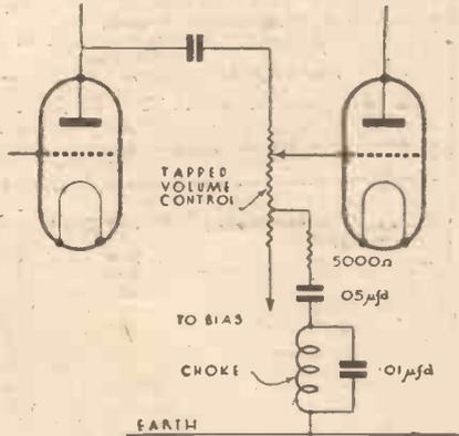
Fig. 1.—The theoretical circuit.
