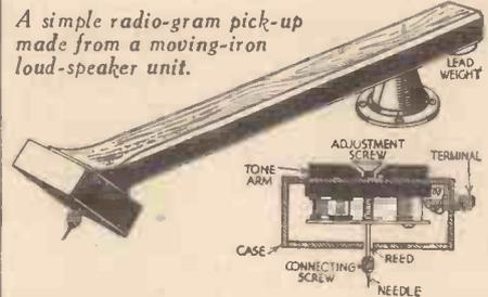
A simple radio-gram pick-up made from a moving-iron loud-speaker unit.
