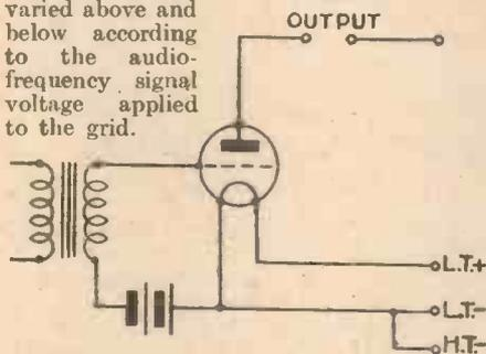
Fig. 1.—A battery-operated Class "A" output stage (triode).
