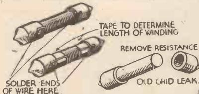
A simple method of making short-wave chokes.
