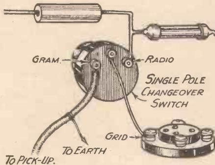
Fig. 1.—A change-over switch to control the pick-up. Note where the screening is employed.
