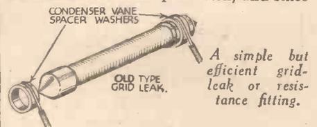
then many have been used as shown in the accompanying sketch. A piece of wire is soldered to the washer before it is pushed over the metal end of the resistance or grid-leak.—D. M. STEWART (Stranraer).
