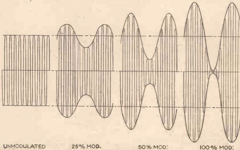
Fig. 2.—Different degrees of modulation.
