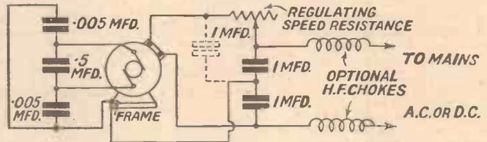
Fig. 7.—Where a sewing-machine motor or fan is fitted with a speed regulator, the additional suppressing devices shown are usually necessary. The metal frames of both motor and regulator should be connected together (not shown), if not already contacted.
