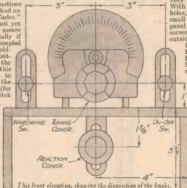
This front elevation, showing the disposition of the knobs, will be of assistance when drilling the cabinet.
