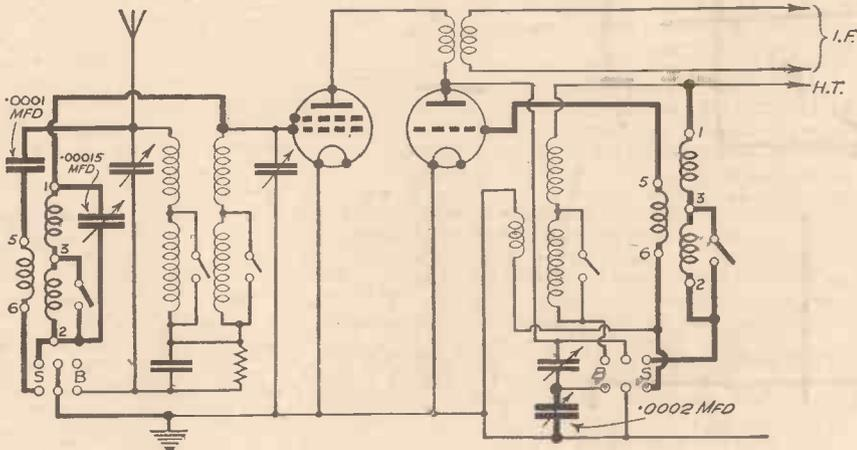
Fig. 1.—A skeleton circuit, showing how short-wave coils and waveband switches can be added to a superhet with separate first-detector and oscillator valves to permit of all-wave tuning. The short-wave circuits are shown by heavier lines for clarity.
