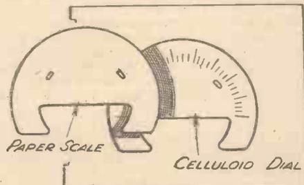
Fig. 2.—After the paper scale is cut to shape it is fixed to the celluloid dial.
