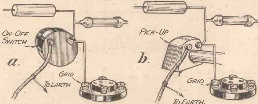
Fig. 2.—Two alternative methods of connection, (a) with a simple on-off shorting switch, and (b) without any switch at all. With this latter connection it is necessary to detune the radio circuits when record reproduction is required.
