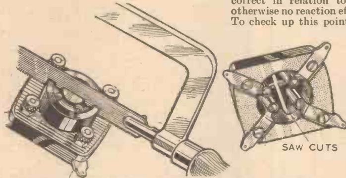
Fig. 4.—Showing the method of modifying an ordinary valve-holder for use in the short-wave set. The bakelite is sawn away between the sockets.
