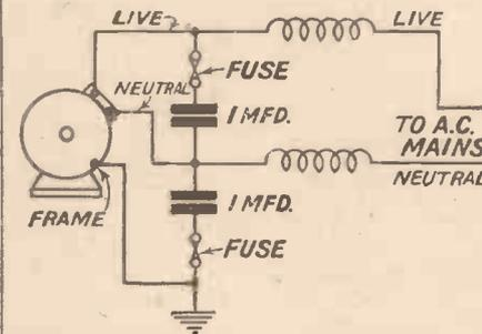
Fig. 2.—Stationary fractional-H.P. universal or A.C. motors operating on A.C. are best silenced as shown, the condensers being 1 mfd. each. Chokes need only be added in difficult cases. The wiring of the condensers depicted is recommended where the brushes are inaccessible. Note that the mains plug must not be reversible.
