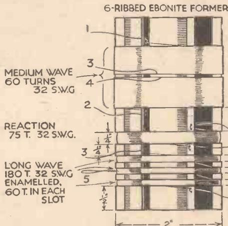
Fig. 2.—This drawing, reproduced from a previous article of this series, gives constructional details of the coil employed for the H.F. amplifier.
