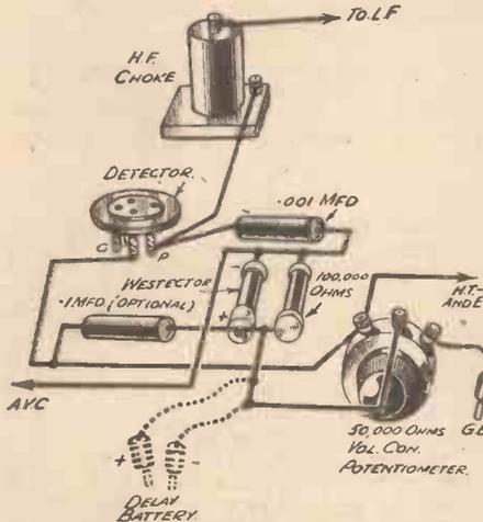
Fig. 4.—Manual and automatic volume control can be obtained by using the connections shown here.
