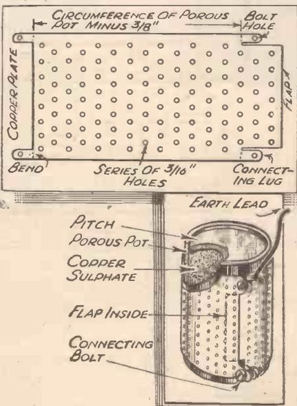
An efficient earth made from a disused Daniell cell.
