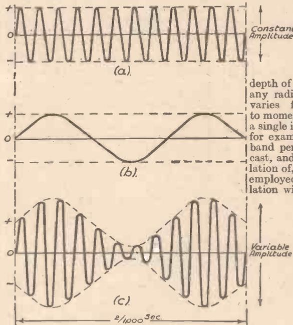
Fig. 1.—Showing how L.F. and H.F. waves are combined to give a modulated H.F. wave.
