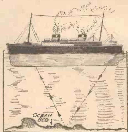
Fig. 3.—The depth of the ocean may be ascertained by means of the reflection of the radio signal. This illustration gives an idea of the method employed.
