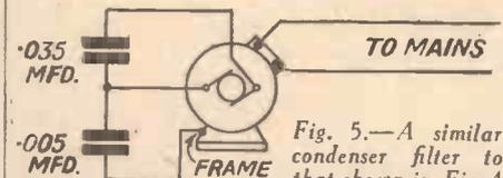
Fig. 5.—A similar condenser filter to that shown in Fig. 4 but connected across the motor brushes.
