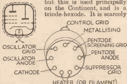
Fig. 1.—The connections and theoretical diagram for a triode-pentode frequency changer.
