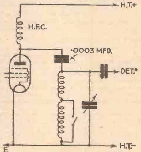
Fig. 4.—A circuit in which a fixed condenser is used as a stopper and also for H.F. coupling.
