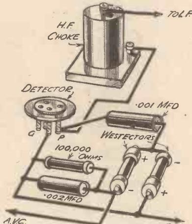
Fig. 3.—A greater measure of A.V.C. can be obtained in a single H.F. receiver by using the "voltage-doubler" rectifier circuit shown here.
