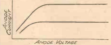
Fig. 2.—Showing how with a screened pentode valve the anode current is constant after a certain minimum anode voltage is reached.
