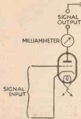
Fig. 4.—Checking modulation with an anode circuit milliammeter.
