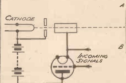
Fig. 3.—Including an amplifying valve in an anode modulation circuit.
