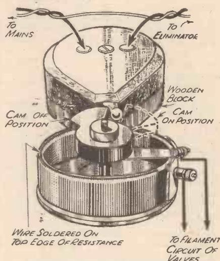
A useful combined filament and eliminator switch.
