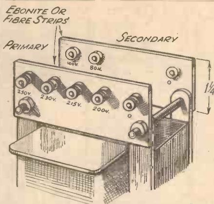
Fig. 4.—This sketch shows a simple method of arranging terminal connections for the mains transformer.
