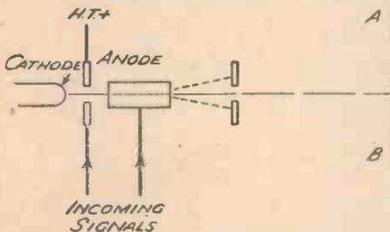
Fig. 5.—Interposing an apertured mask to cut off the electron beam in accordance with incoming signal intensity.
