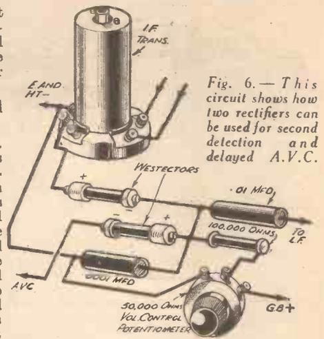
Fig. 6.—This circuit shows how two rectifiers can be used for second detection and delayed A.V.C.
