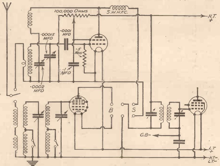
Fig. 2.—Showing how a short-wave converter can be used in conjunction with a modern superhet, a switch causing the broadcast frequency changer to be replaced by the short-wave unit.
