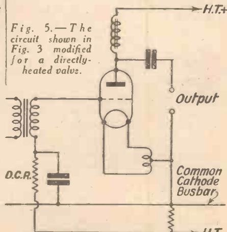
Fig. 5.—The circuit shown in Fig. 3 modified for a directly-heated valve.
