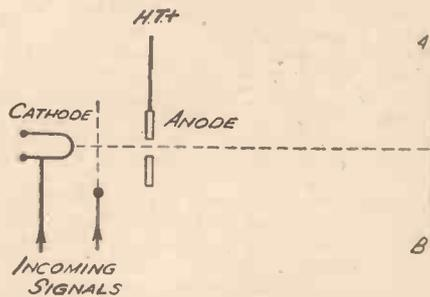
Fig. 1.—Inserting an additional mesh electrode between cathode and anode for modulation purposes.
