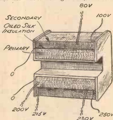
Fig. 5.—The connections for the various transformer tapping are shown in the cut-away sketch.
