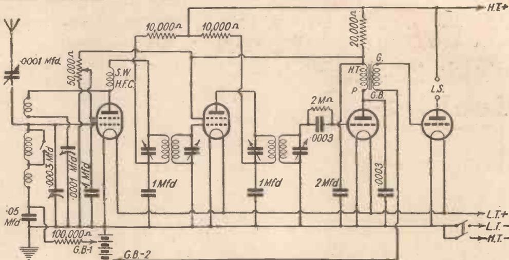
Fig. 3.—Circuit diagram of a short-wave superhet.
