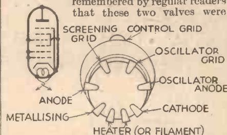
Fig. 3.—Valve base connections and theoretical diagram are here shown for the Mullard Octode FC 13.
