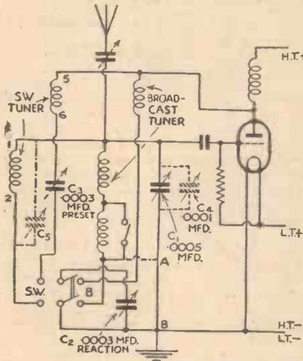
Fig. 1.—This theoretical and pictorial circuit (Fig. 2) show the method of adding a short-wave tuner to a broadcast receiver to enable all-wave reception to be obtained. The condenser shown connected by broken lines, as well as the connections shown by chain lines, is referred to in the text. The link between points A and B should be removed when using the connections shown by chain lines.
