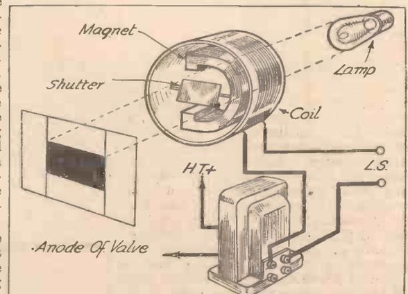
Fig. 5.—A visual tuning indicator in which a shutter is used to vary a band of light for giving the desired indication.
