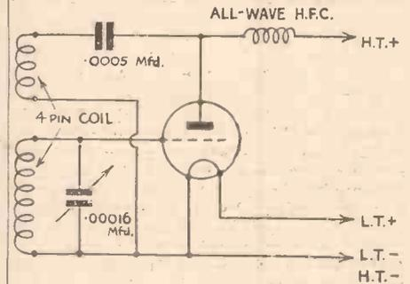
Fig. 5.—Showing the circuit of an oscillator suitable for use as a heterodyne wavemeter.
