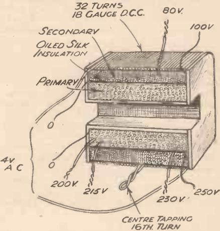
Fig. 1.—Showing how the 4-volt L.T. A.C. winding can be added to the mains transformer previously described.
