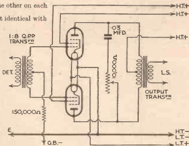
Fig. 4.—A Q.P.P. circuit showing the tone-control components referred to in the text.
