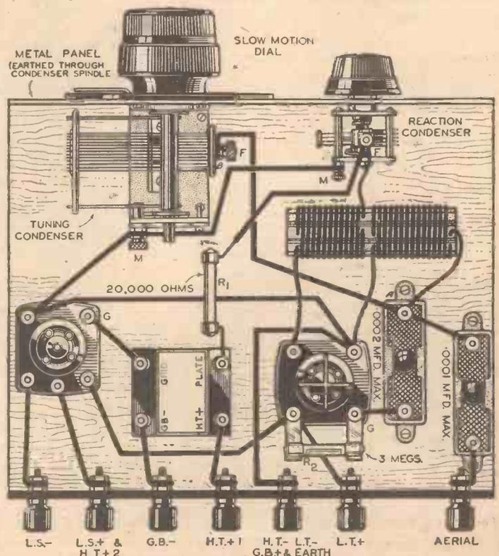
Fig. 2.—Plan of the receiver showing the suggested layout and wiring. The coil is shown in a horizontal position to clarify the connections.
