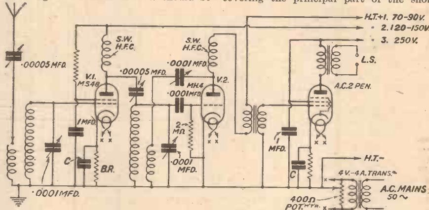
Fig. 2.—Theoretical diagram of a three-valve A.C. short-waver.
