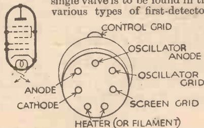
Fig. 2.—Showing the valve base connections and diagram of an indirectly-heated pentagrid or heptode. The base connections are the same for an octode.
