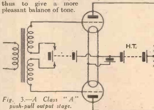
Fig. 3.—A Class "A" push-pull output stage.
