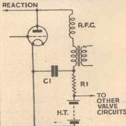
Fig. 4.—A simplified form of the decoupled detector circuit shown in Fig. 2.
