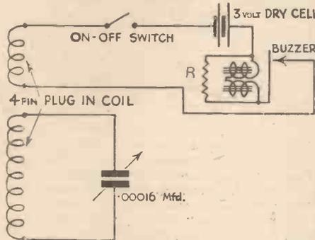
Fig. 4.—The circuit for an efficient buzzer wavemeter of the type described.
