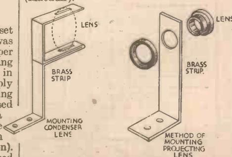
Fig. 3.—Showing the method of mounting the lenses.
