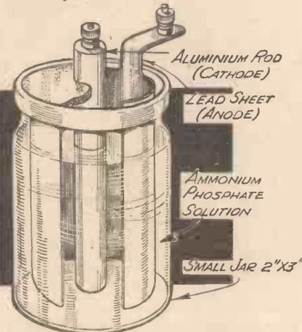
Fig. 2.—Showing how each of the two chemical-rectifier units are made. A fibre disc should be fitted to the cathode to hold it central, but this is omitted from the drawing for clarity.
