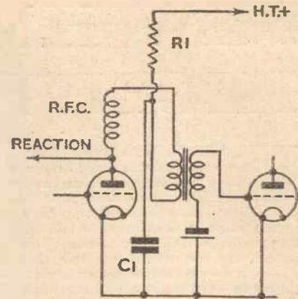
Fig. 2.—The same circuit as in Fig. 1, but with decoupling resistance and condenser added.
