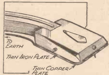
Method of fitting a metal shield to a pick-up for preventing noise.
