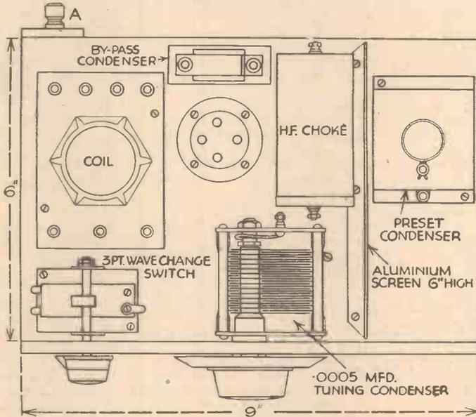
Fig. 6.—This drawing shows a suitable layout for the components of the H.F. amplifier.
