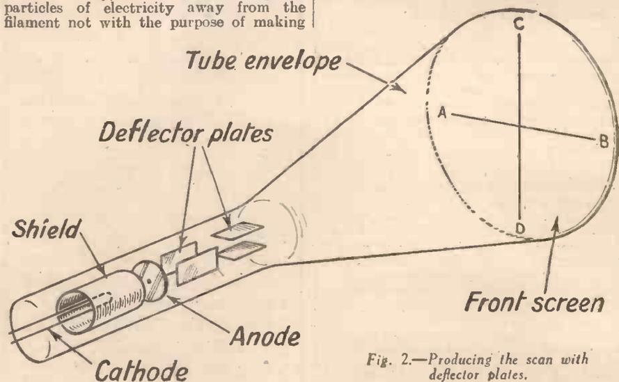
Fig. 2.—Producing the scan with deflector plates.
