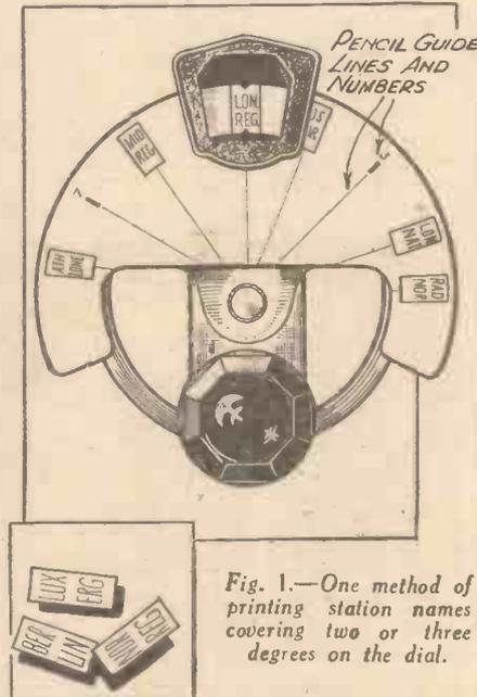
Fig. 1.—One method of printing station names covering two or three degrees on the dial.
