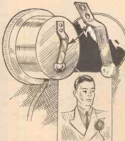
Showing constructional details and method of fixing the microphone to the lapel of a coat. F. J. G. (Ellesmere).
