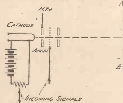
Fig. 2.—Another suggestion for intensity modulation which included a potentiometer control.
