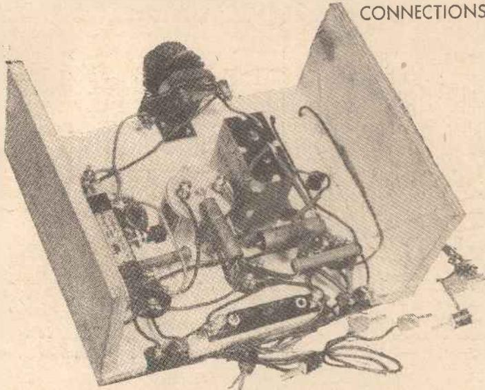
Sub-chassis view of the Hall-Mark Cadet. Examine this in conjunction with the diagram on the next page when wiring the receiver.
