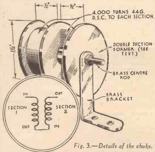
Fig. 3.—Details of the choke.
