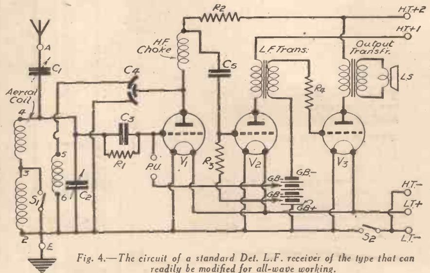
Fig. 4.—The circuit of a standard Det. L.F. receiver of the type that can readily be modified for all-wave working.
