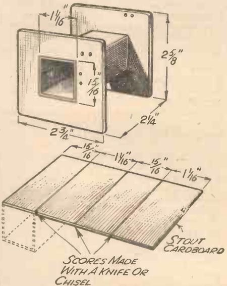
Fig. 3.—Details of the transformer winding spool are given in these sketches.
