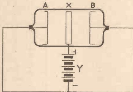
Fig. 1.—A simple diagram of a cold-cathode tube.
