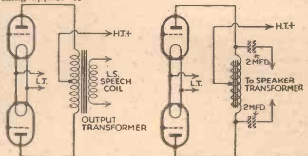
Fig. 3.—Two different methods of feeding the speaker from a push-pull amplifier. The transformer method on the left is best when the speaker is not fitted with its own transformer; that on the right is suitable for use with a speaker provided with an ordinary (not centre tapped) transformer. The two condensers shown in broken lines are optional, but to be preferred in the case of a mains receiver.
