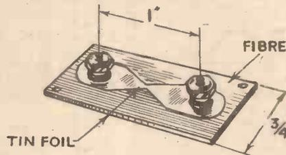
Fig. 4.—This sketch shows how the mains fuses can easily be made.
