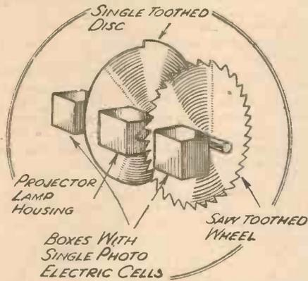
Fig. 4.—Positioning a lamp between two discs, having teeth cut as shown to produce the required signals from photo-electric cells.
