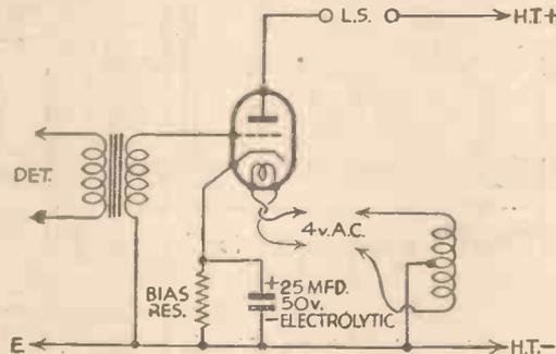
Fig. 4.—Showing the simple modifications required in the L.F. circuit.
