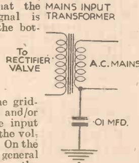
Fig. 6.—Removing modulation hum with a fixed condenser.
