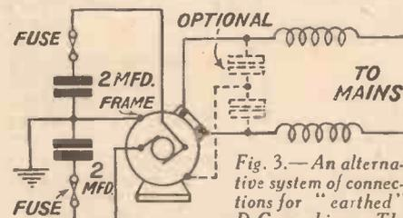
Fig. 3.—An alternative system of connections for "earthed" D.C. machines. The condensers (2 mfd.) are joined directly across the brushes. The chokes are optional.
