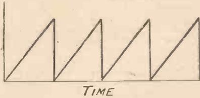
Fig. 1.—A "saw-tooth" movement is in effect traced out by the scanning spot.
