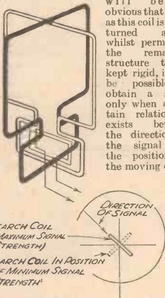
Fig. 1.—Explanatory diagram of a direction-finder (generally referred to as a radio-goniometer), together with a sketch showing how the rotatable coil gives the direction of a transmitter.
