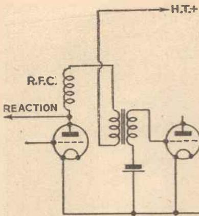
Fig. 1.—The plate circuit of a detector valve without decoupling arrangements.
