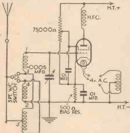
Fig. 5.—The altered connections in the cathode circuit of the H.F. valve are shown here.
