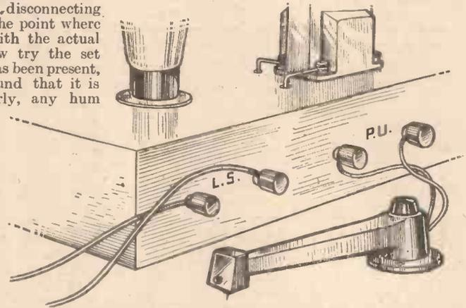
Fig. 3.—The first step in tracing the cause of trouble is to join the pick-up direct to the P.U. terminals, excluding all long (and screened) leads and switches, etc.
