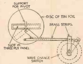
Fig. 2.—Details of the shutter.
