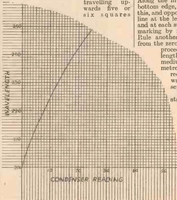
Fig. 2.—Showing how the squared paper is marked out for condenser and wavelength readings.
