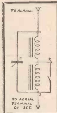
This Circuit shows how simple it is to trap the unwanted signals in your Set and listen free from local interference.
