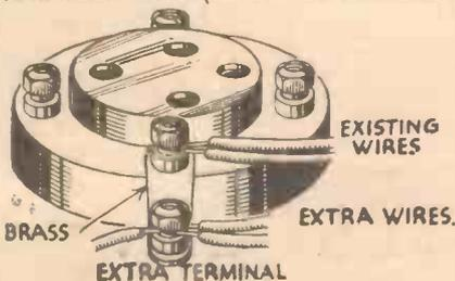
An easily-made wire-connecting link.
