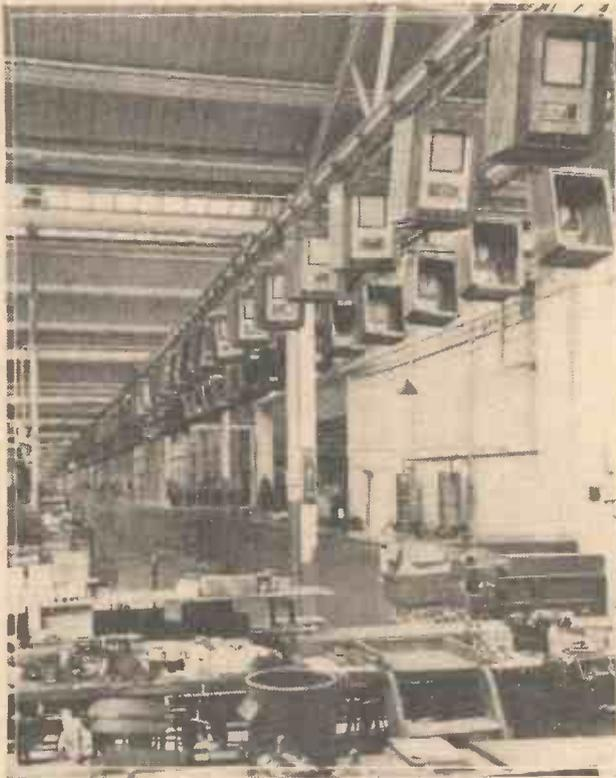
The popularity of the new Ferranti AC/DC receivers is evidenced by the display of activity seen in the above illustration, which shows a large batch of cabinets in the Hollinwood Factory being delivered from the cabinet-making shop to the receiver-assembly department.
