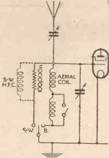
Fig. 3.—Showing how a fixed resistance or S.W. H.F. choke can easily be used in place of the aerial coil in a receiver with an H.F. stage.
