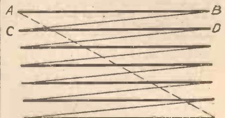
Fig 3.—The heavy and faint lines represent respectively the normal line traverse and quick return stroke.
