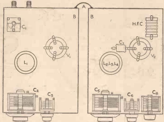
Fig. 3.—A suggested layout for providing efficient screening.
