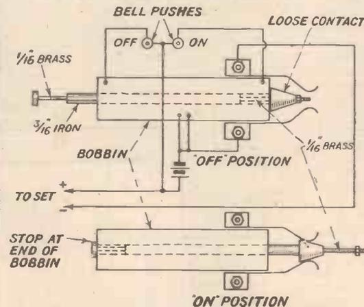
Fig. 1.—Details of a simple remote control switch, showing connections.
