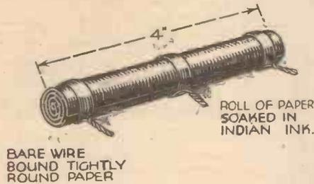
Fig. 5.—This sketch shows how the fixed screening-grid potentiometer can be made.
