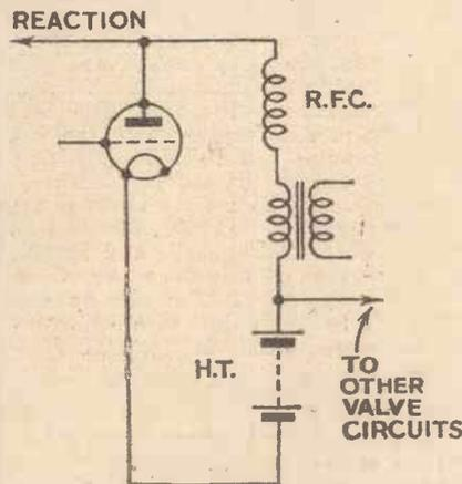
Fig. 3.—A simplified form of the detector circuit shown in Fig. 1.
