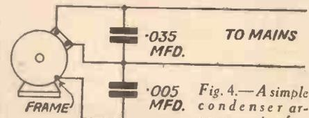
Fig. 4.—A simple condenser arrangement for gramophone motors (D.C. and universal), hair dryers, toy motors, small fans, and similar devices. The system is applicable to commutator motors on both A.C. and D.C. supplies. Earthing the motor frame can be tried, but is not always essential.
