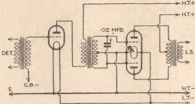
Fig 5.—This circuit is for a complete driver—class B stage. Note the inclusion of a .02 mfd. condenser across the secondary windings of the driver transformer for preventing undue high note response.
