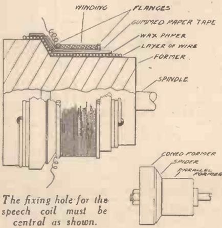
coil can be left for a few hours to dry, after which the binder is removed. Then prepare some very narrow strips of paper, and gum these on the former to form a ridge of the required height.
