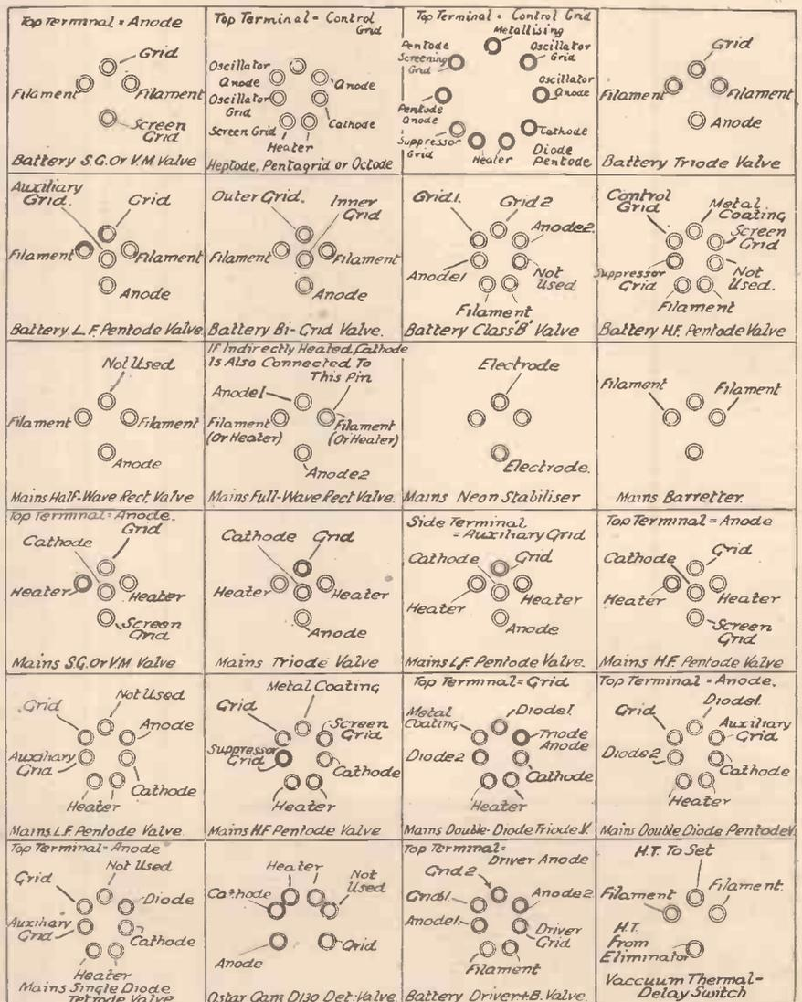
Showing the pin connections for a variety of popular valves. The connections are as seen on top of the valve holder.
