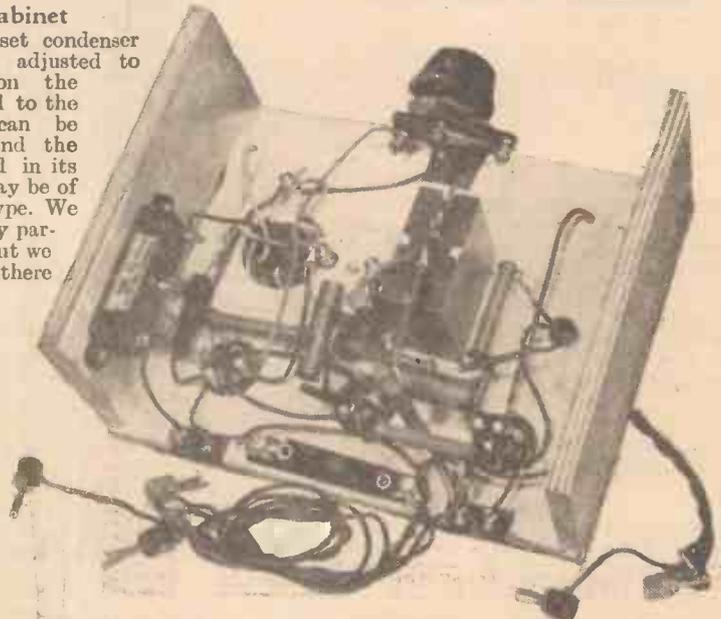
An underneath view of the receiver, which shows the position of the pre-set condenser.
