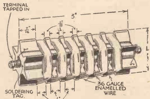
Fig. 3.—Winding data for the choke are given in this drawing.
