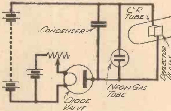
Fig. 5.—The simplest time base circuit to explain the action.
