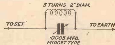
Fig. 3.—A filter for preventing induced hum.
