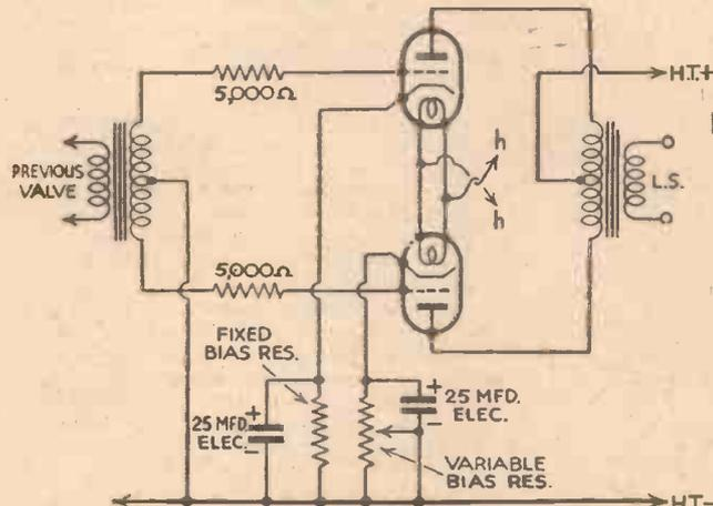
Fig. 2.—When using two indirectly-heated valves in push-pull it is a simple matter to obtain accurate matching by using a variable bias resistance for one valve, as shown here.
