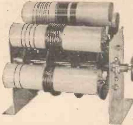
A commercial tuner designed to cover short waves as well as the medium and long.
