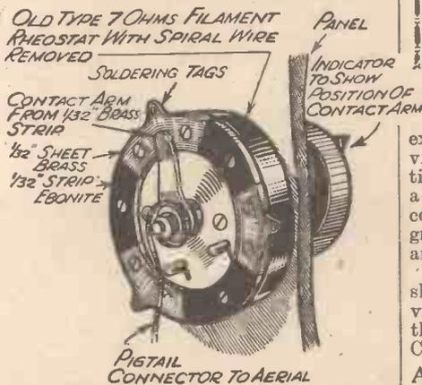
A useful multi-control switch made from an old filament rheostat.
