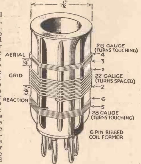
Fig. 5.—The above drawing gives details of short-wave coils suitable for use in carrying out the experiments described. Appropriate numbers of turns for the aerial, grid, and reaction windings for 12-22, 20-50, and 48-90 metres respectively are: 3, 4, and 5; 5, 7, and 10; and 4, 6, and 8.
