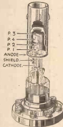
Fig. 5.—The electrode system of a cathode-ray tube in which the Wehnelt cylinder is indicated as a shield.
