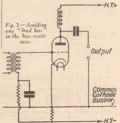
Fig. 3.—Avoiding any "load loss" in the bias resistance.
