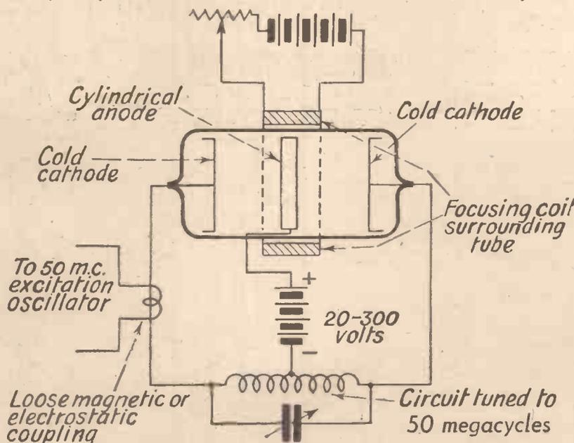
Fig. 2.—The complete circuit for a cold-cathode "valve."
