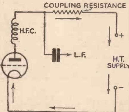
Fig. 2.—A theoretical circuit showing how the coupling resistance is virtually in parallel with the valve, the H.T. supply completing the circuit.
