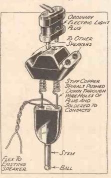
Method of connecting additional speakers by using a three-way lighting plug.
