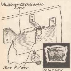
An easily-arranged light-line indicator for a tuning dial.
