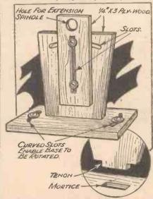
An extension-rod support which provides for universal movement.
