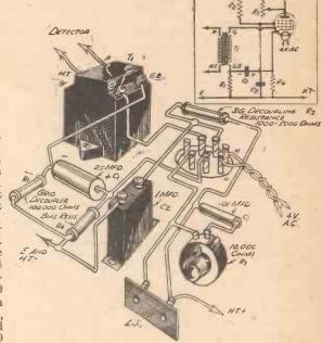
Fig 3.—Showing the method of decoupling the grid and screening-grid circuits of an indirectly-heated pentode.
