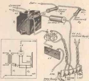
Fig. 4.—Showing the connections for a directly-heated output valve.
