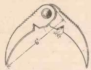
A multiple tool made with parts of a hack-saw blade.
