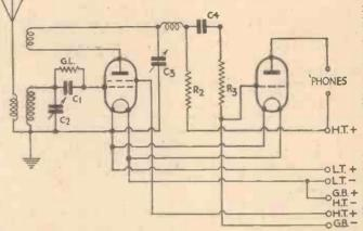
Fig. 2.—A circuit incorporating S.G. Detector, and R.C.C. L.F. stage. C1=.0001 mfd., C2=.0001 mfd. to .00016 mfd., C3=.0001 mfd. to .00016 mfd., C4=.01 mfd., GL=3 megohms, R2=.0001 mfd. 100,000 ohms, and R3=1 megohm.
