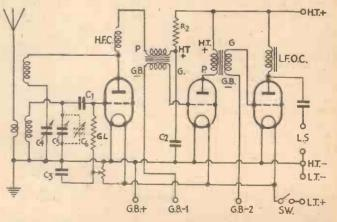
Fig. 3.—Circuit for a straight three-valve short-wave receiver with two stages of L.F. transformer coupling. C1=.0001 mfd., C2=2 mfd., C3=1 mfd., C4=.00016 mfd., C5=.00016 mfd., C6=B and Spread (capacity will depend upon coils used), R2=20,000 ohms, GL=2-3-5 megohms, R3=400 ohms potentiometer. SW=on-off switch.
