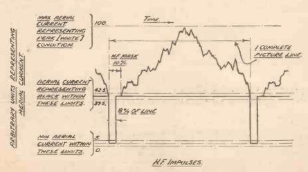
Fig. 1.—Picture modulation and synchronising impulses of the Baird system. These drawings are made from tracings taken from the vision transmitter monitoring oscillograph.
