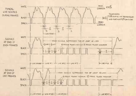
Fig. 2.—The transmitted wave-form of the Marconi-E.M.I. high-definition system.
