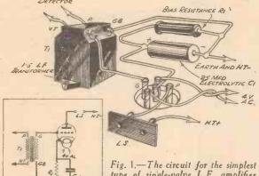
Fig. 1.—The circuit for the simplest type of single-valve L.F. amplifier using an indirectly-heated triode
