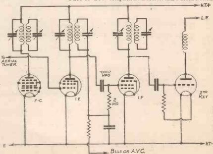
Fig. 3.—A skeleton circuit showing the connections used in eliminating the frequency-changes when there are two I.F. valves.
