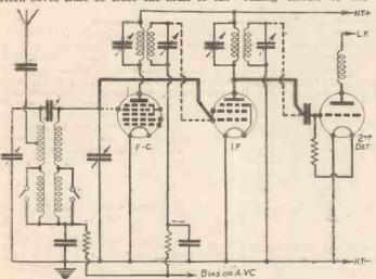
Fig. 1.—This skeleton circuit shows how the frequency-changer of a typical superheterodyne can be cut out of circuit, so converting the set into a "straight" arrangement. Broken lines indicate original connections, and heavy lines the new connections.
