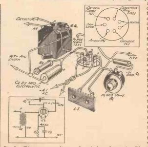
Fig. 2.—The connections for an indirectly-heated pentode. The pictorial view shows the valve connections when using a pentode with side-base screening-grid terminal, but inset are connections when using a seven-pin valve.
