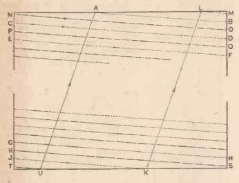
Fig. 3.—Diagram explaining the E.M.I. system of interlaced scanning.
