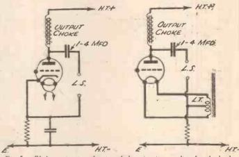
Fig. 5.—Skeleton circuits, showing choke-capacity coupling for the loudspeaker when using indirectly- and directly-heated valves.
