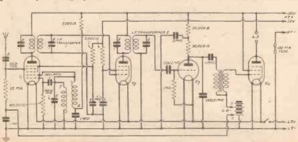
Fig. 1.—The simple circuit of the four-valve battery-operated superhet described.
