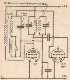
Fig. 4.-When a double-diode-triode tupe of valve is used as second detector the I.F. transformer which feeds it should be replaced by a double-wound tuner and .0005 mfd. variable condenser as shown here.
