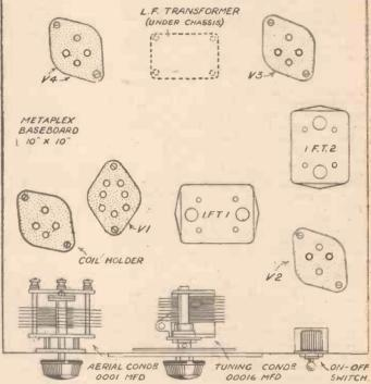
Fig. 2.—This illustration gives a good idea of a suitable component lay-out for the circuit described.
