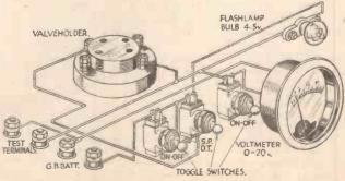
A simple apparatus for testing valve filaments.
