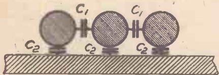
Fig. 1.—This diagram illustrates the stray capacities which exist in a coil.
