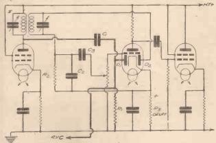
Fig. 4.—A circuit for Delayed A.V.C. using a double-diodetriode valve.
