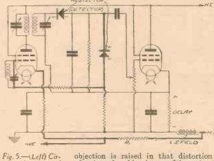
Amplified Delayed A.V.C. using a
