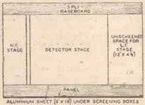
Fig. 3. - Details of construction of baseboard, panel, and screening compartments.
