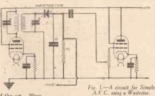
as Simple A.V.C., and using a Westector, is shown in Fig. 1.
