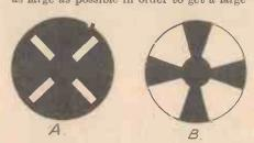
Fig. 7.—The image appearing on the screen of the Mullard electron beam tuning indicator, under conditions of (A) no signal, and (B) maximum signal.
