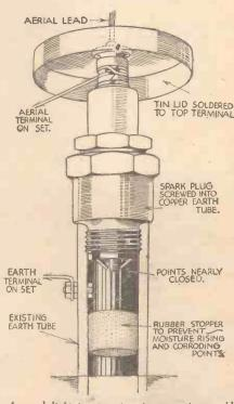
A novel lightning arrester, incorporating an old sparking plug.
