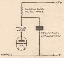
Fig. 1.—This diagram shows how a shorted decoupling condenser will short-circuit the H.T., and probably damage the decoupling resistance.
