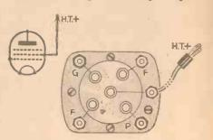
Fig. 3.—This illustration shows the theoretical representation of a pentode valve and how the additional connection is made to the 5-pin valveholder.
