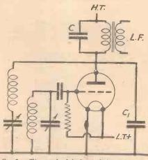
Fig. 3.—The standard leaky-grid detector circuit.
