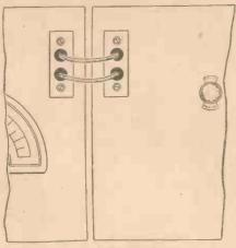
4.—How the crystal set and the amplifier are connected together.
