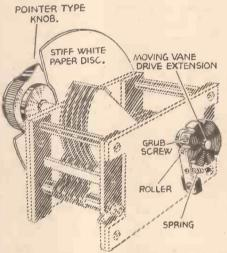
A method of setting a band-spread condenser.
