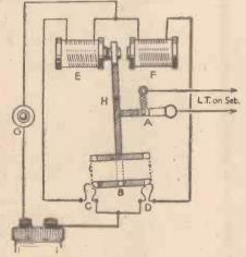
General arrangement and connections for a singlepush remote control.
