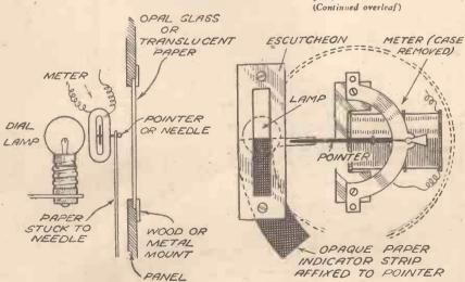
Fig. 3.—Elevation and side view of the method of converting an ordinary milliammeter to give an indication of tuning by light or shadow.
