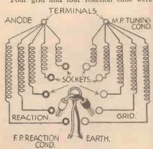
Diagram of connections for a five-range short-wave coil.
