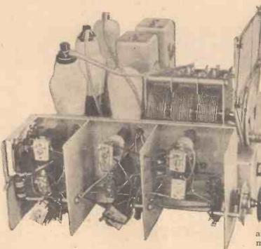
A view of the coil unit with screen removed to show the general
