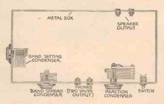
Fig. 2.—A different scheme in which 'phone connections may, be easily made, and the tuning circuit is more efficiently wired.
