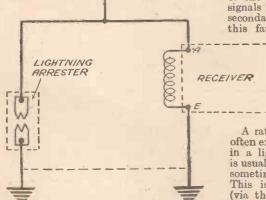
Fig. 2.—How the lightning arrester is included across the aerial coil.
