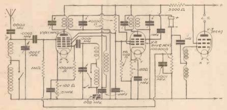
Fig. 1.—Circuit of the set described. It is a modification of the A.C. version of the "£5 Superhet."
