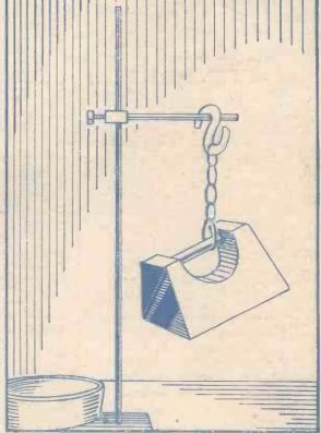
An amazing experiment with Liquid Air. Here you see a hook of meroury, made solid by freezing in Liquid Air, suspending a 7lb, weight.
