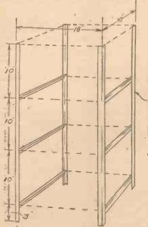
Fig. 1.—Method of building up the rack frame-work for the 10-watt transmitter.
