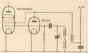
Fig. 3.—Showing the addition of a triode to a pentagrid for improved S.W. reception.
