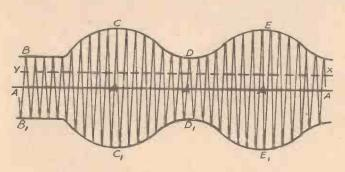
Fig. 1.—Diagram of carrier wave and audio-frequencies, showing correct (A), and incorrect (X) tuning points.
