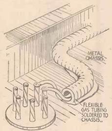
Using flexible metallic tubing for screening heater leads.
