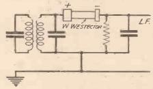
Fig. 6 .- In a superhet the second detector may take this form if a Westector is employed.
