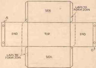
Fig. 2.—Developed blank for making the metal cover for the mains units
