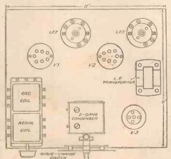
Fig. 2—Approximate positions of the principal components on the baseboard, which is mounted on 1-in. side runners.
