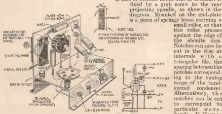
General view and theoretical circuit diagram of a pre-detector H.F. amplifier unit. (Stroud).
