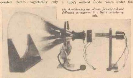
cathode, modulator and single anode constitute the whole electrode assembly. The scheme adopted for focusing, therefore, must be one which performs its function external to the neck of the tube. For this fasciculating action the rather complicated multiple anode assembly is replaced by a solenoidal coil of wire slipped over the neck
