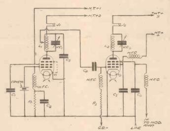
Fig. 4.—The oscillator and power amplifier circuit.
