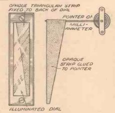
Fig. 4.—Method of arranging for an "eye".
