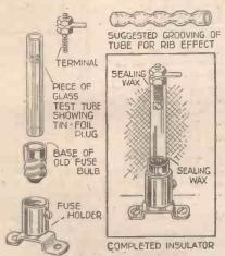
A method of making small stand-off insulators.
