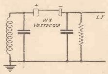
Fig. 5.—Circuit of a detector stage utilising a Westector.
