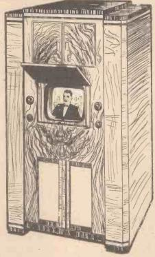
The G.E.C. Television Receiver. Note that the panel controls are reduced to a minimum, and a protecting cover is provided for the end of the C.R. tube.
