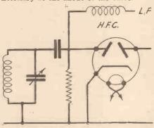
Fig. 4.—The diode detector stage in theoretical
