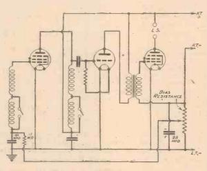
Fig. 4.—A method of obtaining fixed and variable bias "automatically." There are disadvantages in this arrangement and these are described in the text.
