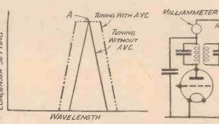
Fig. 2.—A.V.C. tends to give an apparent flattening of the tuning, thereby losing the exact resonant point A.
