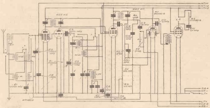
Theoretical Circuit of the "Vitesse" All-waver. It will be noted that certain components do not bear any reference number or value, and these parts are already included in the special coil unit. The make and type numbers of the remaining components may be seen in the list given below.
