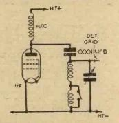
1.-Simplest arrangement of Fig. tuned-grid coupling.
