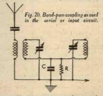
responsible for greater secondary e.m.f. at the upper end of the frequency range. Very small capacity values are used for top end coupling condensers.
