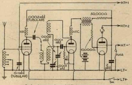
Fig. 3. A conventional untured H.F. short-wave receiver circuit.
