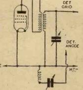
Fig. 4.—A double-wound coil used for tuned - transformer coupling. Reaction connections are also shown.
