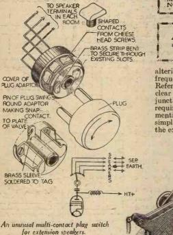
by passing these brass strips through the slots and bending over, as shown.
