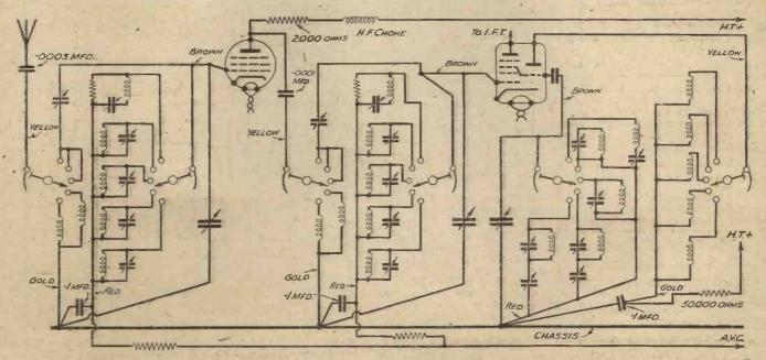
Fig. 2.—Theoretical diagram of the tuner. Note that various earth connections are made to single points to keep the circuits separate
