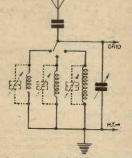
Fig. 7.- A simple method of all-wave tuning by using three separate coils with a three-way switch.
