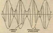
Fig. 2.—Showing the shape of the modulation envelope after the L.F. oscillation has been applied to the train of C.W.
