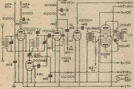
Theoretical circuit diagram of Mr. G. C. Castle's short-wave battery receiver with Q.P.P. output.
