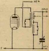
Fig. 5.—It is necessary to use a D.P.D.T. wavechange switch in a circuit of this kind.
