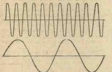
Fig. 1.—A train of continuous waves before modulation is applied. The lower curve represents an L.F. oscillation which will be used for modulating purposes.
