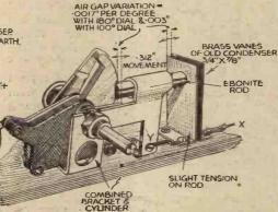
A novel device for modifying the tracking of a condenser.
