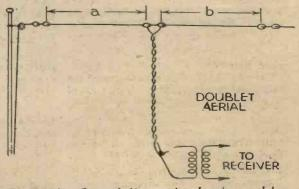
Fig. 3.—An efficient doublet aerial. Lengths a and b are equal to a wavelength depending on the waveband concerned.
