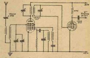
Fig. 5.-Skeleton diagram of a converter for use with a broadcast It incorporates both frequency - changer and I. F. superhet. valves.
