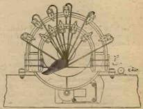
These illustrations show the Ekco mechanism and the arrangement of the motor and selector clips.
