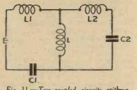
Fig. 11,-Two coupled circuits with a common inductance.
