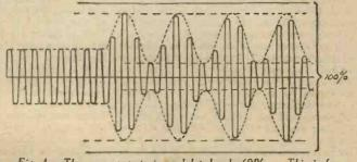
Fig. 4.- The same wave-train modulated only 60%. This is far better than Fig. 5.
