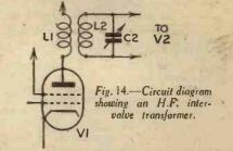
The primary current sets up a secondary e.m.f. equal to  $\omega MI_1$  volts (where  $I_1$  is primary current). As the secondary is in resonance its impedance will simply be R2 (R2 representing the H.F. resistance of the secondary circuit), so the secondary current will be  $\omega MI_1/R2$  amps.
