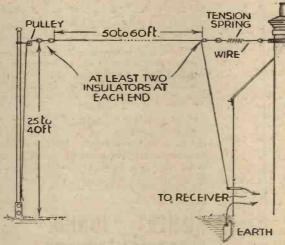
Fig. 2 .- An ideal arrangement for an inverted "L" type of aerial.
