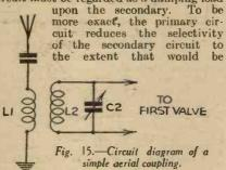
caused by an extra H.F. resistance of  $(cM)^2/Ra$  thrown into the secondary. This brings to light two interesting facts: (1) The resistance (Ra) of the valve has a considerable bearing upon the selectivity, and (2) Selectivity, as well as amplification, is dependent upon the coupling. Selectivity, however, progressivly improves with loosening of the coupling.
