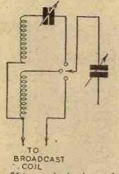
Fig. 5.—Efficiency on the ultra-short wavelengths may be increased by including a small capacity in series with the ultra-short-wave coil.
