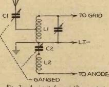
Fig. 2.—A circuit for providing constant selectivity.
