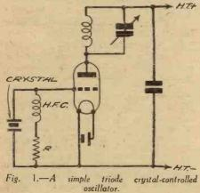
amateurs as they possess many desirable features which help to overcome some of the snags encountered with triode circuits. It will be remembered that a crystal has certain safe working limits; it must not be subjected to excessive strains or currents, thus the power output obtainable is usually low compared to that so often desired.
