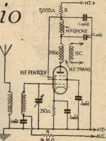
A typical circuit for an H.F. amplifier.
