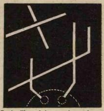
Fig. 1.—Wires which cross without touching are always indicated by one of the schemes shown above.
