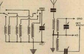
Fig. 8.—An improved form of the all-wave tuning system, shown in In this case each tuned Fig. 7. winding has its own primary or aerial winding.
