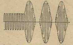
Fig. 5.—Showing the effects of over modulation. Note the wave form distortion and breaks in the carrier.
