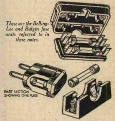
component possesses the advantage that the mains leads are protected and the removal of the lid which contains the fuses in clips still permits the live leads to be protected so that the nser cannot receive a shock.
