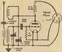
Fig. 2.—An S.W. adapter circuit which replaces the detector and preceding valves (if any) in the broadcast set.
