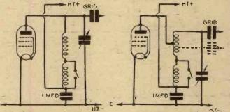
Fig. 3.-Tuned-anode coupling, using tapped and untapped dual-range coil.
