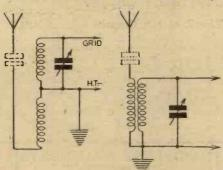
Fig. 4.-Although they appear different. these circuits for a separate aerial winding are identical.
