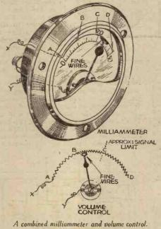
vice versa. In the construction of such an instrument as described it is important that the surface of the resistance AD should be level and parallel to the path of the needle, otherwise the latter may stick.-T. H. PHILLIPS (Shirley).
