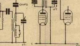
Fig. 8.—Usual connections for an untapped I.F. transformer.
