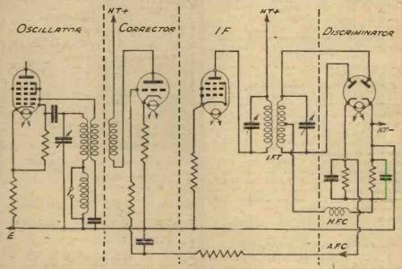
This skeleton diagram illustrates the principles described, and shows how the discriminator and corrector values are connected.
