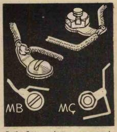
Fig. 3.—Common earth return points are joined to screws or bolts in the chassis, and are indicated as shown in this illustration.
