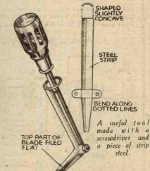
small nut and bolt. This tool will be found useful for such jobs as holding small nuts in place, picking up blobs of solder, etc. With the steel jaw removed the bent driver is handy for removing stubborn valves from their sockets, adjusting trimming con-densers, and many other little jobs where an ordinary screwdriver would be useless. --G. H. HUNTER (Ashington).
