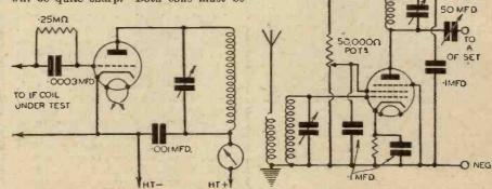
checking the frequency of I.F. coils.
