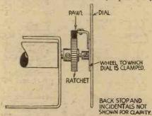
Fig. 3.—The ratchet device which provides the "locator."
