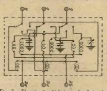
Fig. 2.—The circuit which is employed in the Wearite all-wave tuner.
