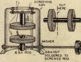
Fig. 1.—Details of a variable coupling 1.F. transformer, arranged so that one coil can be rotated through an angle of 90 degrees.
