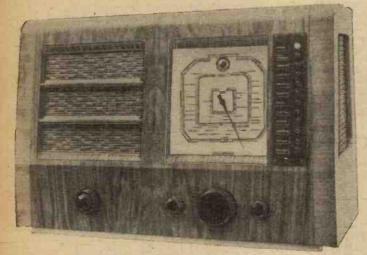
The Ekco receiver, which embodies the motor tuner.
