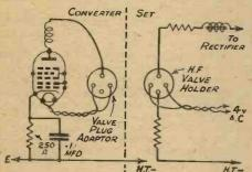
Fig. 4.—How an A. C. converter can be fed with H. T. and L. T. from most existing H. F.-type A. C. receivers.
