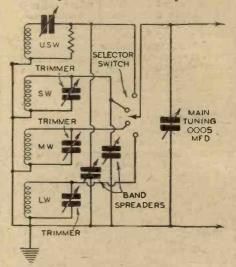
Fig. 7.- A comprehensive all-wave tuning circuit, showing how to incorporate all refinements as mentioned in this article.
