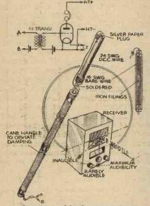
A novel tester rod for detecting resonance.
