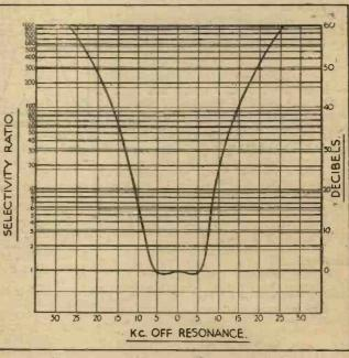
Fig. 22.-Graph showing the selectivity rating of a receiver.
