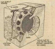
An effective method of mounting a microphone to avoid "boom" effects.
