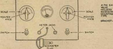
Fig. 6.- A suggested lay-out for the panel of the Tritet section. Keep
