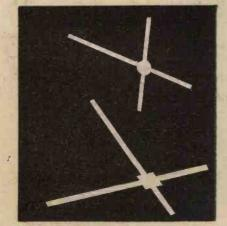
Fig. 2.—Wires which are connected or attached to each other are shown as above.
