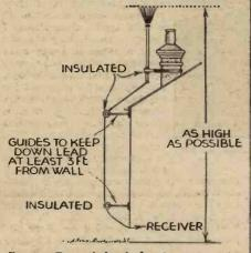
Fig. 4.-Essential details for the erection of a vertical aerial arrangement.
