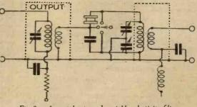
Fig. 2.- A crystal gate and variable selectivity filter.
