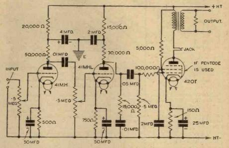
Fig. 6.—The circuit of the modulator stage, fixed tone control being applied and a jack inserted in the output anode circuit for current indication.
