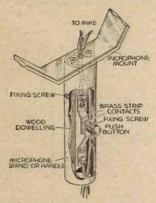
A safety-switch for a home-made microphone stand.
