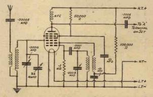
Fig. 3.—A converter circuit using a pentagrid frequency-changer.
