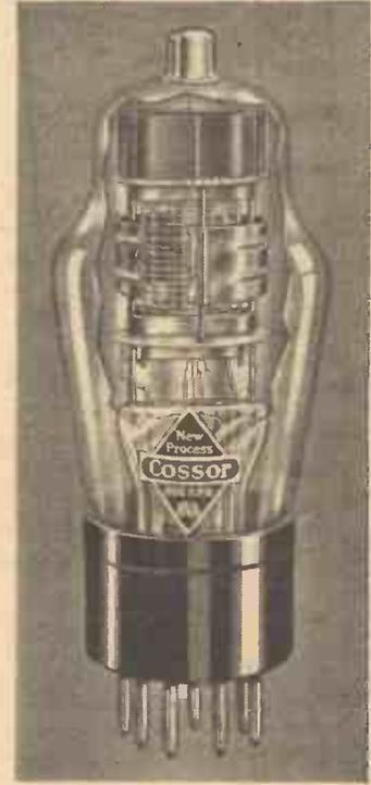
The 202 S.P.B. is an indirectly heated valve intended for use in universal receivers. It is characterized by its high slope and is particularly suitable for use as a grid detector. The control grid is connected to the top cap which is convenient in all-wave receivers and in addition, minimises the pick-up of mains hum.
