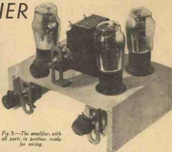
Fig. 3.—The amplifier, with all parts in position ready for wiring.
