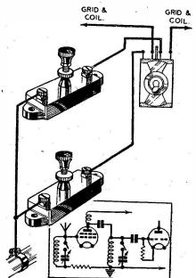
Fig. 2—A simple scheme in which ordinary on/off switches are employed. Only two are shown, but any number may be used.
