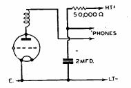
Fig. 3.—Showing an alternative method of feeding the phones.
