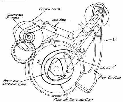
Fig. 5.—Simplified diagram of the H.M.V. unit showing cluich mechanism, gearing, and pick-up cams.
