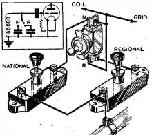
Fig. 4—A change-over switch to bring in the required pre-set.
