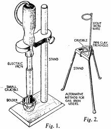
A novel method of keeping soldering irons tinned while in use.
