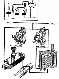
Fig. 3—For tuning more than one circuit, combination switches of this type may be employed.
