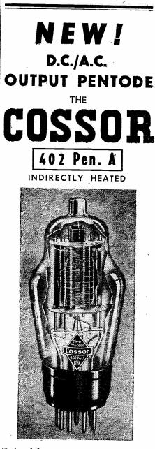
Designed for series running in A.C./D.C. receivers, the Cossor 402 Pen. A is an output pentode of the indirectly heated cathode type. It has been designed for maximum anode and screen voltages of 150 since, in general, greater voltage is not available in the receivers in which it is used. Its maximum anode dissipation is 10 watts-sufficient to give an undistorted output adequate for all domestic purposes.
