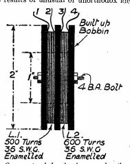
Constructional details of a quench coil.
