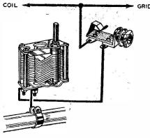
Fig. 7—A separate jack enables manual tuning to be used.
