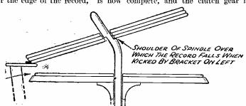
and the separator plates, which have Fig. 6.—Diagram showing the principle of operation of the latest Garrard mechanism. been isolating the The little pegs on the arms of the bracket shown on the left cause the bottom record bottom record to be shifted slightly to the right, thus passing over the shoulder of the spindle. of the pile from
