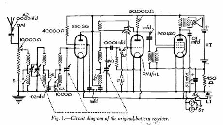
transformer connected to a leaky-grid triode detector. The latter is, in turn, connected to a pentode output valve through a parallel-fed transformer, and automatic bias is applied to the output stage by means of a 450-ohm resistor. Volume control is by means of a potentio-meter connected across the aerial coil meter connected across the aerial coil.
