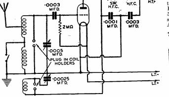
Fig. 1.—A simple scheme for an all-wave set. Plug-in coils may be added.
