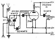
Fig. 1.—Theoretical circuit diagram of a supersimple single-valve short-wave receiver.
