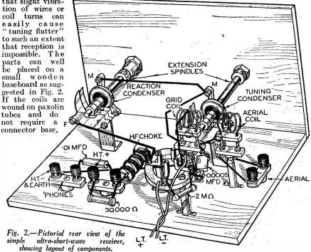
(Continued from previous tage) sections of five turns each, spacing these about <sup>1</sup>/<sub>1</sub>gin. apart. The spacing is to about <sup>3</sup>/<sub>3</sub> in. apart. The spacing is to reduce the capacity as much as possible. The ends of the winding can be brought
