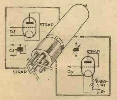
A method of utilising the inter-electrode capacity of a value.
