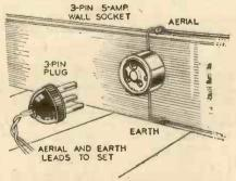
Fig. 2.—A neat arrangement for aerial-carth connections.
