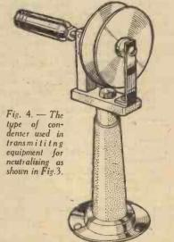
in turn, should be mounted on a bracket which is threaded (or to which a nut has been soldered so that by adjusting the rod the disc may be moved inside the coil winding. A combination of the inductance match and trimming condenser should enable the coils to be accurately matched throughout every part of the range.
