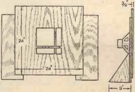
Fig. 2.—Front and side views of the suggested loudspeaker baffle.
