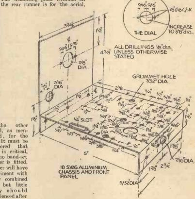
Fig. 4 .- Perspective sketch of chassis giving drilling dimensions.
