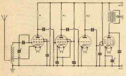
Fig. 1.-Theoretical circuit diagram of a 4-value superhet using resistance coupling throughout.
