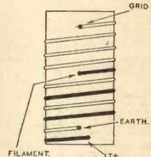
Fig. 5.-Showing the construction of an ultrashort-wave coil, the winding in series with the L.T. positive lead being wound between turns of the tuning coil.
