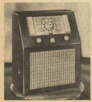
The Cossor auto-tuning system operates direct on the tuning condenser without trimmers.
