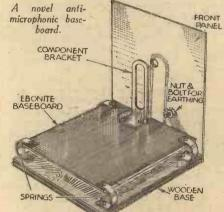
earth connections can be made to a small nut and bolt, as shown in the sketch.-RICHARD J. SHELL (W. Hampstead).
