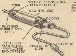
Fig. 3.-Method of arranging the H.F. choke in the H.T. lead
