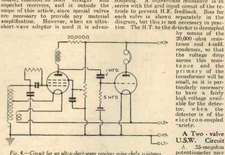
Fig. 4.-Circuit for an ultra-short-wave receiver using choke resistance coupling to the L.F. stage.
