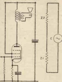
Fig. 1.—Theoretical and equivalent circuit for the output stage. Z2=L/S impedance; Z1=ValveRa; E=100v=voltage induced by alternating component of Ia.
