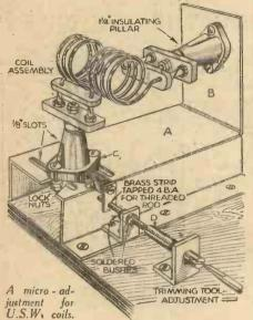
contrive a novel micro-adjusting movement, and one which will give a coupling unre-stricted by the coil supports. From the accompanying illustration, it will be seen that the horizontally mounted coiland pillar "B" whilst an adjustable slot fitting is provided for the vertical coil assembly. A brass band "C" is bent round the base of the horizontal coil support pillar,
