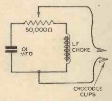
Fig. 1.-Simple circuit of a "two-way" tone control.
