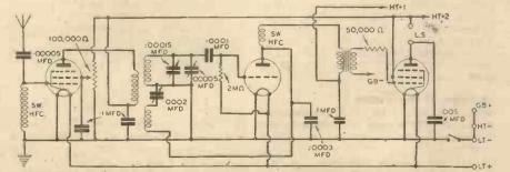
Fig. 2.—A useful three-valve combination, with one stage of untuned H.F. amplification.
