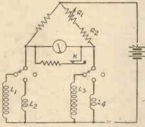
Fig. 1.—Circuit of resistance test, Wheatstone Bridge type, for loudspeaker test. R1 is calibrated in % of R2. L1 L3 Std. and Test fields. L2 L4 Std. and Test speech coils. K is meter shunt key. normally closed, to prevent inductive "kick" of field from damaging meter movement.
