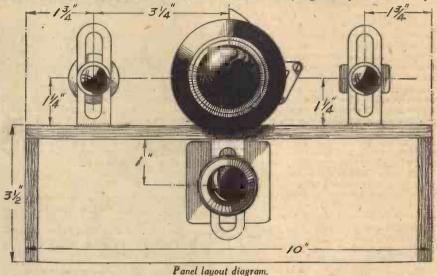
Stations are located by turning the main tuning condenser, and the strength is increased by the reaction condenser, but this should be used judiciously.
