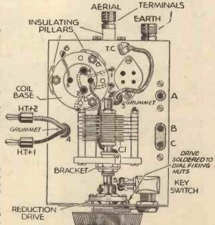
Fig. 2.- Plan view of the chassis showing layout of components.
