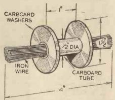
Fig. 2.—Details of the bobbin and core for the iron-core choke.
