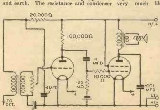
Fig. 3.- Circuit diagram of a high-gain L.F. amplifier to follow an ultra-short-wave detector.
