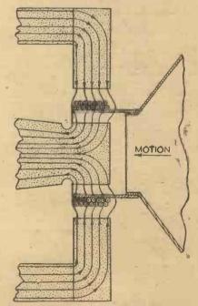
Fig. 3 .--Diagram showing distorted field due to speech current flowing in the coil.
