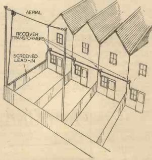
Fig. 3.—A single aerial may be erected out of the field of interference and connected to several sets by means of special transformers.
