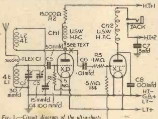
Fig. 1.—Circuit diagram of the ultra-shortwave two-valver.
