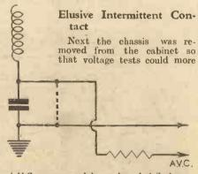
A.V.C. action ceased due to the end of the by-pass condenser touching the chassis and shorting the A.V.C. line, as indicated by the broken line. The same trouble can arise due to shorting of the con-denser wired in parallel with the A.V.C. diode load resistor.
