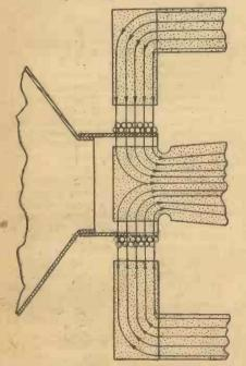
Fig. 2.—Diagram showing flux distribution when no speech current is flowing.
