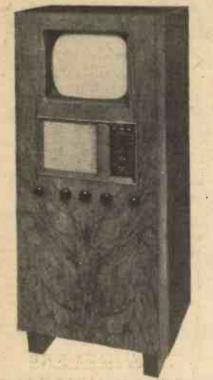
One of the new Baird television receivers which combines an all-wave radio receiver.
