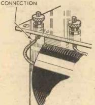
A loose connection between the transformer secondary winding and the terminal resulted in the set going off after running for a short time.
