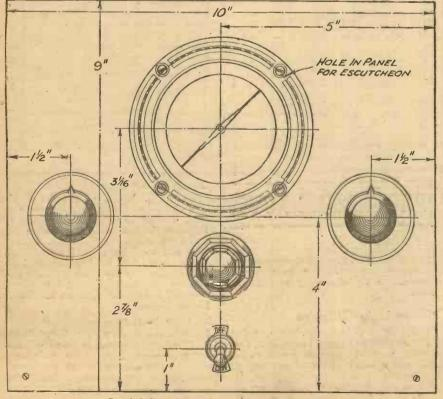
Panel drilling dimensions for the "Fleet" 2-valver.
