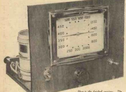
Here is the finished receiver. The crystal is on the right of the panel.
