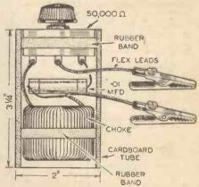
Fig. 3.—A conventent method of assembling the three components required.
