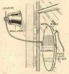
Fig. 1.—An effective lead-in arrangement when it is not wished to bore through the window or frame.
