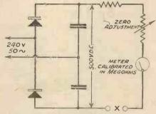
Fig. 2.—Megger test for insulation. Main voltage rectified by voltage-doubler circuit. Mains
