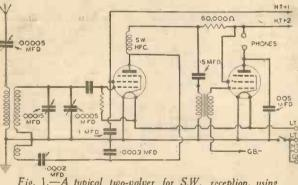
Fig. 1.—A typical two-valver for S.W. reception, using an S.G. valve and detector.
