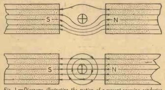
Fig. 1.—Diagrams illustrating the motion of a current-carrying conductor in a magnetic field,
