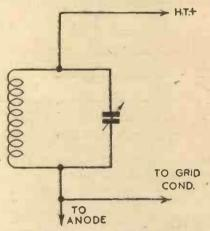
Fig. 2.—Resistances R and RI (Fig. 1) may be replaced by this tuned anode circuit.
