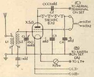
Fig. 1.—Theoretical circuit diagram of the one-value pre-R.F. amplifier.
