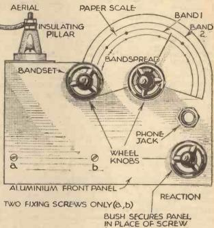
Fig. 4.-Panel layout, showing the novel dial arrangement.
