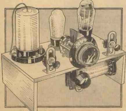
This is the finished receiver, showing the neat layout.
