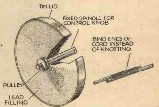
Fig. 2.—A fly-wheel made from a tin lid filled with lead, and the best method of joining driving cords.
