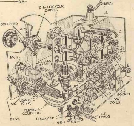
Fig. 2.-Pictorial view of rear of chassis showing layout of components.
