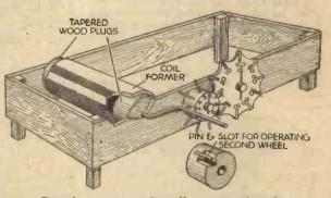
General arrangement of a self-counting coil winder.
