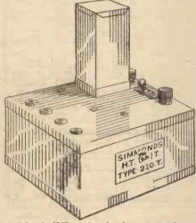
A 2-volt HT. unit with vibratory rectifier. come by using the mains unit which is fed from a battery, and which converts the low voltage into an interrupted supply which is in turn stepped up to the necessary high voltage for supplying H.T. The Simmonds unit illustrated above is designed for oper-ation from a 2-volt battery and delivers 120 volts at 10 mA. Other models are available as follows:
