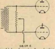
Fig. 6.- A balance for push-pull may be obtained with an ordinary transformer as shown here.
