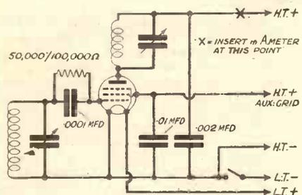
Fig. 1.—The fundamental T.P.T.C. oscillator circuit without crystal control.
