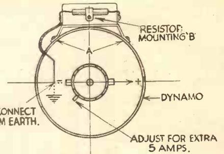
Fig. 3.—Mounting the parts on the dynamo.
