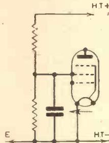
Fig. 4.—The condenser indicated by an arrow should have a low self-inductance.
