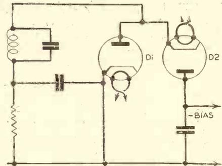
Fig. 5.—A signal limiter built round two diodes.
