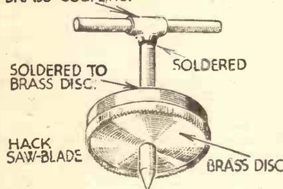
A handy tool for cutting large-diameter holes in a metal chassis.
