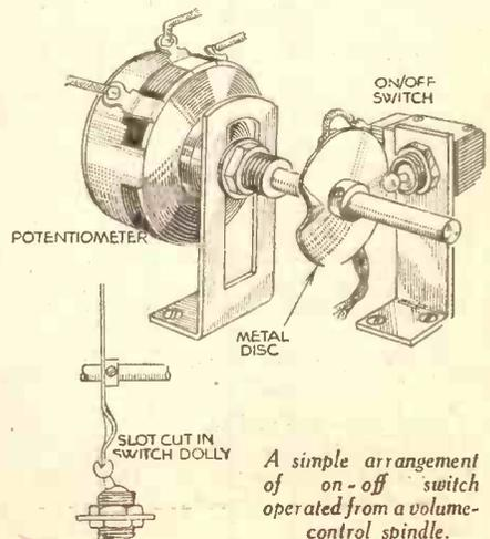
A simple arrangement of on-off switch operated from a volume-control spindle.
