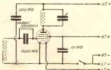
Fig. 2.—A slight modification of Fig. 1, known as the T.N.T. circuit. The grid coil is untuned.
