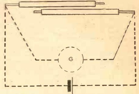
Fig. 1.—Two parallel wires form a small condenser, which can be charged and discharged.
