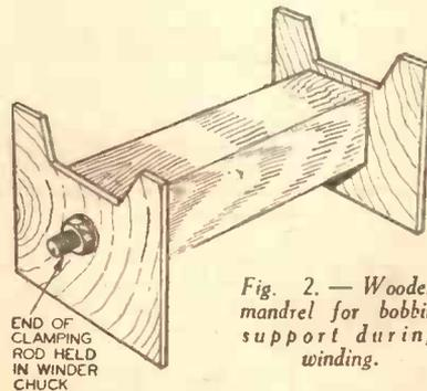
Fig. 2.—Wooden mandrel for bobbin support during winding.
