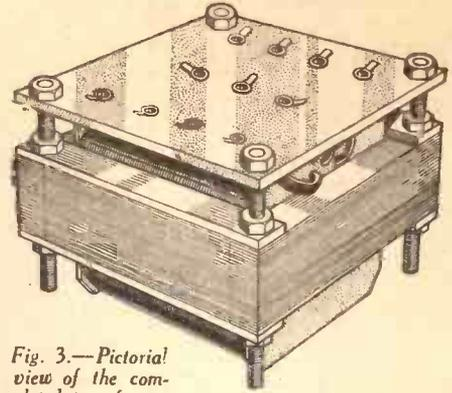
Fig. 3.—Pictorial view of the completed transformer.
