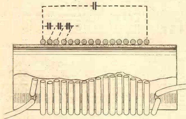
Fig. 2.—Capacity between adjacent turns of a coil is equivalent to connecting a small condenser in parallel with the winding.
