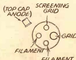
Fig. 4 (right). Connections to the valve-holder of the S.G. valve.
