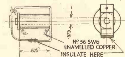
Fig. 2.—Constructional details of the relay.
