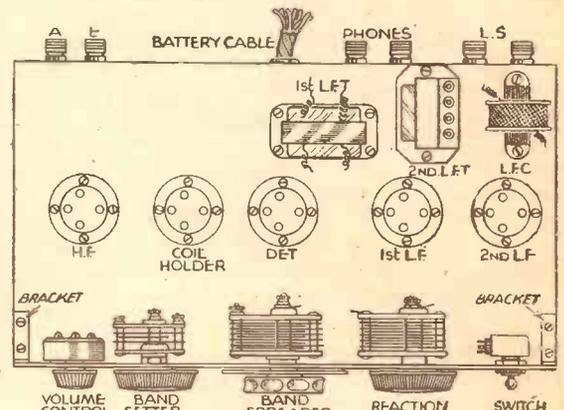
Fig. 2.—A suggested layout for the 4-valver.
