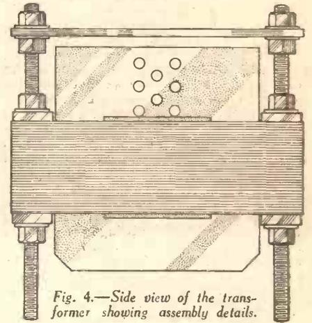
Fig. 4.—Side view of the transformer showing assembly details.
