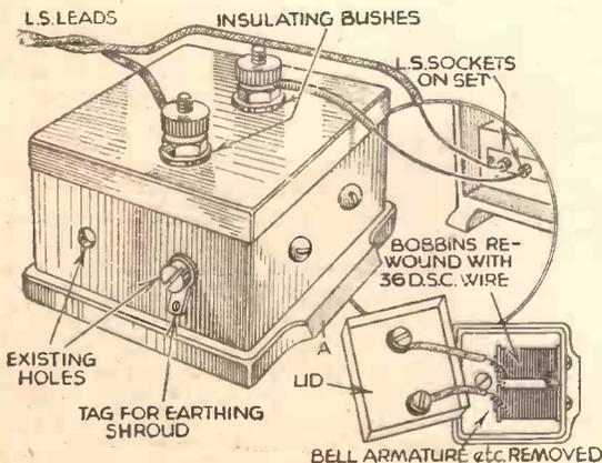
A useful output H.F. filter unit can be made as shown here.
