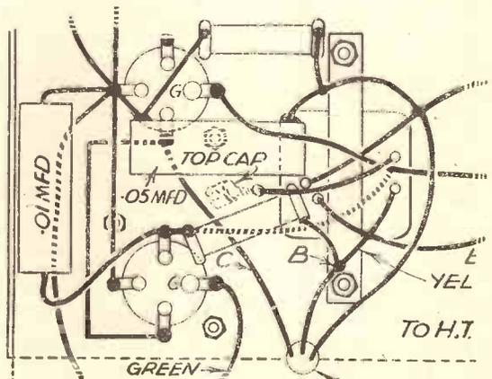
Fig. 2.—How the original wiring is altered to adopt the circuit shown in Fig. 1.
