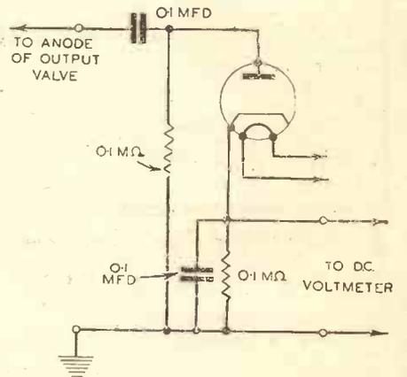
Fig. 7.—A successful output meter rectifier using a diode valve.
