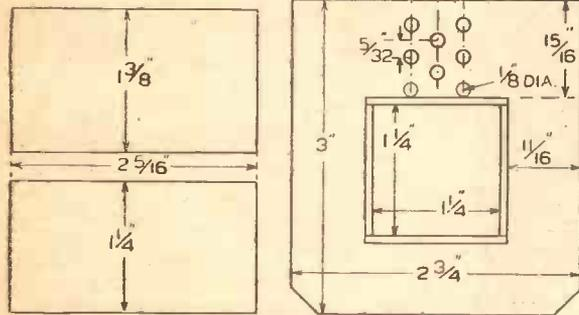
Fig. 1.—The end cheeks and core strips for the former.
