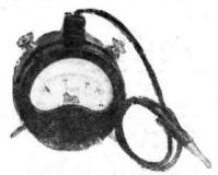
A simple 3-range tester such as is used by many listeners for general test purposes.
