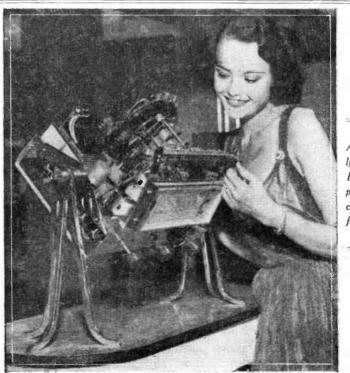
A visitor to Radiolympia inspecting an Ekco "Radio Brain" press-button set in chassis form. It has fifteen press-buttons.
