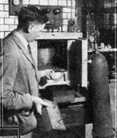
Fig. 2.-The perishability of rubber insulation is quickly gauged by accelerated life test to which it is subjected in the chamber of this humidity cabinet.
