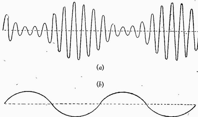
(a) Is a radio carrier wave of constant amplitude; and (b) is a programme or audio wave for modulating (a).
