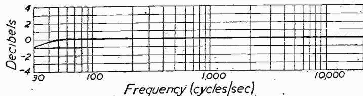
Fig. 1.—Response curve (practically "straight line") for a high-fidelity amplifier.
