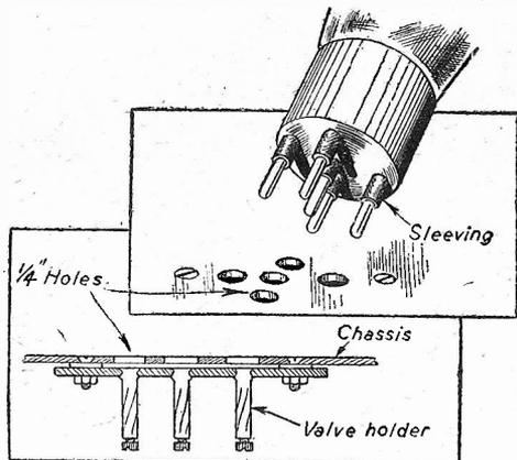
A novel method of fitting sub-chassis valveholders
