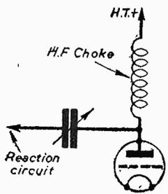
Fig. 3.—The standard reaction H.F. choke.
