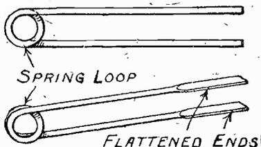
A handy pair of tweezers made from a piece of springy wire.
