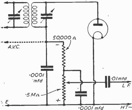
Fig. 4.—A more practical form of the circuit shown in Fig. 3. It includes an H.F. filter.
