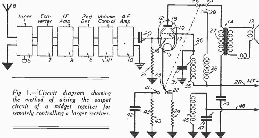
Fig. 1.—Circuit diagram showing the method of wiring the output circuit of a midget receiver for remotely controlling a larger receiver.
