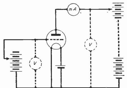
Fig. 3.—How a triode is connected for taking anode volts, anode current and grid volts figures for drawing curves of the kinds illustrated in Figs 4 and 5.
