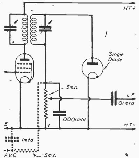
Fig. 3.—A very simple method of obtaining A.V.C. (see broken lines) when using a single diode for second detection.
