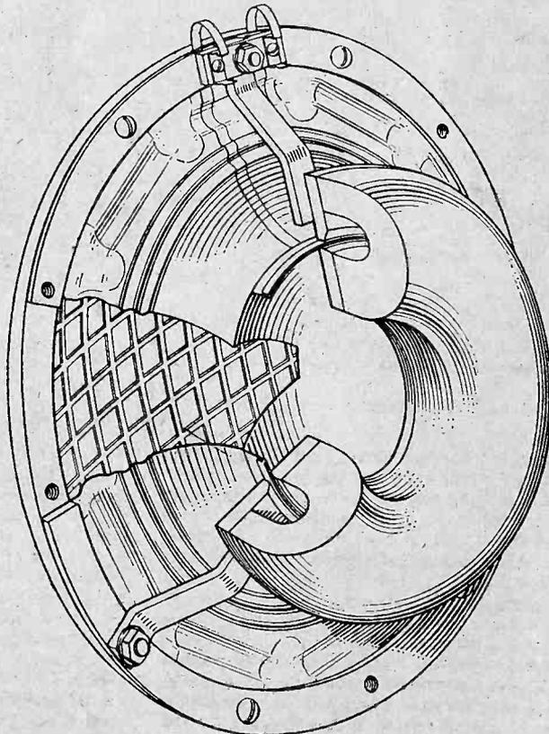
Fig. 2.—The driving coil vibrates in a narrow slot in the ring-shaped field magnet.
