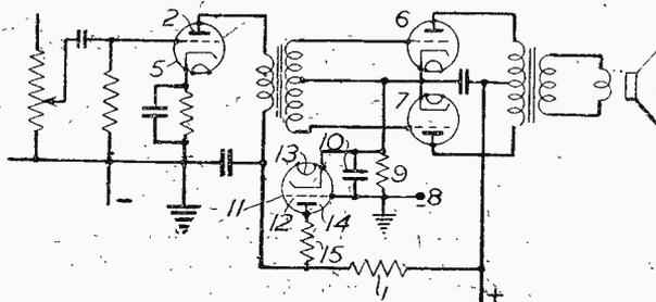
Fig. 4.—Circuit diagram of an output amplifier stage.
