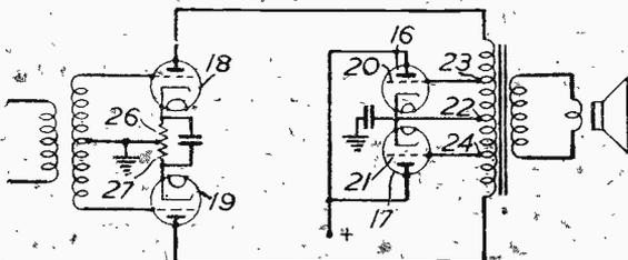
Fig. 5.—An automatically-operated output circuit.
