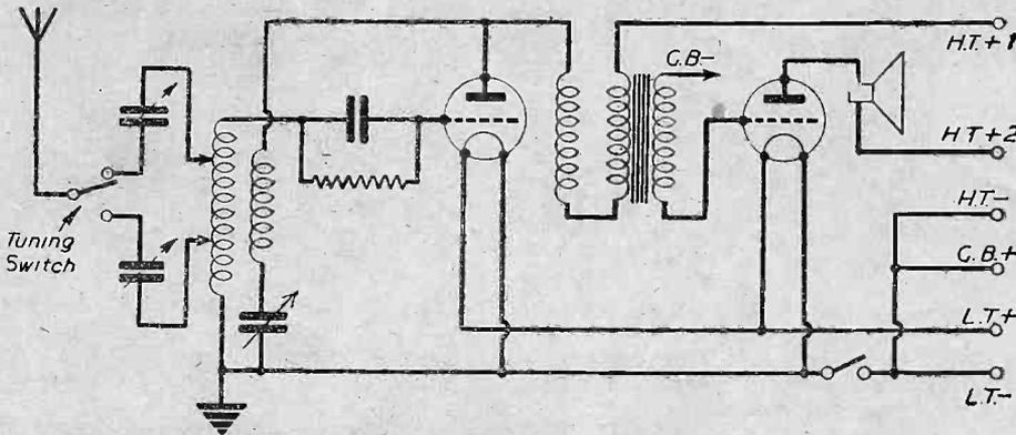
Circuit diagram of A. W. Jump's two-valver.
