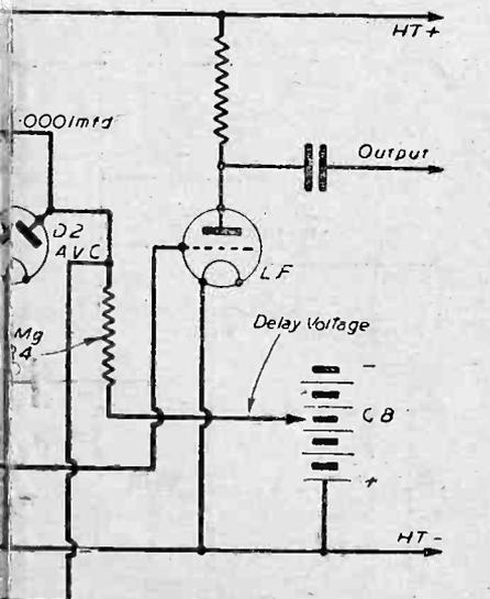
Fig. 5.—A delayed A.V.C. circuit in which the amplification provided by the L.F. pentode is controlled to a certain extent at the same time as pre-detector stages are controlled. "Normal" bias is obtained across R6, additional bias being provided by the A.V.C. section of the D.D.T.
