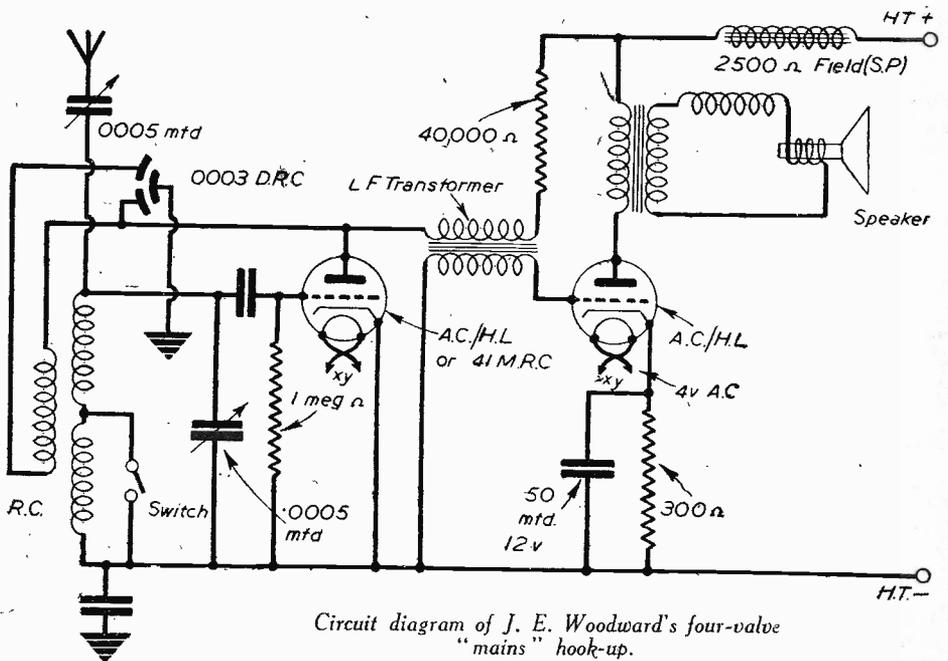
Circuit diagram of J. E. Woodward's four-valve "mains" hook-up.
