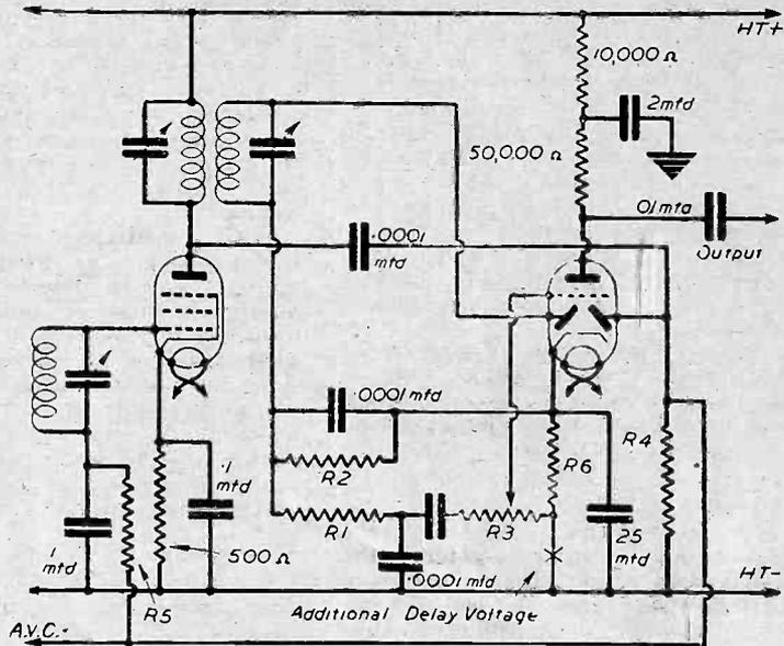
Fig. 6.—An arrangement similar in principle to that shown in Fig. 5, but using mains valves and a double-diode triode for second detection, A.V.C. and L.F. amplification.
