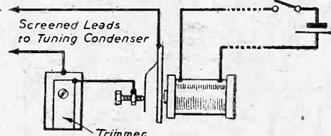
A simple remote control switching device.
