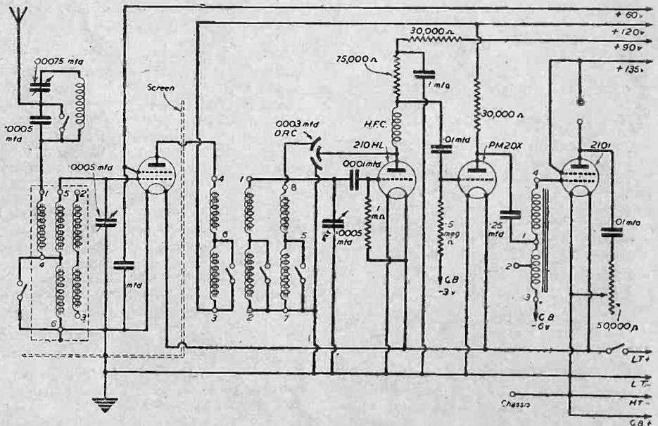
This is the circuit diagram of J. Robinson's four-valve set.
