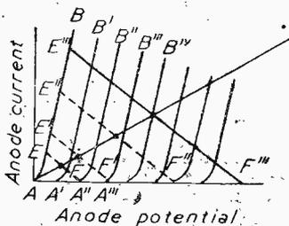
Fig. 1.—(Left) Anode current-potential curve.
