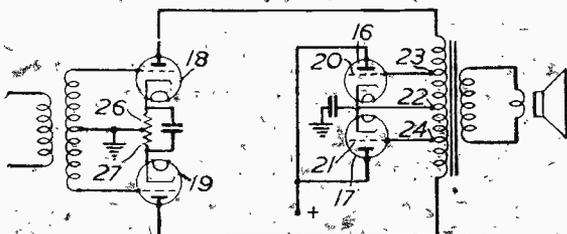
Fig. 5.—An automatically-operated output circuit.
