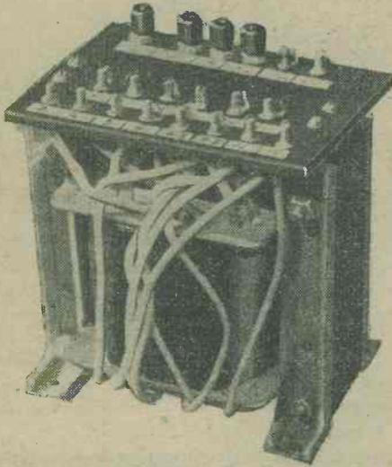
The completed component, showing how the tapping leads are taken to the terminal board.
