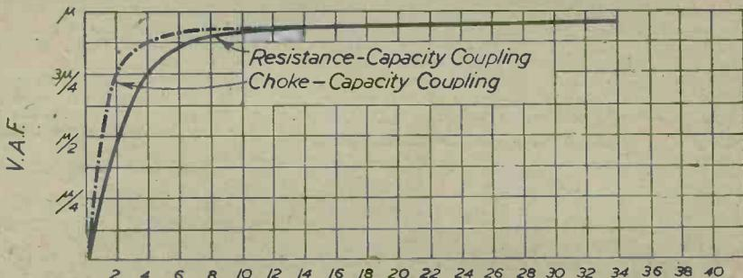
Fig. 3.—Curves which show how the amplification  $R/R_a$  provided by a valve varies with the resistance or reactance of the anode load.
