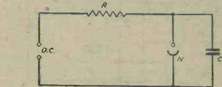
Fig. 12.—A simple electrically controlled oscillator using a neon lamp.
