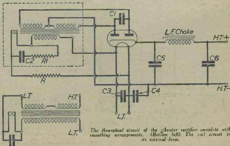
The theoretical circuit of the vibrator rectifier complete with smoothing arrangements. (Bottom left) The coil circuit in its original form.
