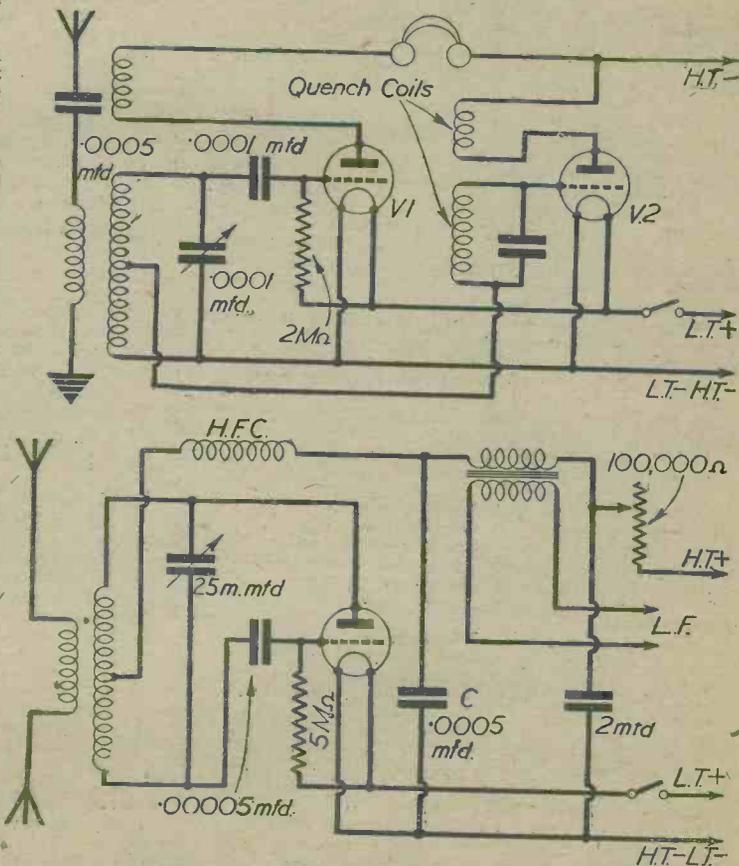
Two super-regenerative circuits. In the top circuit a separate quenching valve is used; this circuit resembles the original Armstrong super-regenerative circuit and is nowadays regarded as obsolete.
