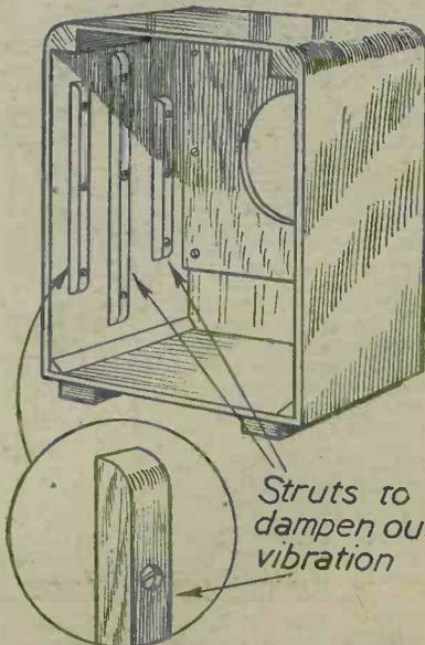
Struts to dampen out vibration
