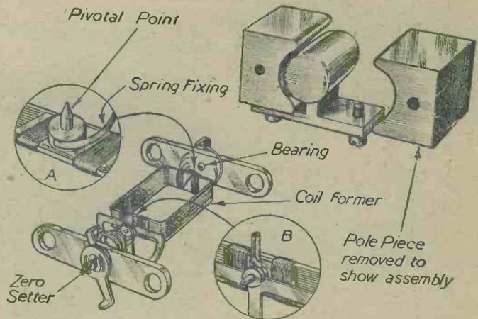
A. How the pivot point plate is bound to coil former. B. Shows the pointer holder and part of counter-balance.
