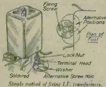
such a manner that the leads from the latter could be connected to components above and below chassis easily, and also to allow of easy removal of the transformers when necessary. The sketches show how simple feet were added to the fixing shanks of the transformers to allow of this. Large copper washers were used for the feet, to which were soldered terminal heads as shown, the height from the chassis and position of feet being fixed by lock nuts.—R. L. GRAPER (Chelmsford).
