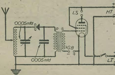
Fig. 1.—A normal crystal detector circuit followed by a pentode L.F. stage. A good set for reception of the local transmission, but a high degree of selectivity must not be expected.
