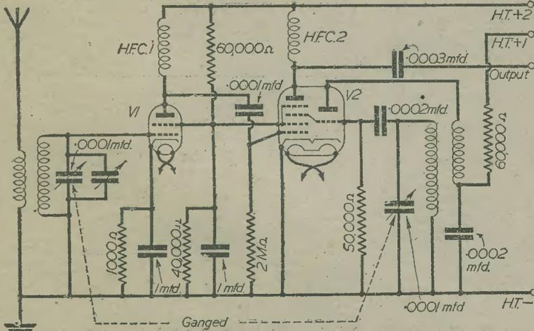
Fig. 15.—An efficient S.W. Converter for A.C. mains. It is known as the W.M. A.C. Short-wave Converter, blueprint No. W.M. 408.
