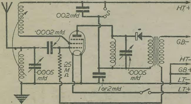
Fig. 1.—The circuit of a pentode-crystal combination in which the valve acts as an H.F. and L.F. amplifier.
