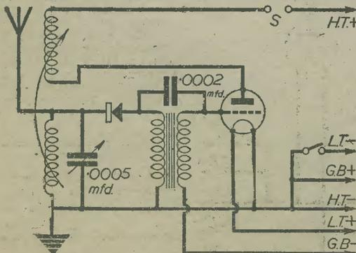
Fig. 2.—A suggested circuit using valve and crystal; the former acting as L.F. amplifier
