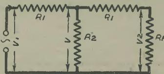
Fig. 4.—An arrangement to show how *K*—the attenuation ratio—is obtained.
