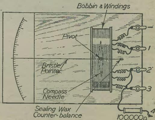
Fig. 2.—A plan of the instrument. Note the location of the compass needle, the pointer and scale.
