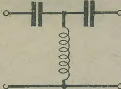
Fig. 9. - A high-pass filter arrangement.
