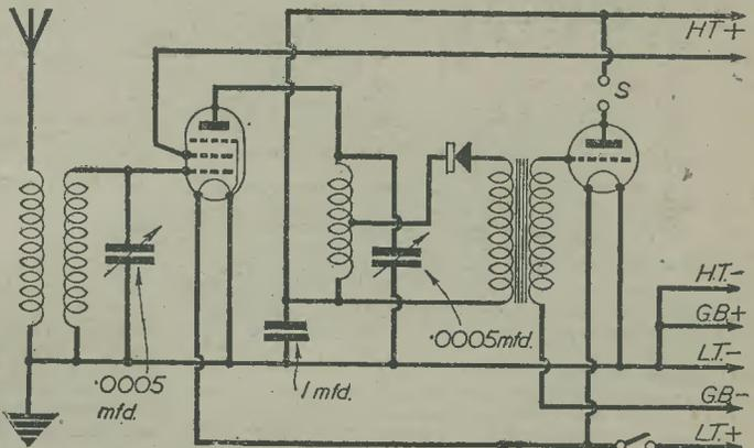
Fig. 5.—An H.F. plus detector plus L.F. stage circuit which should give good volume and quality.
