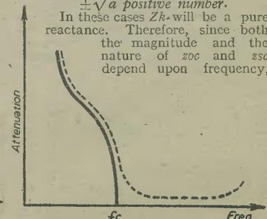
Fig. 10. - The curve produced by a well designed high-pass filter.
