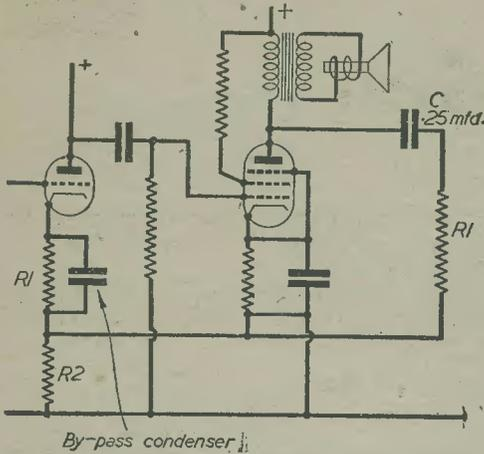
Fig. 3.—An improved version of Fig. 2. Both sides of the potentiometer can now be varied.
