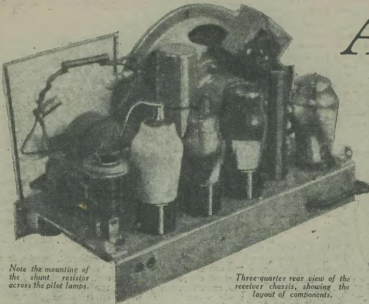
Note the mounting of the shunt resistor across the pilot lamps.
