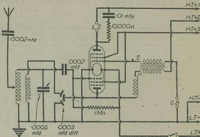
Fig. 4.—The two pentode sections of a Q.P.P. valve are used in this circuit as detector and L.F. stage.
