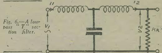
Fig. 6. - A low-pass "T" section filter.
