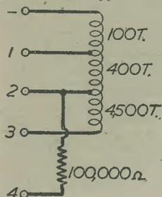
Fig. 1.—Shows the winding data and how the tapping points and resistor are connected.
