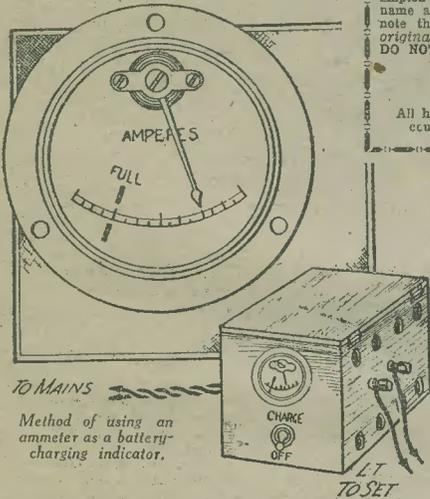
Method of using an ammeter as a battery-charging indicator.
