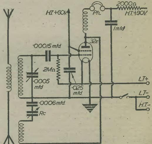
Circuit diagram of D. Melville's one-valve short-wave set.
