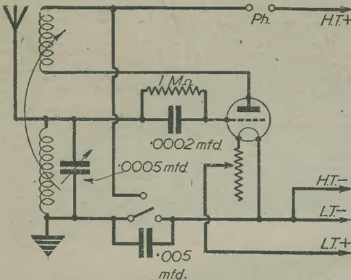
Fig. 4.—This arrangement is based on the "Flewellyn" circuit, and calls for special care in use.
