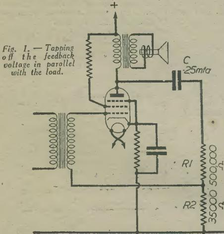
Fig. 1.—Tapping off the feedback voltage in parallel with the load.
