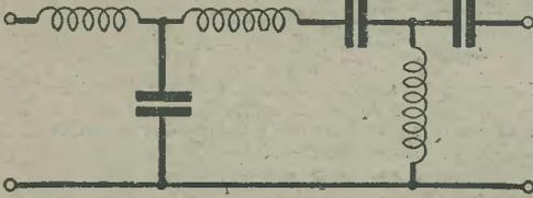
termination is correctly adjusted, the impedance of the circuit at all frequencies below a certain critical frequency is more or less constant, above the critical frequency the impedance goes up very rapidly. This circuit is a "Low-pass" filter, since it passes without attenuation (ideally) all frequencies below a critical—cut-off—frequency.
