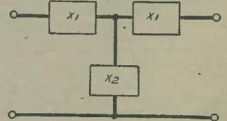
Fig. 5.—A "T" section filter in which *X*<sub>1</sub> and *X*<sub>2</sub> represent reactors of opposite kind.
