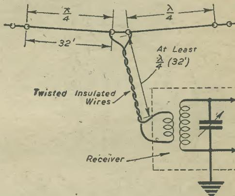
Fig. 5.—(Right) One of the best types of general purpose aerial systems. It will give good results on both medium and short waves.
