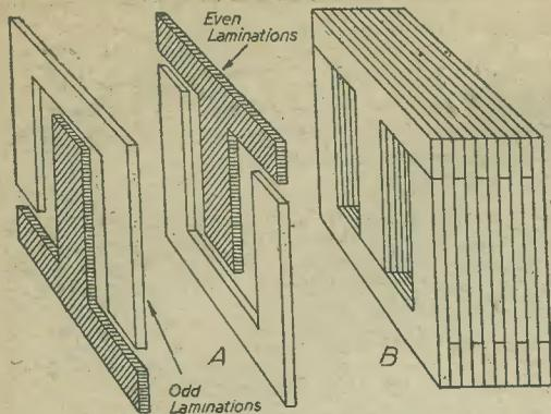
Fig. 5.—Method of interleaving stampings.
