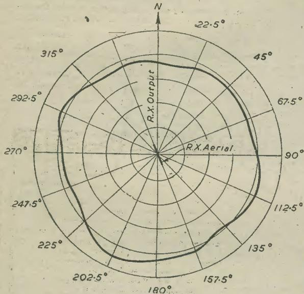
Fig. 1.—A polar diagram, showing the relative pick-up by a receiving aerial from various points.
