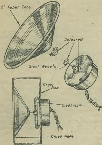
An efficient midget speaker made with an earphone.
