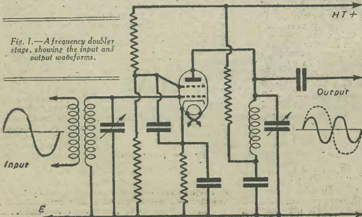
Fig. 1.—A frequency doubler stage, showing the input and output waveforms.
