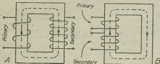
Fig. 1.—Core-type construction.
