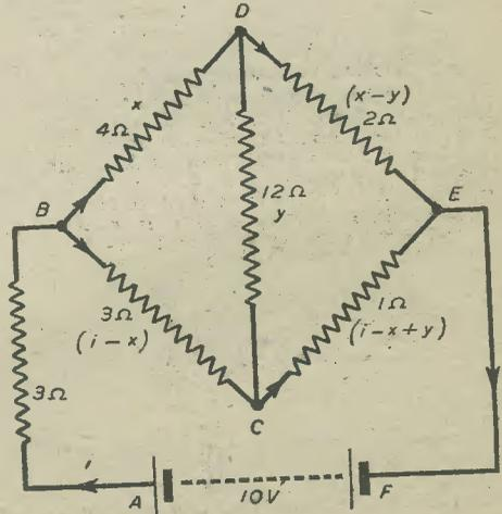
Fig. 5.—An example in which the battery has an internal resistance of 3 ohms.
