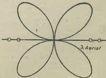
Fig. 3.—Polar diagram of full-wave aerial.
