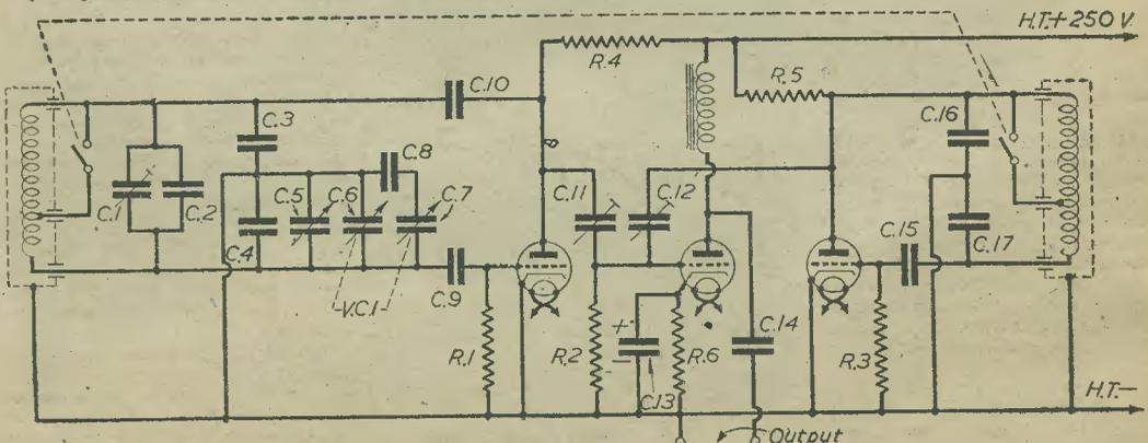
Fig. 3.—Circuit diagram of the beat-frequency oscillator; C1 .0003 mfd. preset; C2, C3 and C4, .0005 mfd. fixed; C5, .00005 mfd. set zero; VC1 (C6, C7, C8) .0007 mfd.; C6, C7, .0005 mfd. ganged; C8, .0003 mfd. fixed; C9, C15, .0001 mfd. fixed; C10, .01 mfd.; C11, C12, 10 mmsfd. preset (see text); C13, 25 mfd. 25 v. fixed; C14, 2 mfd.; C16, C17, .002 mfd.; R1, R2, R3, 1.0MΩ; R4, R5, R6 depend on valve used (see text).
