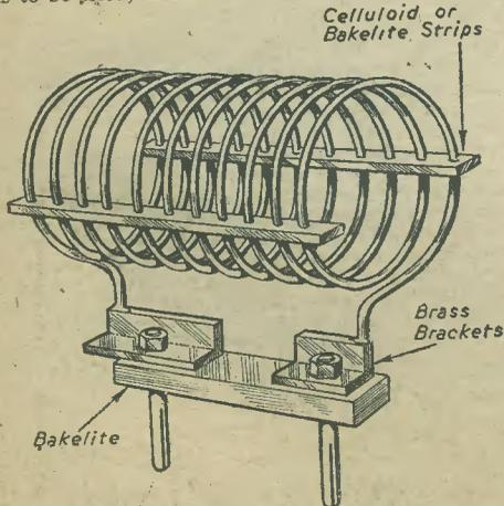
An air-spaced coil of 16-gauge wire, wound double, and threaded through bakelite supporting strips.
