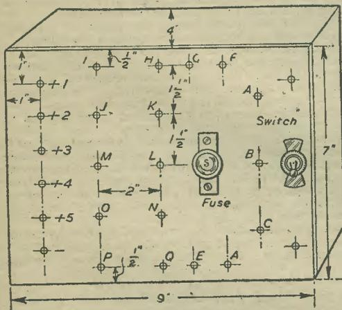
Fig. 5.—Layout and drilling template of the panel. Dimensions of a suitable case are also shown.
