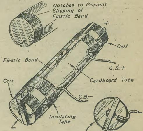
A novel dodge for using a torch battery for grid bias.
