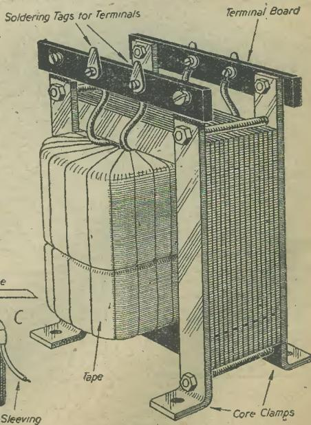
Fig. 7.—Typical shell type transformer.
