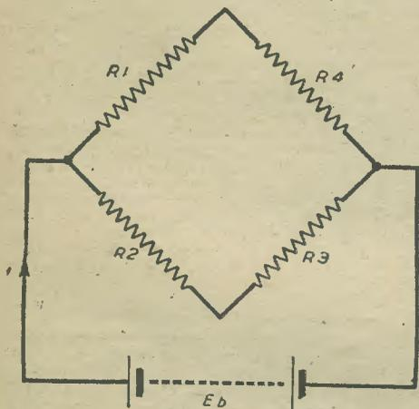
Fig. 1.—A simple series-parallel circuit, involving only an application of Ohm's Law.
