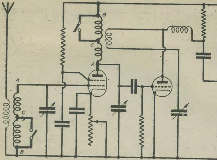
Fig. 4.—Windings and connections to be retained using two typical coils.
