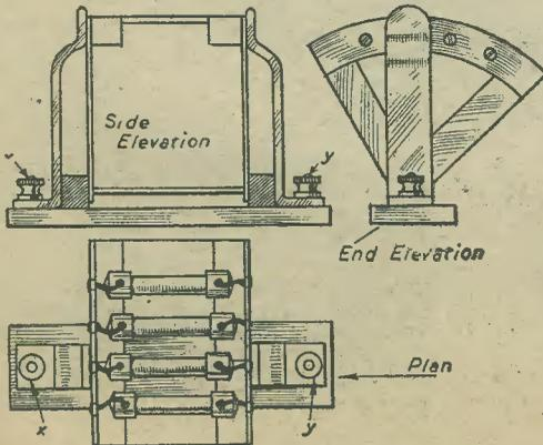
A simple method of making quick connections.
