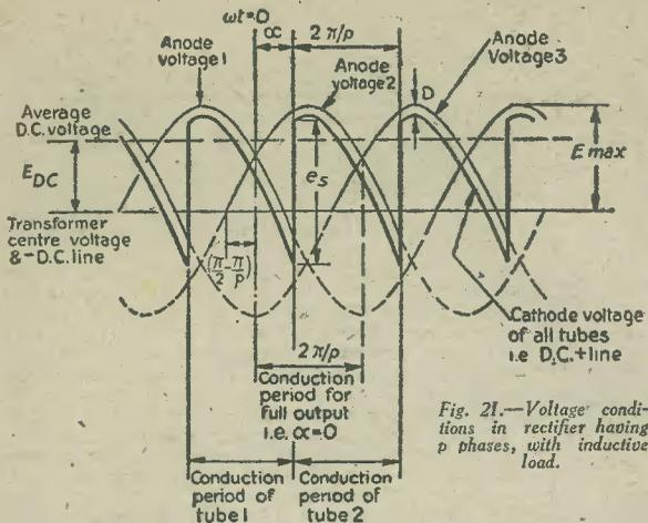
Fig. 21.—Voltage conditions in rectifier having  $p$  phases, with inductive load.
