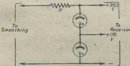
Fig. 3.—Two stabilisers in series for higher voltage; a tapping is provided for an intermediate voltage.
