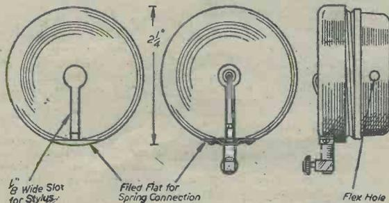
Fig. 1.—Showing how the earphone cover is filed, with front and side views of finished piece.
