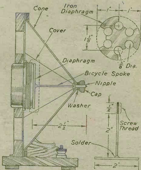
Fig. 3.—Sectional side view, with details of sheet iron diaphragm.
