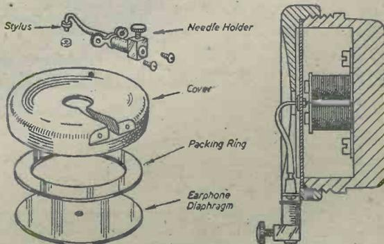
Fig. 2.—Assembly of parts, and sectional view.
