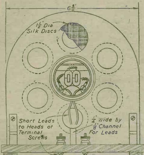
Fig. 2.—A back elevation, showing earphone piece in position and groove to be cut for flex wires.
