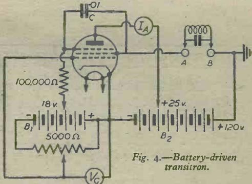
Fig. 4.—Battery-driven transitron.
