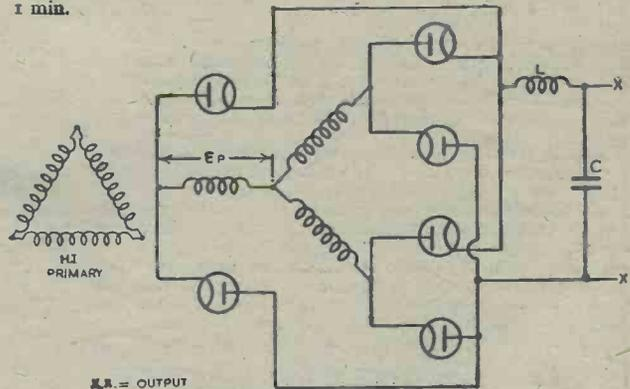
Fig. 6.—Three-phase full-wave rectification.
