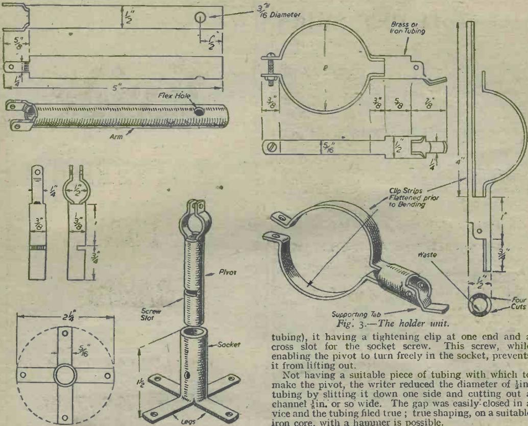
Fig. 4.—Details of arm piece, pivot and socket.
