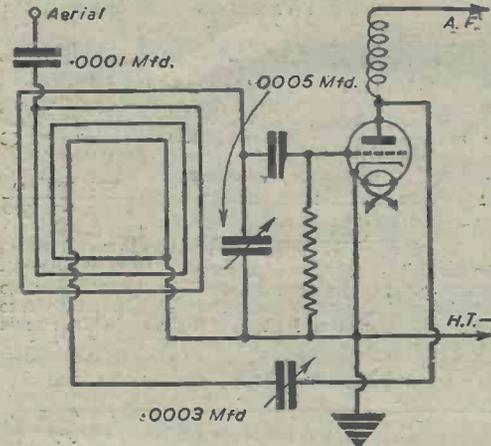
Fig. 6.—How a frame may be used with a Det. L.F. receiver with reaction.
