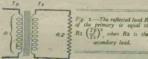
Fig. 1.—The reflected load R of the primary is equal to  $R_2 \left(\frac{T_p}{T_s}\right)^2$ , when R2 is the secondary load.
