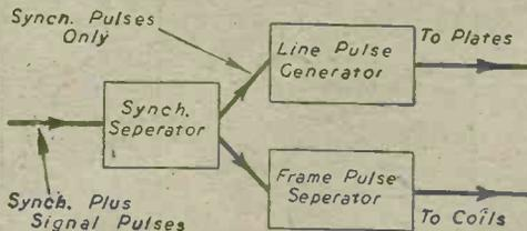
Fig. 16.—Block diagram of the synch. signal, line and frame separator systems.
