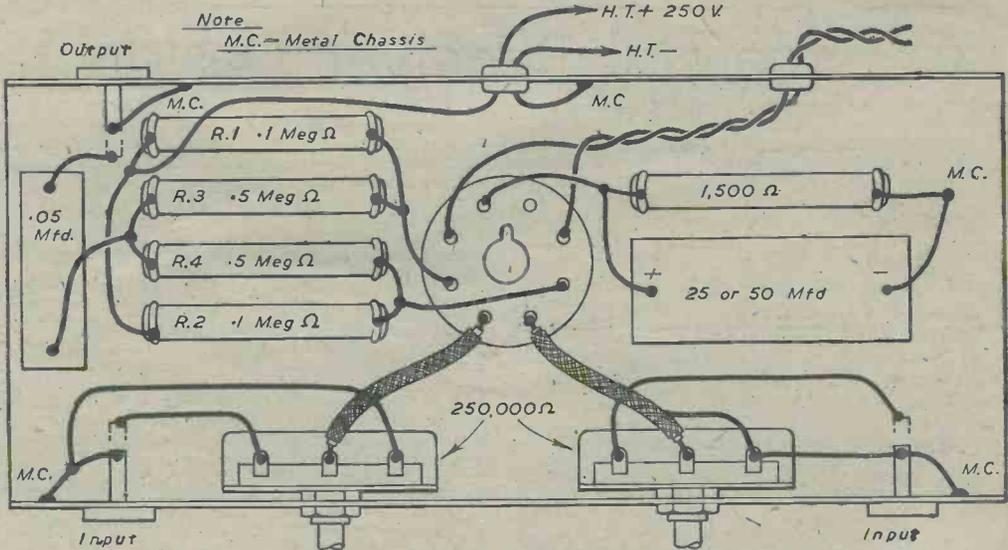
Fig. 3.—The layout and wiring of a two-channel mixer using a 6NT6 valve.
