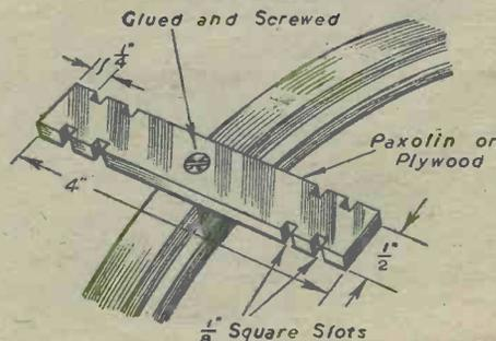
The detail shows the method of supporting the windings.
