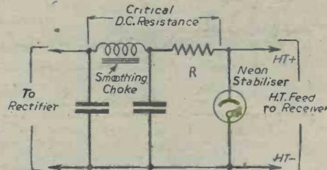
Fig. 2.—The connections for a neon voltage stabiliser. The resistance R is a protective device for the stabiliser and also acts as a ballast.
