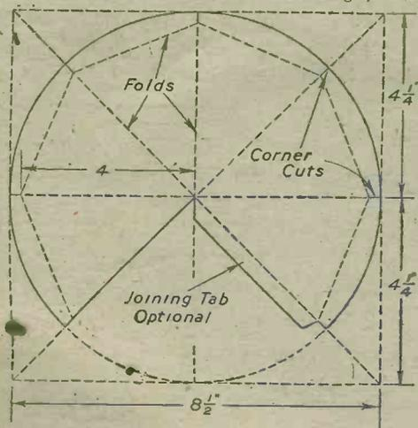
Fig. 4.—Layout of paper pattern which forms the cone.
