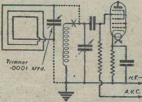
Fig. 5.—The method of connecting a frame to a superhet or an H.F.-Det.-L.F. receiver with ganged tuning.
