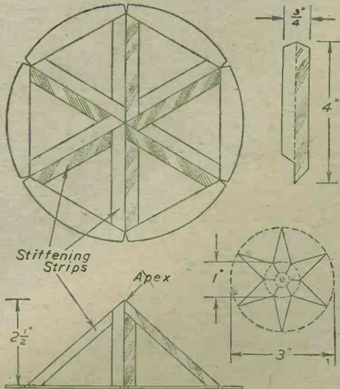
Fig. 5.—Top plan of cone, with side view, showing how stiffening strips are attached, with sizes of strips and apex star.
