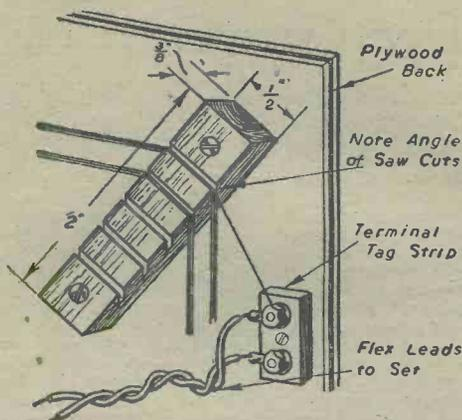
Fig. 3.—A simple form of construction for a frame aerial fitted to the back board of the receiver cabinet.
