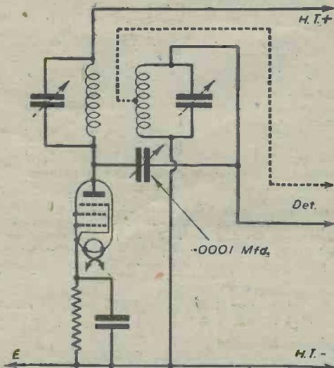
Fig. 1.—Variable-selectivity I.F. by using "top capacity" variable coupling and a means of increasing selectivity by taking the "detector" lead from a centre tap instead of from the end of the I.F. transformer secondary.
