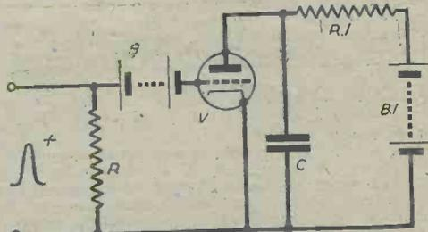
Fig. 12.—A simple saw-tooth generator triggered by positive synchronising pulses.
