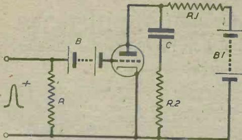
Fig. 14.—A circuit suitable for producing a voltage wave of the shape shown in Fig. 13 (c).
