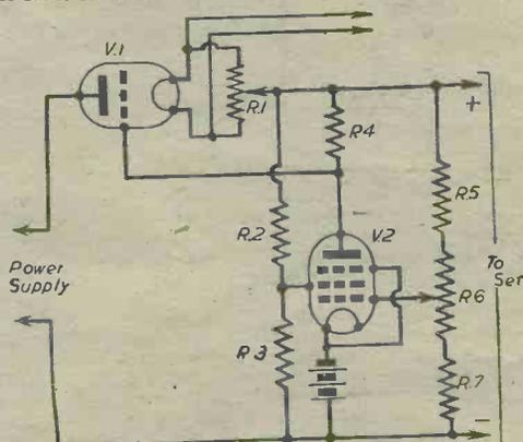
Fig. 6.—A voltage-stabiliser circuit which gives a very good range of control. The components shown are: V.1, triode of high anode current rating; V.2, pentode control valve; R.1, "humdinger"; R.2 and R.3, screening grid potentiometer; R.4, pentode anode load; R.5, R.6, and R.7, control grid potentiometer.
