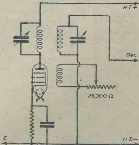
Fig. 2.—Variable I.F. selectivity by using a third winding of few turns with a 25,000 ohm variable resistor in parallel.
