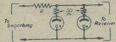
Fig. 4.—Increased current variation can be dealt with by connecting stabilisers in parallel as shown.
