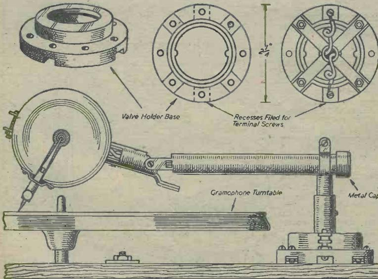
Fig. 5.—Side elevation of the pick-up, with details of socket base.
