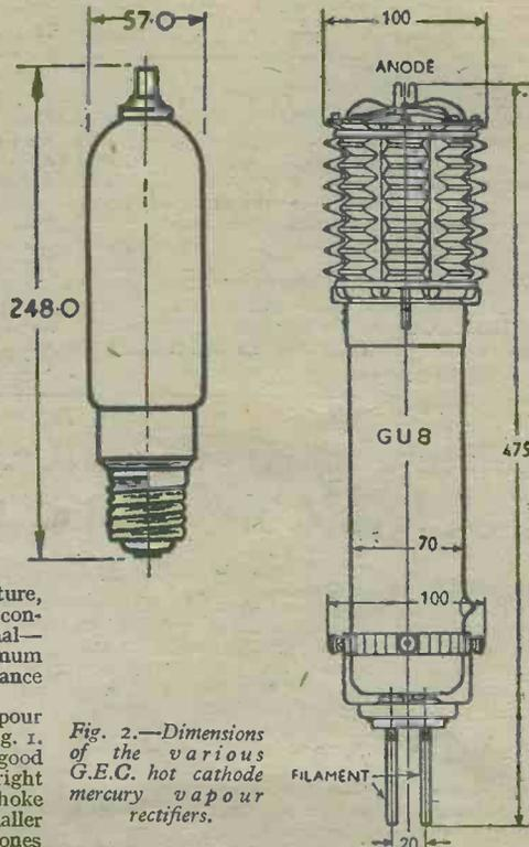
Fig. 2.—Dimensions of the various G.E.C. hot cathode mercury vapour rectifiers.
