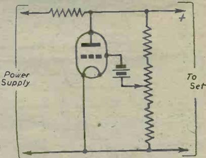
Fig. 5.—A triode valve used as a voltage regulator.
