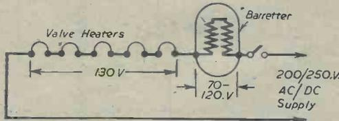
Fig. 1.—How a barretter is used to regulate the current passed by the heaters of an A.C./D.C. receiver intended for use on mains voltages between 200 and 250. The voltage figures given are representative values added for the purpose of giving an example.
