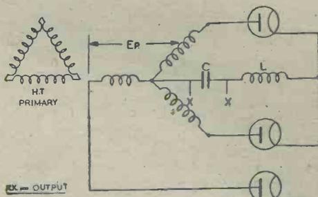
Fig. 5.—Three-phase half-wave rectification.
