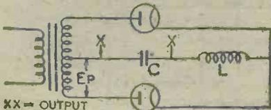
Fig. 3.—One application of the mercury vapour rectifier—biphase half-wave rectification.
