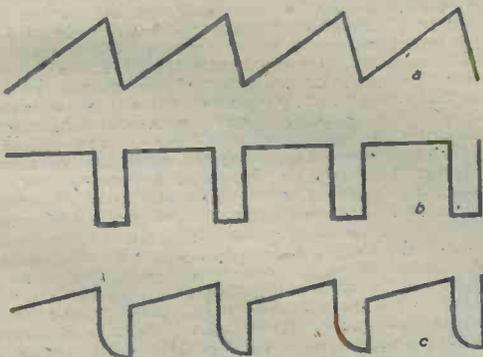
Fig. 13.—Voltage waves which must be applied to (a) resistance only, (b) inductance only, (c) resistance and inductance in order to produce a pure saw-tooth current wave.
