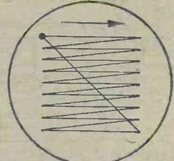
Fig. 15.—Exaggerated diagram depicting a spot tracing out an area by a series of lines.
