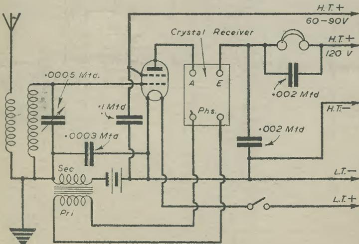
Fig. 11.—A simple reflex circuit.
