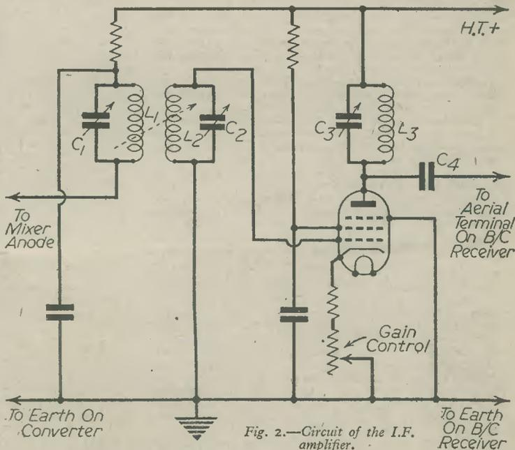
Fig. 2.—Circuit of the I.F. amplifier.
