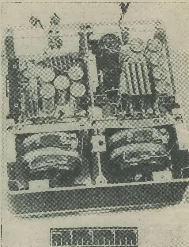
Fig. 7.—R.F. section of latest S.W. transmitter FuG. 10. Note the use of "straw" type condensers.
