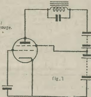
Fig. 1 shows the most interesting component of this new device, the coil to be tested having to be placed over the stack of laminations. The wire is wound on a bobbin with presspahn flanges to keep it snug. Insulated wedges assure rigidity. Fig. 2 shows the basic circuit of the dynatron oscillator.
