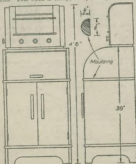
Fig. 1.—A front and side elevation, with receiver in position.
