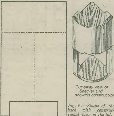
Fig. 6.—Shape of the back with constructional view of the lid.
