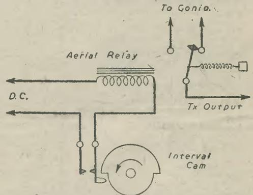
Fig. 12.—The interval cam runs at half the speed of the identification cam, connecting the transmitter output first to one aerial and then to the other while the two-letter identification is sent out. In practice, the contacts of all three cams are interconnected and the cams are operated through a somewhat complex system of gears.
