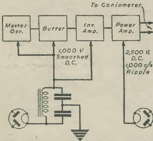
Fig. 4.—Block diagram of a representative radio range transmitter. Audio modulation is obtained from the 1,000 c/s. ripple on the H.T. supply to the power amplifier.
