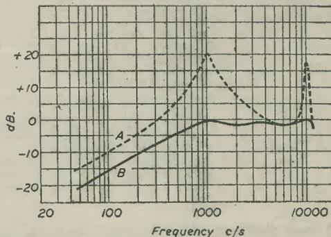
Fig. 2.—Frequency response of damped and undamped cutting-head. A is without viscoloid damping block, and B is with damping block inserted.
