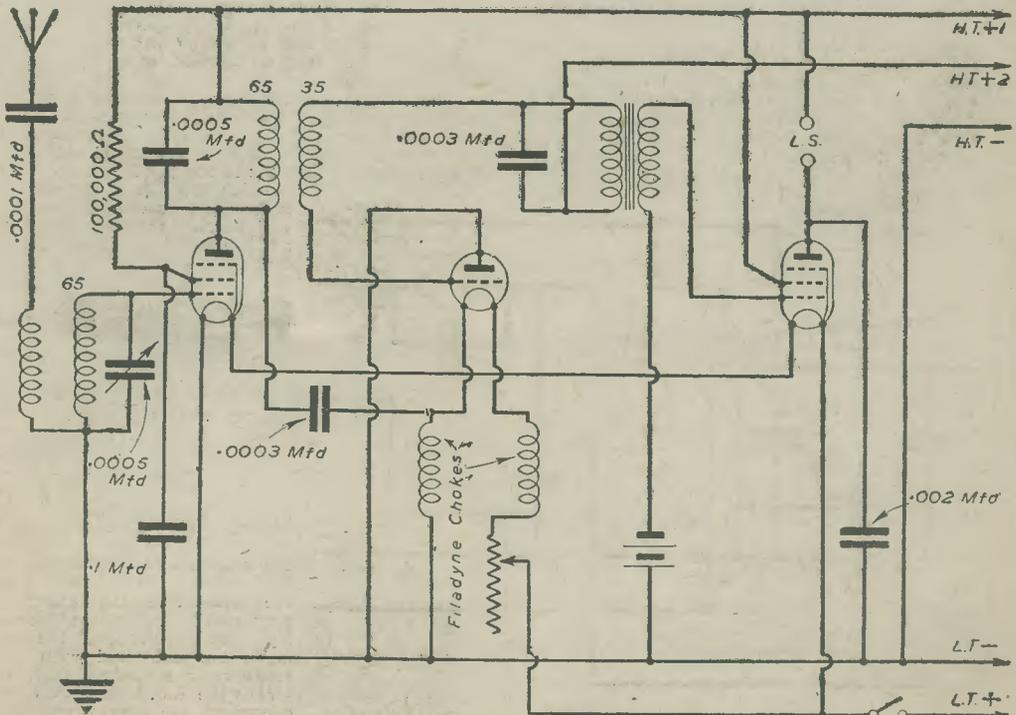
Fig. 8.—An interesting modification of the Filadyne circuit.
