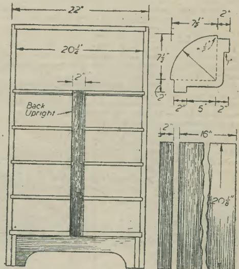
Fig. 4.—A back view of the carcass, with details of the lid.
