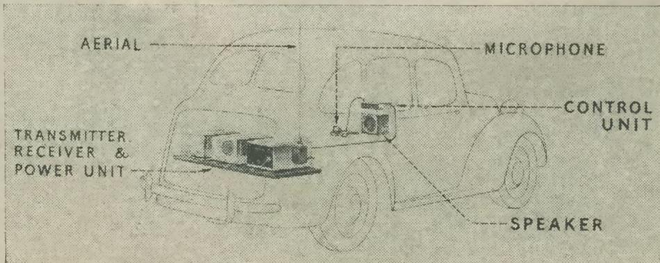
Diagram showing the layout of the equipment in a patrol car.
