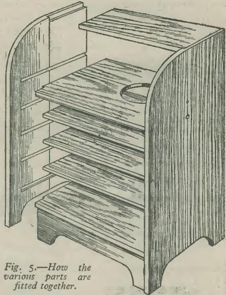
Fig. 5.—How the various parts are fitted together.
