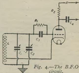
Fig. 4.—The B.F.O. circuit.
