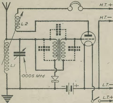
Fig. 12.—The Hale circuit.
