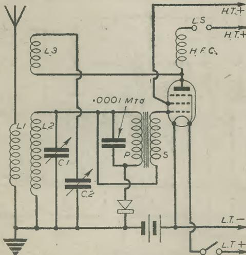
Fig. 13.—A modified Hale circuit.
