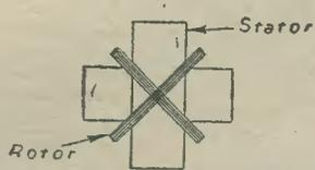
Fig. 7.—The theoretical radiation pattern from the crossed aerial loops when the stator and rotor windings of the goniometer are parallel to each other (gonio scale reading 360—0 degrees).
