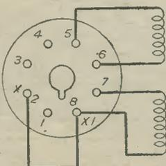
Figs. 1 and 2 (left). — The coil and details of connections to the coil pins. Fig. 3 (right). — Circuit showing how the lamp switching is effected.
