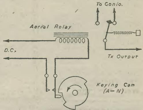
Fig. 10.—Diagrammatic representation of the action of the A N keying cam, which is used to operate a biased relay. This relay transfers the transmitter output from one aerial to the other, through the goniometer.
