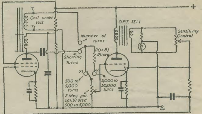
Fig. 4 depicts the simple circuit modifications necessary for approximating the position of the shorting turns. Constant values, not shown, are as for Fig. 3.
