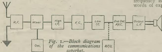
Fig. 1.—Block diagram of the communications superhet.
