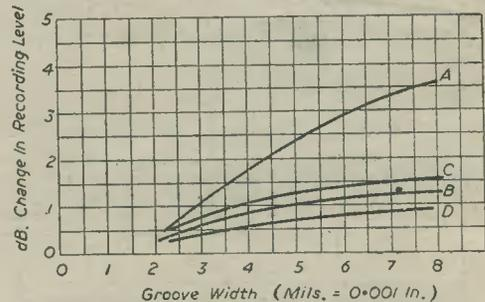
Fig. 4.—Change in recording level at 1,000 c/s, with groove width representing groove depth. A is inside of 33½ r.p.m. disc, sapphire stylus; B is outside of 78 r.p.m. 12in. disc, sapphire stylus; C is inside of 33½ r.p.m. disc, steel stylus; D is outside of 78 r.p.m. 12in. disc, steel stylus.
