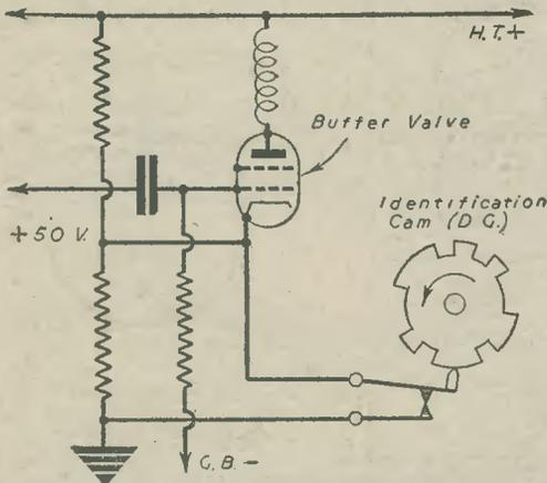
Fig. 11.—The identification cam, which automatically keys the transmitter with a two-letter call sign, operates a pair of contacts which open and close the bias circuit to the buffer valve connected between the R.F. oscillator and the intermediate amplifier stage.
