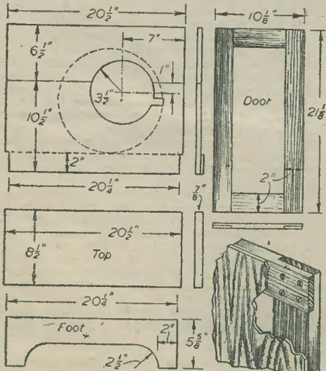
Fig. 3.—Size and shape of motor-board, top, foot and door-frame, with details of the door construction.
