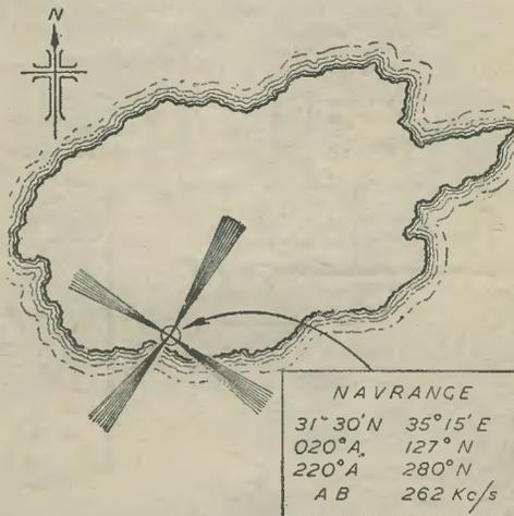
Fig. 2.—On a map showing radio navigational aids a typical radio range would be shown as illustrated here, where the radio range is a hypothetical one on an imaginary island in mid-Atlantic. The range is situated at an airfield called "Navrange," and operates on a frequency of 262 kc/s. with the identification letters AB. The "A" sectors are between 020 degrees—127 degrees and 220 degrees—280 degrees; the "N" sectors are between 127 degrees—220 degrees and 280 degrees—020 degrees.
