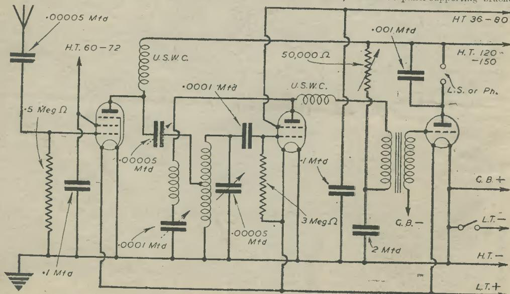
Fig. 1.—Theoretical circuit of the receiver.
