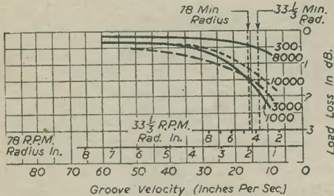
Fig. 3.—Shows cutting load loss, with R.C.A.MI-11850 head, and lacquer-coated disc.
