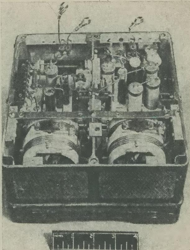
Fig. 6.—R.F. section of latest L.W. transmitter FuG. 10.
