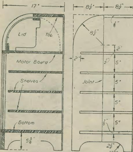
Fig. 2.—Sectional side view, with shape and size of one side, showing the position of the grooves or trenching for shelves, etc.
