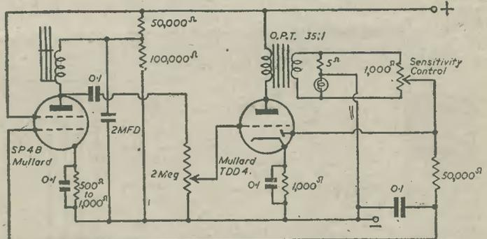
Fig. 3.—The complete circuit, including the amplifier. The exploring stack of laminations is shown in the anode circuit of the SP4B Mullard valve. Circuit constants should be adhered to. If other valves are used, cathode bias resistors must be correspondingly changed in values. Operating potentials are dependent upon the types of valves employed.
