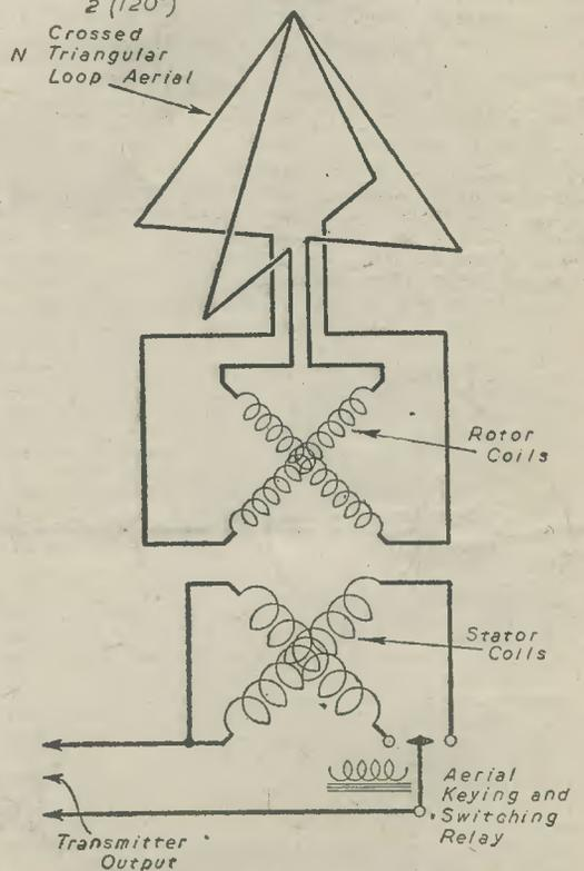
Fig. 6.—The arrangement of a Bellini-Tosi loop aerial system and associated radio-goniometer. The pair of stator and rotor coils are rigidly mounted at right-angles, while the rotor is free to rotate within the stator; a 360 degree scale is provided to indicate the position of the rotor.
