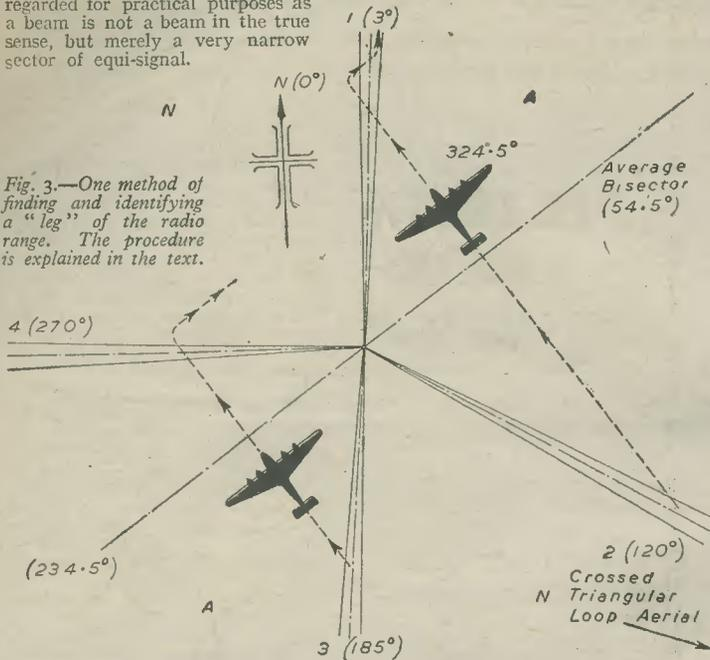
Fig. 3.—One method of finding and identifying a "leg" of the radio range. The procedure is explained in the text.
