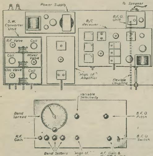
Fig. 3.—Suggested layout of the complete superhet.
