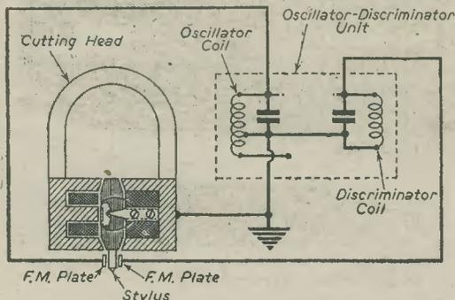
Fig. 1.—Arrangement of plates adjacent to stylus shank in F.M. calibrator for disc cutting-heads.
