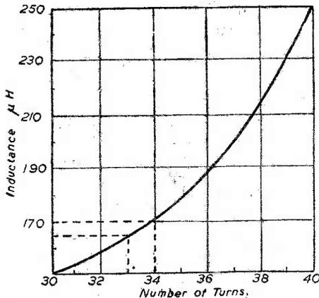
Fig. 5.—An example of inductance calculation.
