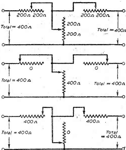
The circuit of the control at "full volume," "half volume" and "off."
