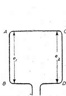
Fig. 1.—The simple loop aerial.
