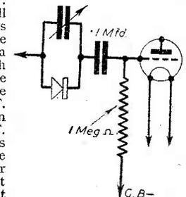
Fig. 20.—Another way of supplying grid-bias to the Crystadyne.
