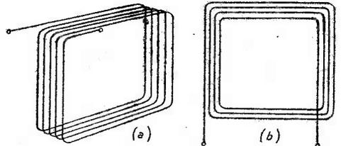
Fig. 3.—The box type (left) and pancake type aerials.
