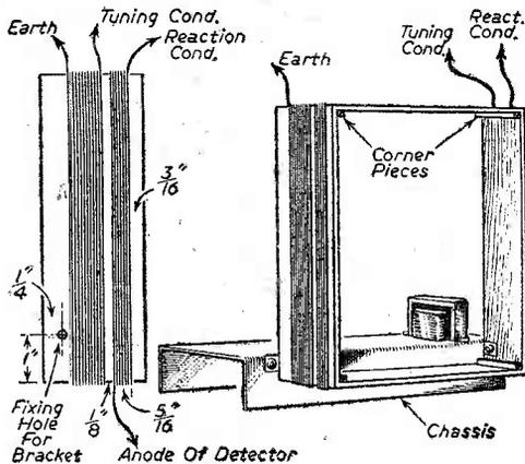
Fig. 2.—Details of the frame aerial.
